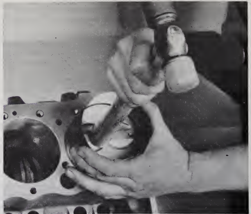
22.9 Gently tap on the top of the piston with a wooden hammer handle to insert the piston into the block
