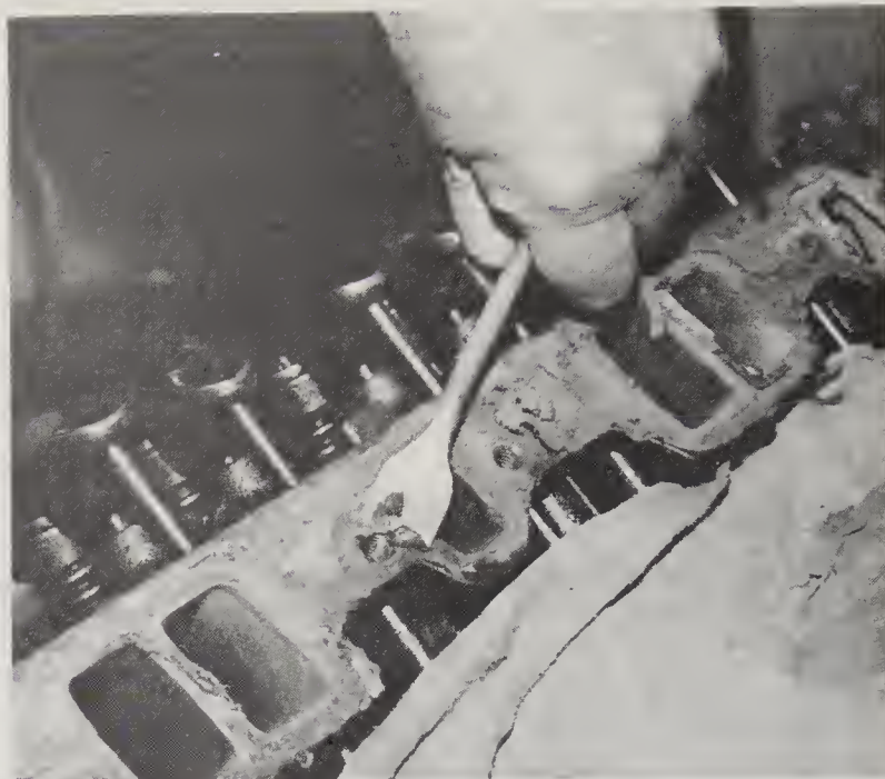
8.2 Use a gasket scraper to remove all traces of old gasket material and sealer from the head
