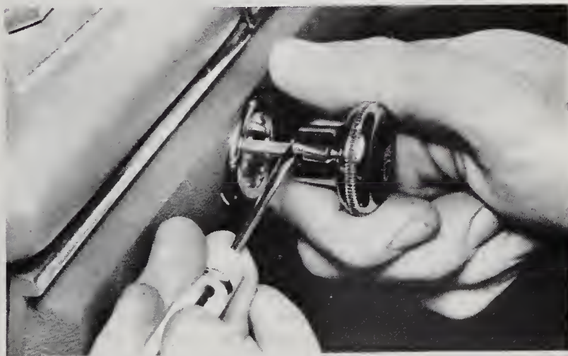
15.3 Remove the light switch knob by inserting a screwdriver into the slot and pressing in on the retaining clip while pulling the knob off the switch shaft
