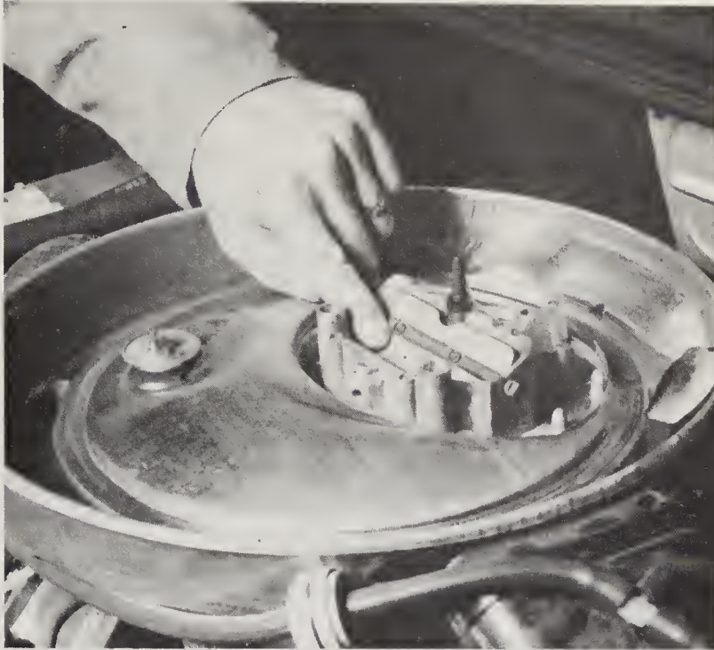
14.3 With the air cleaner top plate removed, the choke plate can be checked
