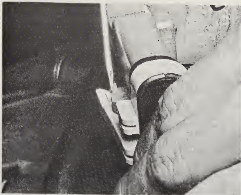
16.18 Disconnect the wiring harness from the distributor
