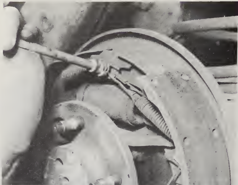
9.4/5 Use a spring removal tool to remove the primary and secondary shoe anchor springs
