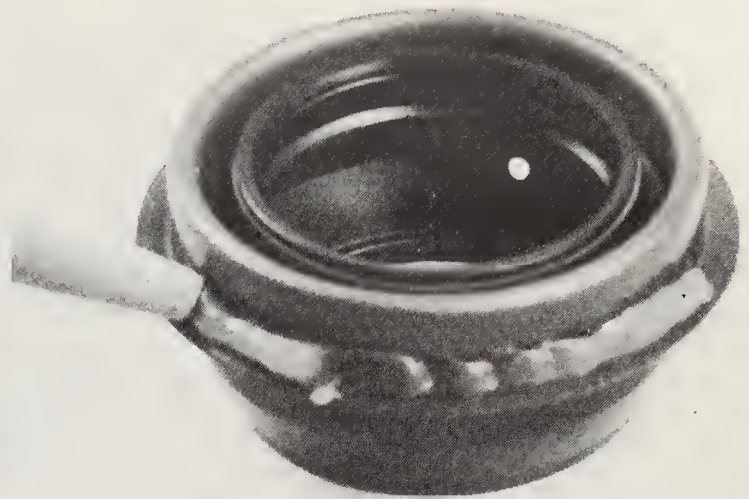
13.6 The outside perimeter of the new seal should receive a generous bead of silicone sealant
