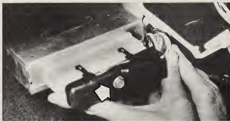
2.6 Remove the bolt (arrow) and unplug the connector from the ECA unit
