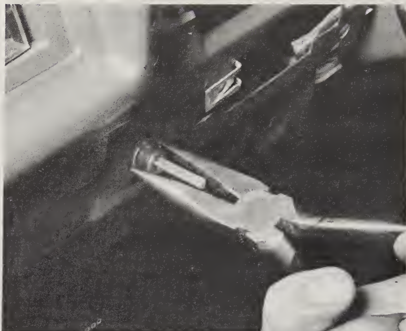
18.2 Remove the light switch retainer with a pair of needle nose pliers
