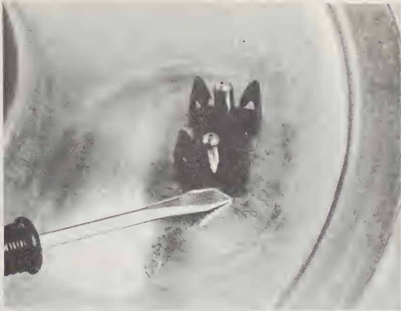
7.8 Thermactor control valve is replaced by prying off retaining clip
