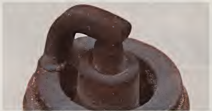
Carbon fouling. Dry, black, sooty deposits. Will cause weak spark and eventually misfire. Fault: over-rich fuel mixture. Check: carburetor mixture settings, float level and jet sizes; choke operation and cleanliness of air filter. Plugs can be re-used after cleaning
