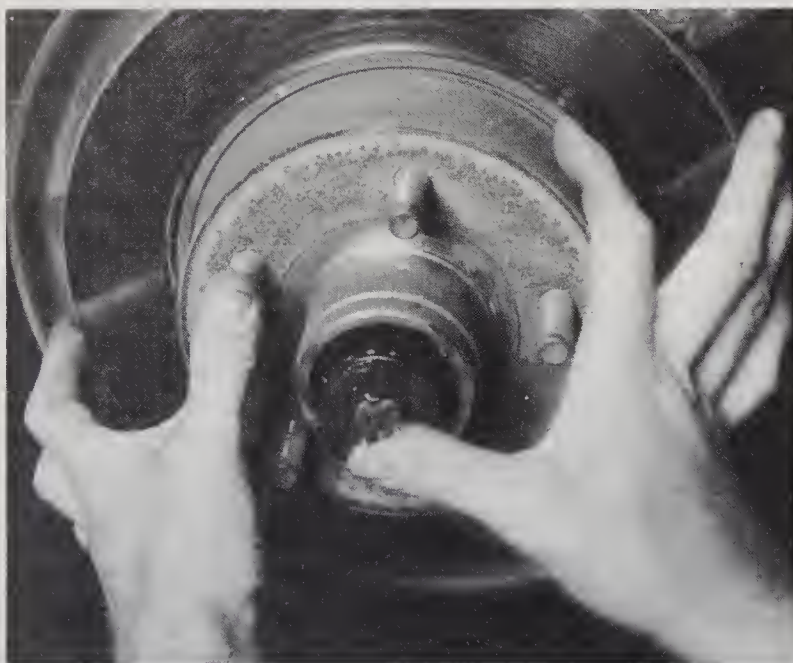
29.9 Pull out on the rotor to loosen the outer bearing
