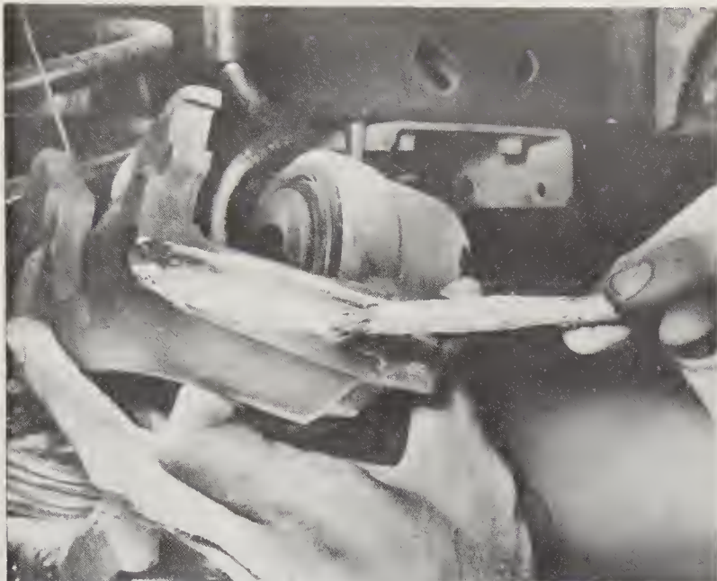
7.20 Lightly lubricate the V-grooves with white grease before assembly
