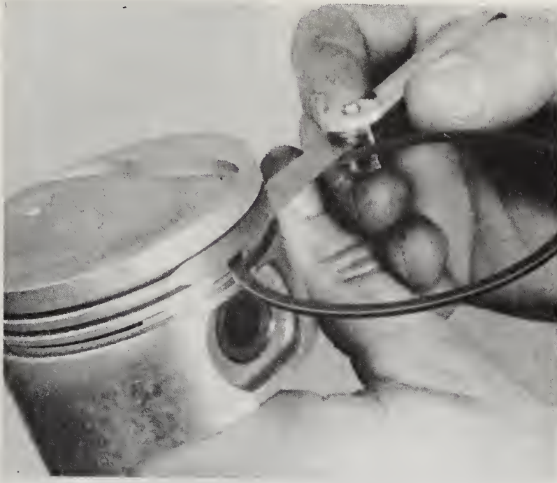
16.10 Insert a ring in the groove then use a feeler gauge to measure the side clearance
