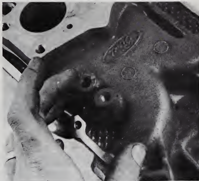
8.15a Apply sealing compound to the bolt bosses prior to installation
