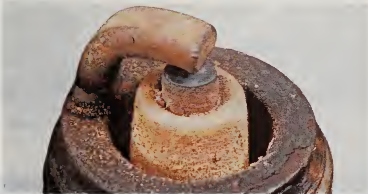
Normal. Gray brown deposits, lightly coated core nose. Gap increasing by around 0.001 in (0.025 mm) per 1000 miles (1600 km). Plugs ideally suited to engine, and engine in good condition
