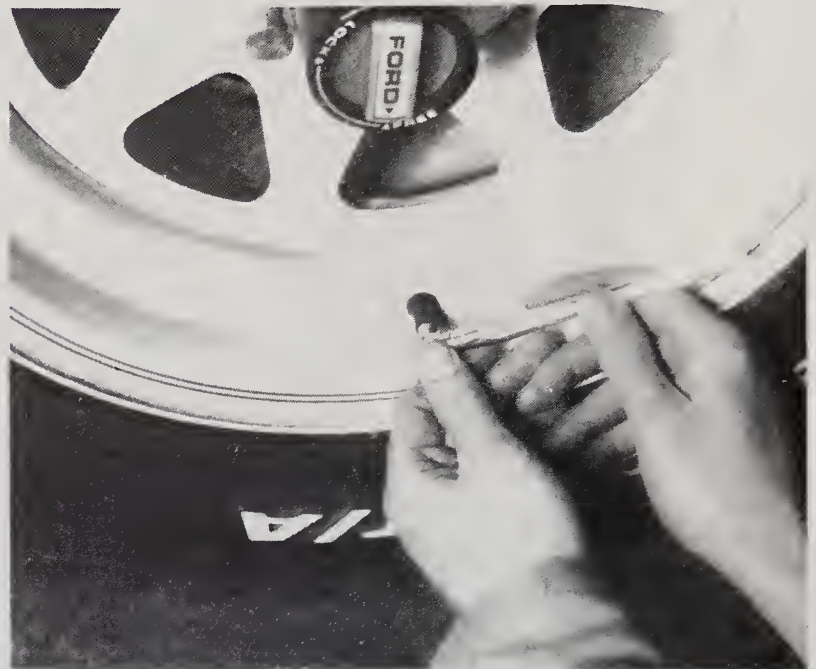
3.6 The use of an accurate tire pressure gauge is essential for long tire life
