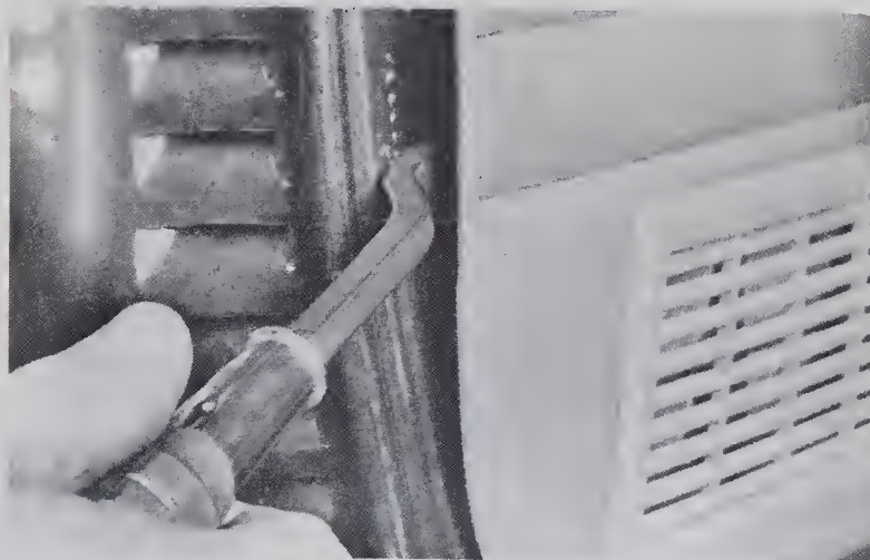
12.5 Wedge a flat screwdriver under the panel and pry near the plastic retainers to remove the panel. Do not pull on the panel or the retainers could pull out of the panel
