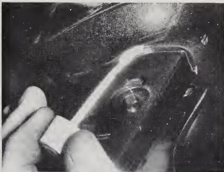
8.3 Paint or scribe alignment marks on the hood to assure proper alignment during installation
