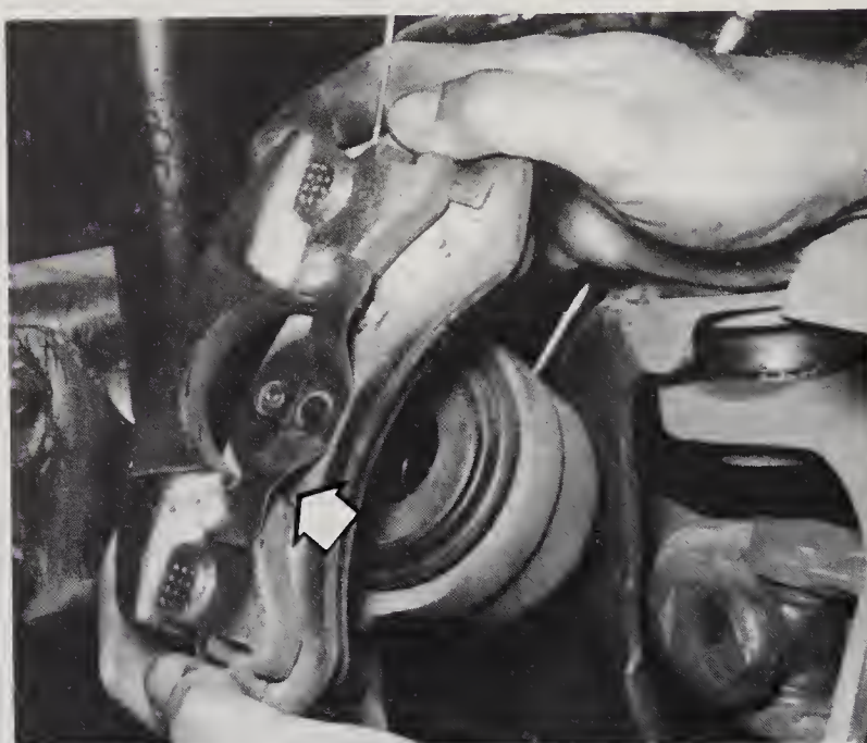
7.10 This spring clip (arrow) holds the outside brake pad to the caliper. Push down and slide out to remove
