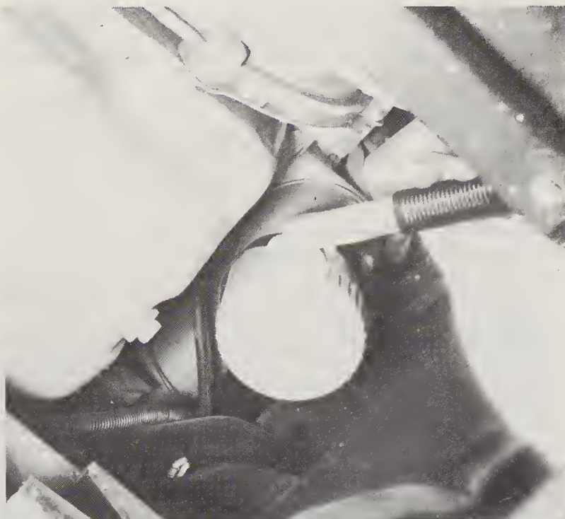
16.14 A strap-type wrench is used to loosen the oil filter
