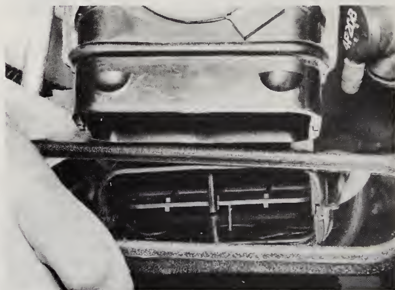
20.6 As the engine warms up the damper door should open
