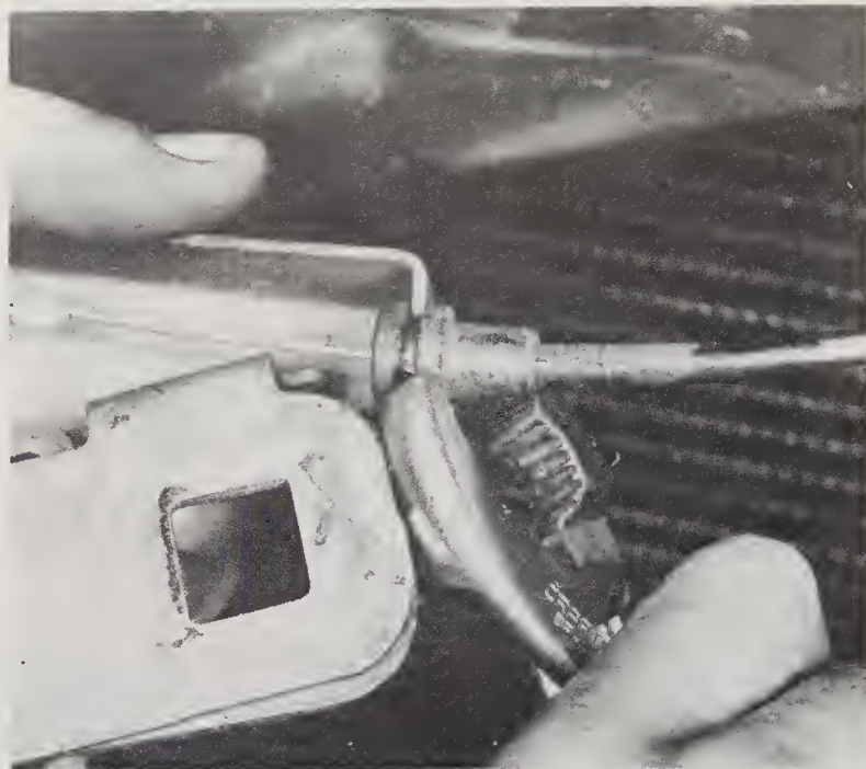
9.4 Use pliers to remove the rubber cable anchor from the latch
