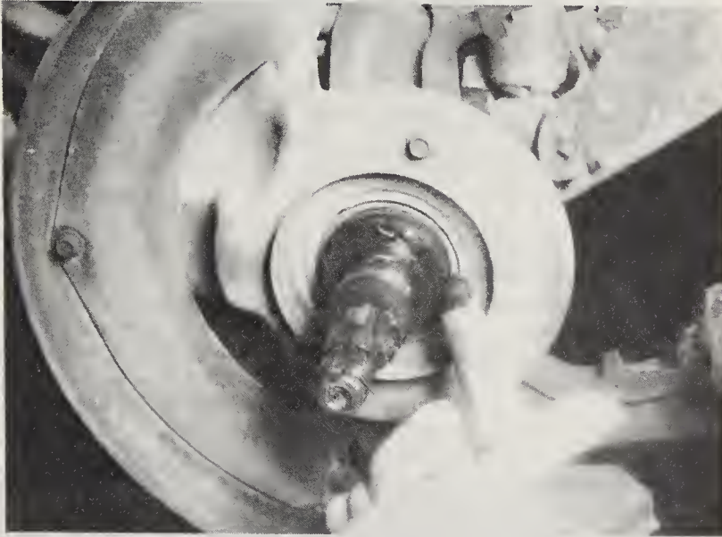
29.17 Apply a thin coat of grease to the spindle surface
