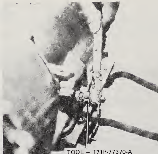
10.3 C3 transmission front band adjustment
