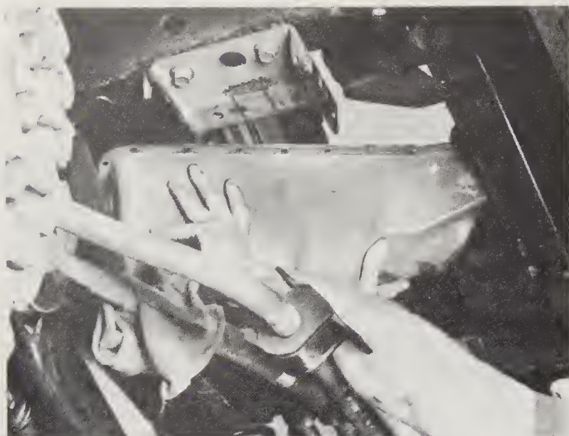
4.22 Drop the oil pump and pick up assembly into the pan and remove the pan from the front
