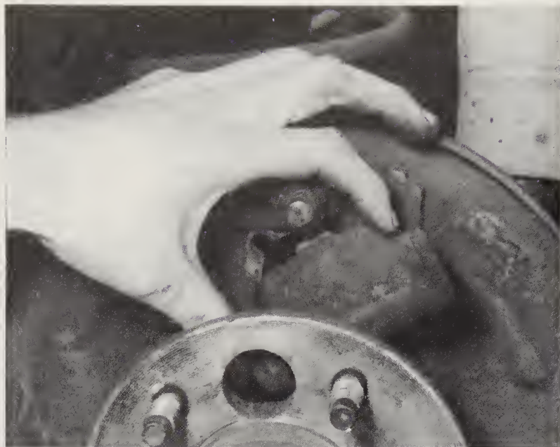
10.3 Remove the bolts from the backing plate and remove the wheel cylinder
