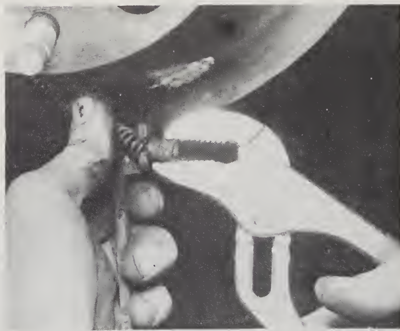
9.4/13 Separate the parking brake cable and spring from the actuating lever
