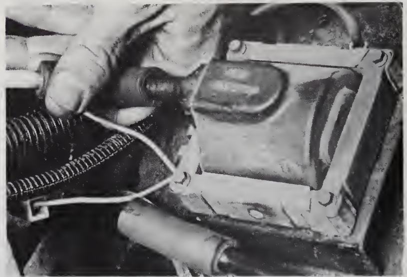
16.14 Disconnect the ignition coil wire
