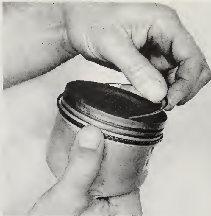
19.9b Roll the oil ring side rails into place above and below the expander
