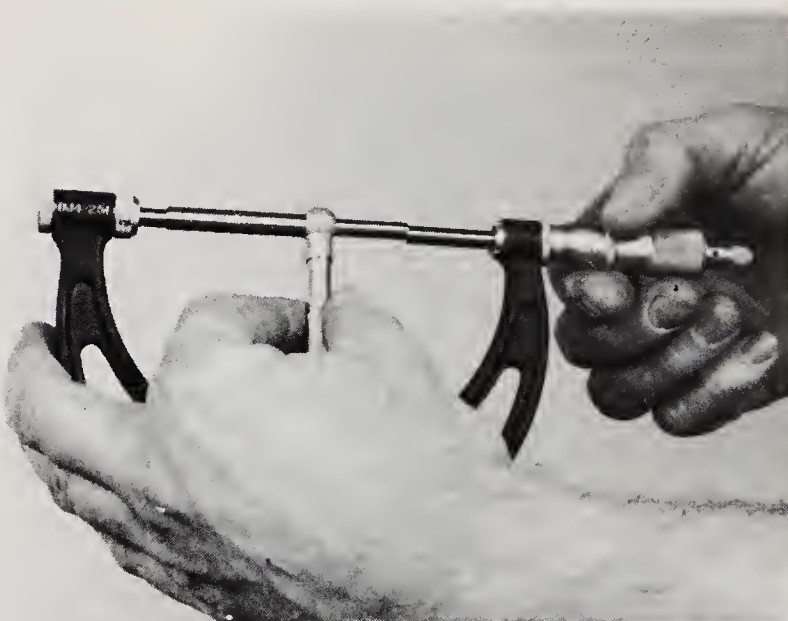
14.4b A micrometer is used measure the snap gauge, giving the bore size
