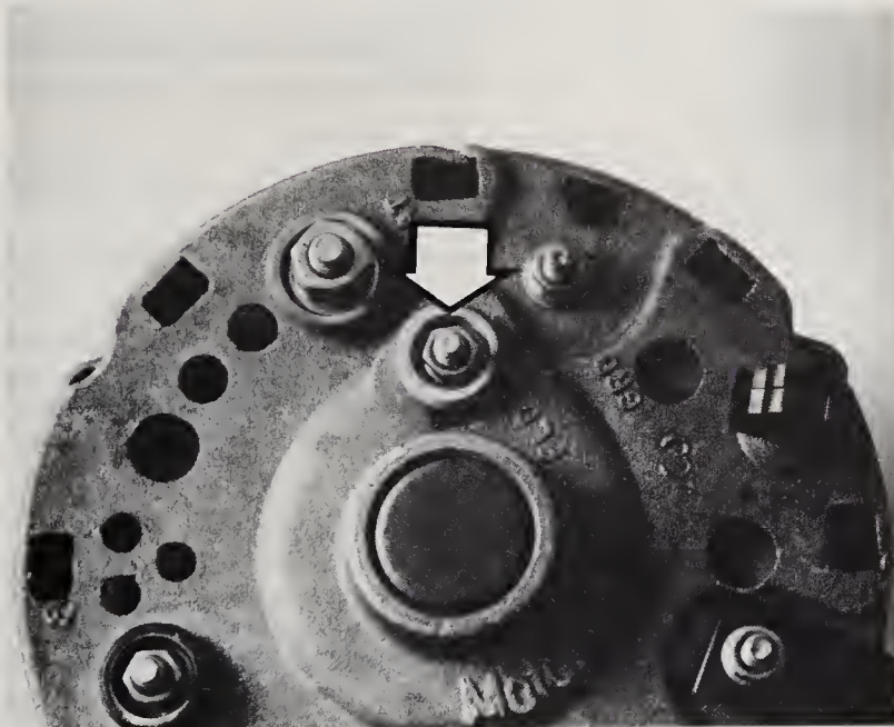
17.5b Remove the rear field housing nut (orange) to remove the remaining brush
