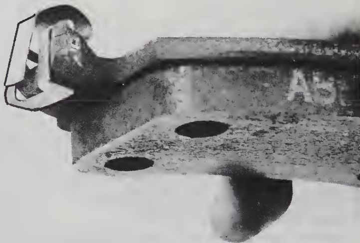
7.21b The anti-rattle spring clip properly installed on the brake pad
