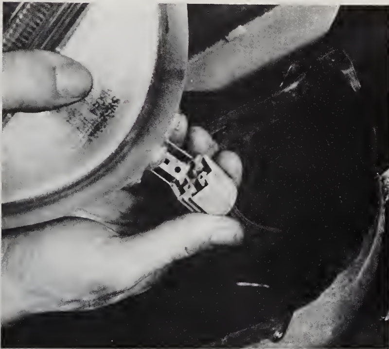
9.4 Support the headlight while you pull the connector off
