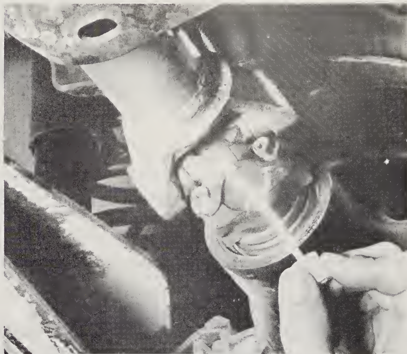
11.2 Index the driveshaft U-joint assembly for reinstallation
