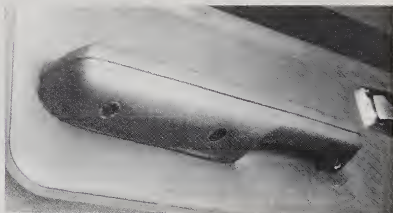
12.1 Remove the three screws retaining the arm-rest to the door
