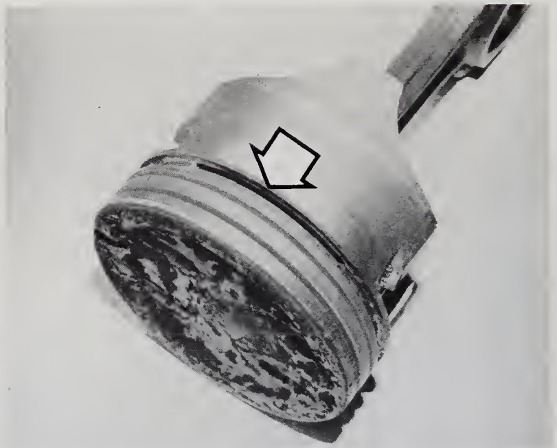
16.5 Make sure the oil return slots (arrow) are clear
