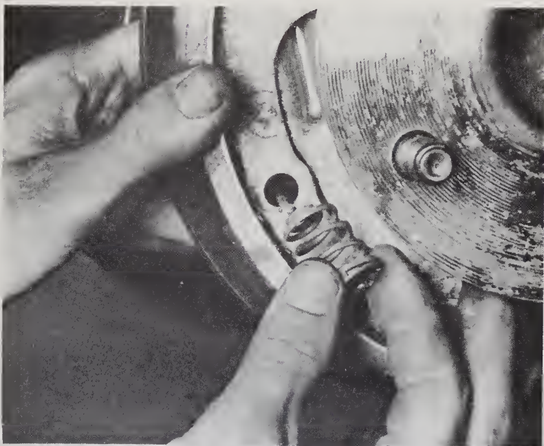
9.4/18 Insert the retaining pins through the backing plate and shoes and put the springs over them
