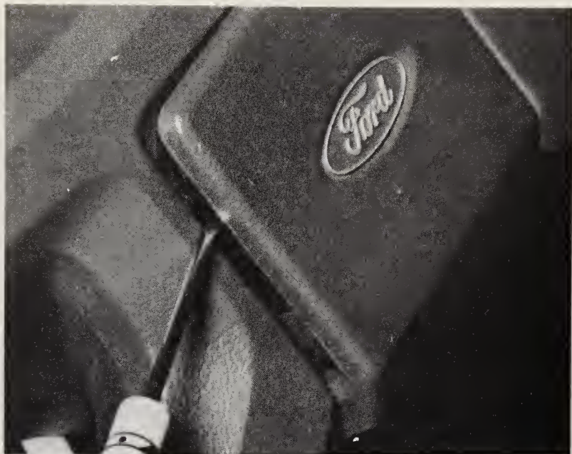
23.1 Pop off the cover over the steering wheel retainer nut (Bronco II shown)
