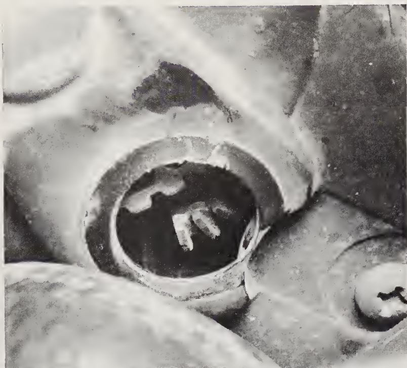
4.30 Remove the timing belt cover access plug and check that the timing mark is lined up with the pointer on the inner belt cover
