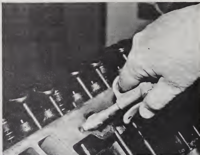
8.5b Use compressed air to clean out the threaded holes after running the tap through them
