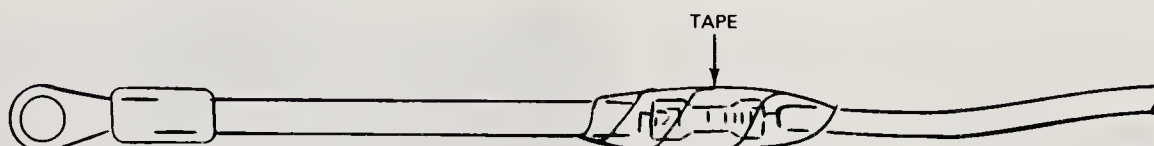
TYPICAL REPAIR USING THE EYELET TERMINAL FUSE LINK OF THE SPECIFIED GAUGE FOR ATTACHMENT TO A CIRCUIT WIRE END
