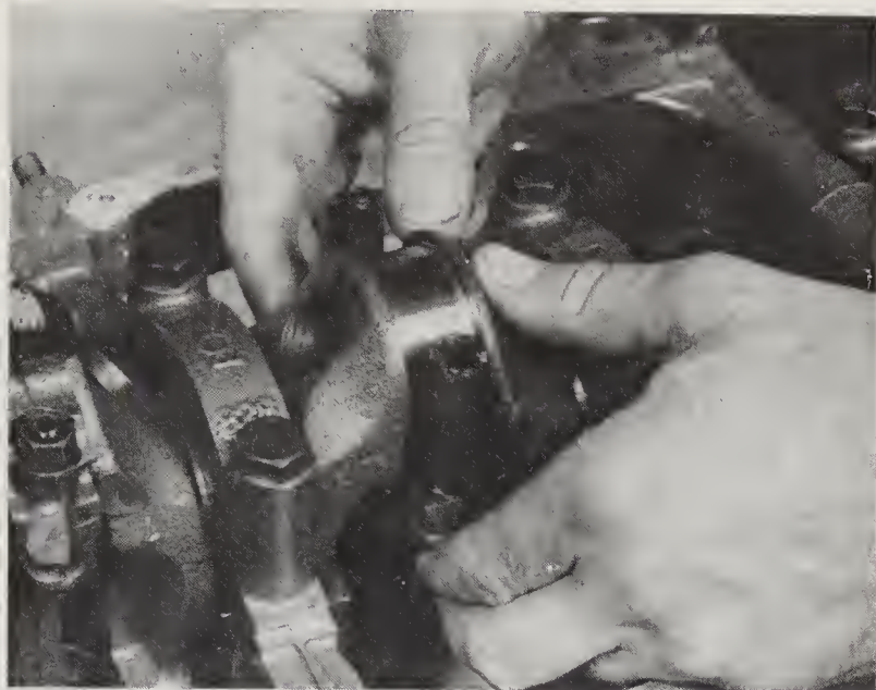
22.13a Pull the connecting rod firmly against the crankshaft
