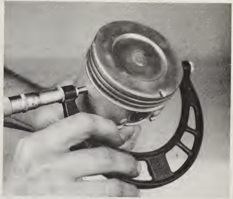
16.11 Measure the piston across the skirt at 90° to the pin
