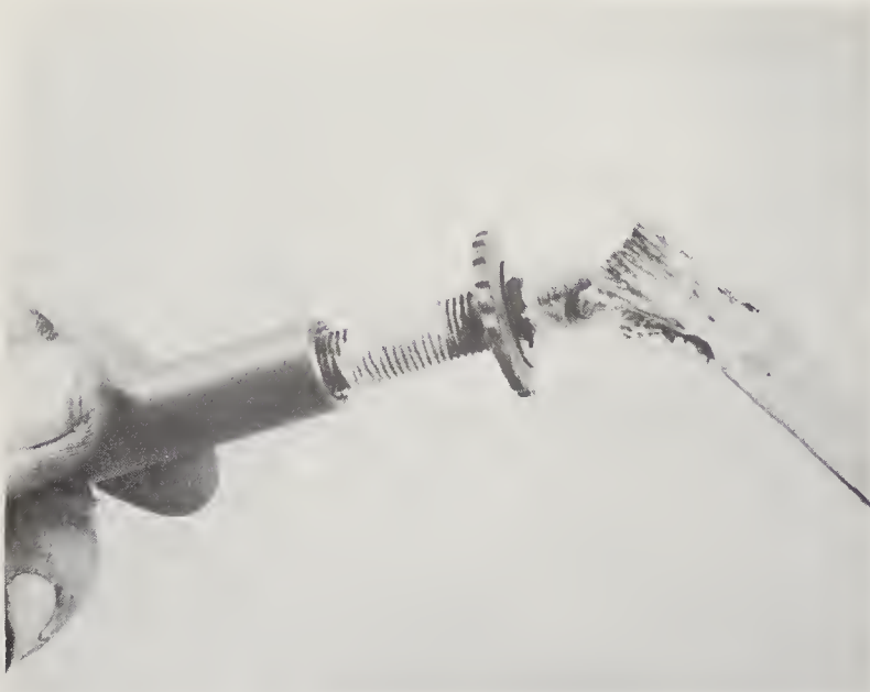
9.4/16 Lubricate the adjusting screw assembly with white grease
