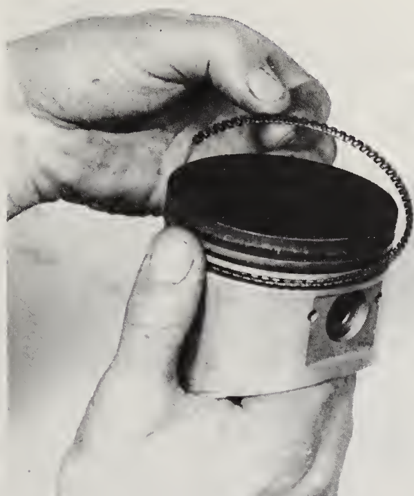
19.9a Install the oil control ring expander in the bottom piston groove
