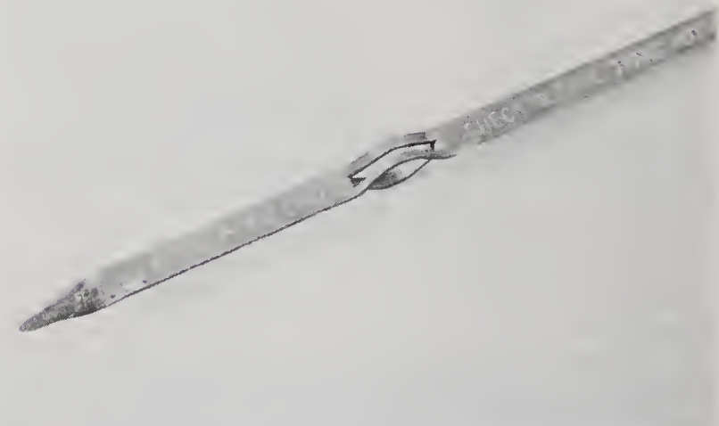
4.37 Follow the directions stamped on the transmission dipstick to get an accurate reading
