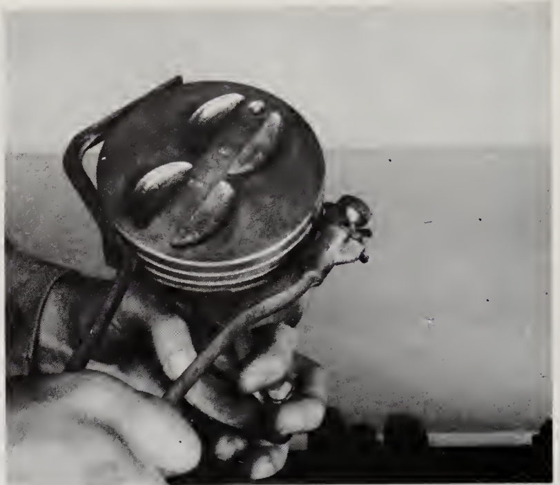
16.4a A cleaning tool can be used to remove carbon build-up from the ring grooves in the piston
