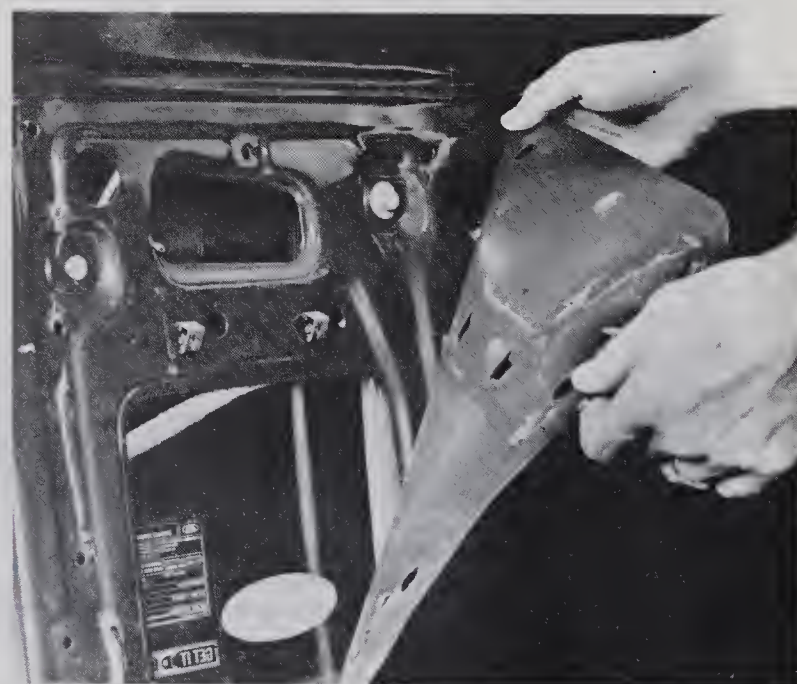
12.6 Pull the weather cover off gently so as not to tear it
