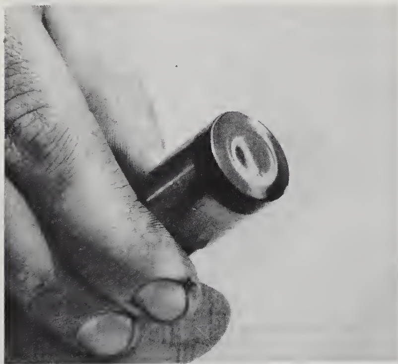
15.15 A concave wear pattern on the base of this lifter indicates the need for a new camshaft and a complete set of lifters
