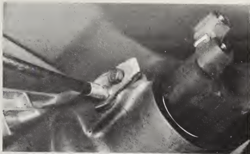
3.11 Remove the retaining bolt and retainer to disconnect the speedometer cable
