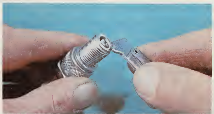
Adjusting plug gap. The plug gap is adjusted by bending the ground electrode inwards, or outwards, as necessary until the correct clearance is obtained. Note the use of the correct tool
