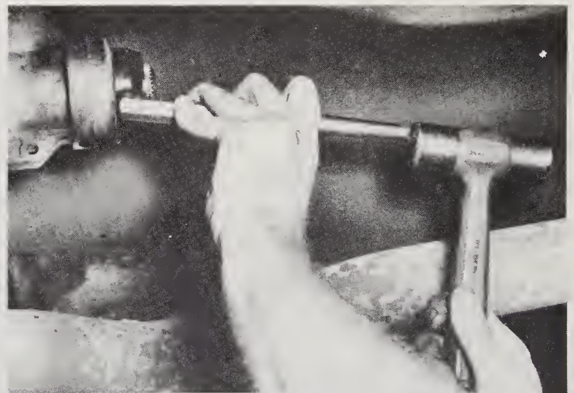
13.7 Installing the new extension housing seal with a punch and hammer. A large socket or length of pipe of the proper diameter may also be helpful as installation tools
