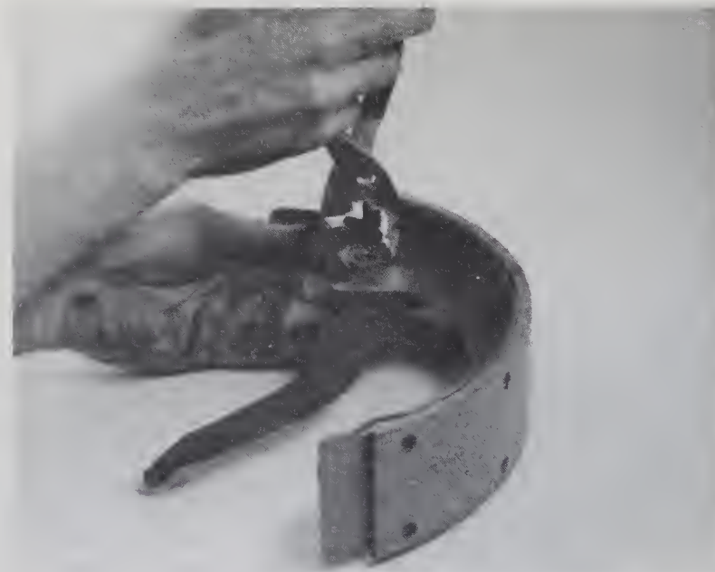
9.4/15 Install the parking brake actuator lever on the new brake shoe and install the E-clip
