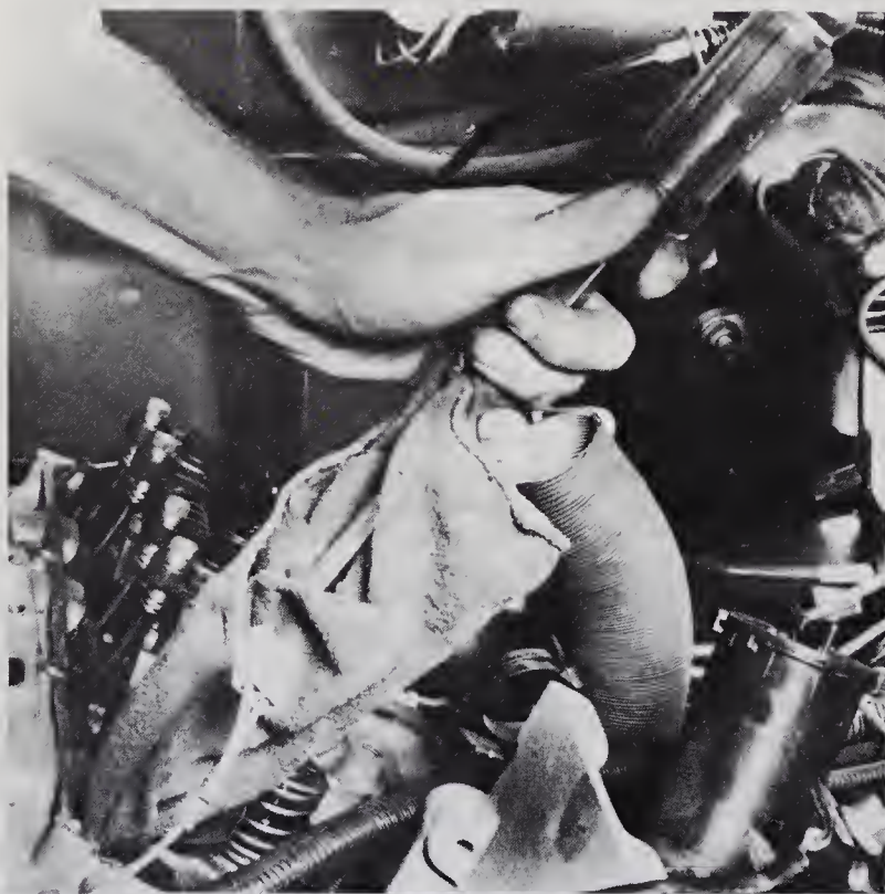
8.12 Use a screwdriver wrapped with a rag and carefully pry up to break the gasket seal
