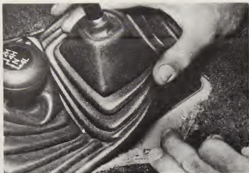
3.2a Hold back the carpet to get at the shifter boot retaining bolts
