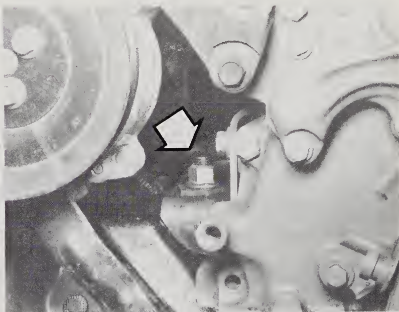
4.16 Remove the attaching nut (arrow) from the front motor mount
