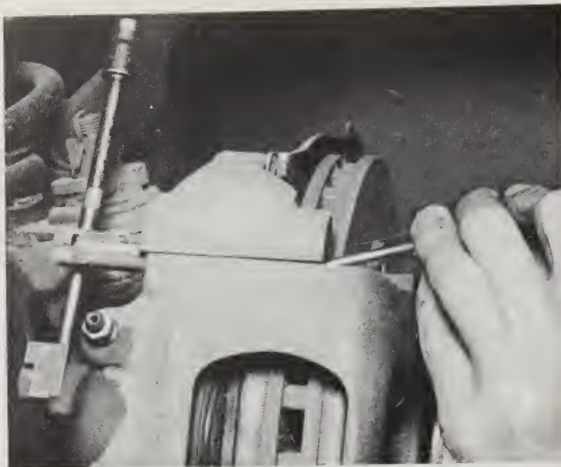
7.7 Drive out the pin with a punch and hammer
