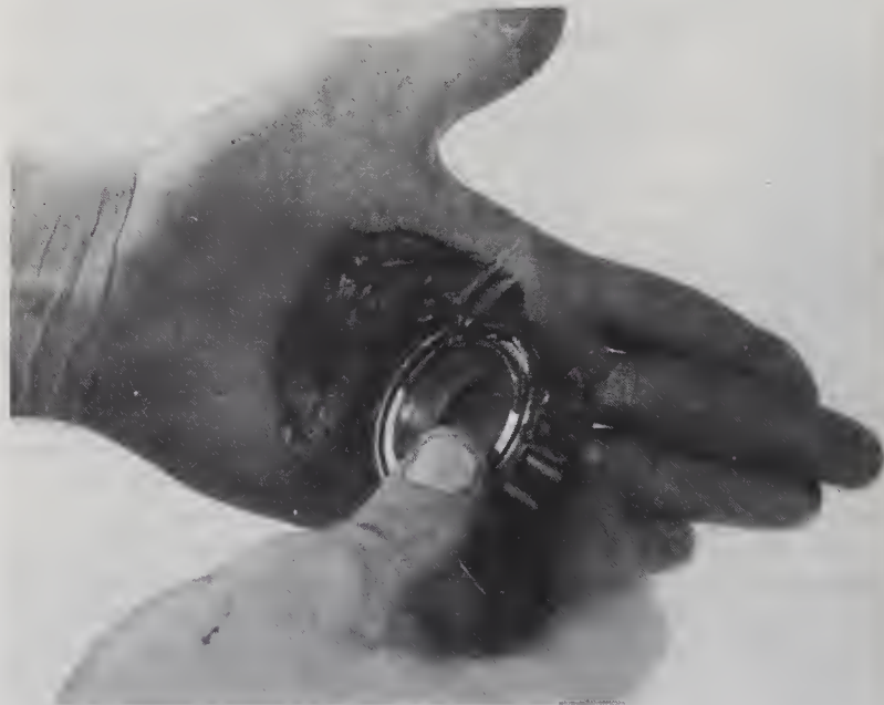
29.15 Packing the bearing with high-temperature wheel bearing grease (work it well into the rollers)
