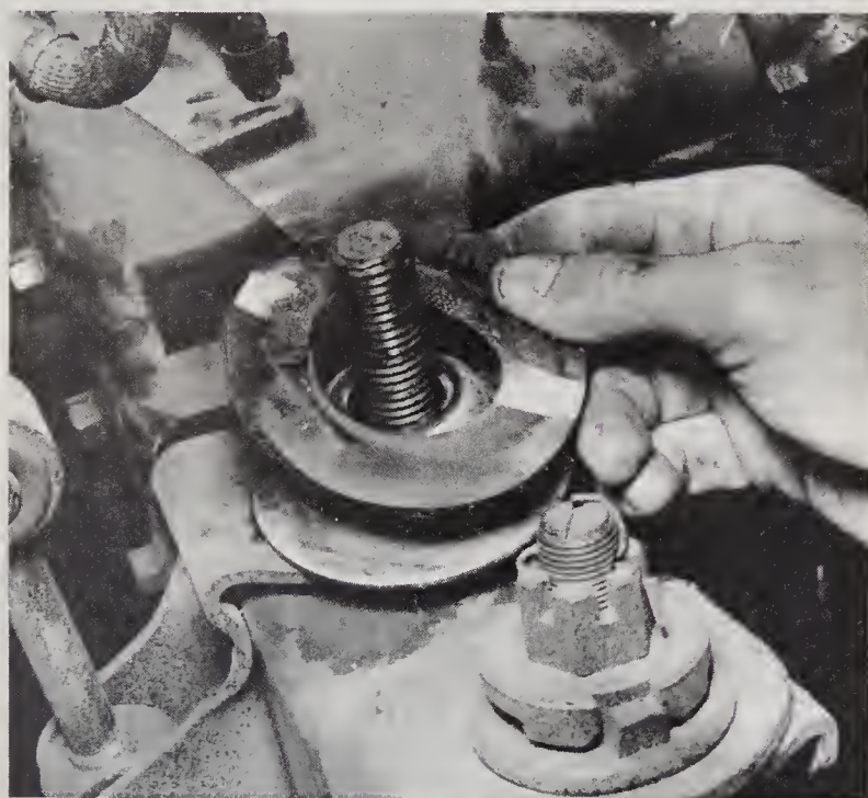
6.9 Before assembly make sure the lower spring seat and insulator are in position
