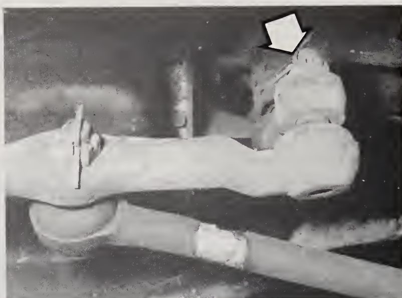
3.3 Remove the cotter pin and nut (arrow) to disconnect the tie rod end
