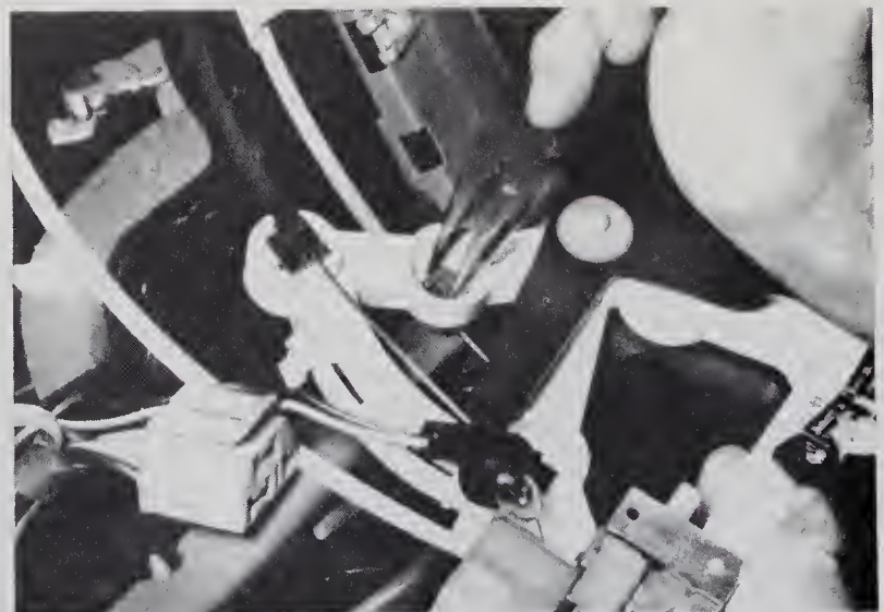
12.13 Release the temperature cable (blue) and air door cable (white) snap-in flags
