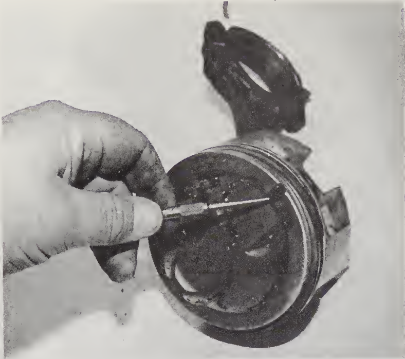
22.8a The pistons will have a notch in the crown, which should point to the front of the engine after the piston is installed
