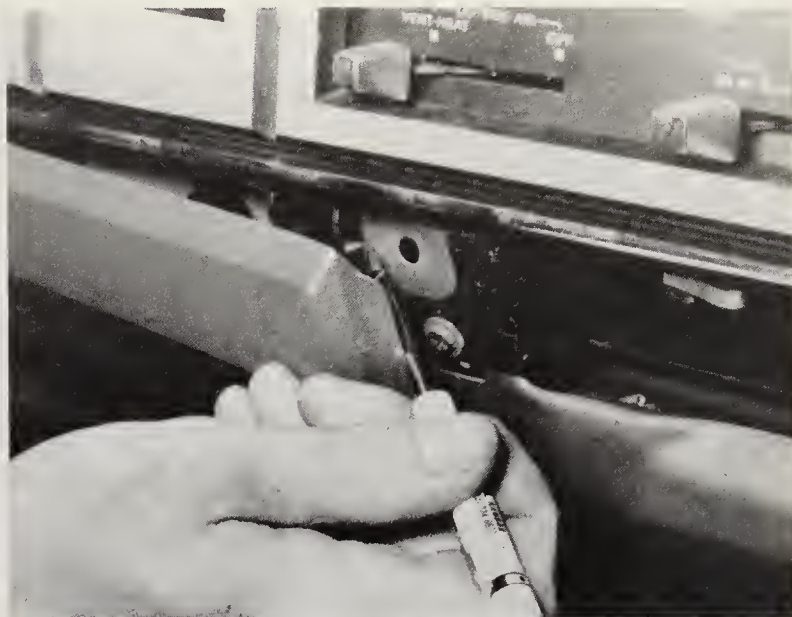
15.2 The bottom dash panels are secured with spring clips
