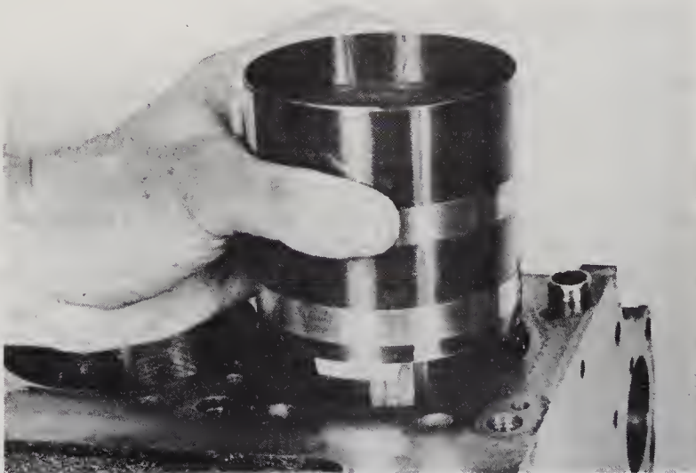
22.8c With the ring compressor installed, slide the piston and rod assembly into the cylinder
