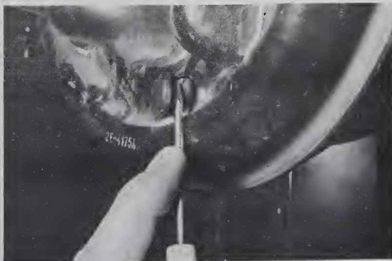
9.4/2 If, after releasing the parking brake, the drum will not slide off the shoes, remove the rubber plug from the backing plate
