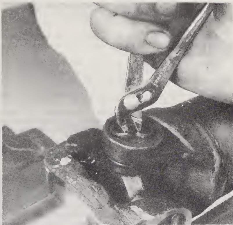
12.2 The universal joint snap rings can be removed with pliers
