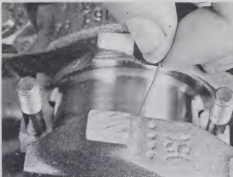
22.12 Cut a piece of Plastigauge and lay it across the crankshaft rod journal
