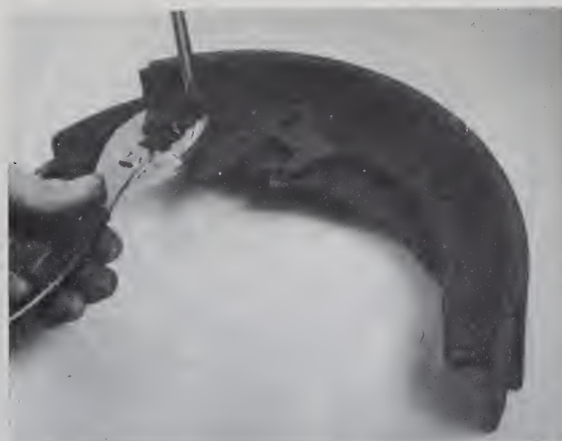
9.4/14 Remove the E-clip which holds the parking brake actuating lever to the brake shoe
