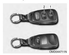
To lock the doors, press the Door Lock button (1) on the remote key.
