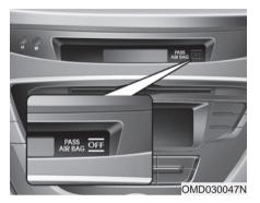
Your vehicle is equipped with an Occupant Classification System (OCS) in the front passenger's seat. The OCS is designed to detect the presence of a properly-seated front passenger and determine if the passenger's front air bag should be enabled (may inflate) or not. The driver's front air bag is not affected or controlled by the OCS.
