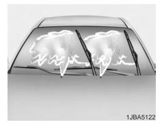
Contamination of either the windshield or the wiper blades with foreign matter can reduce the effectiveness of the windshield wipers. Common sources of contamination are insects, tree sap, and hot wax treatments used by some commercial car washes. If the blades are not wiping properly, clean both the window and the blades with a clean cloth dampened with washer fluid.
