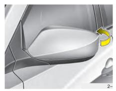
To fold the outside rearview mirror, grasp the housing of the mirror and then fold it toward the rear of the vehicle.
