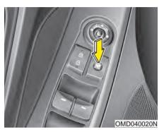
The driver can disable the power window switches on the passengers' doors by pressing the power window lock switch.
