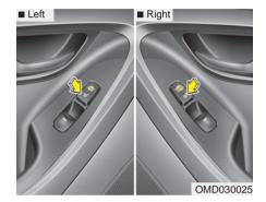
While the engine is running, push either switch to warm the rear seat. During mild weather or under conditions where the operation of the seat warmer is not needed, keep the switches in the "OFF" position.
