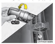
When the light switch is in the AUTO position, the parking (position) light and headlights will be turned ON or OFF automatically depending on the amount of light outside the vehicle.
