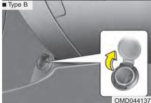
The power outlet is designed to provide power for mobile telephones or other devices designed to operate with vehicle electrical systems. The devices should draw less than 15 amps with the engine running.
