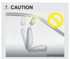
If you recline the seatback towards the front with the headrest and seat cushion raised, the headrest may come in contact with the sunvisor or other parts of the vehicle.
