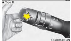
To flash the high beam headlights, pull the lever towards you, then release the lever. The high beams will remain ON as long as you hold the lever towards you.
