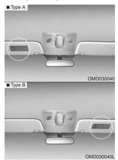
Air bag warning labels, required by the U.S. National Highway Traffic Safety Administration (NHTSA), are attached to alert the driver and passengers of potential risks of the air bag system. Be sure to read all of the information about the air bags that are installed on your vehicle in this Owners Manual.
