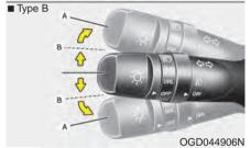
To signal a turn, move the lever up for a right turn or down for a left turn to position (A). The lever will return to the OFF position when the turn is completed.
