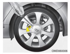
Insert the screwdriver into the groove of the wheel cap and pry gently to remove the wheel cap (If equipped).
