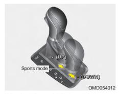
Whether the vehicle is stationary or in motion, sports mode is selected by pushing the shift lever from the D (Drive) position into the manual gate. To return to D (Drive) range operation, push the shift lever back into the main gate.
