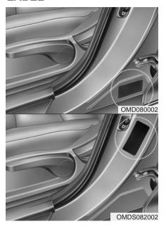
The vehicle certification label attached on the driver's side center pillar gives the Vehicle Identification Number (VIN).
