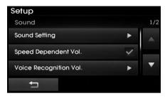
The volume level is controlled automatically according to the vehicle speed. SDVC can be set by selecting from Off/Low/Mid/High.
