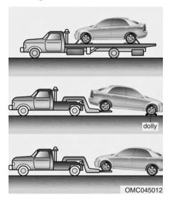
If emergency towing is necessary, we recommend having it done by an authorized HYUNDAI dealer or a commercial tow-truck service. Proper lifting and towing procedures are necessary to prevent damage to the vehicle. The use of wheel dollies or flatbed is recommended.
