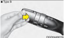
To turn on the high beam headlights, push the lever away from you. Pull it back for low beams.
