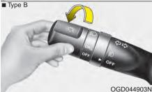
When the light switch is in the parking light position (1st position), the parking lights, taillights, license plate lights and instrument panel lights are turned ON.
