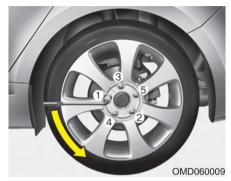
7.Loosen the wheel lug nuts counterclockwise one turn each in the order shown above, but do not remove any lug nuts until the tire has been raised off of the ground.
