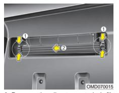
Remove the climate control air filter case by pulling out both sides of the cover.
