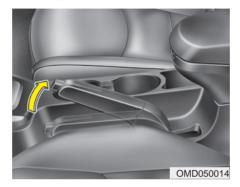
Always set the parking brake before leaving the vehicle, to apply: Firmly depress the brake pedal.
