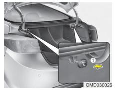
3.Pull on the seatback folding lever located in the trunk.
