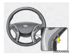
The Driver Selectable Steering Mode controls steering effort as driver's preference or road condition. You can select the desired steering mode by pressing the steering mode button. The driver selectable steering mode stays in the last mode selected when turning the engine on.
