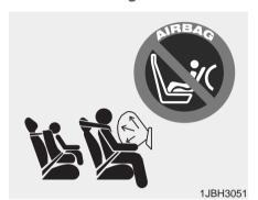
Even though your vehicle is equipped with the OCS, never install a child restraint in the front passenger's seat. An inflating air bag can forcefully strike a child or restraint resulting in serious or fatal injury.
