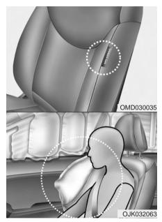
Your vehicle is equipped with a side impact air bag in each seat. The purpose of the air bag is to provide the vehicle's driver and the front passenger with additional protection than that offered by the seat belt alone.
