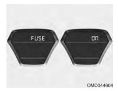
This warning message illuminates if the fuse switch under the steering wheel is OFF.
