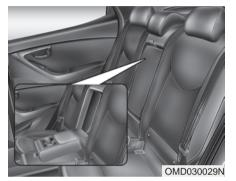
The armrest is located in the center of the rear seat. Pull the armrest down from the seatback to use it. You will find cup holders on the center armrest.
