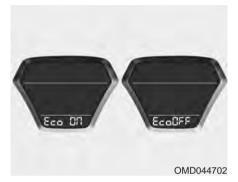
You can turn the Manual transaxle shift indicator ON/OFF on the instrument cluster in this mode.
