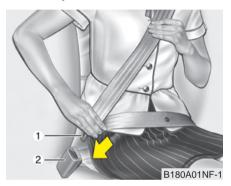
Pull the seat belt out of the retractor and insert the metal tab (1) into the buckle (2). There will be an audible "click" when the tab locks into the buckle.
