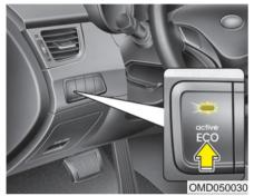
Active ECO helps improve fuel efficiency by controlling the engine and transaxle. Fuel-efficiency is determined by the driver's driving habits and road conditions.
