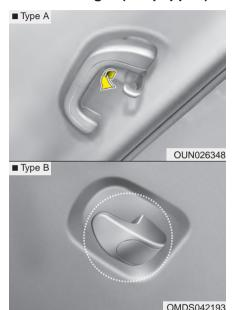
To hang items, pull down the upper portion of the hanger. (Type A) These hangers are not designed to hold large or heavy items.
