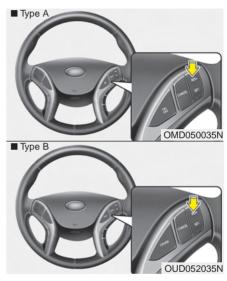
Push the RES+ switch and hold it, while monitoring the SET speed on the instrument cluster. Release the switch when the desired speed is shown and the vehicle will accelerate to that speed.
