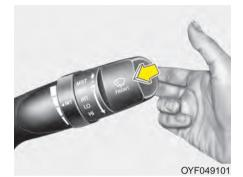
In the OFF position, pull the lever gently toward you to spray washer fluid on the windshield and to run the wipers 1-3 cycles. Use this function when the windshield is dirty.
