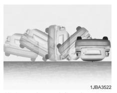
Air bags do not inflate in rollover accidents because vehicle can not detect rollover accident.
