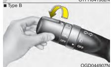
When the light switch is in the head light position (2nd position), the headlights, parking lights, taillights, license plate lights and instrument panel lights are turned ON.
