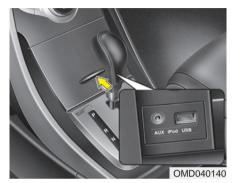
If your vehicle has an aux and/or USB(universal serial bus) port, you can use an aux port to connect audio devices and an USB port to plug in an USB and iPod.
