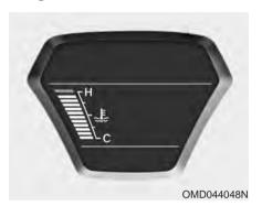
This gauge shows the temperature of the engine coolant when the ignition switch is in the ON position.
