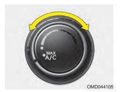
The temperature control knob allows you to control the temperature of the air flowing from the ventilation system. To change the air temperature inside the vehicle, turn the knob to the right for warm air or left for cooler air.
