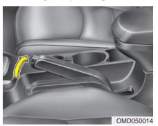
Check the stroke of the parking brake by counting the number of "clicks" heard while fully applying it from the released position. Also, the parking brake alone should securely hold the vehicle on a fairly steep grade. If the stroke is more or less than specified, have the parking brake adjusted by an authorized HYUNDAI dealer.
