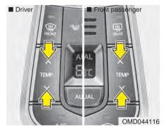
The temperature will increase by pushing the up button. Each push of the button will cause the temperature to increase by 1°F/0.5°C.
