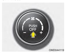
Push the OFF button to turn off the air climate control system. However, you can still operate the mode and air intake buttons as long as the ignition switch is in the ON position.
