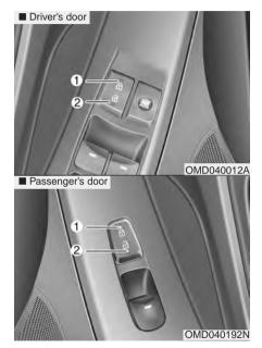
When pressing the (1) portion (1) of the switch, all vehicle doors will lock.
