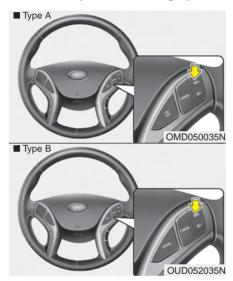
Push the RES+ switch. If the vehicle speed is over 20 mph (30 km/h), the vehicle will resume the preset speed.
