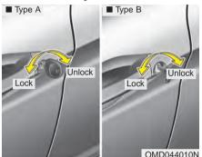
Turn the key toward the rear of the vehicle to unlock and toward the front of the vehicle to lock.
