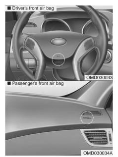
The purpose of the SRS is to provide the vehicle's driver and front passengers with additional protection than that offered by the seat belt system alone. The SRS uses sensors to gather information about the driver's seat position, the driver's and front passenger's seat belt usage and impact severity.
