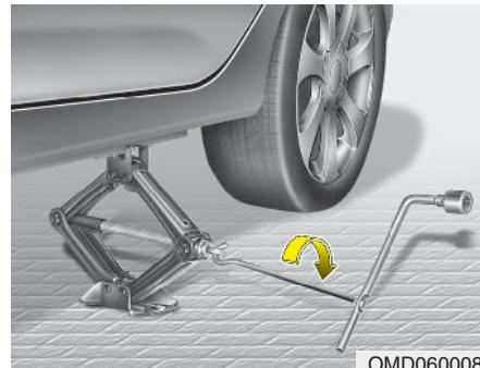
9. Insert the jack handle into the jack and turn it clockwise, raising the vehicle until the tire just clears the ground. This measurement is approximately 1.2 in (30 mm). Before removing the wheel lug nuts, make sure the vehicle is stable and that there is no chance for movement or slippage.
