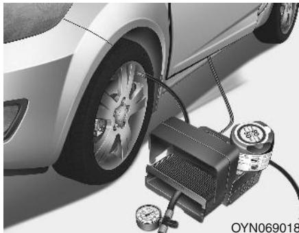
6. Ensure that the compressor is switched off, position 0.
