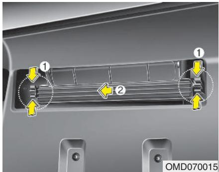
2. Remove the climate control air filter cover (2) while pressing the lock (1) on the right of the cover.
