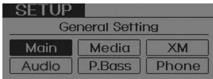
In "SETUP" mode, rotate the knob to move the cursor between items, and push the button to select.
