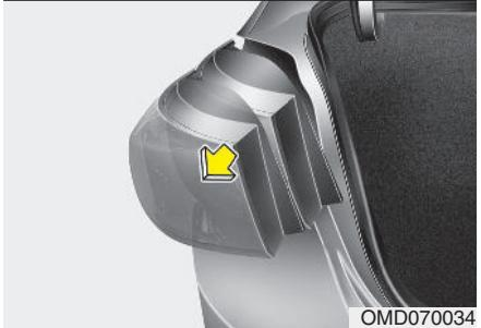
3. Loosen the assembly retaining nuts.
