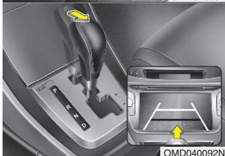
The rearview camera will activate when the back-up light is ON with the ignition switch ON and the shift lever in the R position.
