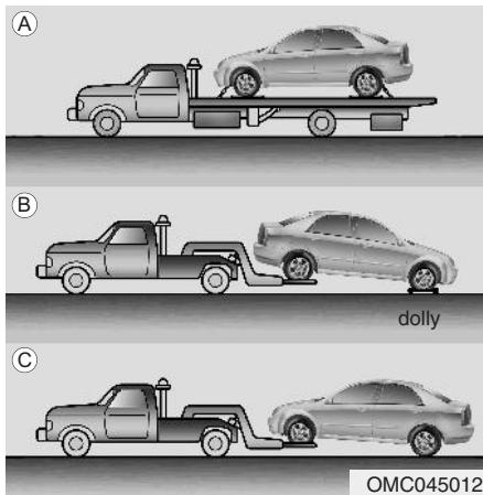
It is acceptable to tow the vehicle with the rear wheels on the ground (without dollies) and the front wheels off the ground. If any of the loaded wheels or suspension components are damaged or the vehicle is being towed with the front wheels on the ground, use a towing dolly under the front wheels.
