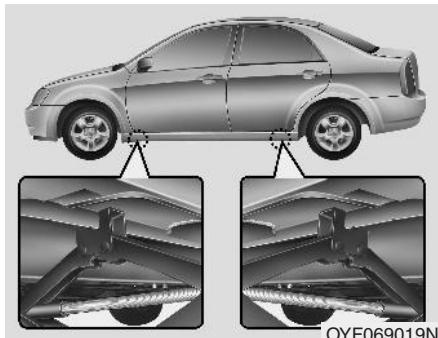
8. Place the jack at the front or rear jacking position closest to the tire you are changing. Place the jack at the designated locations under the frame.
