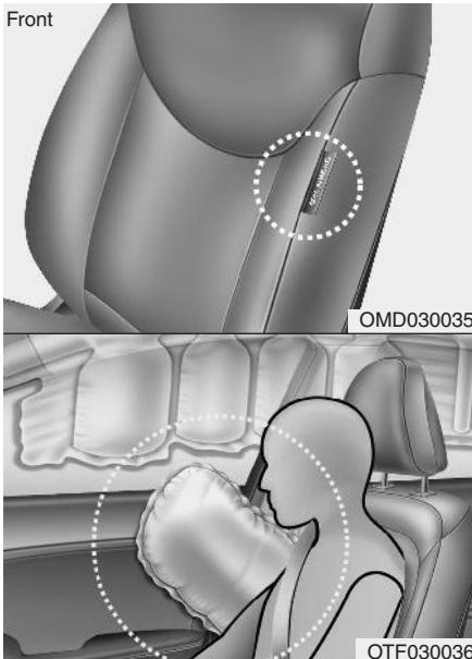
The side impact air bags are designed to deploy only during certain side-impact collisions, depending on the crash severity, angle, speed and point of impact. The side impact air bags are not designed to deploy in all side impact situations.
