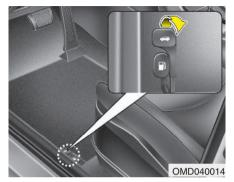
To open the trunk from inside the vehicle, pull the trunk lid release switch.
