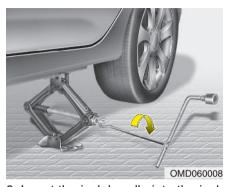
9. Insert the jack handle into the jack and turn it clockwise, raising the vehicle until the tire just clears the ground. This measurement is approximately 1.2 in (30 mm). Before removing the wheel lug nuts, make sure the vehicle is stable and that there is no chance for movement or slippage.
