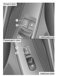
With central door lock switch (if equipped)
