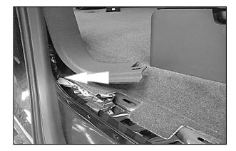
14. Connect the subwoofer body harness (D) to the subwoofer power harness (B).
