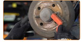
Unscrew the brake drum fastening. Use a drive socket #12. Use a ratchet wrench.
