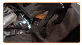
Screw the new filter into its place.
