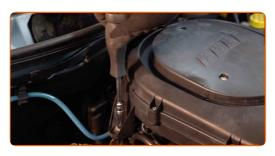
Install the air filter housing retaining spring.
