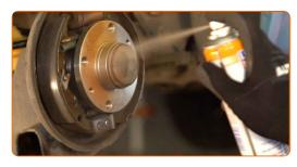
17 Install the brake drum and fasten it.
