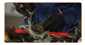
Press out the wheel hub bearing.
