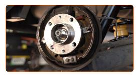
Tighten the hub. Use a drive socket #32. Use a torque wrench. Tighten it to 280 nm torque.
