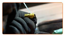
Attach the fuel pressure sensor connector.
