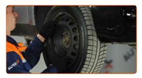
6.1 Unscrew the brake caliper bracket fasteners.
