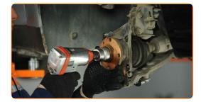
Unscrew the end fastening nut to the steering knuckle. Use a drive socket #17. Use a ratchet wrench.
