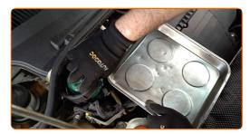
Unscrew the filter housing cap together with the old filter element. Put the old filter cartridge in the container.
