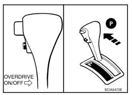
4. Turn ignition switch ON. (Do not start engine.) Does O/D OFF indicator lamp come on for about 2 seconds?
