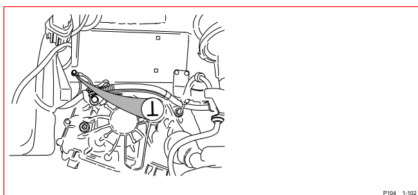
31/110 Ground connection, Right MacPherson strut tower
