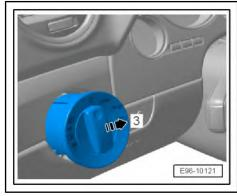
Release connector -arrow- and disconnect.
