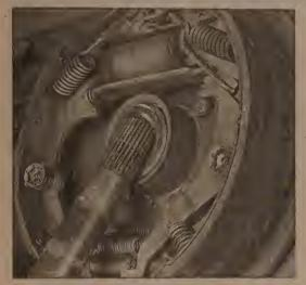
16.2 The axleshaft oil seal can sometimes be pried out with the end of the axle
