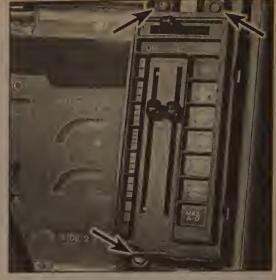
18.3a Air conditioner/heater control mounting screws (arrows) (1985 to 1995 models)
