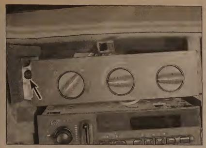
18.3b Air conditioner/heater control mounting screw on 1996 and later models (arrow) - remove the screw and pivot the control away from the instrument panel
