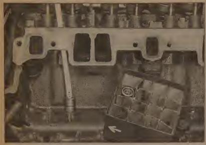
11.12 The lifters on an engine that has accumulated many miles may have to be removed with a special tool - be sure to store the lifters in an organized manner to make sure they are installed in their original locations
