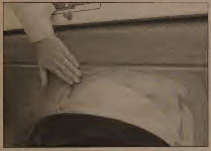
9 You shouldn't be able to feel any ridge at the transition from the filler to the bare metal or from the bare metal to the old paint.
