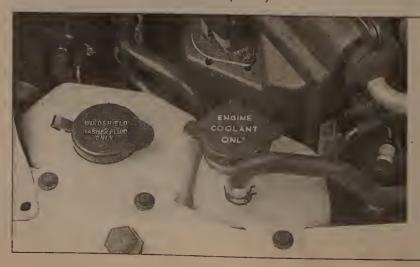
6.2 Coolant reservoir mounting details - note that the windshield washer reservoir must be raised first
