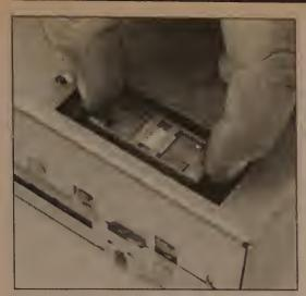
3.13 Grasp the PROM carrier at the narrow ends and gently rock the removal tool until the PROM is disconnected
