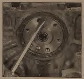
20.5 Carefully pry the oil seal out with a screwdriver - don't nick or scratch the crankshaft or the new seal will be damaged and leaks will develop
