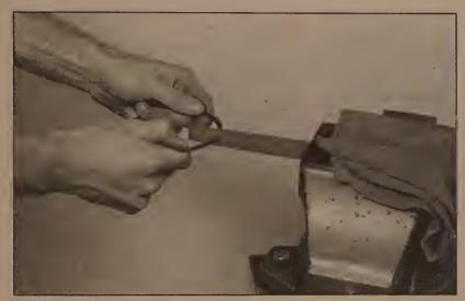
21.5 If the end gap is too small, clamp a file in a vise and file the ring ends (from the outside in only) to enlarge the gap slightly
