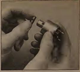
12.11 Gently rotate the fuel injector filter back and forth and carefully pull it off the nozzle
