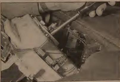
11.3 On 1992 and earlier models, the VSS is located behind the instrument cluster - the VSS electrical connector is secured by a retaining screw
