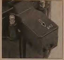
3.3 If your engine has a coil-in-cap distributor, disconnect the wire from the BAT terminal on the distributor cap when checking the compression
