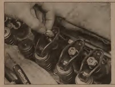
7.11 Moly-base grease applied to the pivot balls will ensure adequate lubrication until oil pressure builds up when the engine is started
