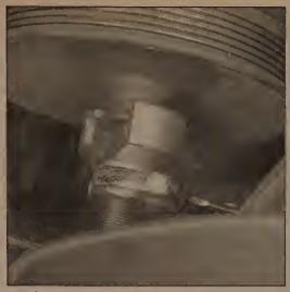
15.9 On models with a serpentine drivebelt the power steering pump pulley must be removed to access the pump mounting bolts. Use a puller like this one to remove the pulley
