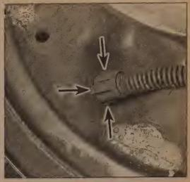
12.5 Depress the retention tangs (arrows) to free the cable and housing from the backing plate
