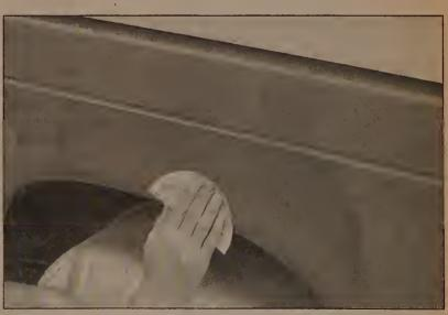
12 Finish sand the primer with very fine sandpaper (400 or 600-grit) to remove the primer overspray. Clean the area with water and allow it to dry. Use a tack rag to remove any dust, then apply the finish coat. Don't attempt to rub out or wax the repair area until the paint has dried completely (at least two weeks)
