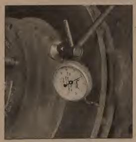
4.4a Check rotor runout with a dial indicator - if the reading exceeds the maximum allowable runout, the rotor will have to be resurfaced or replaced
