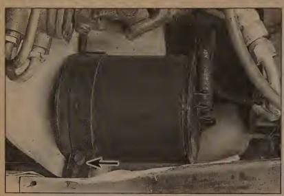
10.19 To remove the carbon canister, label and detach the vacuum lines, then remove the canister clamp bolt (arrow) and lift the canister out (grille, radiator and condenser removed for clarity)
