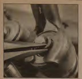
8.3a Use a valve spring compressor to compress the spring, then remove the keepers from the valve stem
