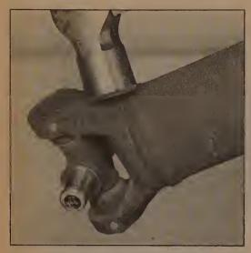
13.9 To relieve stress produced by pressing the bearing caps into the yokes, strike the yoke in the area shown
