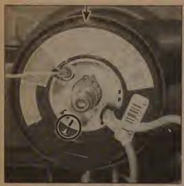
12.9 When properly aligned, the airbag coil will be centered with the marks aligned (in circle here) and the tab fitted between the projections on the top of the steering column
