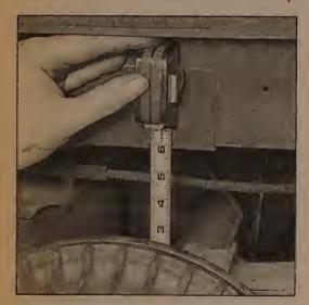
11.15 Before tightening the shackle nuts, raise the axle until the distance between the axle and the frame is 5.9-inches
