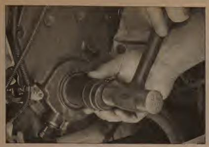
15.4 Installing the front crankshaft oil seal using a deep socket
