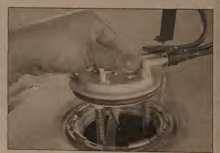
7.16b Withdraw the fuel pump/sending unit assembly from the fuel tank, being careful not to damage the float arm
