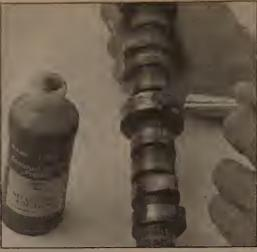
15.34 Be sure to prelube the bearing journals and lobes prior to camshaft installation
