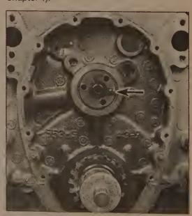
11.20 After the camshaft is in place, turn it until the dowel pin (arrow) is in the 3 o'clock position as shown here
