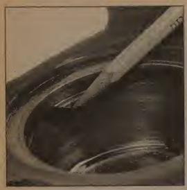
3.10 Remove the piston seal with a wooden or plastic tool to avoid scratching the bore and seal groove
