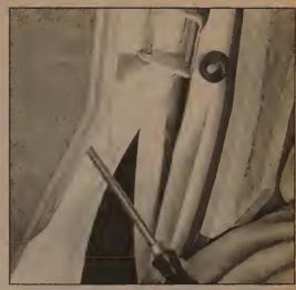
20.5 Insert a screwdriver behind the door panel and pry out very carefully to disengage the retainers
