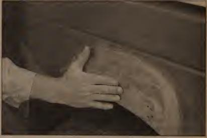
4 When the paint is removed, touch will probably be more helpful than sight for telling if the metal is straight. Hammer down the high spots or raise the low spots as necessary.
