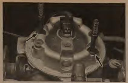
13.51 Remove the throttle body mounting studs (arrows)
