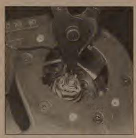
12.6a A pair of snap-ring pliers can be used to remove the safety clip (if equipped) from the shaft
