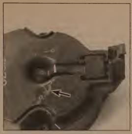
43.4b Carbon tracking on the rotor is caused by a leaking arc seal between the distributor cap and the ignition coil (always replace both the seal and rotor when this condition is present) (coil in cap-type distributor)
