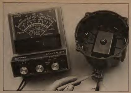
9.10 Measuring the HEI ignition coil (in cap) primary resistance, between the TACH and BAT terminals - the resistance should be nearly zero
