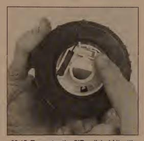
20.15 To center the SIR coil, hold it with its underside facing up, depress the spring lock and rotate the hub in the direction of the arrow on the coil assembly until it stops
