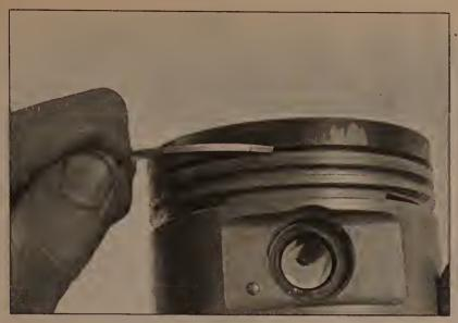
17.4b ... or a section of a broken ring
