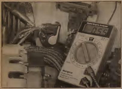
15.125a Use straight pins to backprobe the TPS electrical connector DARK BLUE (+) and BLACK (-) wires. With the throttle closed, the voltage should be approximately 0.5 volts (CMFI engine shown)
