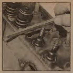
8.3b If the valve won't pull through the guide, deburr the edge of the stem end and the area around the top of the keeper groove with a file
