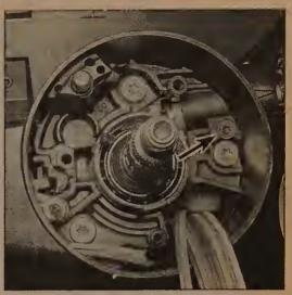
8.13 Remove the lock cylinder retaining screw (arrow), rotate the key to the On position and pull it out of the steering column
