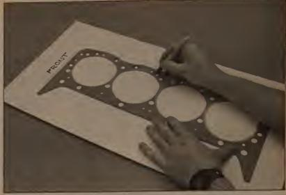
8.15 To avoid mixing up the head bolts, use a new gasket to transfer the bolt hole pattern to a piece of cardboard, then punch holes to accept the bolts
