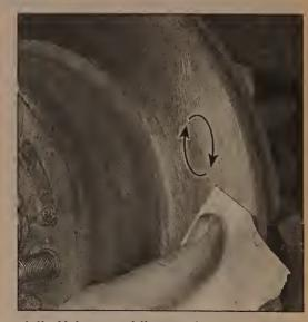
4.4b Using a swirling motion, remove the glaze from the rotor with medium-grit emery cloth
