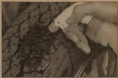
5.4b If the valve core is tight, raise the corner of the vehicle with the low tire and spray a soapy water solution onto the tread as the tire is turned slowly - slow leaks will cause small bubbles to appear
