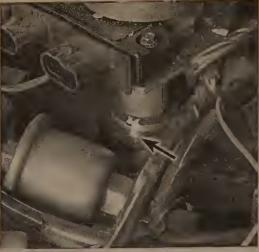
6.24 Mark the position of the distributor in relation to the engine (arrow) before loosening the distributor hold-down clamp
