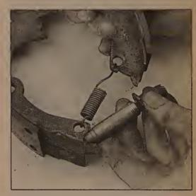
5.4j Spread the bottom of the shoes apart and remove the adjusting screw assembly
