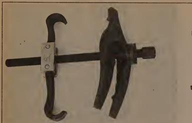
8.5 A typical aftermarket internal type spring compressor: The hooked arms grip the upper coils of the spring, the plate is inserted between the lower coils, and when the nut on the threaded rod is turned, the spring is compressed
