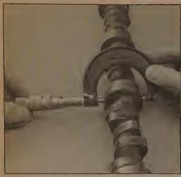
15.28 The camshaft bearing journal diameters are checked to pinpoint excessive wear and out-of-round conditions
