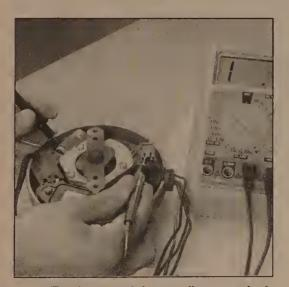
8.5a Testing the pick-up coil on a typical V6 distributor (1990 and earlier)
