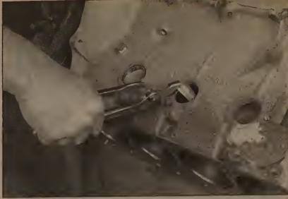
14.1 Use a hammer and a large punch to knock the core plugs sideways in their bores, then pull them out with pliers
