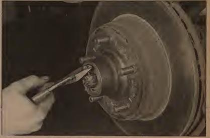
36.7 Remove the cotter pin and discard it - use a new one when the hub is reinstalled
