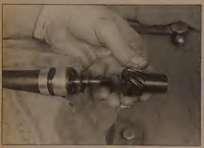
8.10b Remove the driven gear and spacer washers from the end of the shaft, making sure to note the order in which you remove any spacers
