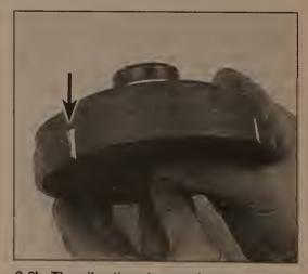
9.6b The vibration damper has two marks
