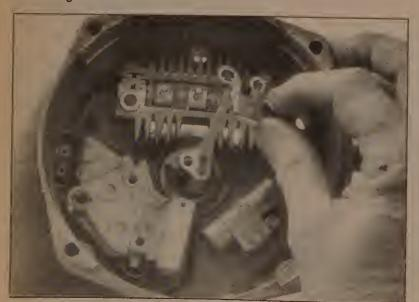
14.5 Remove the screw attaching the diode trio to the end frame and remove the trio
