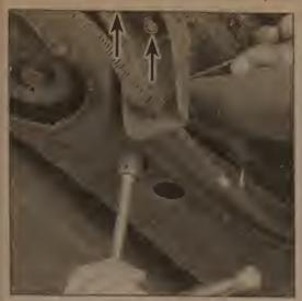
7.18 Remove the angled bracket bolts on both sides of the vehicle (arrows) and the crossmember mounting bolts (being removed here with a socket and back-up wrench)
