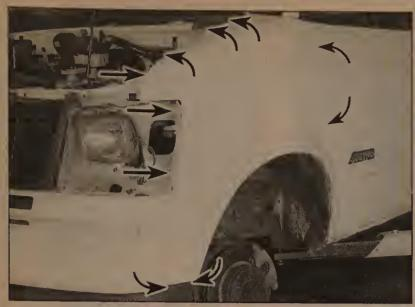
12.7 Remove the fender mounting bolts (arrows). The rear fender bolts (two right arrows) are accessed with the door open
