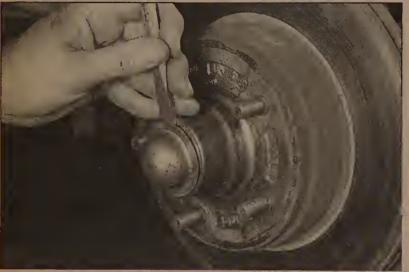
36.6 Dislodge the dust cap by working around the outer circumference with a hammer and chisel
