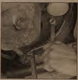
7.15b Remove the converter-to-driveplate retaining bolts (here, a flywheel wrench is being used to prevent the driveplate from turning, but a wrench on the crankshaft vibration damper bolt will also work)
