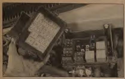
3.2 On 1996 and later models, the Underhood Electrical Center is located inside the engine compartment mounted on the firewall on the driver's side - Fuse and relay circuit identification is located on the underside of the cover
