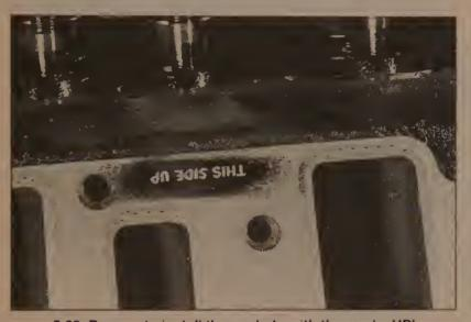
5.32 Be sure to install the gaskets with the marks UP!
