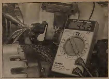
15.125b With the throttle wide open, the voltage should increase smoothly to approximately 4.5 volts (CMFI engine shown)
