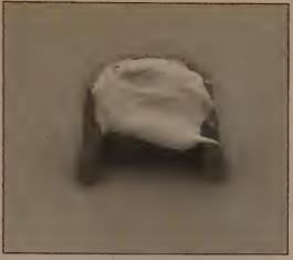
4.17 Keepers don't always stay in place, so apply a small dab of grease to each one as shown here before installation - it'll hold them in place on the valve stem as the spring is released
