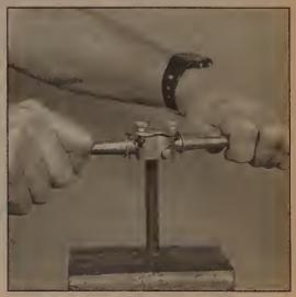
10.23 A die should be used to remove sealant and corrosion from the head bolt threads prior to installation
