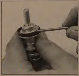
7.15a Pry the secondary piston spring retainer off with a small screwdriver, then remove the seal
