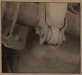
10.2a The left side lower shock absorber mount (if the vehicle is equipped with gasfilled shock absorbers it may be necessary to raise the shock with a jack to insert the bolt through the mounting hole)
