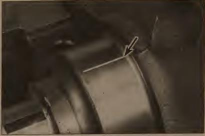
22.10 Lay the Plastigage strips (arrow) on the main bearing journals, parallel to the crankshaft centerline
