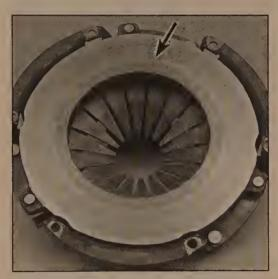
3.14 The machined face of the pressure plate must be inspected for score marks and other damage - if damage is slight, a machine shop can make the surface smooth again
