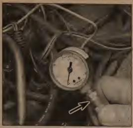
2.4 The oil pressure can be checked by attaching the gauge to the fitting block near the distributor (V6 engine shown)
