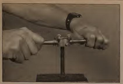
8.22 A die should be used to remove sealant and corrosion from the head bolt threads prior to installation
