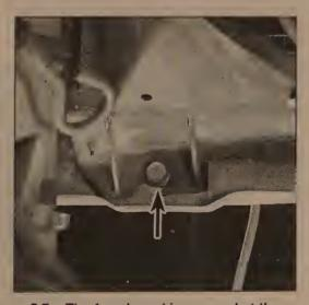
5.7a The fan shroud is secured at the bottom by a bolt in each corner
