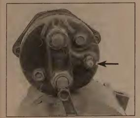
16.6 Typical starter solenoid "S" terminal location (arrow)
