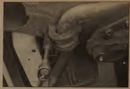
2.3 Remove the stabilizer bar bracket bolts - the nuts are welded to the frame, so there's no need to put a wrench on them to prevent them from turning
