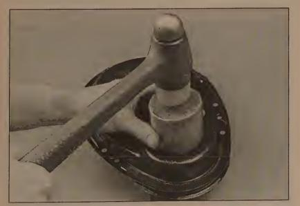
15.8 Clean the bore, then apply a small amount of oil to the outer edge of the seal and drive it squarely into the opening with a large socket and hammer - DO NOT damage the seal in the process!
