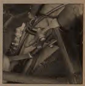
14.5 Use a puller to remove the Pitman arm from the Pitman shaft
