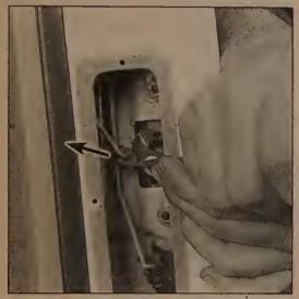
26.4 Push the rod clip off in the direction shown (arrow)
