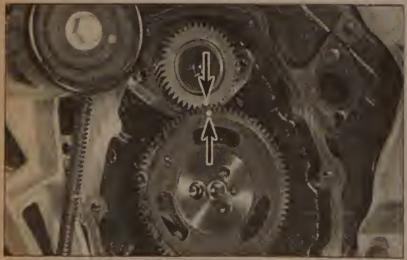
10.14 Before installing the camshaft sprocket, make sure the timing marks on the balancer shaft gears are properly aligned (arrows) Note: Engine set on TDC at number 4 piston
