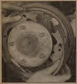
5.4n Spread the shoes apart and slide them into position on the backing plate
