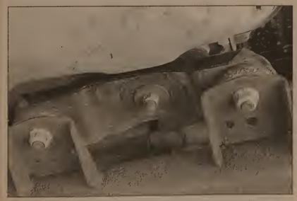
8.3 The transmission mount-to-support bracket nut (center) should be removed before the support bracket bolts are removed
