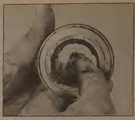
4.6b Lubricate the inner groove and the thrust side (where the release fingers contact it) of the release bearing with high-temperature grease
