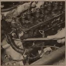
10.17 If the head is stuck, pry it up at the overhang just behind and below the thermostat housing
