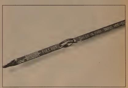
6.6 When checking the automatic transmission fluid level be sure to note the fluid temperature
