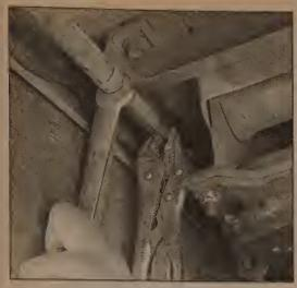
11.4 To adjust the parking brake cable, turn the adjusting nut on the equalizer while preventing the cable from turning with a pair of locking pliers clamped to the end of the adjuster rod
