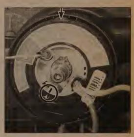
8.14 When properly installed, the airbag coil will be centered with the marks aligned (circle) and the tab fitted between the projections on the top of the steering column (arrow)
