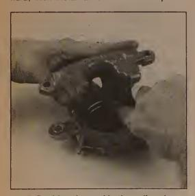
3.15 Position the seal in the caliper bore groove, making sure it isn't twisted
