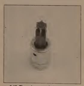
3.13 The valve cover bolts require a , T-30 Torx bit for removal
