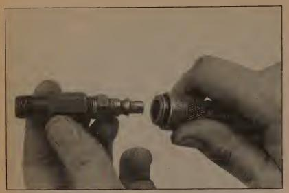
4.4 This is what the air hose adapter that threads into the spark plug hole looks like - they're commonly available from auto parts stores
