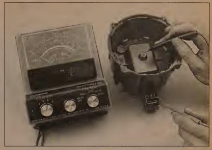
, 9.11a Measuring the HEI ignition coil (in cap) secondary resistance between the rotor button and the TACH terminal
