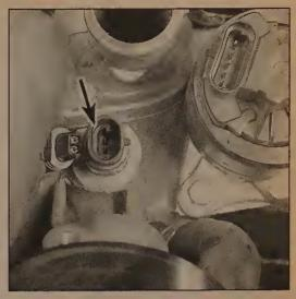
4.22 Engine Coolant Temperature sensor location (arrow) (V6 CSFI engine shown)
