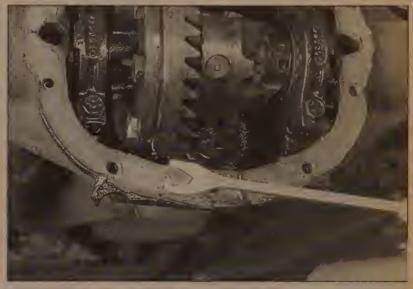
35.8 Carefully scrape the old gasket material off to ensure a leakfree seal with the new gasket
