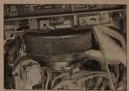
31.5 Lift the air cleaner element out of the housing; on V6 models it's a tight fit
