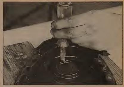
15.6 While supporting the cover near the seal bore, drive the old seal out from the inside with a hammer and punch or screwdriver
