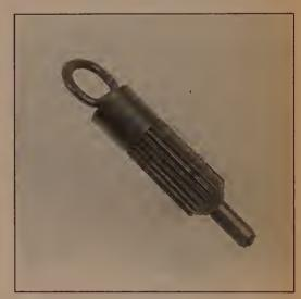
3.16 A clutch alignment tool can be purchased at most auto parts stores and eliminates all guesswork when centering the clutch plate in the pressure plate
