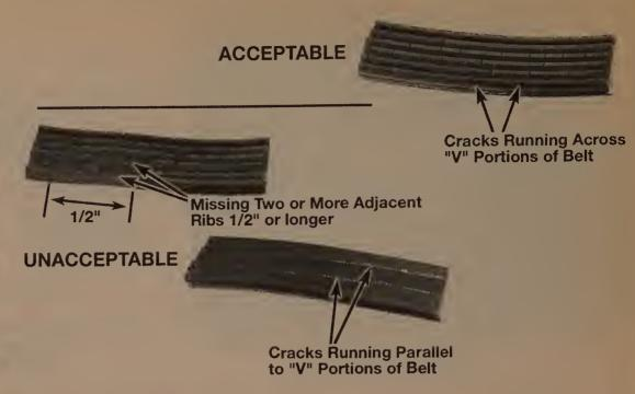
25.3b Small cracks in the underside of a V-ribbed belt are acceptable - lengthwise cracks or missing pieces are cause for replacement
