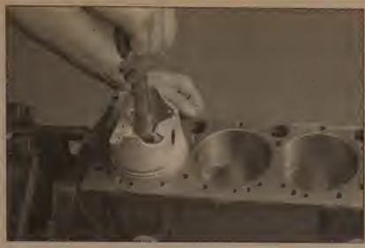
21.3 When checking piston ring end gap, the ring must be square in the cylinder bore (this is done by pushing the ring down with the top of a piston as shown)
