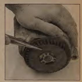
8.31 The filter can be pulled out of the air pump with needle-nose pliers
