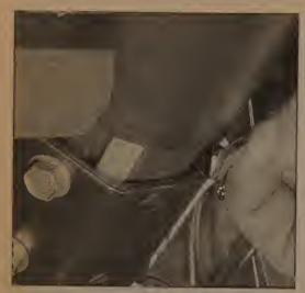
9.4 The instrument cluster shift indicator cable is attached to the steering column shroud
