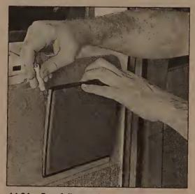
14.24a Carefully pry the rear door speaker grille off with a small screwdriver...
