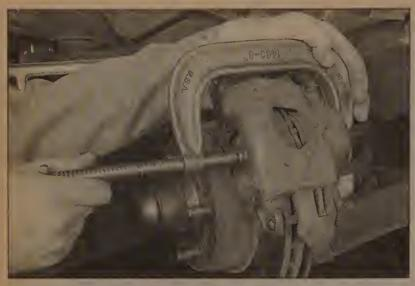
2.5 Using a large C-clamp, push the piston back into the caliper bore - note that one end of the clamp is on the flat area near the brake hose fitting and the other end (screw end) is pressing against the outer brake pad
