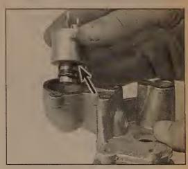
12.8b Note the position of the terminals on top and the dowel pin on bottom of the injector in relation to the fuel meter cover when you lift the injector out of the cover
