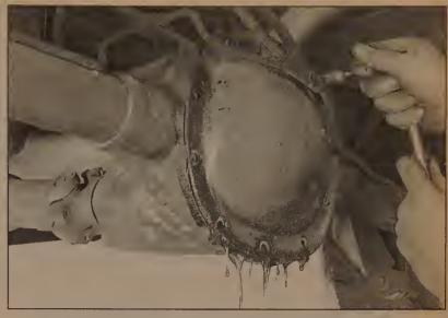
35.6b ... then loosen the top bolts and let the oil drain
