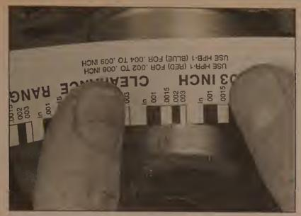
24.13 Measuring the width of the crushed Plastigage to determine the rod bearing oil clearance (be sure to use the correct scale - standard and metric scales are included)
