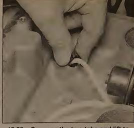
15.38a Squeeze the two tabs and lift to remove the poppet nozzle from the intake manifold (CMFI engine shown)
