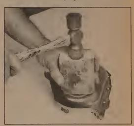
12.8b ... or a block of wood and a hammer - don't damage the seal in the process!
