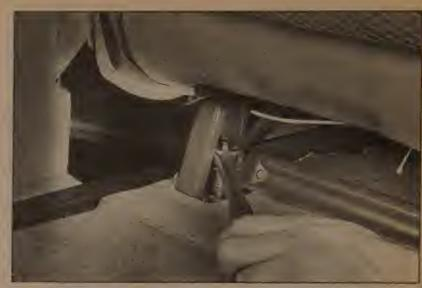
33.3 Use a socket wrench to remove the front seat mounting nuts
