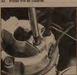
13.5 Remove the injector retaining screw and retainer
