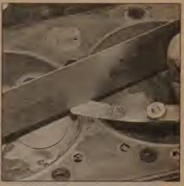
9.12 Check the cylinder head gasket surface for warpage by trying to slip a feeler gauge under the straightedge (see the Specifications for the maximum warpage allowed and use a feeler gauge of that thickness)
