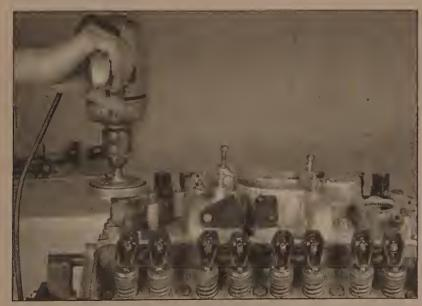
25.5 A drill motor connected to the modified distributor shaft drives the oil pump - make sure it turns clockwise as viewed from above
