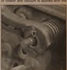
11.7 Make sure the O-ring seal under the retainer is seated in the groove and not twisted before installing the keepers
