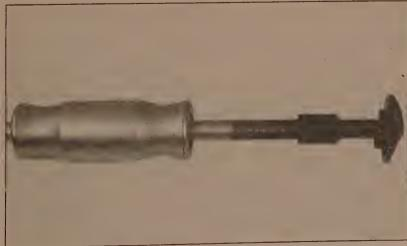
17.2 A slide hammer with a special bearing puller attachment is required to pull the axleshaft bearing from the axle housing
