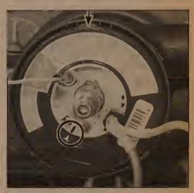
20.17 When properly installed, the airbag coil will be centered with the marks aligned (circle) and the tab fitted between the projections on the top of the steering column (arrow)
