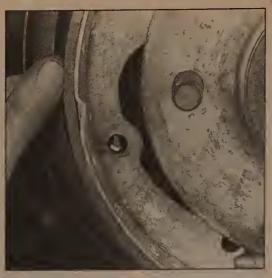
5.40 Install the hold down-pin and spring through the backing plate and primary shoe
