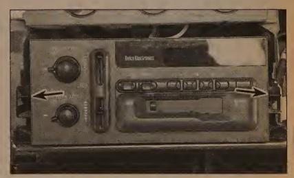
14.7a On 1996 and later models, the radio slides into the mount and is secured on each side by retaining clips (arrows)
