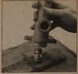
7.9 To remove the secondary piston, tap the cylinder against a block of wood
