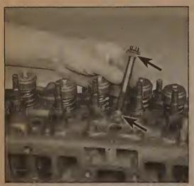
10.25 The cylinder head mounting bolts should be coated with sealant at the locations shown (arrows) before installation
