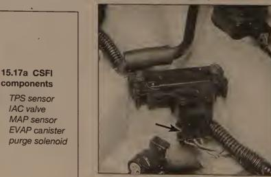
15.17b Disconnect the MAP sensor electrical connector (CMFI engine shown)
