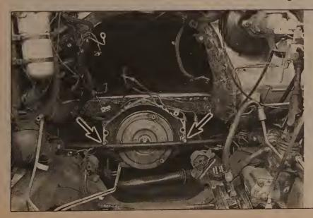
5.38 The automatic transmission torque converter is supported following engine removal by a pipe laid across the frame rails - stick bolts through the holes in each side of the bellhousing (arrows)
