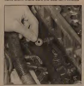
5.13 Don't forget to install new rubber sealing washers around the pushrod cover mounting studs or oil will leak past the studs
