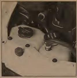
4.8 The engine coolant and windshield washer fluid reservoirs are located next to each other - DO NOT mix them up when adding fluids!
