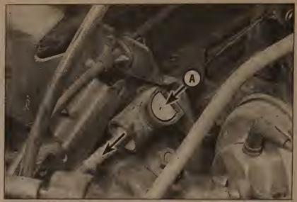
3.8 Depress the throttle valve (TV) cable re-adjust tab (A) and pull the slider back (arrow) until it rests on its stop - release the tab and open the throttle completely
