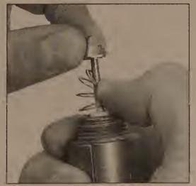
14.41b To adjust an IAC valve without a collar, compress the valve retaining spring while turning the valve clockwise...
