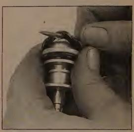
7.15b Remove the secondary seals from the piston (some only have one seal)
