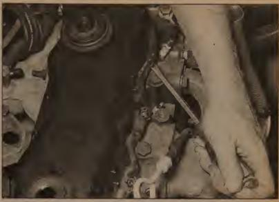
3.11 The rocker arm cover is sealed with RTV - if you have to pry it off the head, try to avoid bending the flange
