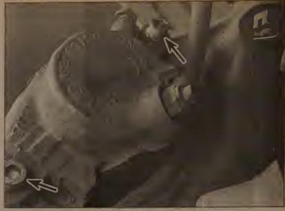
2.6a Remove the two caliper-to-steering knuckle mounting bolts (arrows) (this will require the use of an Allen head socket wrench)
