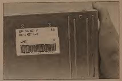
3.8a If you are replacing the PCM compare the service numbers on the label on the old unit to the numbers on the new one
