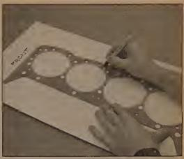
10.15 To avoid mixing up the head bolts, use a new gasket to transfer the bolt hole pattern to a piece of cardboard, then punch holes to accept the bolts...
