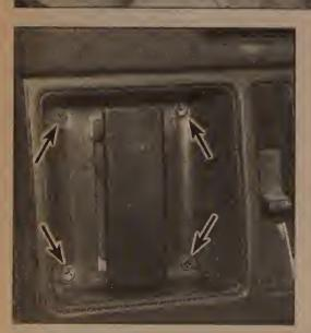
20.25 Remove the side door handle cover retaining screws (arrows)
