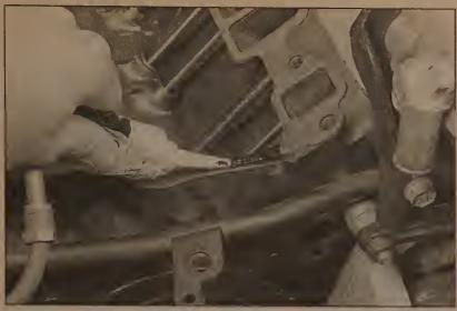
5.30 Apply a 3/16-inch bead of RTV sealant to the front and rear manifold mating surface of the block
