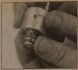
14.21 Slide the new filter onto the nozzle of the fuel injector
