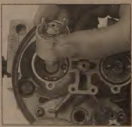
14.25 Make sure that the lug is aligned with the groove in the bottom of the fuel injector cavity
