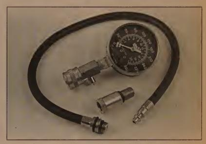
Compression gauge with spark plug hole adapter
