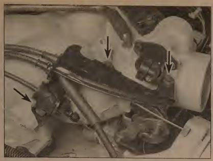
15.20 Remove the three bolts (arrows) from the plenum and lift the cable bracket off the plenum (CMFI engine shown)
