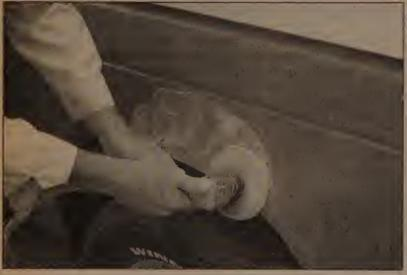
3 Using coarse-grit sandpaper, remove the paint down to the bare metal. Hand sanding works fine, but the disc sander shown here makes the job faster. Use finer (about 320-grit) sandpaper to feather-edge the paint at least one inch around the dent area
