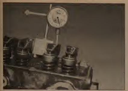
15.3 When checking the camshaft lobe lift, the dial indicator plunger must be positioned directly above and in line with the pushrod
