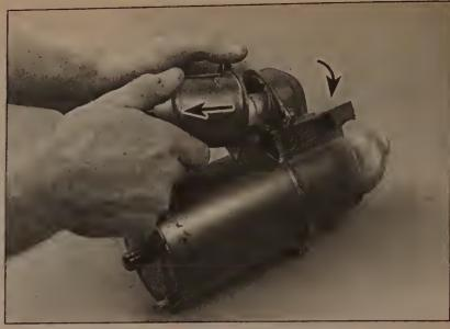
18.5 To remove the starter solenoid from the starter motor, remove the solenoid-to-starter frame mounting screws, then turn the solenoid in a clockwise direction and pull
