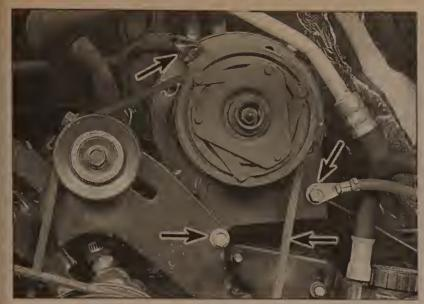
14.6 Detach the wire harness and ground wire (arrows) before removing the compressor drivebelt and mounting bolts (arrows)
