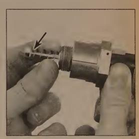
14.41c ... then return the spring to its original position with the straight portion aligned in the slot under the flat surface of the valve
