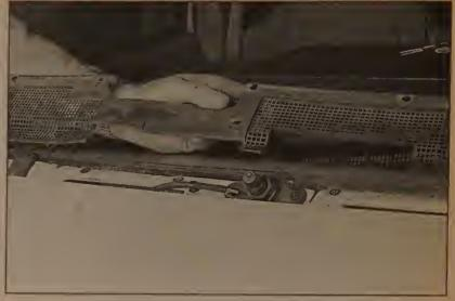
19.3 Remove the retainers and lift the grille out
