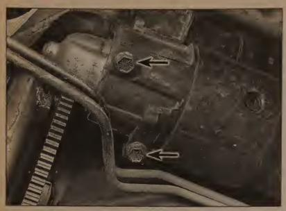
17.5 To remove the starter from the engine, detach the electrical wires from the solenoid terminals, then remove both mounting bolts (arrows)
