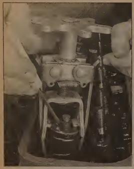
4.8a Once the spring is depressed, the keepers can be removed with a small magnet or needle-nose pliers (a magnet is preferred to prevent dropping the keepers)
