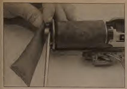
7.18 Inspect the fuel strainer for dirt; if too dirty to be cleaned carefully pry the fuel strainer from the inlet pipe
