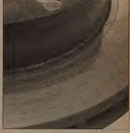
4.3 Check the rotor for deep grooves and score marks (be sure to inspect both sides of the rotor)
