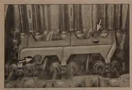
11.11a On 1993 and earlier models with roller lifters, the guide plate is retained by two bolts (arrows). The guide plate presses against the six restrictors that pair the lifters together - be sure all components are reassembled in the same orientation
