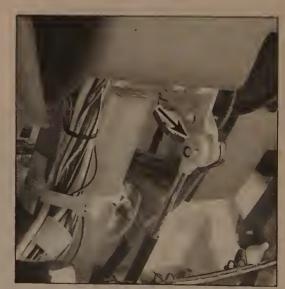
12.12 Use a screwdriver to pry the shift cable end (arrow) from the shift lever at the steering column
