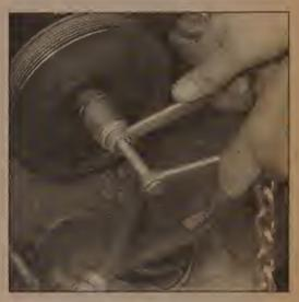
15.16 Using an installation tool (or a fabricated tool, as shown) press the pulley onto the pump shaft until it's flush with the shaft, but no further
