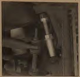
4.4 A special tool, available at most auto parts stores, is required to push the balljoints out of the steering knuckle (an alternative tool can be fabricated from a large bolt, nut, washer and socket)
