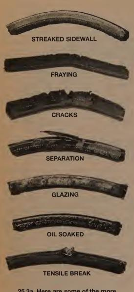
25.3a Here are some of the more common problems associated with drivebelts (check the belts very carefully to prevent an untimely breakdown)
