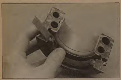
15.15a Using the tool like a "shoehorn", attach the seal section to the bearing cup . . .
