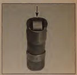
7.13 The roller on roller lifters must turn freely - check for wear and excessive play as well
