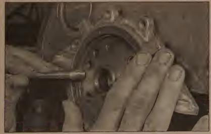
15.26 Lubricate the seal lip, then work it over the crankshaft with a blunt tool, such as the drive end of a socket extension
