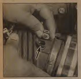
4.30 Intake Air Temperature sensor location (arrow) (V6 CSFI engine shown)
