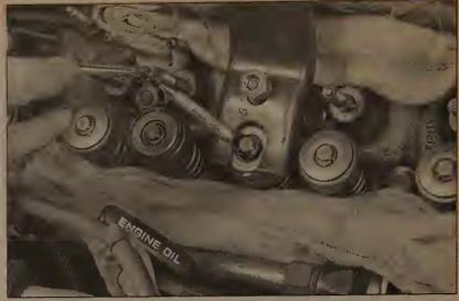
4.8a A lever-type valve spring compressor is used to compress the spring and remove the keepers to replace valve seals or springs with the head installed
