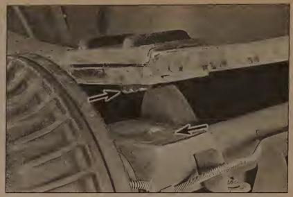
11.13 When raising the axle into position, the lug on the spring must engage with the pocket in the axle
