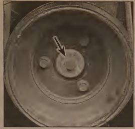
10.2 The vibration damper bolt (arrow) is usually very tight, so use a six-point socket and a breaker bar to loosen it (the three other bolts hold the pulley to the vibration damper)
