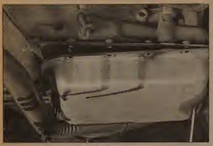
33.7 With the rear bolts in place but loose, pull the front of the pan down to let the transmission fluid drain
