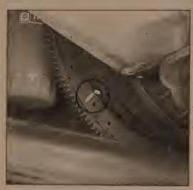
7.15a Mark the relationship of the torque converter to the driveplate
