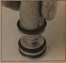
7.16 Install a new spring retainer over the end of the secondary piston and push it into place with a socket
