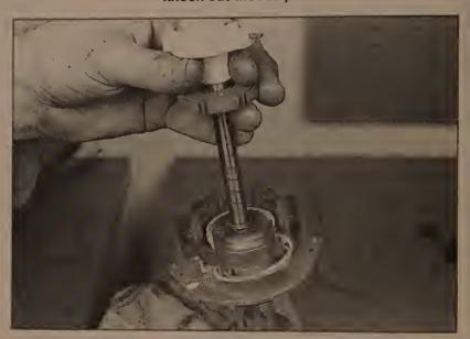
8.10c Remove the shaft from the distributor
