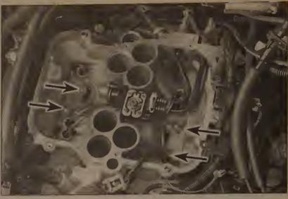
5.26 On CMFI engines, don't forget the 4 bolts (arrows) located inside the lower intake manifold
