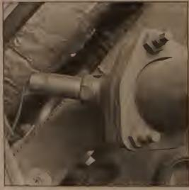
5.1b The oxygen sensor on the V6 engine is located in the left exhaust manifold (TBI engine shown)
