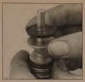
7.15d Install a new primary seal on the secondary piston with the seal lip facing in the direction shown
