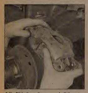
2.6b Slide the caliper up and off the rotor
