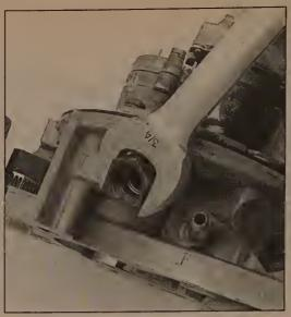
14.50 Remove the fuel inlet and outlet nuts from the fuel meter body
