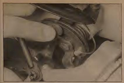
16.9 While pulling the throttle back, lift the accelerator cable from the notch on the throttle valve (CMFI engine shown)
