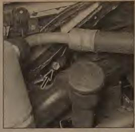
11.1a Use a large screwdriver to unscrew the right side engine cover screw (arrow). . .
