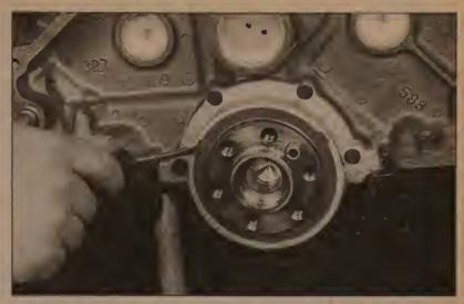
15.23 To remove the seal from the housing, insert the tip of the screwdriver into each notch (arrows) and lever the seal out
