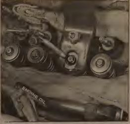
4.8b The stamped steel lever-type valve spring compressor is usually less expensive than the type that grips the spring coils
