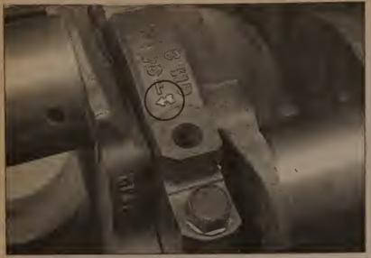
13.4c The arrow on the main bearing cap indicates the front of the engine
