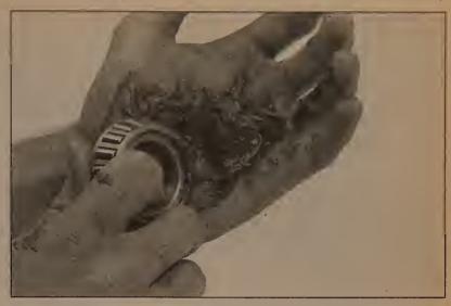
36.15 Work the grease into each bearing until it's full
