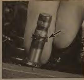
4.9 The O-ring seal (arrow) should be replaced with a new one each time the keepers and retainer are removed
