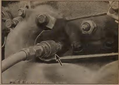
4.4 Use compressed air, if available, to hold the valves closed when the springs are removed - the air hose adapter (arrow) threads into the spark plug hole and accepts the hose from the compressor
