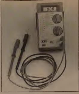
2.1 Digital multimeters can be used for testing all types of circuits; because of their high impedance, they are much more accurate than analog meters for measuring millivoltage-voltage in computer circuits
