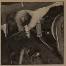
38.2 The PCV valve fits into the rocker arm cover - place your finger over the opening to feel for suction and shake the valve, listening for a rattling sound
