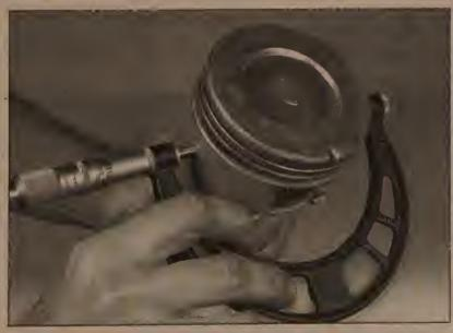
17.11 Measure the piston diameter at a 90-degree angle to the piston pin and in line with it
