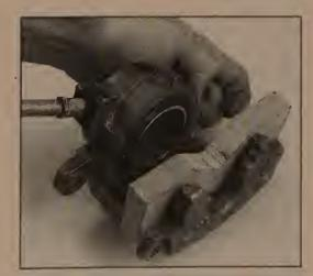
3.8 With the caliper padded to catch the piston, use compressed air to force the piston out of the bore - make sure your hands or fingers are not between the piston and caliper!
