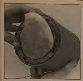
10.8 To replace the canister filter, peel it out and install a new one
