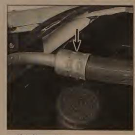
10.1 Air conditioning hoses are best identified by the metal tubes used at all bends (arrow) - DO NOT disconnect or accidentally damage the air conditioning hoses as the system is under high pressure
