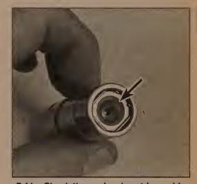
7.11c Check the pushrod seat (arrow) in the top of each lifter for wear
