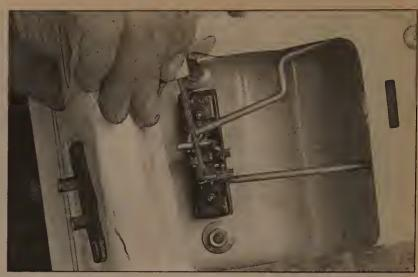
26.9a Push the clip down with a small screwdriver and disengage the rod
