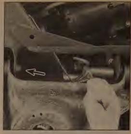
8.7 Remove the control arm mounting bolts (arrow indicates the front pivot bolt)
