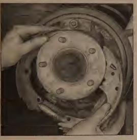
5.4h Spread the top of the shoes apart and slide the assembly around the axle
