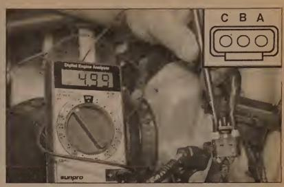
4.50 Checking the MAP sensor reference voltage - the voltage reading should be approximately 5.0 volts (V6 CMFI engine shown)
