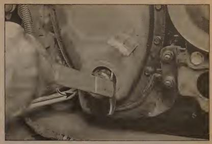
12.2 The front crankshaft seal can be removed in the vehicle with a seal removal tool or a large screwdriver (V6 engine shown four-cylinder similar)
