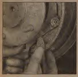
5.4t Install the lever return spring over the tab on the actuator lever, then push the spring up onto the brake shoe
