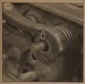
4.16 Make sure the O-ring seal under the retainer is seated in the groove and not twisted before installing the keepers
