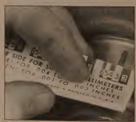
22.14 Compare the width of the crushed Plastigage to the scale on the container to determine the main bearing oil clearance (always take the measurement at the widest point of the Plastigage); be sure to use the correct scale - standard and metric scales are included
