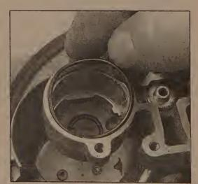
14.24 Lubricate the upper O-ring with transmission fluid then install it on top of the steel washer
