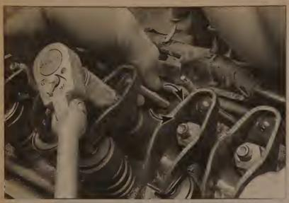
7.13 Rotate each pushrod as the rocker arm nut is tightened to determine the point at which all play is removed, then tighten each nut an additional one full turn
