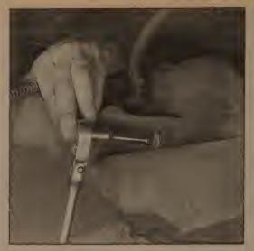
17.2 Use a ratchet or breaker bar and a 3/8-inch drive extension to remove the differential check/fill plug
