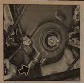
4.15 The crankshaft position sensor (arrow) is located at the bottom of the timing chain cover (V6 engines only)
