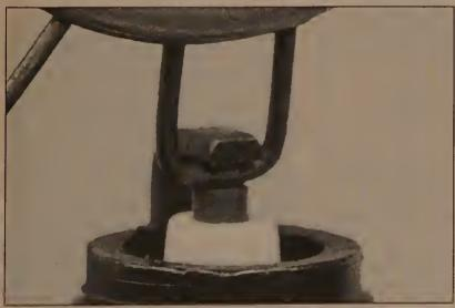
41.5a Spark plug manufacturers recommend using a wire-type gauge when checking the gap - if the wire does not slide between the electrodes with a slight drag, adjustment is required
