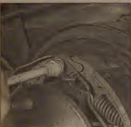
5.4b Remove the shoe return springs the spring tool shown here is available at most auto parts stores and makes this job much easier and safer
