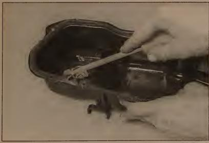
3.12 Remove the old sealant from the rocker arm cover flange and the cylinder head with a gasket scraper, then clean the mating surfaces with lacquer thinner or acetone
