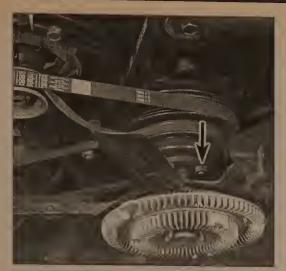
4.12 The fan is attached to the clutch assembly or water pump hub with four nuts or bolts (arrow)
