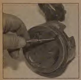
24.8 The notch in each piston must face the FRONT of the engine as the pistons are installed
