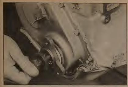
11.9 Use the pulley hub bolt to press the hub onto the crankshaft
