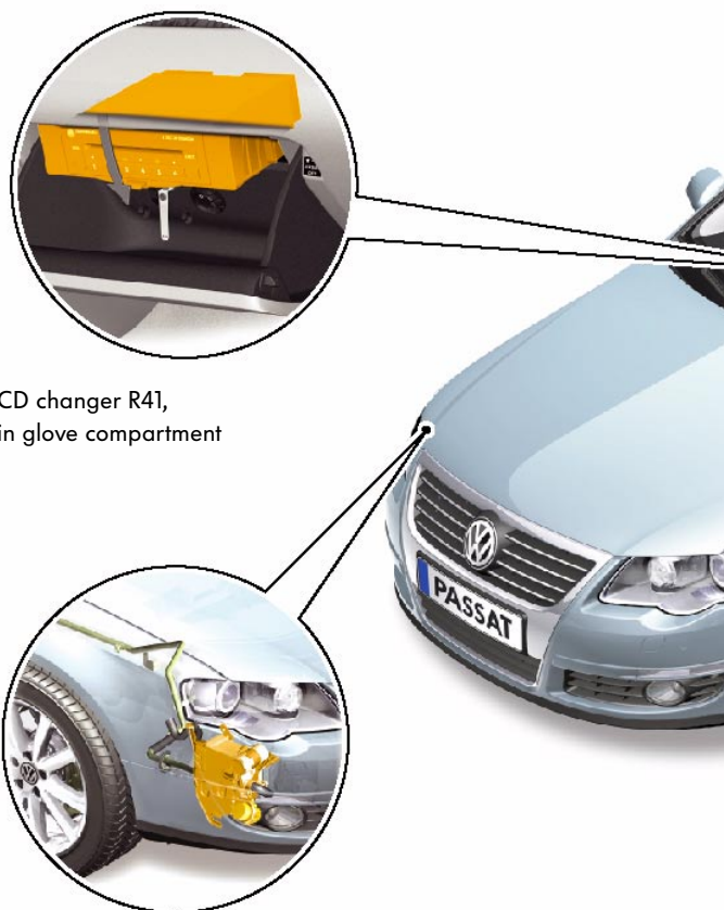
Auxiliary heater control unit J364, in right wheel housing
