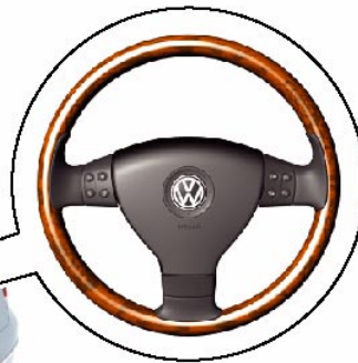
Multifunction steering wheel control unit J453, in the steering wheel
