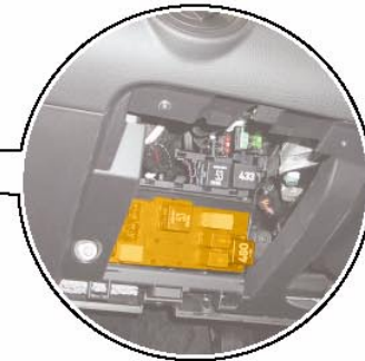
Relay carrier on onboard power supply control unit, on left under dash panel
