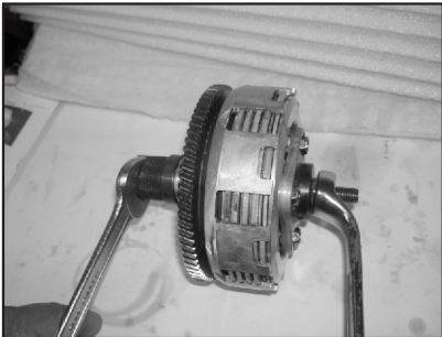
Clutch Dismantling Tool Part No. : F4 1AJA 58 Application : To dismantle & assemble clutch assembly.
