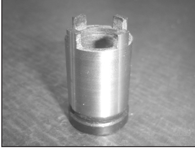
Socket for Clutch Nut Part No. : 37 10DJ 43 Application : To loosen / tighten special nut securing clutch.
