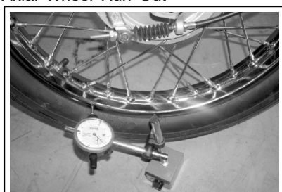
Axial Wheel Run Out
