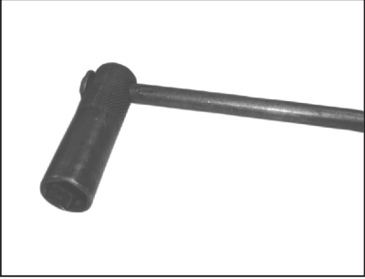
Spark Plug Spanner Part No. : 37 1040 51 Application : For removing and refitting spark plug.
