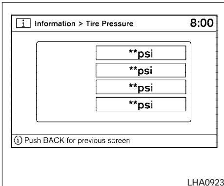
Tire pressure rises and falls depending on the heat caused by the vehicle's traveling condition and the temperature.
