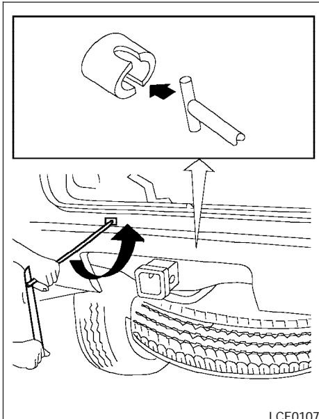
5. Fit the square end of the jack rod into the square hole of the wheel nut wrench to form a handle.
