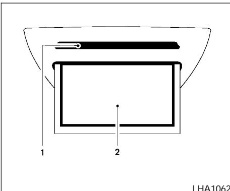
1. Infrared transmitter lens\*
