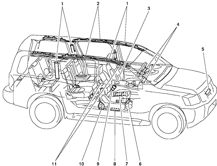
1. Roof-mounted curtain side-impact and rollover supplemental air bag inflators (if so equipped)
