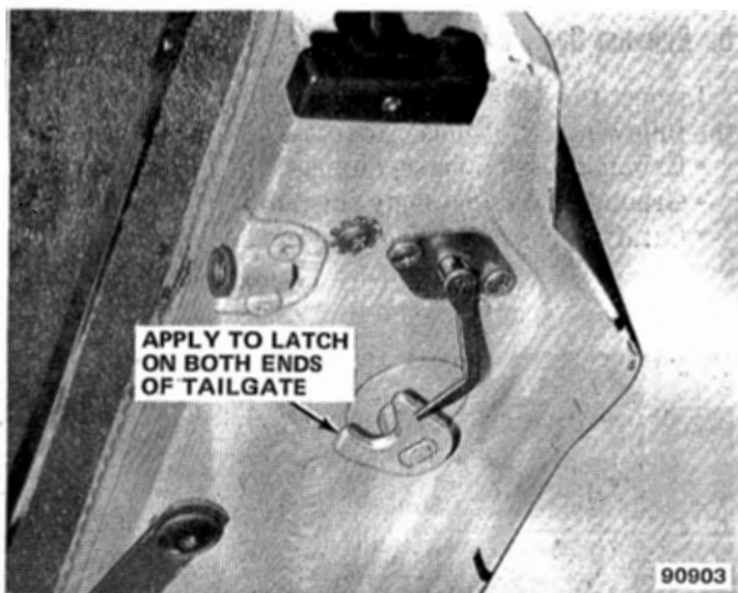
Fig. B-17 Tailgate Lubrication Points—Cherokee-Wagoneer Models
