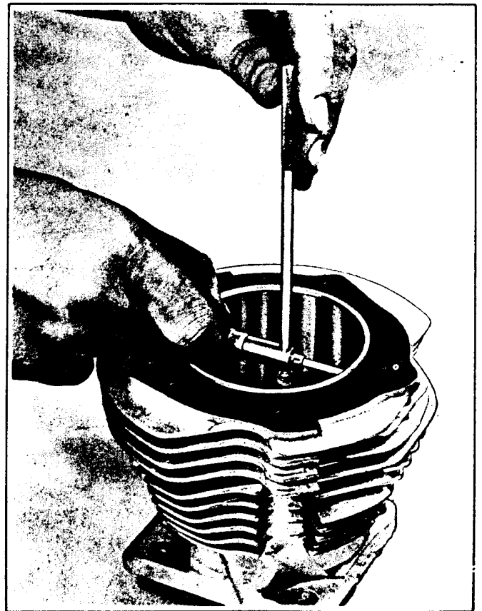
Figure 3C-4. Measuring Cylinder Bore
