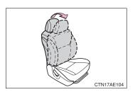
When you have to use a child restraint system in the front passenger seat, adjust the seatback to the most upright position.
