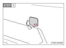
Remove the eyelet cover by pushing outside of it.
