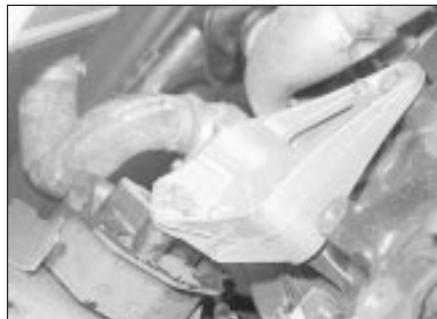
23.20b Engine/transmission right-hand mounting
