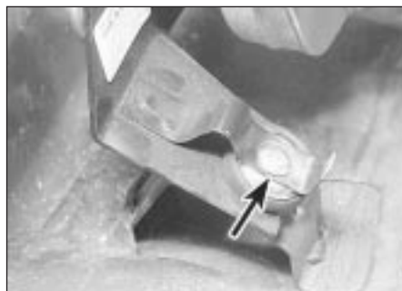
20.7 Wiper motor securing screw (arrowed)
