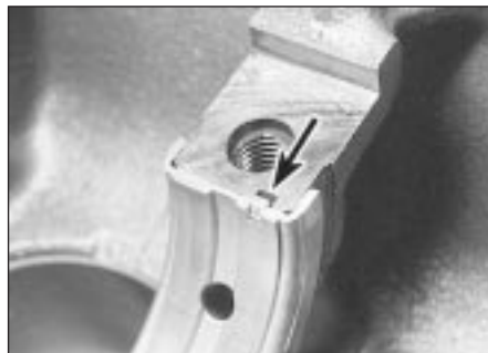
20.10 Main bearing shell correctly fitted, with tag and groove (arrowed) engaged
