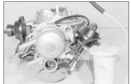
22.2b 2E3 carburettor - choke cover side view
