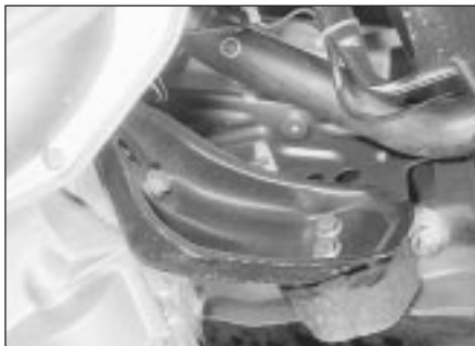
23.20a Engine/transmission left-hand mounting
