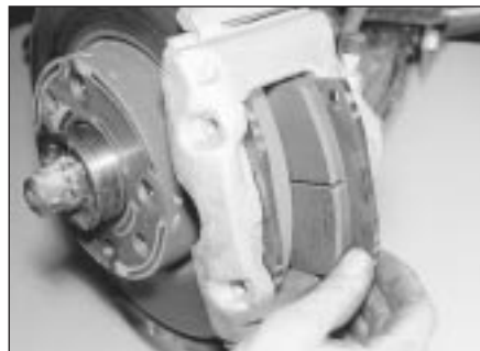
4.6 Removing the inboard pad
