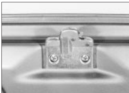
26.2 Boot lid lock securing screws
