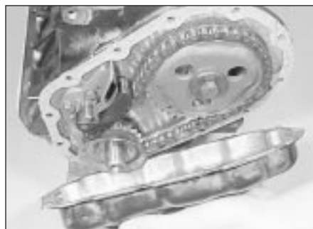
14.21 Refitting the timing cover
