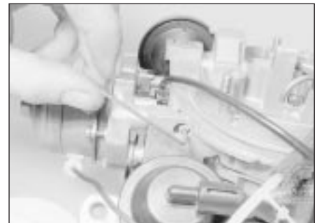
15.9b Choke pull-down adjusting screw
