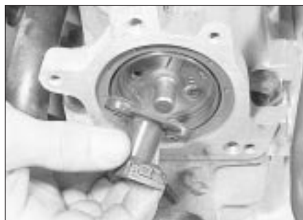
3.10b . . . and remove the rotor
