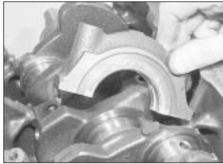
20.16a Fitting a main bearing cap
