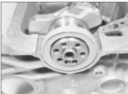
20.15a Crankshaft rear oil seal
