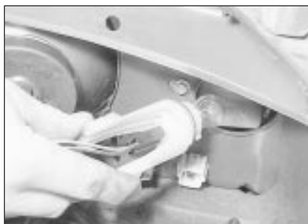
11.9 Removing a direction indicator bulb and holder
