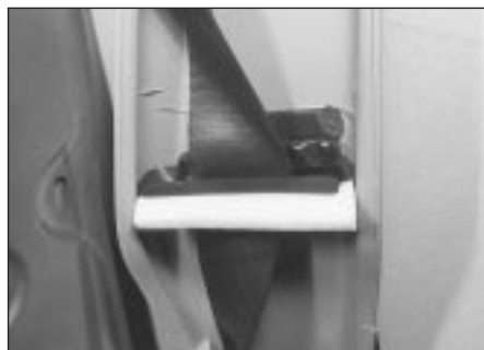
37.6b Belt feeds through guide in pillar trim
