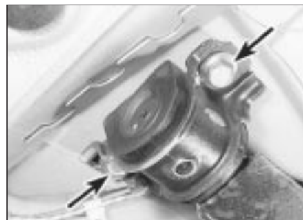
5.4 Control arm clamp bolts (arrowed)
