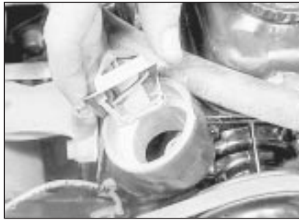
4.3b . . . and withdraw the thermostat - 1.2 litre model
