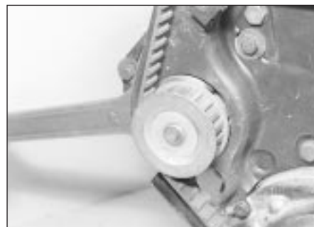
7.9 Swivelling the water pump using a spanner on the flats
