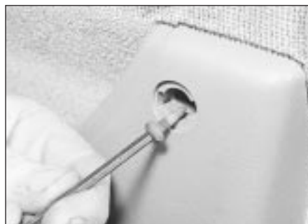
12.5b Removing a door pocket screw
