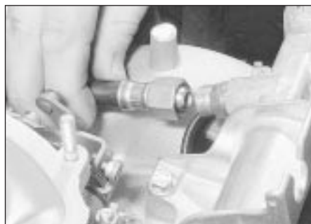
12.60 Disconnecting the fuel supply line from the fuel rail
