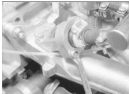
12.8 Undoing a fuel injector retaining bolt
