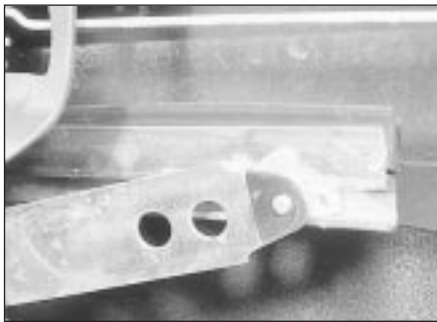
18.6 Scissors lifting mechanism slider
