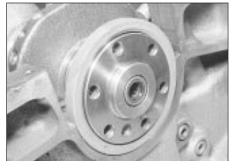
20.14 Crankshaft rear oil seal
