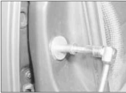
13.4 Adjusting a door lock striker
