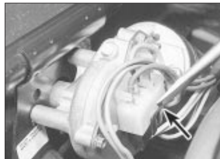
20.6 Releasing the wiper motor electrical plug
