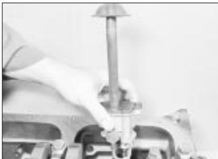
12.2b . . . and remove the oil pump
