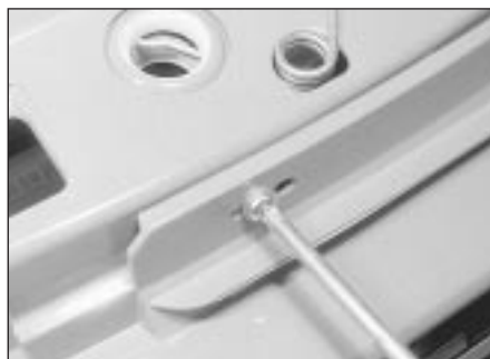
8.2 Undoing a front trim panel screw
