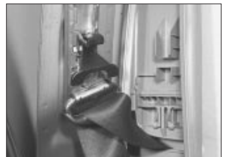
37.6a Front seat belt adjustable top mounting
