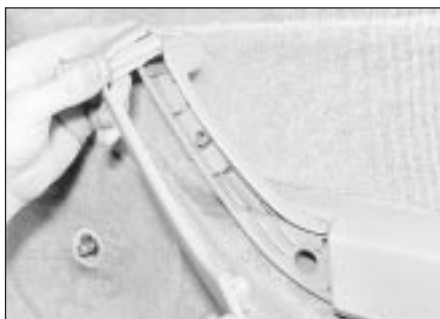
12.6a Removing the armrest screw cover
