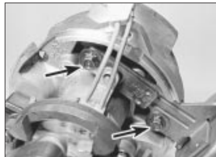
4.5 Vacuum unit retaining screws (arrowed)
