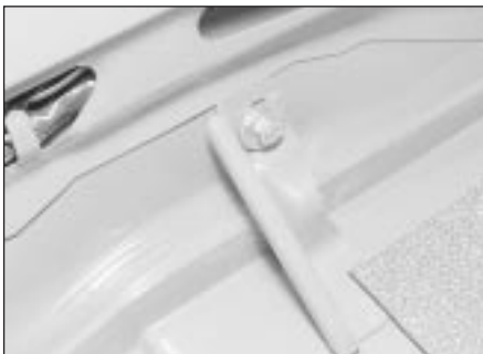
9.2 Rear trim panel securing nut
