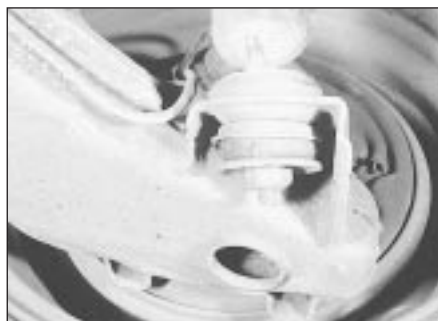
12.13 Rear shock absorber lower mounting - Estate
