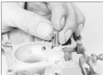
21.8 Removing the accelerator pump delivery tube
