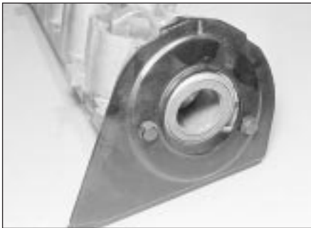
9.7 Camshaft belt cover backplate (1.3 litre engine shown)
