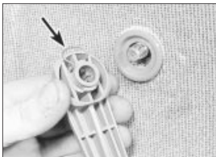
12.2 Window winder handle spring clip (arrowed)
