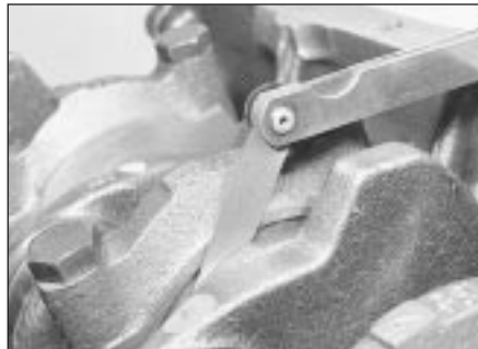
20.19 Checking crankshaft endfloat
