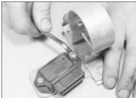
7.3 Unbolting the ignition module (1.8 litre model shown)
