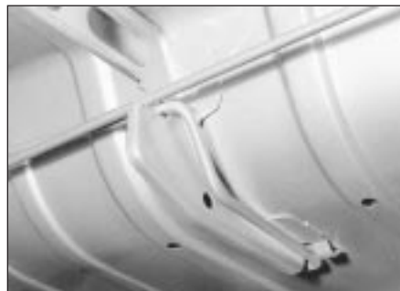
25.5a Torsion rod central housing bracket
