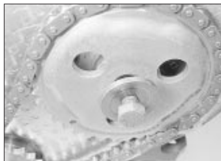
14.10 Camshaft sprocket retaining bolt and washer
