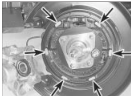
20.6 Anti-seize compound applied to rubbing points (arrowed)
