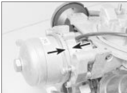
15.12 Choke cover alignment marks (arrowed)
