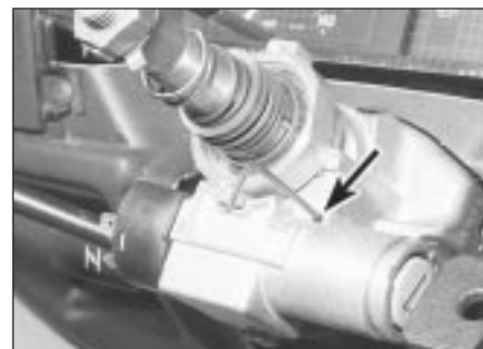
23.6 Releasing the steering lock detent spring with an Allen key (arrowed)
