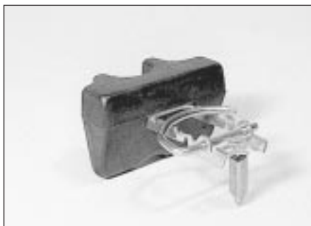
23.13 Float and needle valve
