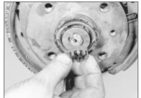
10.6b . . . the washer and the castellated nut
