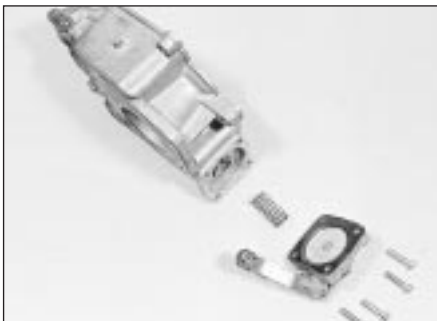
19.9 Accelerator pump components
