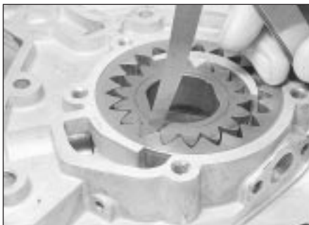
14.2 Checking oil pump gear teeth backlash
