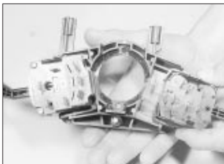
4.14b Unclipping a steering column switch - assembly removed for clarity
