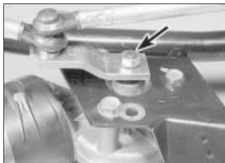
20.8a Wiper motor spindle nut (arrowed)
