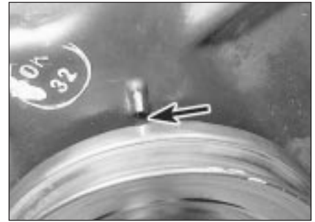
7.7 Ignition timing marks (arrowed) in alignment
