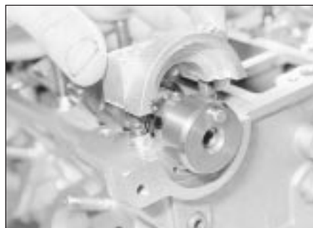
10.11 Fitting a camshaft bearing cap
