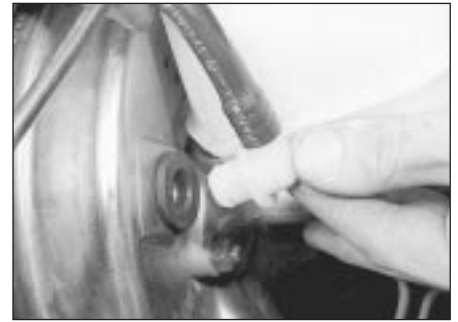
15.3 Brake servo vacuum connection at servo
