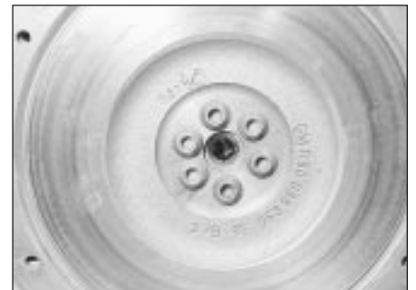
16.4 Flywheel retaining bolts are socket-headed
