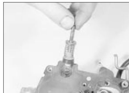
23.10 Accelerator pump plunger and spring
