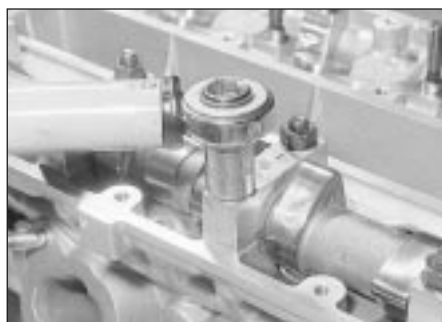
10.12 Tightening a camshaft bearing cap nut
