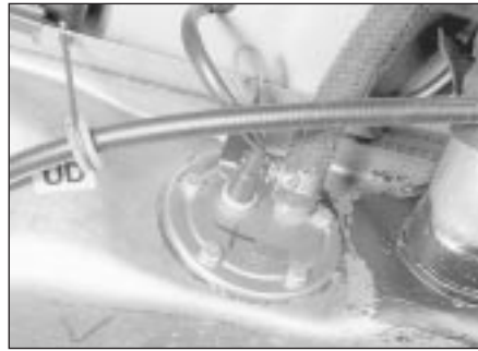
6.3 Fuel gauge sender unit secured by bolts
