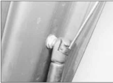
22.2 Releasing a tailgate strut spring clip
