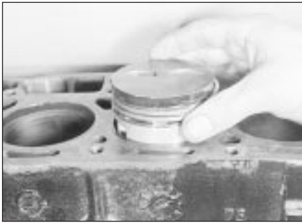
15.11 Offering the piston to the bore
