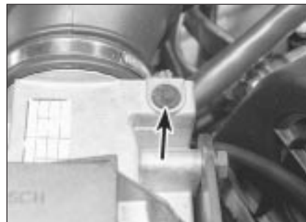
11.13 On 1.8 litre fuel-injected models the mixture adjustment screw is located under the cap on the airflow sensor
