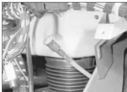
10.2 Speedometer cable at instrument panel end
