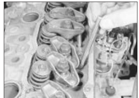
8.17 Removing the pushrods
