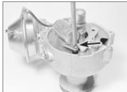
7.5 Undoing the condenser retaining screw
