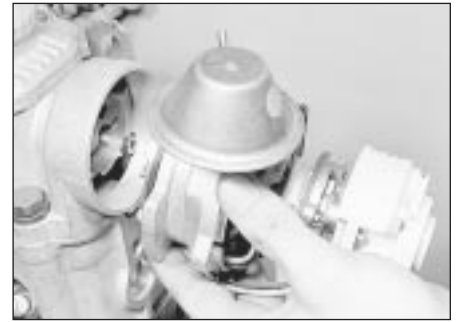
3.5 Removing the distributor from the camshaft housing
