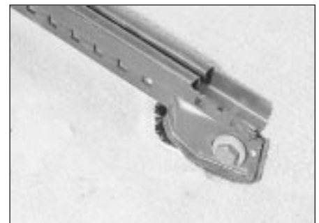
31.2b Seat rail rear retaining bolt (one of two)
