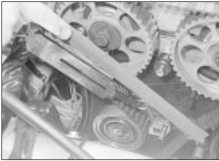
7.18 Checking the belt tension using a spring balance and ruler
