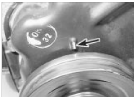
6.3 Ignition timing marks (arrowed) in alignment
