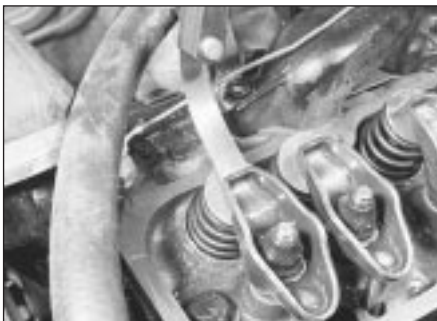
7.10 Checking a valve clearance
