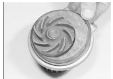
5.17 Fitting a new sealing ring to the pump
