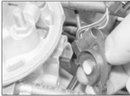
11.3b Throttle valve potentiometer removal
