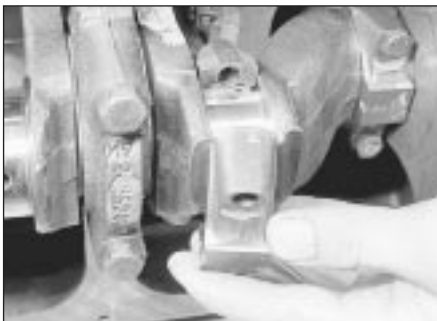
15.14a Fitting a big-end bearing cap
