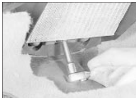
9.17a Removing the heater matrix lower screw
