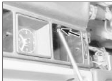
10.3 Removing a centre vent housing screw
