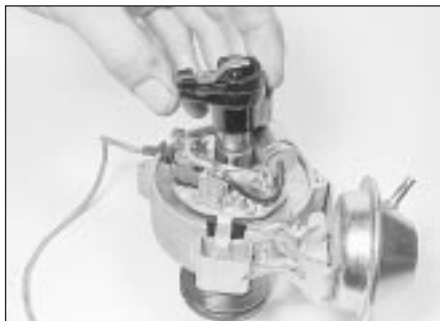
4.2 Removing the rotor arm
