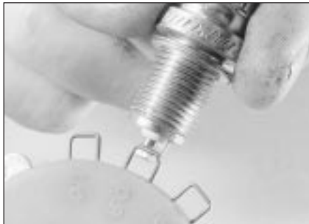
7.10b Measuring a spark plug electrode gap using a wire gauge
