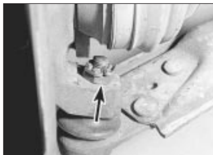
5.3 Control arm balljoint nut (arrowed)
