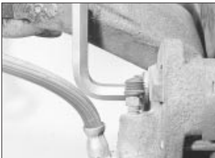
10.6b . . . then unscrew the caliper bolts . . .
