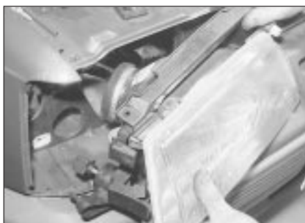
12.3c Removing a headlamp lens
