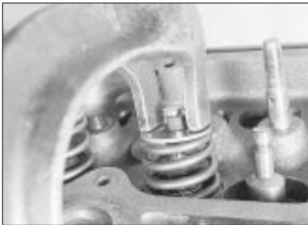
9.20 Compress the spring and fit the collets
