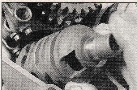
18.3 Disengage the shift fork guide pins from the shift drum and remove the drum
