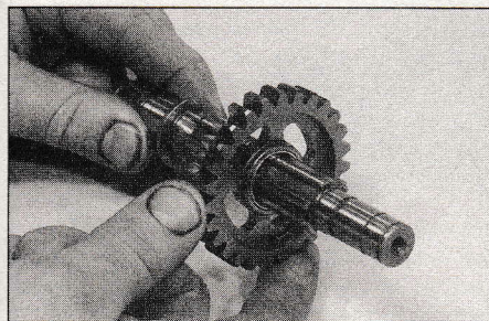
19.25b . . . and slide on second gear pinion with flat side against shaft collar . . .
