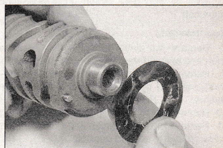
18.12 Disc fits over neutral contact pin in the end of shift drum - note locating hole in disc
