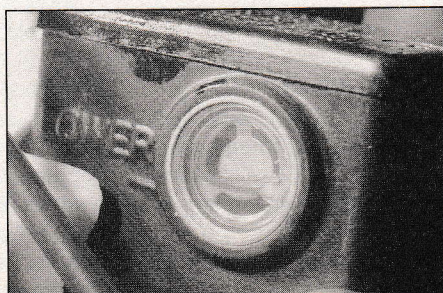
3.9 Front brake master cylinder fluid level must be above line cast in reservoir with the bike held upright on level ground
