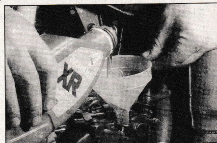
3.5 Transmission oil is topped up via filler cap on top of right-hand engine cover
