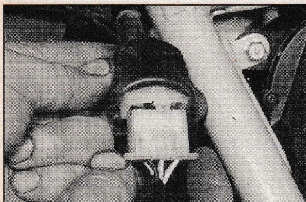
5.22a Trace and disconnect engine wiring at the connectors (alternator and neutral switch wire connector shown)
