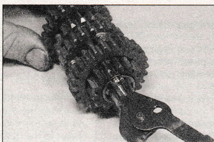
19.23b . . . and secure with a new circlip
