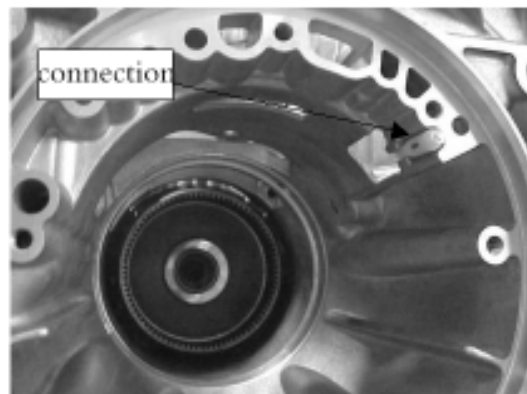
Figure 8.16 Connecting position of coil 7
