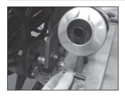
Clean the silencer drain hole by using silencer drain hole cleaning tool as shown in photograph.
