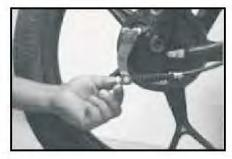
Loosen nut securing front brake cable (14mm AF) & take out the front brake panel assembly.
