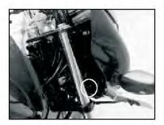
Remove 4 nos. bolts of head light fairing mounting.
