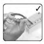
Use only distilled water to top up battery.
