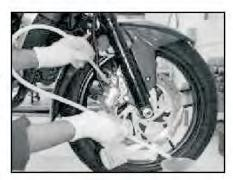
· Drain brake fluid from caliper assembly by opening air bleeder screw.
