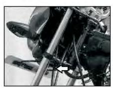
• Route the speedometer cable with grommet through 'U' type clamp provided on lower T.
