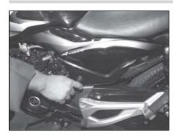
Remove LH Side panel by using vehicle key.
