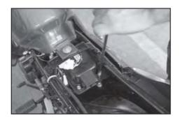
Remove the air filter cover rear side two bolts / screw by using the 10 mm T spanner.
