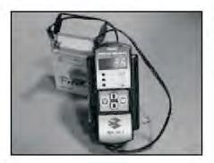
Connect Battery tester clamps to battery terminals, observing correct polarities.
