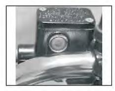
Conduct the brake bleeding procedure & maintain the brake fluid level above MIN. mark.
