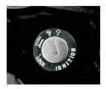
To Lock the Steering: Turn the handle bar to the left or right. Push & Rotate the key to "LOCK" position & remove the key.
