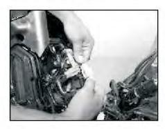
Remove speedometer cable, Headlamp assembly wiring harness coupler connections & take out headlamp assembly
