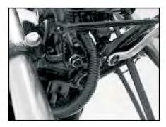
· Remove 2 nos. front number plate mounting bracket nuts.
