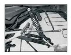
Remove lower bolt of LH & RH RSA & take out LH & RH chain adjuster.
