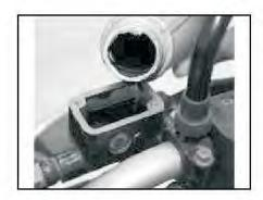
• Fill the master cylinder reservoir by using DOT-3 / DOT-4 brake fluid.
