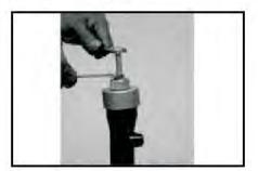
Tighten the special tool 17mm nut by holding 12 mm nut so that special tool lug holds the oil seal.
