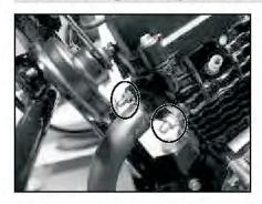
Remove silencer by removing 2 nos. mouth holding bolts & 1 no. silencer bracket bolt.
