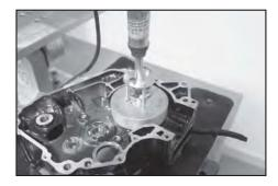
• Before re-fitment of crankshaft assembly, heat the clutch side crankcase with heater at 1500 C then fit the crankshaft assembly.
