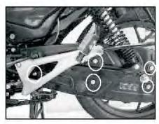
Remove chain cover by removing 3 nos. each flange bolt by 10 mm T spanner.
