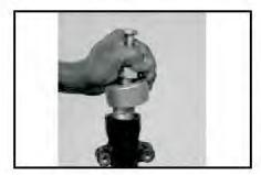
Insert oil seal extraction special tool in outer tube.
