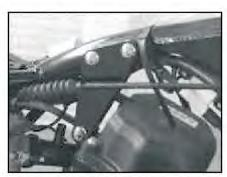
· Connect the accelerator cable at carburettor end as shown in photograph.
