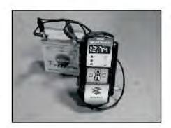
Voltage indication and green & yellow LED's are glowing-Battery is partially charged. Charge the battery using Metafab make VRLA battery charger
