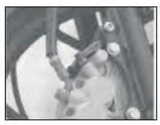
First remove hose pipe by removing banjo bolt & then remove caliper assembly from fork mounting location.
