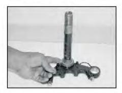
• Lubricate lower cone & ball bearings by HP Lithon RR-3 grease.
