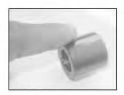
· Smear silicon grease on piston OD & rubber seals.
