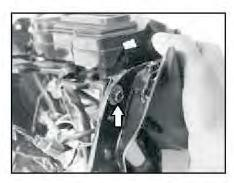
Remove 2 nos bolts mounted on fairing structure LH & RH with 10 mm T spanner.
