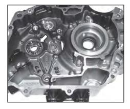
By using Bearing driver set 37103061 Remove
