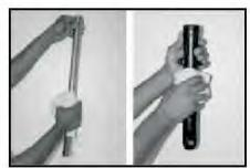
Before re-fitment, clean Fork leg assembly thoroughly with diesel.
