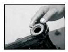
• Lubricate upper cone & ball bearings by HP Lithon RR-3 grease.
