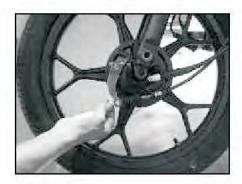
Remove front brake cable & take out front wheel.
