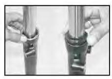
· Assemble the Oil seal lock & dust seal.
