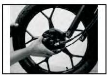
Tighten14 mm nut securing front brake cable & Refit the front brake panel in front wheel.
