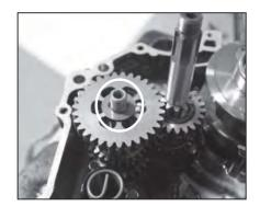
Assembly of I/P & O/P shaft thrust washers
