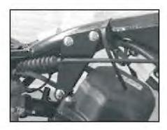
Route accelerator cable from out side the engine top mounting hanger as shown in photograph.
