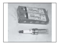
Replace spark plug as per the interval given in the Periodic Maintenance Schedule.
