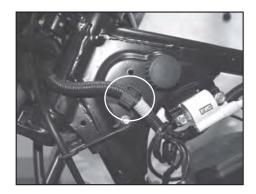
Route wiring harness through button clamp located near LHS petrol tank rubber damper.
