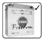
Al ways maintain electrolyte level between maximum & minimum level marks.
