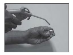
Clean sediment bowl thoroughly with low pressure compressed air & nylon brush.
