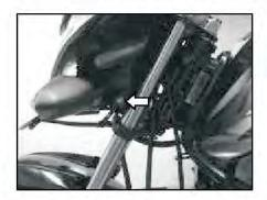
Remove Headlamp assembly mounting bolts (2 nos) mounted on LH & RH side of bracket lower hinge by 10 mm T spanner.
