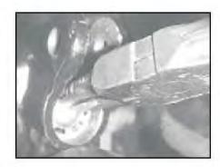
· Insert the circlip with help of plier.
