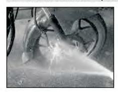
· Clean brake system by keeping nozzle in spray mode.
