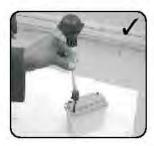
Use hydrometer for checking specific gravity
