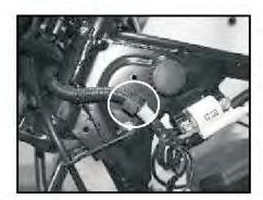
Route wiring harness through button clamp located near LHS petrol tank rubber damper.
