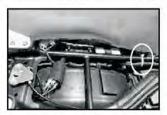
Clamp wiring harness near air filter using PVC clamp.
