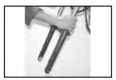
· Assemble front fork leg assembly on vehicle
