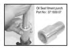
Replace oil seal fitment punch if nylon sleeve found damaged
