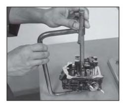
Using Valve Spring compressor Remove
