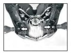
Remove front LH & RH side indicators by removing 2 nos nuts with 14 mm open ended spanner & take out fairing structure LH & RH.
