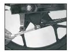
· Remove torque rod nut by removing split pin.
