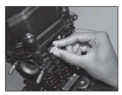
Refit spark plugs by doing pre-fitment manually & thereafter use spanner for tightening.
