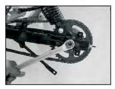
Remove bearing carrier nut & take out coupling along with rear sprocket.
