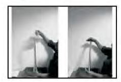
Pour diesel in fork inner pipe by closing other end with hand.
