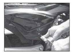
Remove the Screw of RH Side panel and take out the panel.
