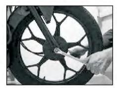
· Remove front axle bolt & take out front axle.
