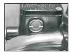
During this process continuously monitor and maintain the brake fluid level in the master cylinder reservoir slightly above the minimum mark.
