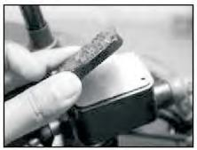
· Remove PVC Cap & rubber diaphragm.
