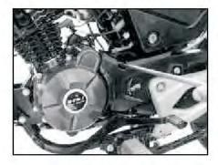
Remove small sprocket cover by removing 2 nos. bolts by 8 mm T spanner.
