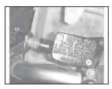
Keep the container below the master cylinder for oil collection during opening.
