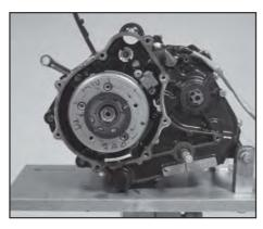
Skill Tip: Always put plastic cap on starter clutch rollers while removing nut & pulling out rotor.
