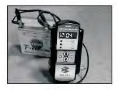
Voltage Indication & yellow LED is glowing-Battery is discharged. Charge the battery using Metafab make VRLA battery charger
