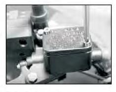
· Remove reservoir cover by removing 2 nos. phillips head screws.
