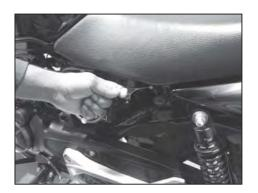
Remove the seat assembly by pulling seat lock cable.
