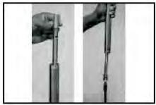
· Assemble the oil lock cap & fork inner pipe.
