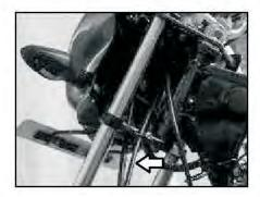
Route the front brake cable along with speedometer cable up to speedometer.
