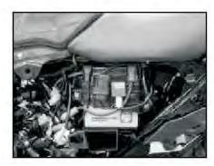
Disconnect battery terminals. Always remove negative wire first, then remove positive wire
