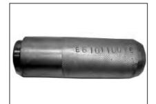
Driver for Fitting Bushing Gear Shift
