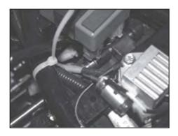
Remove the air filter cover front side bolt / screw by using the 10 mm T spanner.
