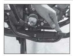
Check the smooth operation of rear brake pedal.
