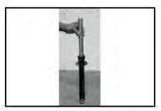
Remove cylinder piston holder & hold the fork leg assembly as shown in photograph.
