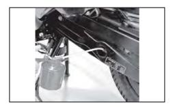
Lubricate chain with SAE 90 oil. Ensure oil is directed on to the ends of the bushes & links on either side.
