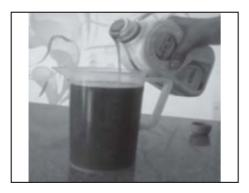
In case oil top up is required, add required qty of fresh to match 1000 ml volume & refill in engine.
