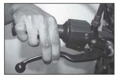
Check the smooth operation of front brake lever.
