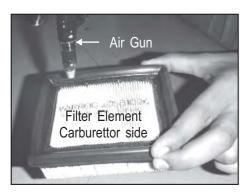
Clean the paper filter element as per the SOP. Use low pressure point (1.75 Bar) for paper filter cleaning.
