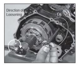
Using Special Socket for clutch nut F41ZJA54 Remove
