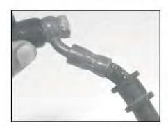
Remove the hose pipe fitment benjo bolt from both ends (master cylinder & caliper assembly)
