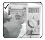
Check open circuit voltage by multi meter.
