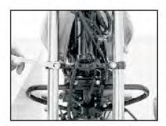
· Loosen under bracket assembly bolts.
