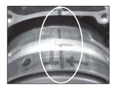
Aligning TDC Position marks for Valve Timing
