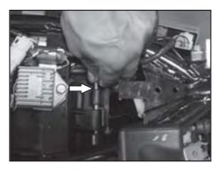
Per-fit the long pivot bolt / screw by hand & tighten the rear side bolt / screw.
