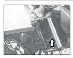
· Route the cable from outside of rod joining lamp shade.
