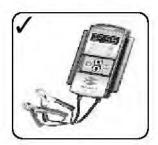
Use midtronics battery tester for checking battery charge condition.
