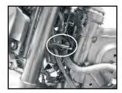
Route wiring harness beneath the rod joining lamp shade through LHS.
