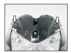
Remove 2 nos allen bolts mounted on headlamp fairing by 4 mm allen key.
