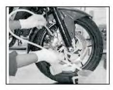
Drain the brake fluid from caliper assembly by loosening air bleeder screw & using transparent PVC tube which will avoid spillage of brake fluid on caliper body / disc pads & also powder coating peel off / inefficient braking.
