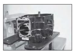
Spit the crankcase & remove crankshaft assembly.
