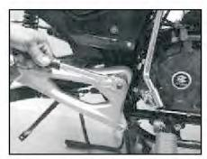
· Remove nut of swing arm shaft.
