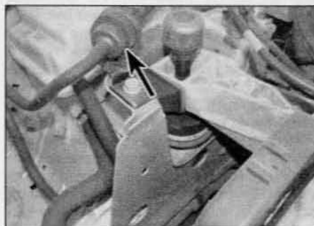
2.7 On early models, the purge valve (arrowed) is located on the right-hand side of the engine compartment
