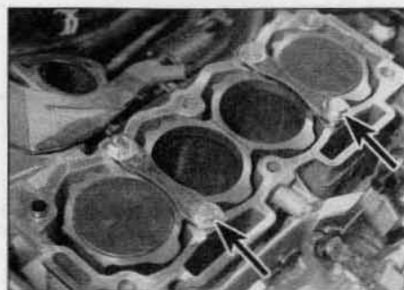
11.17 Clamp the cylinder liners in position before rotating the crankshaft (clamps arrowed) – 1.4 litre engines
