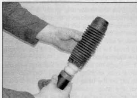
5.8b Fit the piston dust cover . . .
