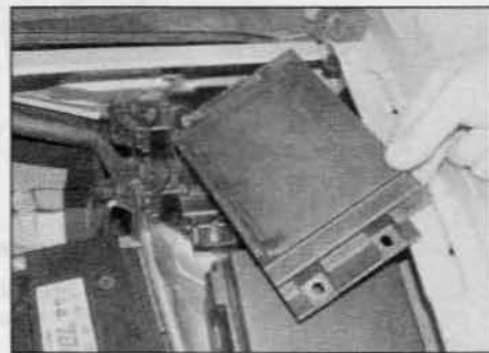
12.14b . . . and lift off the ECU cover – later 1.9 litre models
