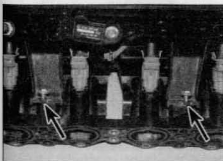
13.14 Undo the two bolts (arrowed) and remove the fuel rail from the manifold – 1.6 litre models
