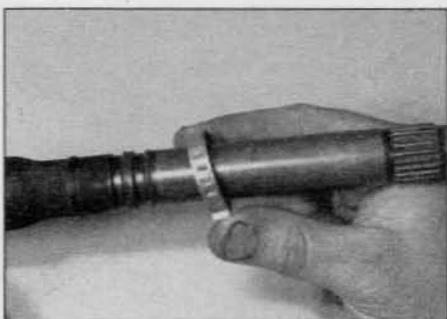
3.21a Slide on the inner retaining collar ...
