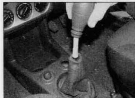
29.5 Twist and remove the gear lever knob off the gear lever
