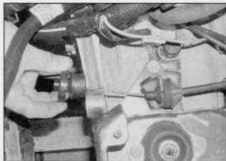
2.3a On MA5 and BE3/5 transmissions, release the clutch inner cable end fitting from the release fork lever . . .
