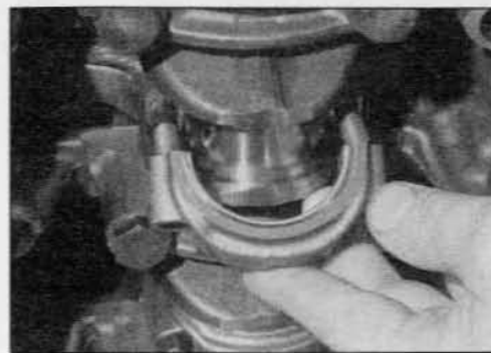
10.5 Removing a big-end bearing cap and shell
