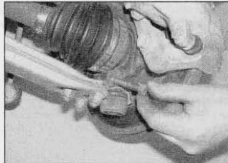
2.8 Undo the nut and withdraw the lower suspension arm balljoint clamp bolt from the swivel hub
