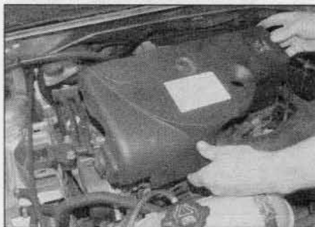
4.1c ... then remove the cover from the engine – 1.9 litre engines
