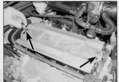
4.5a Remove the spacers (arrowed) from the studs . . .
