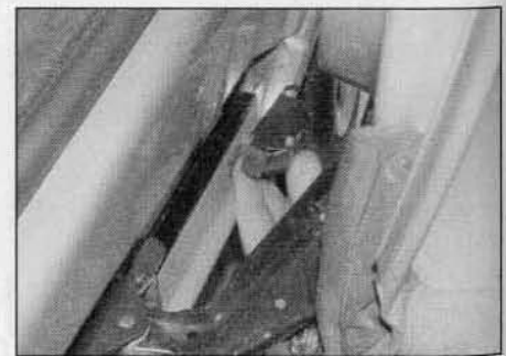
10.9b ... and remove the side door lower carriage end stop from the rear end of the lower guide rail
