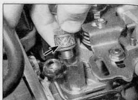
5.9b Refitting the fuel supply banjo bolt with a small section of fuel hose (arrowed) to prevent dirt entry – Bosch pump
