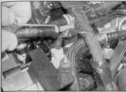
6.28 Disconnect the fuel supply and return hose quick-release fittings – 2.0 litre engines
