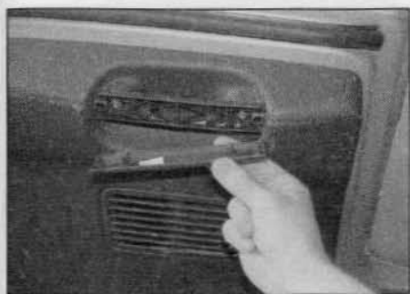
28.36 Carefully prise the cover(s) off the tailgate grab handle(s)
