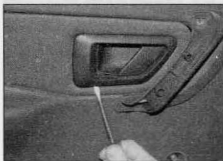
11.4a Carefully prise up the interior door handle surround ...
