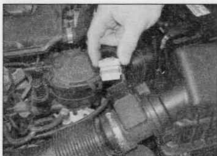
20.13 Disconnect the wiring connector from the airflow meter – later DW series engines
