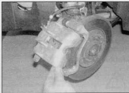
4.5 Slacken the upper guide pin bolt, and pivot the caliper upwards off the brake pads
