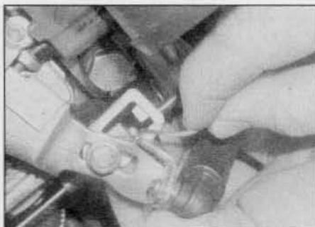
4.1a Free the accelerator inner cable from the lever . . .
