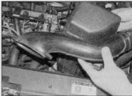
3.35b . . . then remove the air cleaner housing and intake duct as an assembly – later 2.0 litre models
