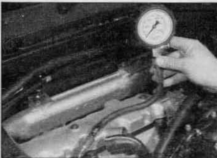
2.2 Performing a compression test
