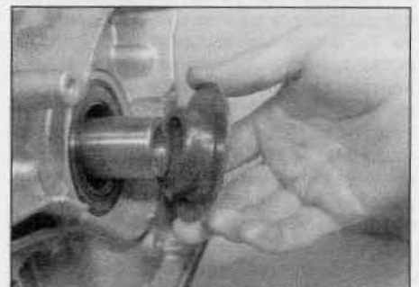
7.13 Remove the Woodruff key and flanged spacer (where fitted) from the crankshaft
