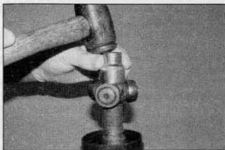
4.22b Mount the driveshaft in a vice, engage the tripod over the splines and tap it fully into position
