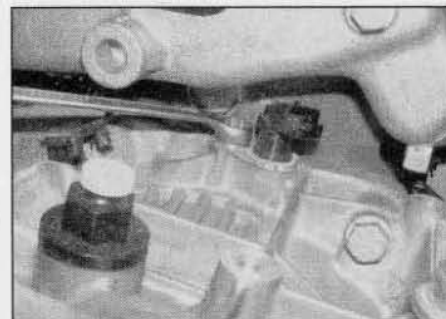
12.31a Slacken the mounting bolt ...
