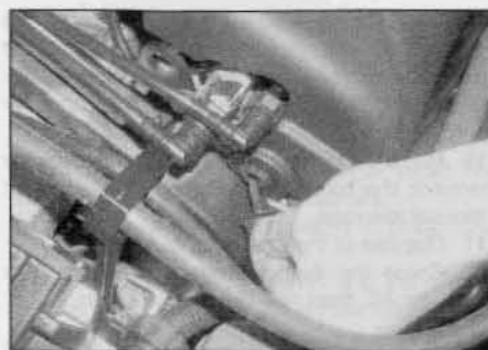
4.6a On 1.9 litre DW series engines, remove the fasteners from the right-hand side ...
