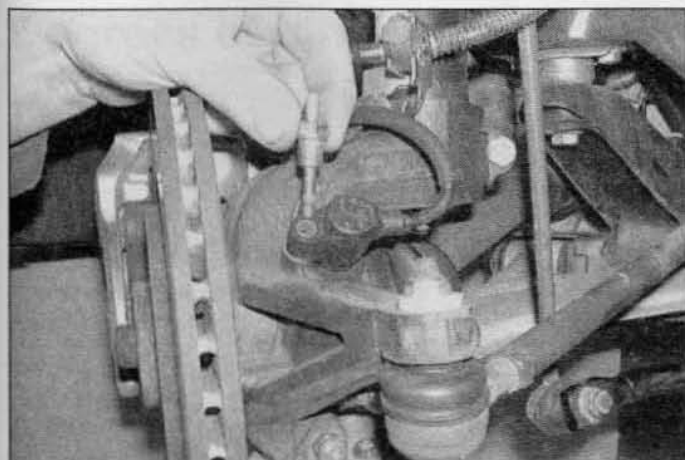
20.18a Unscrew the securing stud . . .
