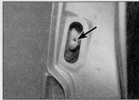
12.10a The lock cylinder retaining clip has a hole (arrowed) in its side to allow a threaded removal tool to be screwed into it
