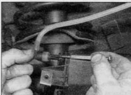
2.5 To release the quick-release hose connectors, depress their centre collars with a small flat-bladed screwdriver
