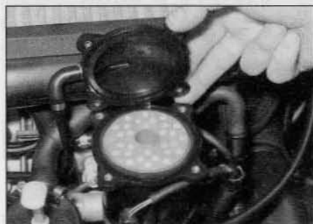
19.4 Lift off the fuel filter cover . . .
