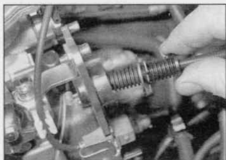
11.2 Pulling the accelerator outer cable from the bracket
