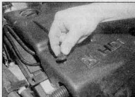
8.3d On 2.0 litre diesel engines, rotate each fastener through 90° to release it ...
