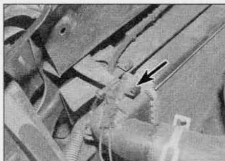
3.6 Lift the ends of the radiator retaining clips (arrowed) and move the top of the radiator toward the engine
