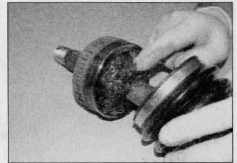
4.12j ... working it well into the ball tracks while twisting the joint
