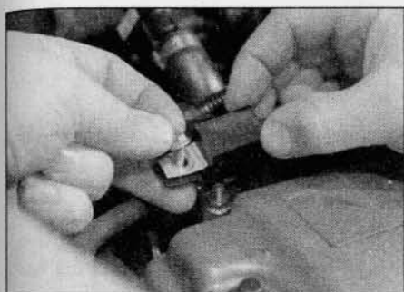
3.8a Remove radio suppresser from the right-hand end of the coil unit . . .
