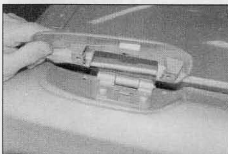
16.7 Undo the two screws and remove the hinge cover plates from the tailgate
