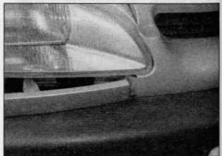
25.4 Pull the trim outwards to release the lug under the headlight, then slide the trim away from the centre of the car to remove – early models
