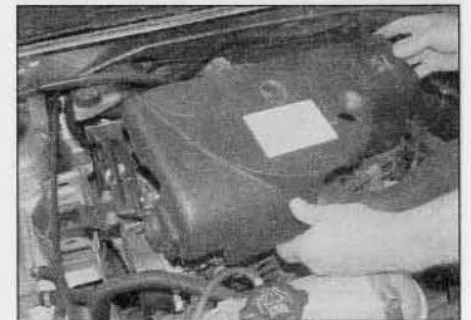
3.1c ... then remove the cover from the engine – 1.9 litre models
