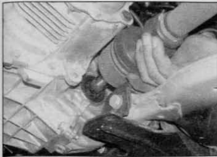
2.12 Support the driveshaft, then withdraw the inner constant velocity joint from the transmission
