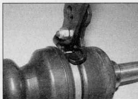
4.22j Position the outer retaining clip over the gaiter and compress the raised portion using pincers or side-cutters
