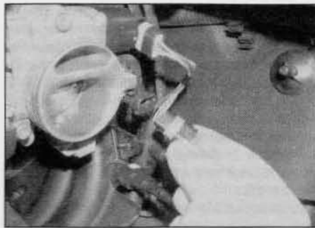
12.3 Disconnect the wiring connectors from all the throttle housing components – 1.4 litre model shown
