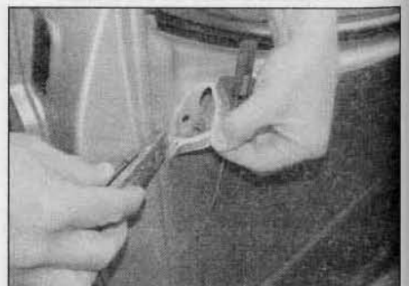
12.7 Using a sharp knife, carefully release the plastic sealing sheet from the adhesive bead
