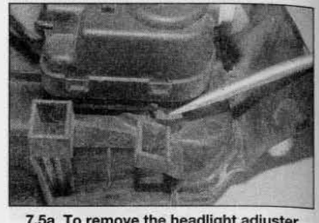
7.5a To remove the headlight adjuster motor, lift the tag and turn the motor through 90° ...
