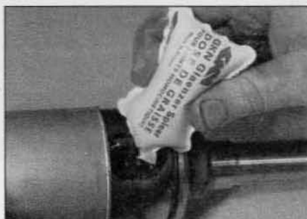
3.26b ... then apply the remainder of the grease ...
