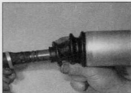
3.21b ... and the gaiter/cover assembly
