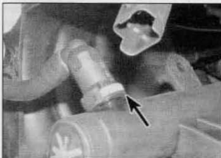
13.7 Depress the retaining clip (arrowed) and disconnect the fuel hose from the fuel rail – 1.4 litre models
