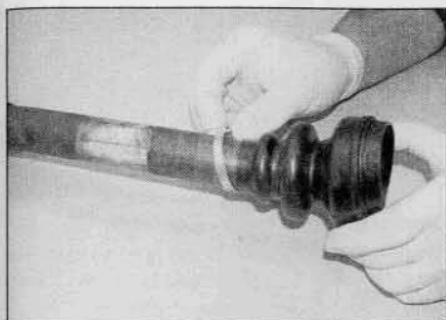
4.22a Slide the new inner retaining clip and the gaiter onto the driveshaft
