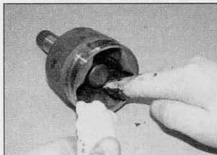
4.22g . . . then pack the outer member with the remaining grease
