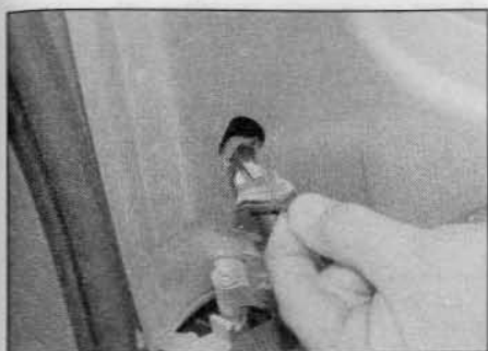
10.20 Release the tailgate wiring harness grommet, then withdraw the harness from the door
