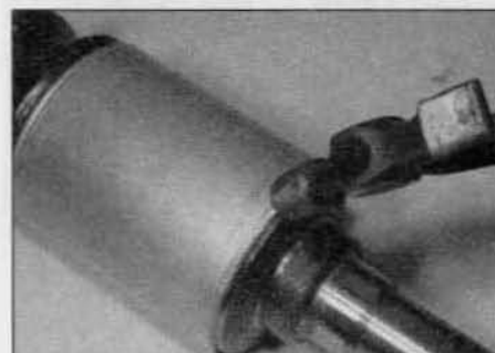
3.26c ... and peen over the end of the cover
