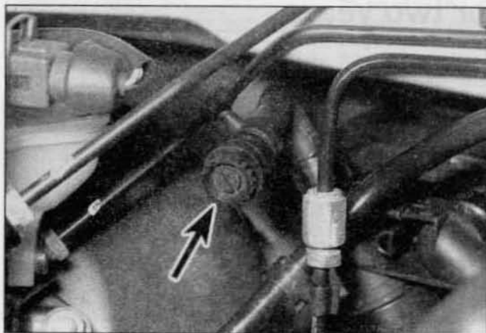
25.4a Heater hose bleed screw (arrowed)
