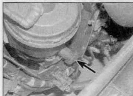
4.13 Fuel filter drain plug location – 2.0 litre engines
