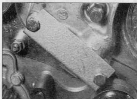
9.15b Tool in place to hold tensioner plunger in engine mounting bracket – timing belt removed for clarity
