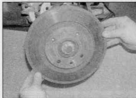
6.8b . . . and remove the front brake disc
