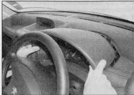
9.10a Pull the instrument panel upper trim upwards and towards the steering wheel to release the retaining clips – later models
