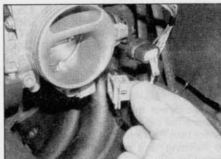
13.47 Disconnect the wiring connector . . .
