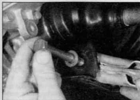
6.3 Remove the lower arm front pivot bolt ...
