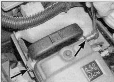
5.1a Unscrew the retaining bolts (arrowed) ...
