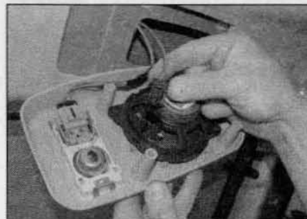
18.4a Disconnect the speaker wiring . . .
