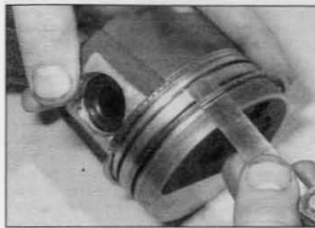
13.2 Removing a piston ring with the aid of a feeler blade
