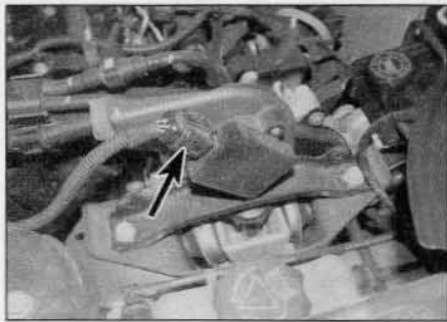
12.97 Disconnect the wiring connector (arrowed) from the accelerator pedal position sensor – later 2.0 litre models
