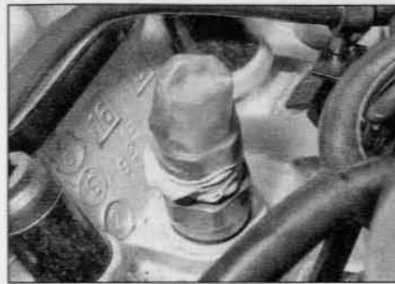
5.12b Cover the open end of the injector to prevent dirt entry
