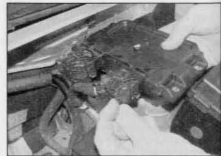
12.15 Lift the ECU off the mounting bracket, then disconnect the wiring connectors – later 1.9 litre models
