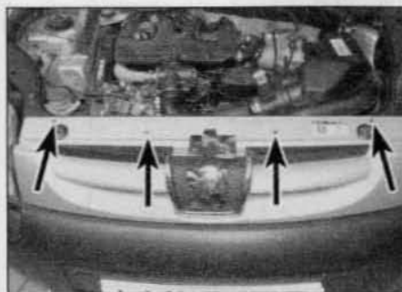
25.7 Undo the four screws (arrowed) along the top edge of the grille
