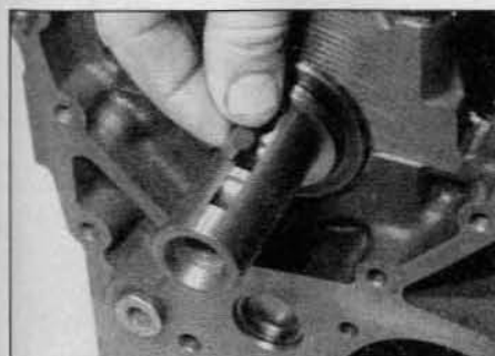
11.5c ... and remove the Woodruff key from the crankshaft
