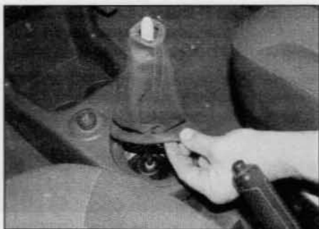
29.6 Unclip the gear lever gaiter from the front console and slide it up and off the gear lever
