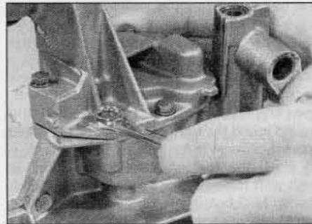
15.5a Remove the oil pump cover retaining bolts ...
