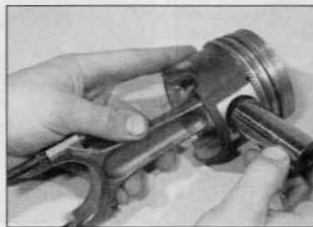
13.13b ... withdraw the gudgeon pin ...
