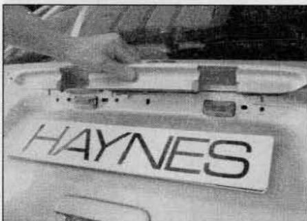
5.51 Remove the exterior moulding above the number plate lights - models with a tailgate
