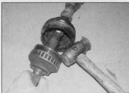
4.5 Sharply strike the edge of the outer joint to drive it off the end of the shaft
