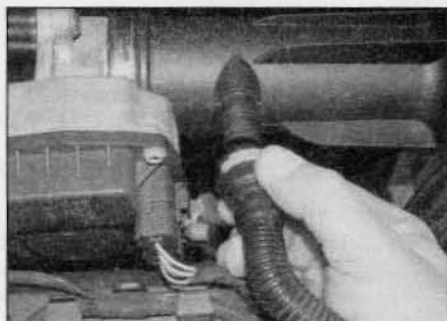
2.7 Depress the quick-release fitting and detach the breather hose from the air cleaner lid
