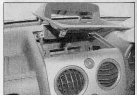
10.1 Carefully prise the multi-function display surround from the fascia
