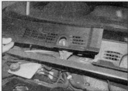
24.10 Release the fasteners on the right-hand side scuttle grille panel, then lift off the right-hand panel
