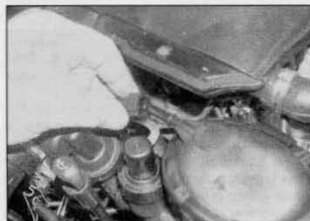
19.11 Release the retaining clip and detach the fuel outlet pipe from the filter housing cover – 1.9 litre DW series engines
