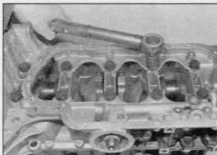
17.10 Tighten the ten main bearing bolts to the specified torque – 1.4 litre engines
