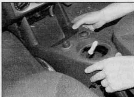
29.9 Disengage the centre console front section from the fascia, and lift it up at the rear to clear the gear lever
