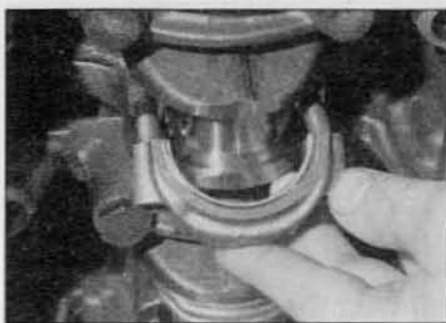
9.5 Remove the big-end bearing shell and cap
