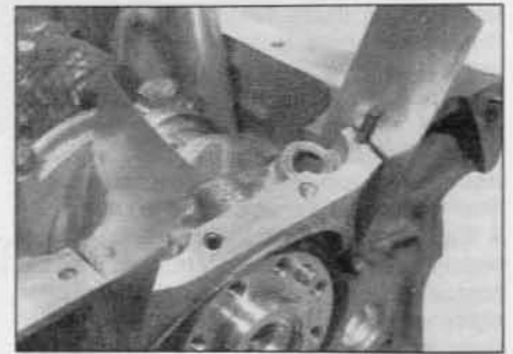
18.10a Fitting No 1 main bearing cap, using metal strips to retain the side seals
