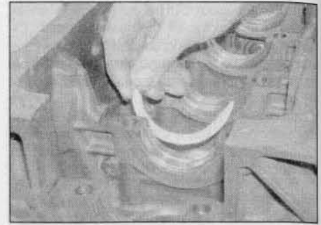
18.3 Fit the upper thrustwashers to the No 2 main bearing location with the oilway grooves facing outwards
