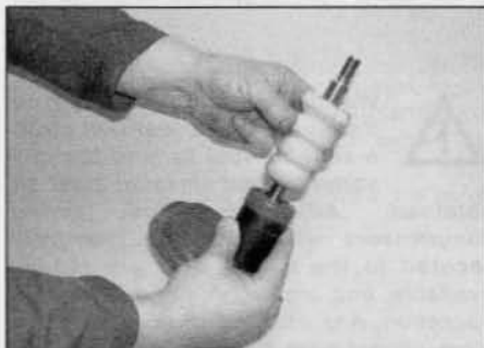
5.8a Pull the piston rod out as far as it will go and fit the damper stop
