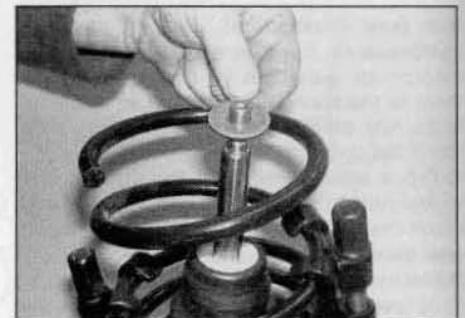
5.8e Place the flat washer in position . . .
