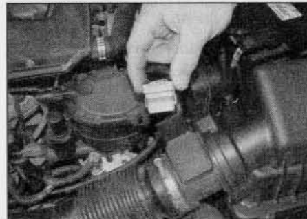
12.25 Disconnect the airflow meter wiring connector – later 1.9 litre models
