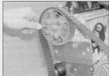
8.16c ... camshaft sprocket ...
