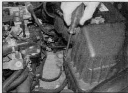
12.45a Undo the air cleaner lid retaining screws ...
