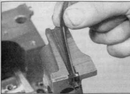
18.9a Fitting a sealing strip to No 1 main bearing cap
