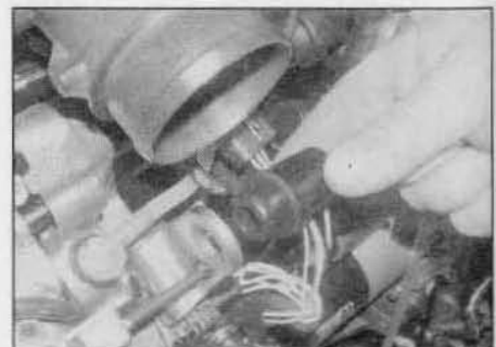
4.1c Remove the cable locating collar from the pump whilst the cable is removed – 1.9 litre models
