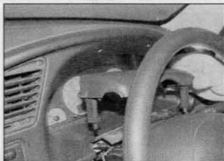
30.2 Remove the lower shroud, then lift up and remove the upper shroud from its location
