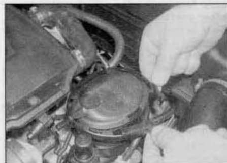
19.12 Release the clip and lift off the filter housing cover – 1.9 litre DW series engines
