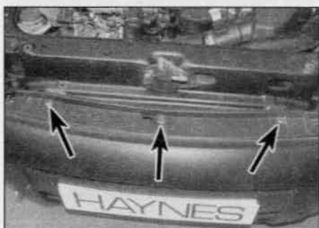
6.11 Undo the bolts (arrowed) securing the upper front edge of the bumper to the bumper bracket – later models
