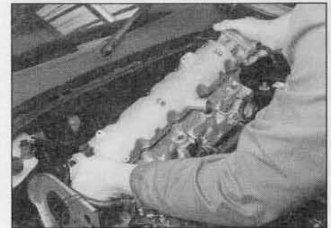
13.22 Removing the cylinder head
