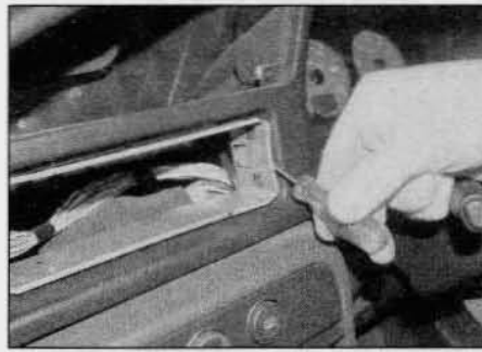
17.5 On early models, use a small screwdriver to release the mounting frame lugs . . .
