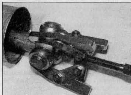
3.17a Using a three-legged puller to remove the inner tripod joint
