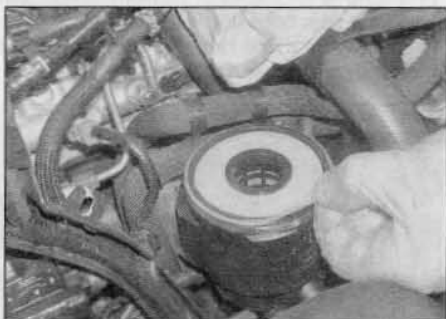
19.26c . . . and the O-ring seal . . .
