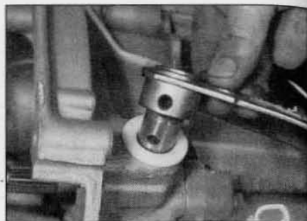
5.4b ... and remove the release lever from the top of the release fork shaft – MA5 and BE3/5 transmissions
