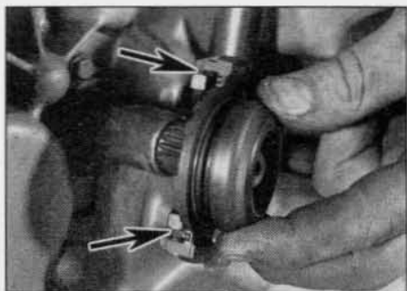
5.3 Unhook the release bearing from the fork, and slide it off the input shaft – MA5 and BE3/5 transmissions
