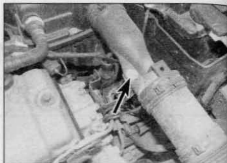
2.3 Undo the bolt (arrowed) securing the air intake duct to the support bracket – early 1.4 litre models
