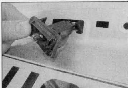
7.27 Depress the tabs and push out the number plate light unit – models with a tailgate
