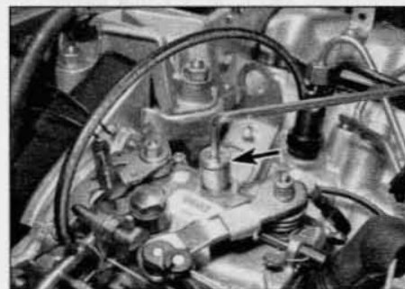
7.3 Removing the injection pump timing inspection plug – Lucas pump
