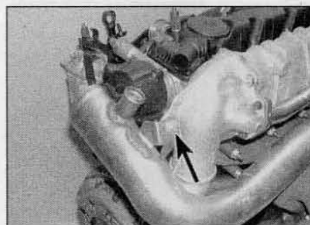
3.27 Undo the upper mounting bolt (arrowed) securing the rigid inlet duct to the inlet manifold – early 2.0 litre models
