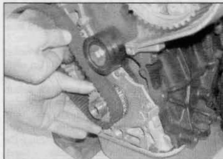
8.16a Retain the timing belt on the crankshaft sprocket and feed it around the idler pulley ...
