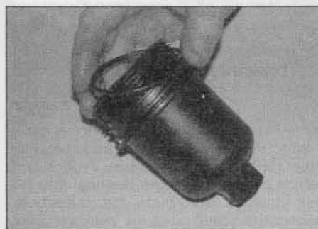
3.11b ... and recover the O-ring seal
