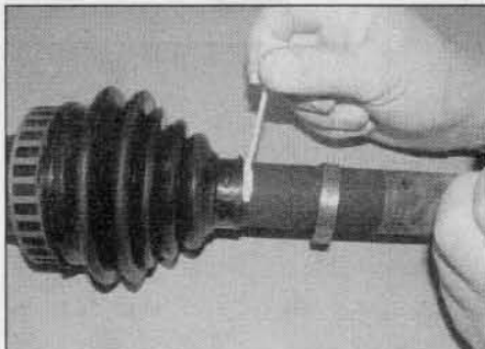
4.3b . . . then mark the position of the end of the gaiter on the driveshaft
