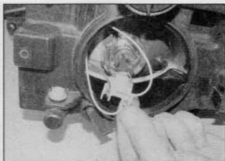
5.8 Disconnect the wiring connector from the headlight bulb – later models
