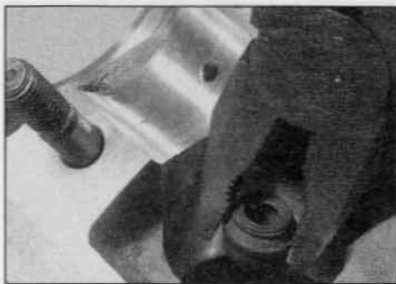
7.5e Remove the valve stem oil seal using a pair of pliers ...
