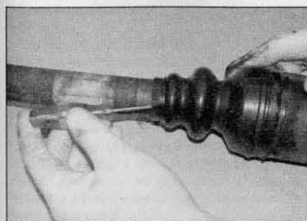
4.22i Push the outer member fully into position over the tripod, while lifting the gaiter inner end to expel trapped air
