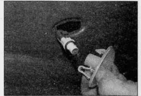
5.28a Rotate the bulbholder anti-clockwise to release it . . .
