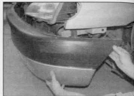
6.6 Carefully pull the bumper forward and off the car – early models
