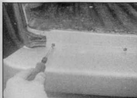
7.7 Undo the screws securing the upper edge of the bumper to the bumper bracket
