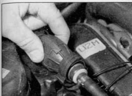
2.2 Hand-operated fuel system priming pump
