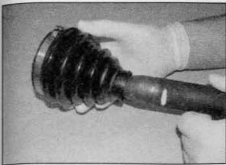
4.12b ... followed by the new gaiter with the outer retaining clip in place
