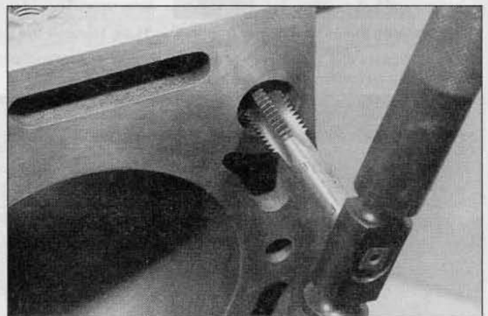
12.9 Cleaning a cylinder block threaded hole using a suitable tap
