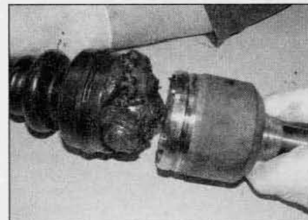
4.22h Locate the outer member over the tripod and engage the gaiter with the outer member groove
