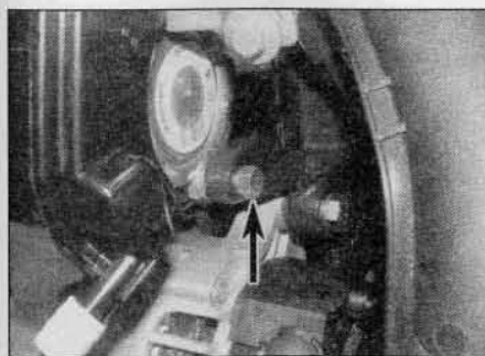
22.10a Power steering pump rear mounting bolt (arrowed) ...
