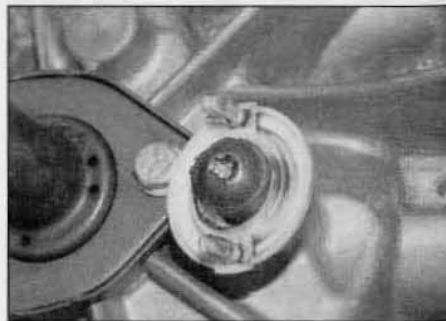
5.6c ... then unscrew the pivot ball-stud – BE4/5 transmissions
