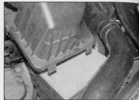
12.45b ... disengage the two retaining lugs and lift the lid from the air cleaner housing – 2.0 litre models
