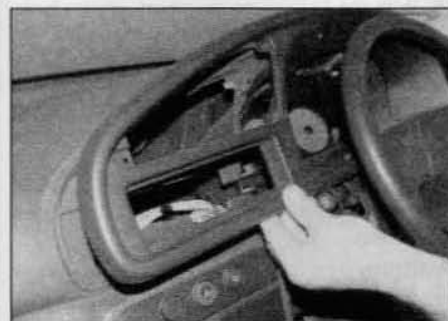
30.9 Pull the upper panel from its location to release the retaining clips
