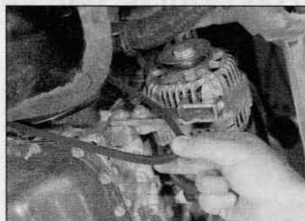
10.9b . . . then slip the drivebelt from the pulleys - models with a manual adjuster on the alternator lower mounting
