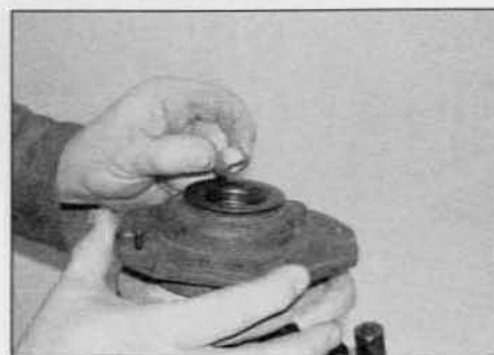
5.8k ... then fit and tighten the piston rod nut
