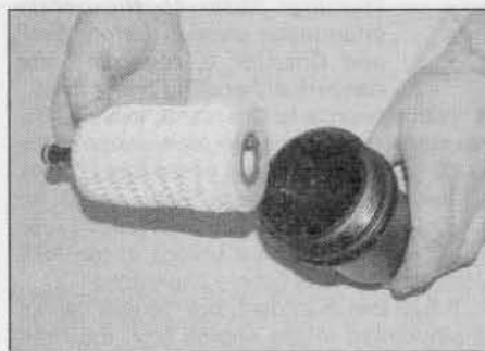
3.14a Fit the new element into the cover ...
