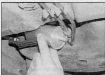
20.4 Release the tab of the retaining strap and slide the fuel filter out of its holder
