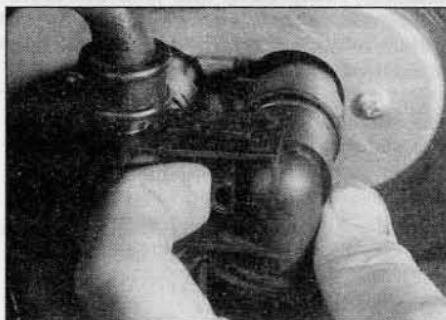
10.13c . . . then release the plastic retaining clip . . .
