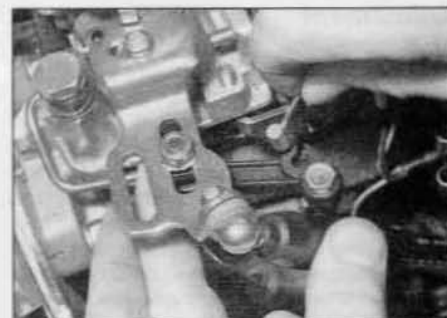
11.1 Releasing the accelerator inner cable from the lever on the injection pump
