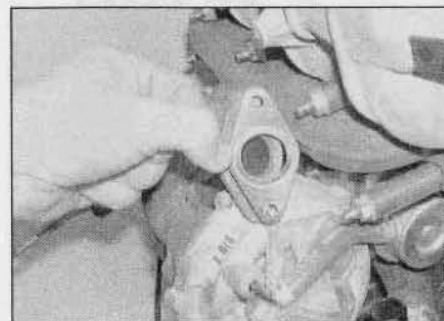
3.29b . . . then withdraw the valve and pipe assembly and recover the gasket at the EGR pipe flange – 2.0 litre models
