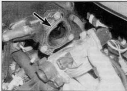
12.4b ... then remove the throttle housing from the manifold and recover the sealing ring – 1.4 litre model shown
