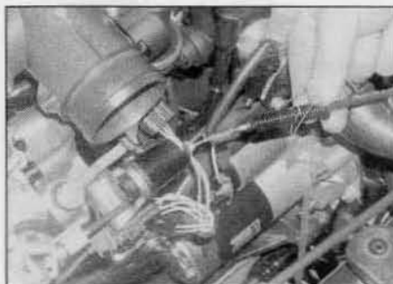
4.1b . . . then withdraw the outer cable from the pump bracket, complete with spring clip – 1.9 litre models
