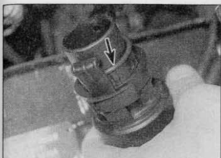
2.17 On refitting, fit a new O-ring (arrowed) to the hose union
