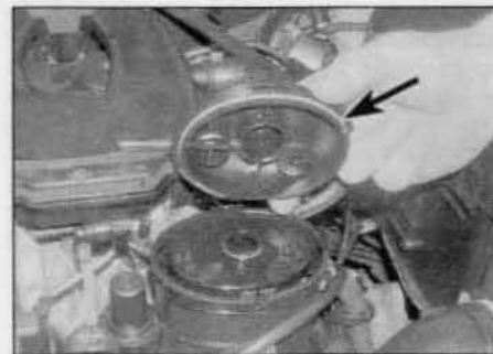
19.16b . . . and the new large sealing ring (arrowed) is correctly fitted to the housing cover – 1.9 litre DW series engines
