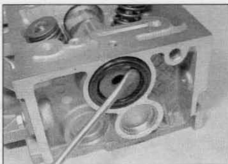
10.10a Prise out the oil seal . . .
