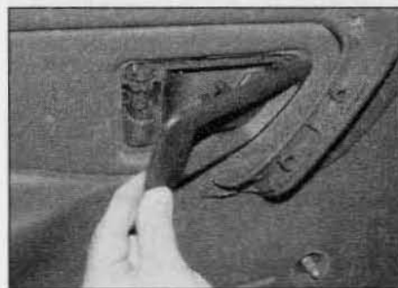
11.4b ... and disengage it from the handle
