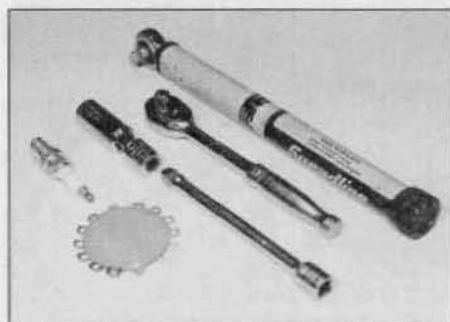
18.5 Tools required for spark plug removal, gap adjustment and refitting
