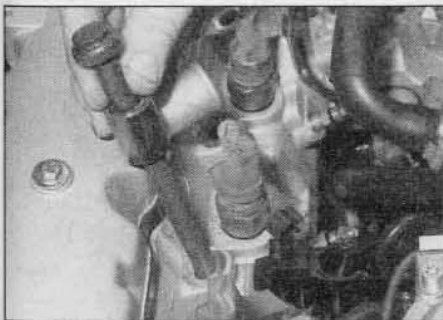
13.20 Removing a cylinder head bolt and spacer
