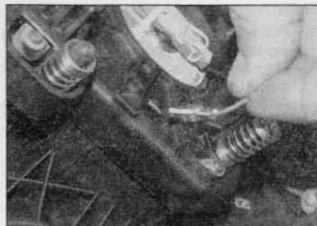
21.9a Disconnect the horn push earth connector . . .
