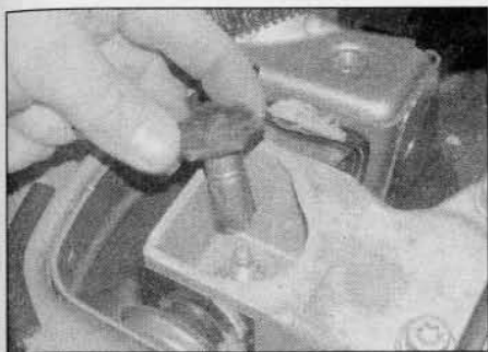
20.21 Unscrew the domed buffer nut from the top of the mounting to gain access to the mounting nut – 2.0 litre engines
