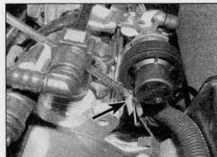
10.4 Slacken the retaining screw (arrowed) then slide the end fitting off the fast idle cable – 1.9 litre models
