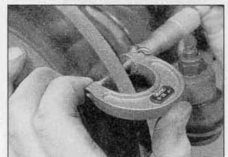
6.3 Using a micrometer to measure disc thickness
