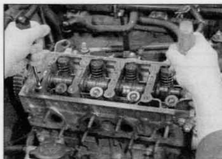
11.16 Use two stout screwdrivers to rock the cylinder head free from the block – 1.4 litre engines
