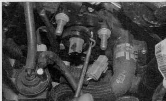
6.15 On later models, prise out the sensor retaining circlip then remove the sensor and sealing ring from the housing
