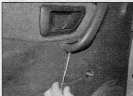
11.2a Carefully prise off the base of the door pull handle trim ...
