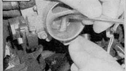
The inlet air temperature sensor clips can be released by passing a close-fitting ring spanner over the end of the sensor.
