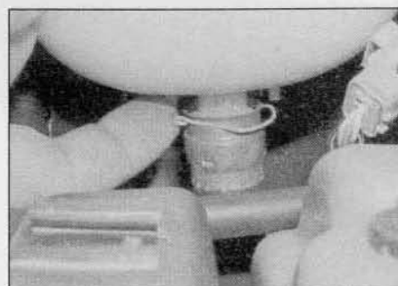
2.25 Where spring clip hose connections are used, remove the spring clip then disconnect the hose
