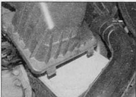
20.21b . . . lift up the lid and disengage the two retaining lugs from the air cleaner housing – 2.0 litre engines
