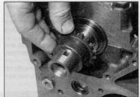
11.5b ... then slide off the drive sprocket ...
