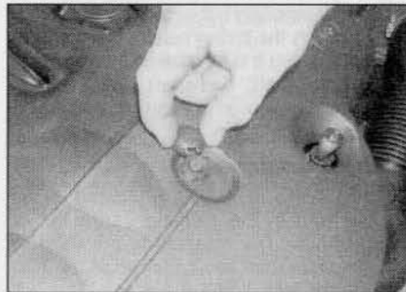
4.1b ... and top of the engine cover ...
