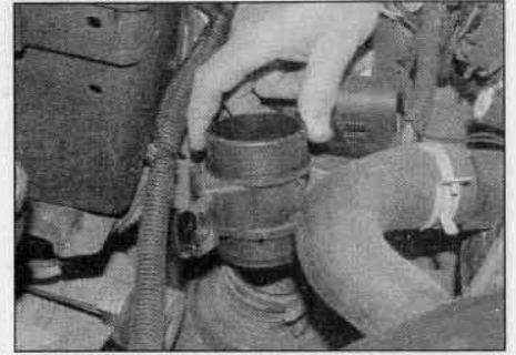
12.21 Slacken the retaining clip and lift off the airflow meter – early 1.9 litre models
