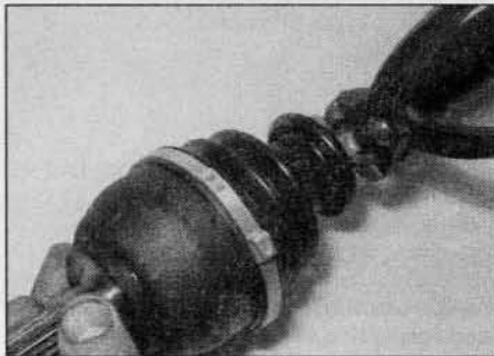
3.10 Securing a gaiter securing clip using side-cutters
