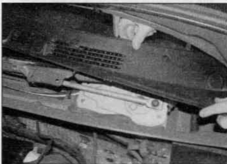
24.11 Remove the left-hand scuttle grille panel in a similar fashion
