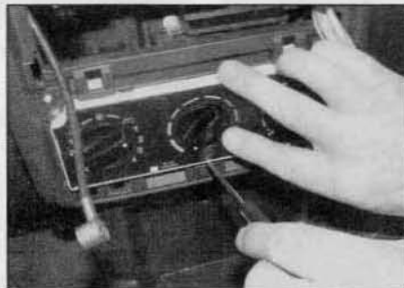
10.4 Release the lug at the lower centre of the heater/ventilation control unit and withdraw the unit from the facia
