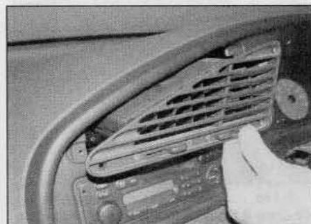
9.3b . . . and remove the centre vent unit from the facia – early models
