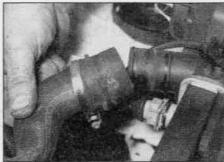
2.5 Disconnecting the radiator top hose
