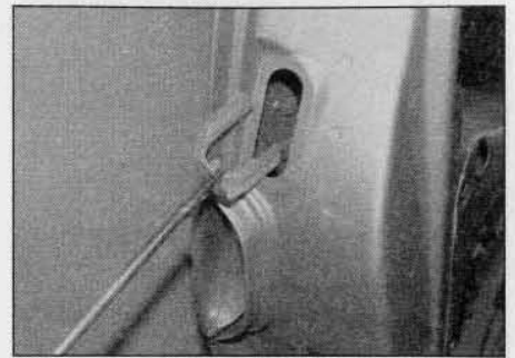
12.10b Using a suitable removable tool, extract the retaining clip from the lock cylinder
