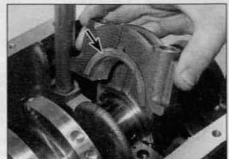
11.7 Removing No 2 main bearing cap. Note the thrustwasher (arrowed)
