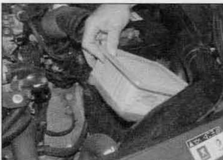
20.22 Withdraw the filter element from the housing – 2.0 litre engines
