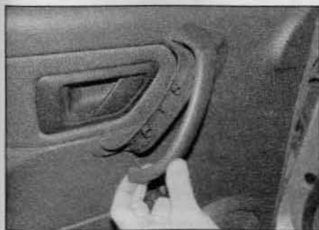
11.2b ... lift the handle trim off the upper locating lug and remove it from the handle
