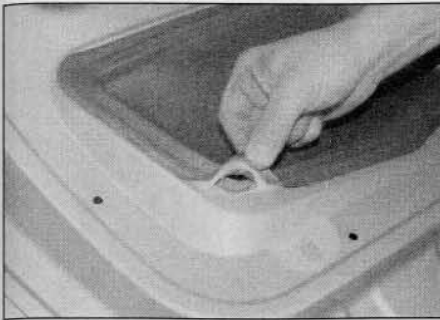
13.20 Release the plastic sealing sheet from the adhesive bead and remove the sheet from the door
