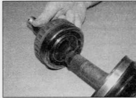
4.12f Slide the CV joint onto the splines, and position the inner member up against the cable tie
