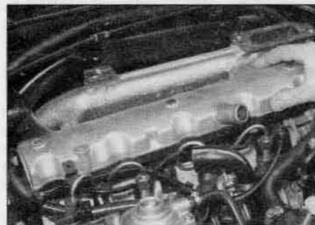
4.6 ... and lift off the cylinder head cover
