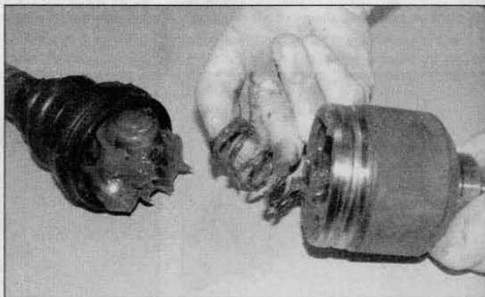
4.17b . . . and recover the spring and thrust cap from inside the outer member
