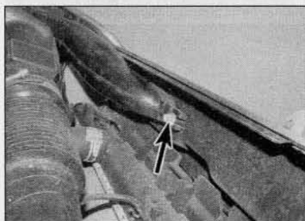
3.15 Undo the nut (arrowed) securing the air intake duct to the front body panel – later 1.9 litre models
