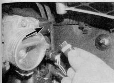
13.38 Disconnect the wiring connector from the idle speed stepper motor (arrowed) . . .
