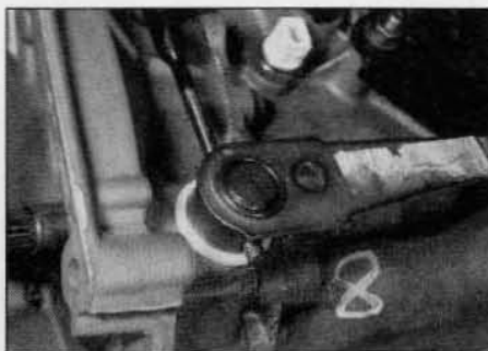
5.4a Drive out the roll-pin using a suitable punch ...
