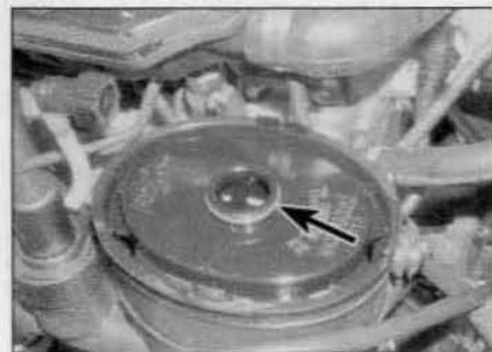
19.16a Ensure that the new small sealing ring (arrowed) is correctly fitted to the fuel filter . . .
