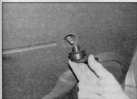
11.1 On models with manual windows, pull the winder handle off the spindle
