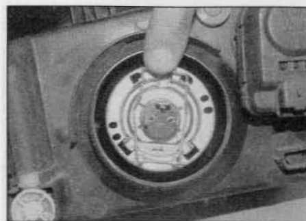
5.3a Release the spring clip ...
