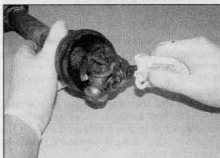
4.22d Pack the tripod and the gaiter with half the recommended quantity of the grease . . .
