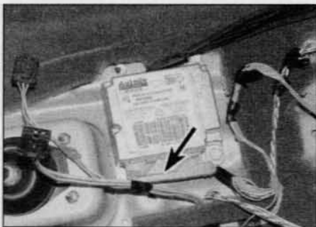
21.34 Release the retaining clip and disconnect the wiring connector (arrowed) from the airbag control unit
