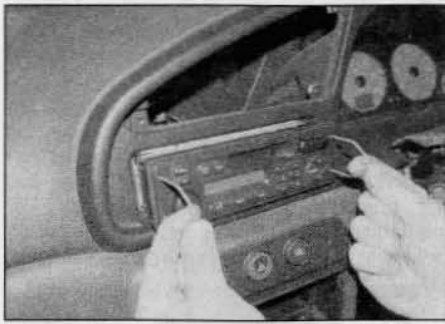
17.3 Insert the removal tools into the holes on the audio unit and withdraw the unit from the fascia
