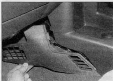
29.8 Detach the side ventilation panel, on each side, from the centre console and fascia
