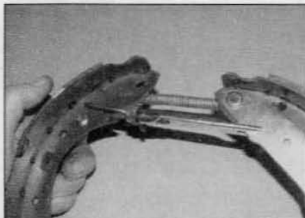
5.18 Engage the adjuster strut with the leading shoe and handbrake lever
