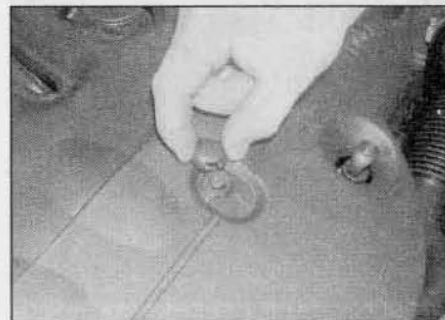
3.1b ... and top of the engine cover ...
