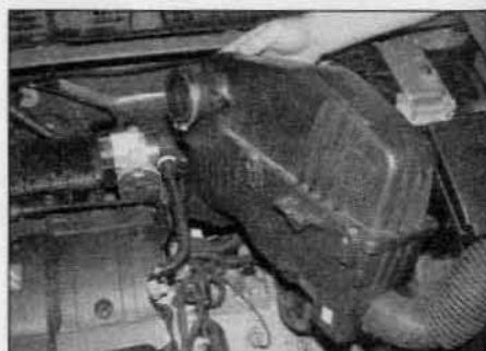
2.10b . . . then lift the air cleaner assembly upwards to release the lower mounting – later models
