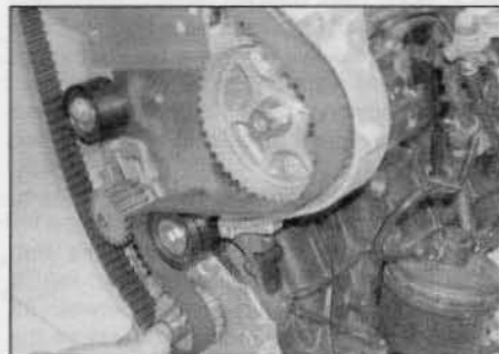
8.16b ... high pressure fuel pump sprocket ...
