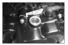
**Note**: Always ensure that the piston is at the end of compression stroke and 'T' is seen from 'Timing Inspection Window' at generator cover. When adjusting tappet clearance.
