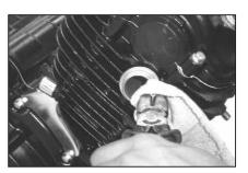
**Note:** Wrap a piece of cloth around the protruding edge of the sleeve spark plug and using a plier, pull out the sleeve.
