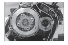
Using Special Tool: Special Nut Puller 37 10DJ43 Primary Gear Holder 3710 DJ28 Remove:
