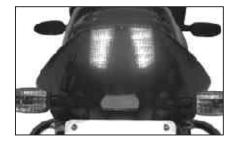
**Tail Lamp:** The illumination for Tail lamp and Brake lamp are done through 2 rows of LED's each. These are high intensity LED's the main advantage of these LED's is they consume very less power. i.e LED consumes 3W power against 21 W power of a conventional brake lamp. When you operate light control switch to glow but intensity will be very low. As soon as you operate brake switch the brightness of LED increases to size you bright light.
