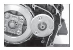
Using Special Tool: Primary Gear Holder - 37 10DJ 28 Using Sp. Tool: Centrifugal Oil Filter Nut - 37 10DJ 43
