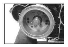
Using Special Tool: Rotor Holder H6 0721 00
