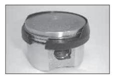
Note: Apply thin layer of oil in cylinder bore and piston assly when sliding inside for ease in fitment.
