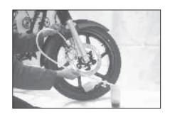
Brake fluid from the reservoir with the help of syringe/syphon pump
