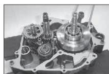
**Caution:** Use a sharp blade or knife to cut off any protruding 'Gasket'. This is very important for preventing any oil leakage from 'Crankcase' and 'Cylinder Block Joint'. Don't apply grease / any adhesive to 'Crankcase Gasket' as these 'Gasket' when comes in contact with oil expands and seals hidden cavities.
