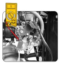
When throttle is open and Reed Switch magnet crosses to straight edge of fix bracket of Reed Switch multimeter should show discontinuity.
