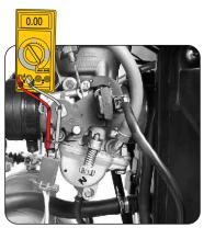
On De-acceleration, when of Reed Switch magnet re-coinsides with straight edge of fix bracket of Reed Switch Multimeter should show continuity.
