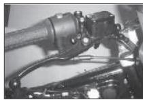
Master Cylinder & Caliper Inspect every 5000 Km for leakage.
