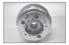
Note: Holding the gear complete starter clutch rotate the rotor and pull it out in Anticlockwise direction to prevent rollers and springs coming out. Rotor puller has left hand threads.
