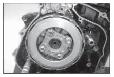
Using Special Tool - Primary gear holder 37 10DJ 28 & Special Nut 37 10DJ 43
