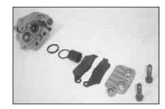
**Warning:** Do not apply high pressure compressed air, which will cause the piston to jump out of the cylinder. The piston should be taken out gradually with moderately compressed air. Care to be taken not to damage the sealing surface of the inlet port while applying air pressure.
