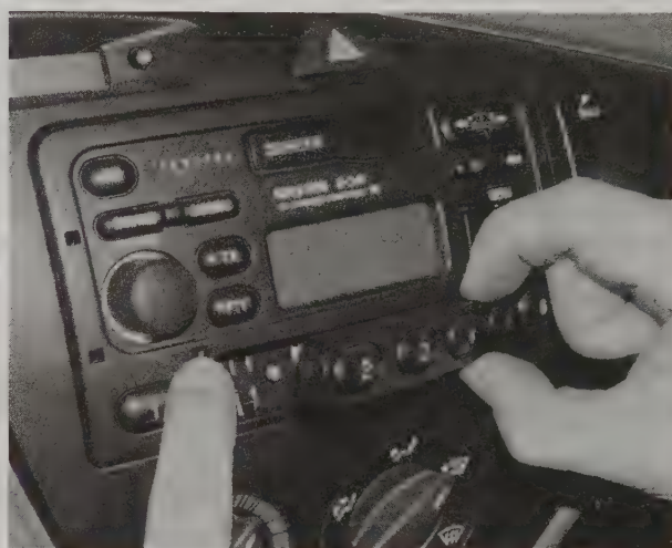
21.1 Press the securing button to release the bezel
