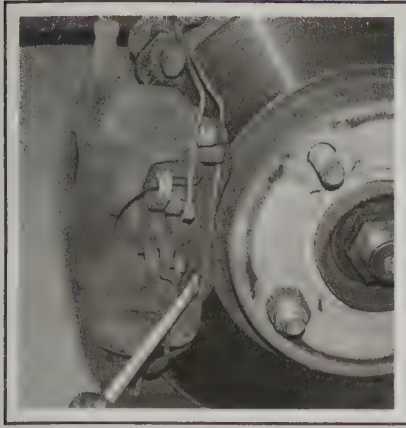
2.2 Pry the pad retaining clip from the caliper
