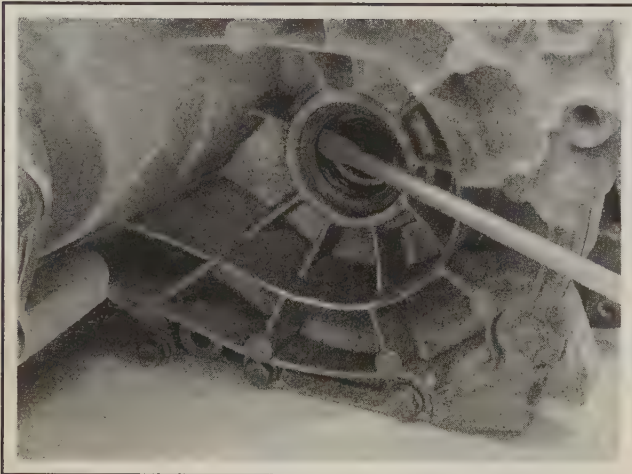
6.4 Pry out the oil seal with a suitable lever
