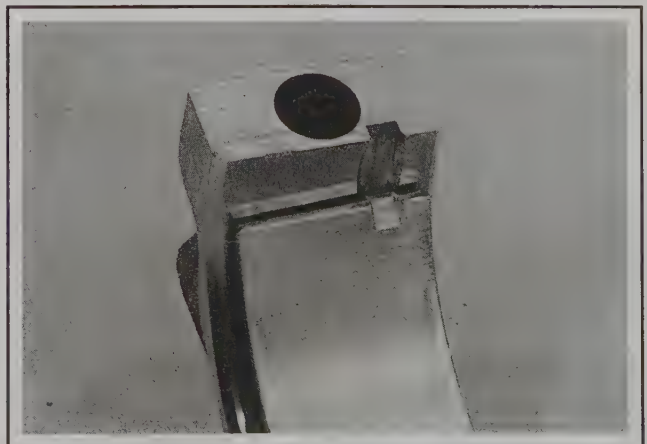
18.3 The locating tab on each connecting rod bearing must engage with the notch in the connecting rod or cap
