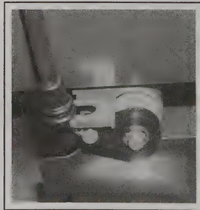
21.4 Unclip the outer cable, then release the inner cable
