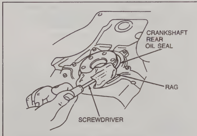
17.5 Pry the seal out with a screwdriver wrapped in a rag
