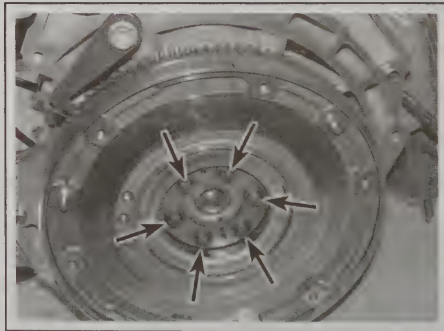
19.4 Lock the flywheel/driveplate while the flywheel mounting bolts are removed
