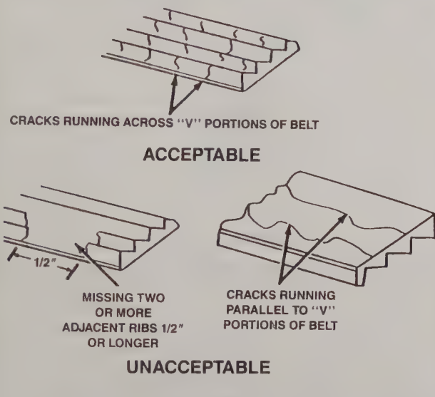
11.6 Check the drivebelt for signs of wear like these. Very small cracks across the ribs are acceptable. If the cracks are deep, or if the drivebelt looks worn or damaged in any way, replace it
