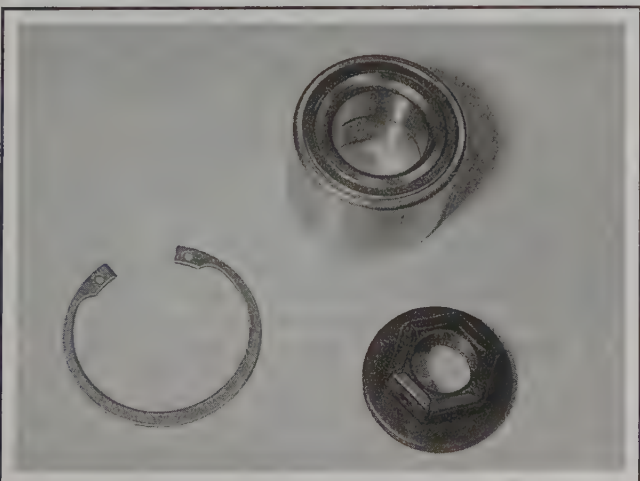
9.1 The wheel bearing is not adjustable
