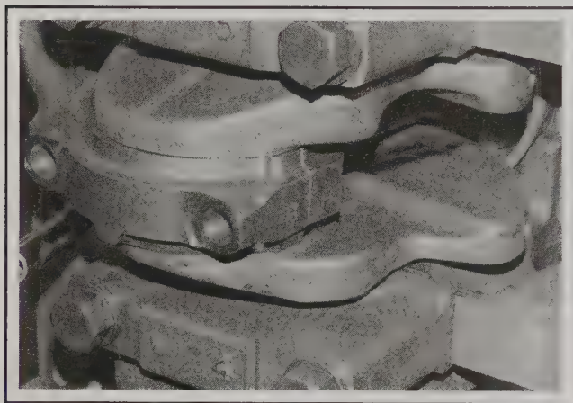
9.4 Each connecting rod and cap can be marked on the flat, machined surfaces
