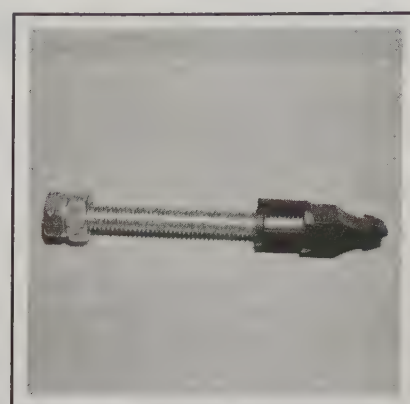
32.12c . . . then unscrew the retaining clip from the bolt for installation
