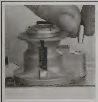
18.8b . . . install the lock cylinder, and insert the plunger . . .
