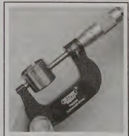
11.8 Measure the cam follower outside diameter at several points
