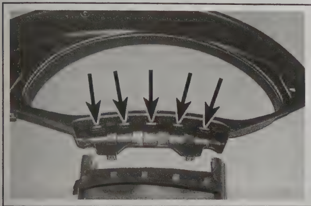
10.3a The upper steering shroud clips into the slots (arrows) in the instrument cluster bezel
