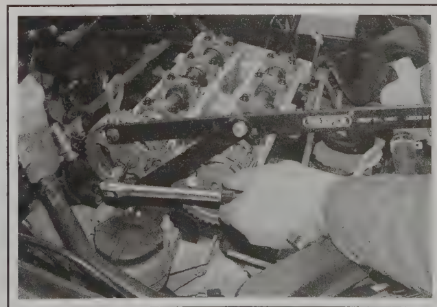
8.19 Use a sprocket holding tool while loosening the camshaft sprocket bolts
