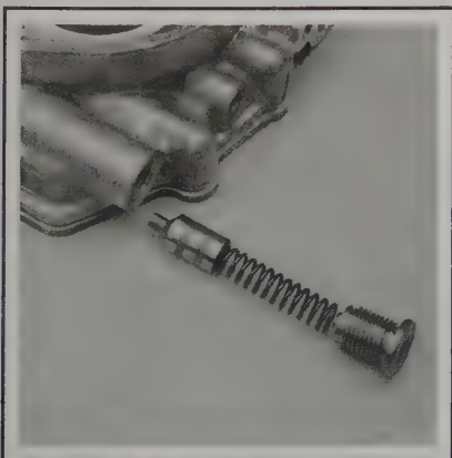
14.10 Oil pump pressure relief valve components (seen with oil pump removed)
