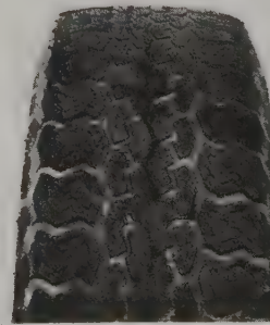
FEATHERING DUE TO MISALIGNMENT
