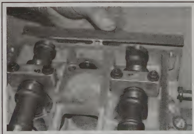
4.5 Slide the tool/metal bar into the slots in the ends of the camshafts
