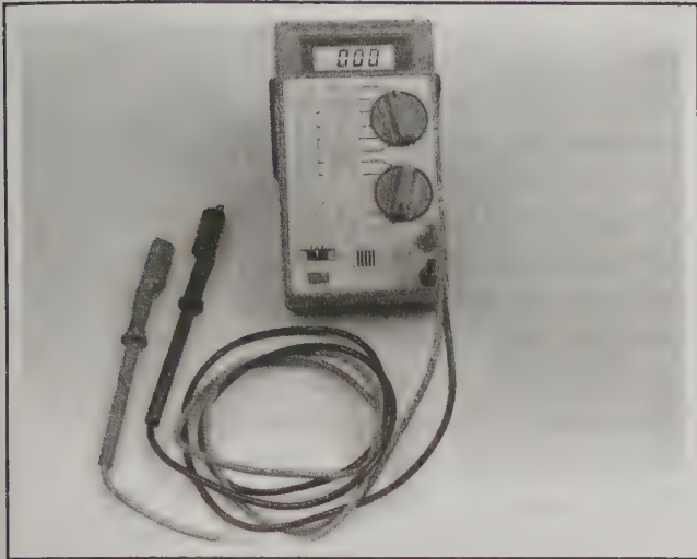
7.28 Digital multimeters can be used to test all types of circuits. Because of their high impedance, they are more accurate than analog meters for measuring voltage in low-voltage circuits
