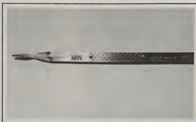
4.4 The oil level should be in the Safe range - if it's below the MIN or ADD mark, add enough oil to bring it up to or near the MAX or FULL mark
