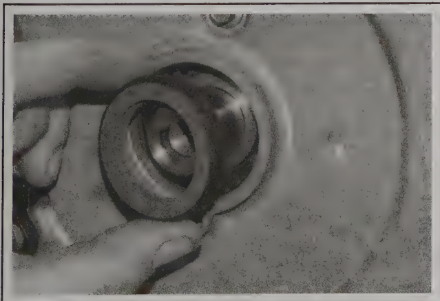
18.4a Make sure the oil seal remains square as it is being inserted into the timing cover
