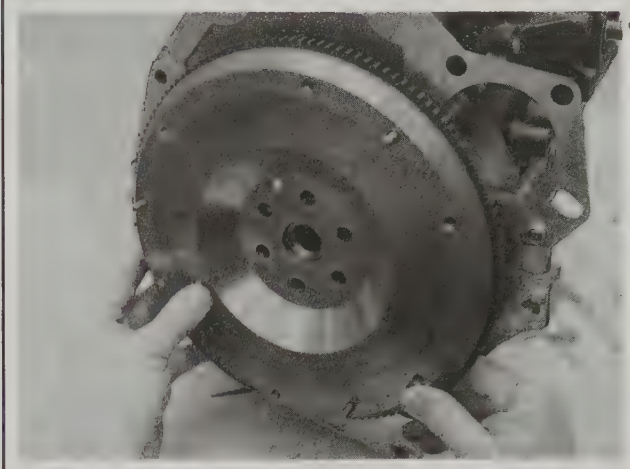
17.10a Place the flywheel into position . . .
