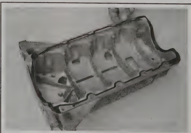
14.19a Fit the new gasket . . .
