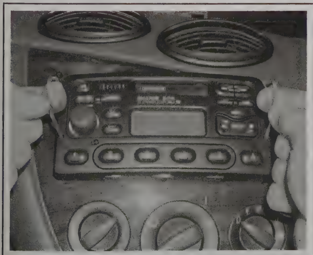
21.6 Using the U-shaped tools to remove the radio
