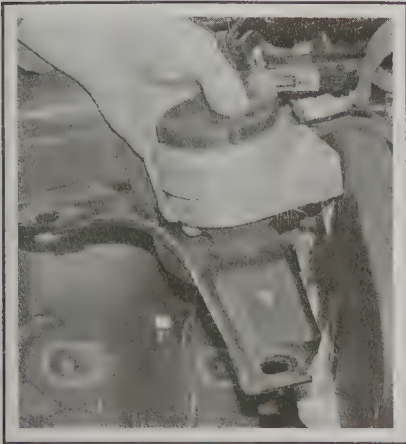
7.5c . . . and take off the engine mount
