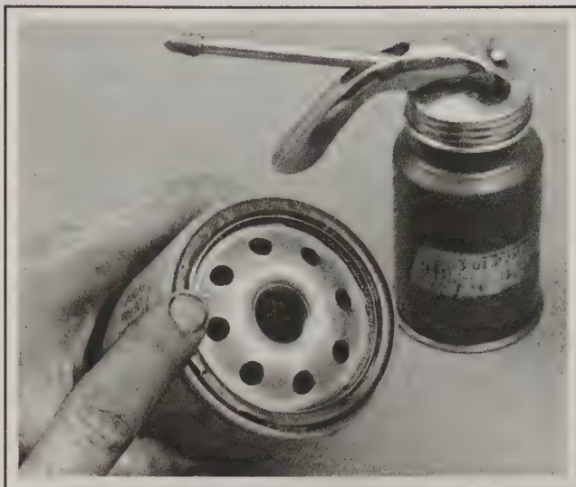
8.16 Lubricate the oil filter gasket with clean engine oil before installing the filter on the engine
