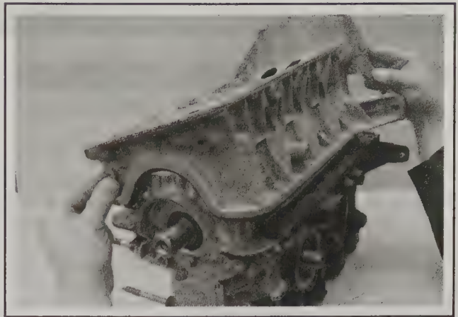
18.22b . . . then install the lower crankcase
