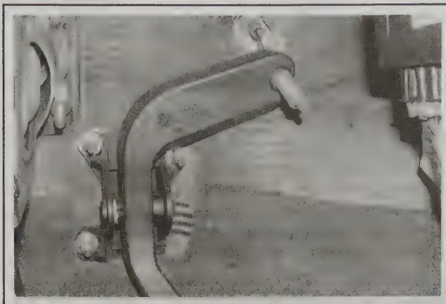
7.2 Accelerator pedal, showing cable attachment and mounting nuts
