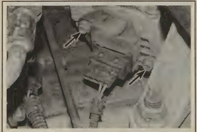
5.6 Disconnect the multi-plug, then unscrew the two retaining bolts (arrows) - MTX 75 transaxle
