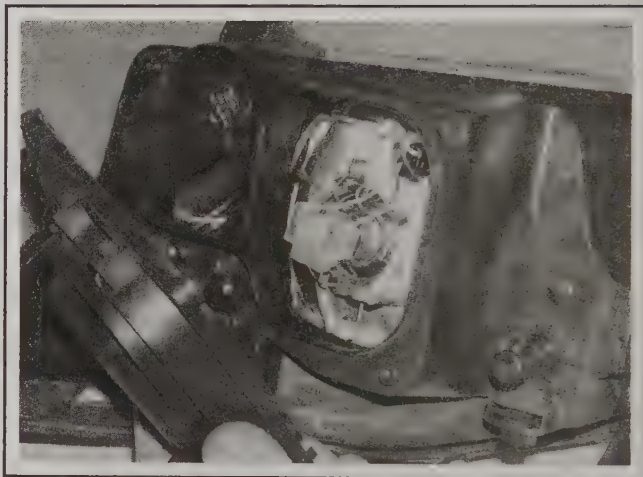
9.3 Remove the rear headlamp cover
