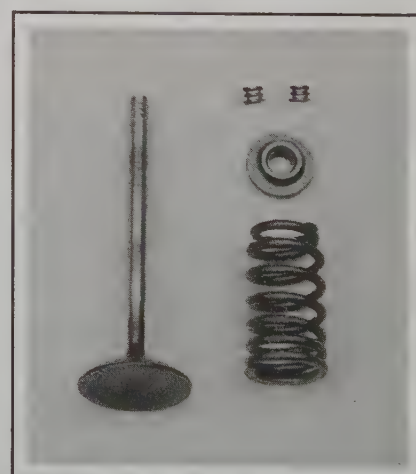
6.8a Valve, keepers, retainer and valve spring
