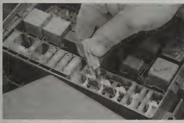
2.3 Remove fuse No. 12 to disable the fuel pump
