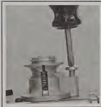
18.8c . . . then install the retaining screw, using Loctite sealer on the threads
