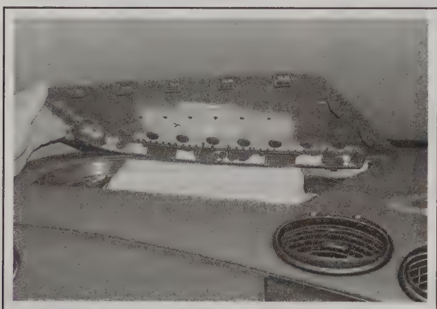
25.7b . . . then hinge the trim towards the windshield to access the airbag
