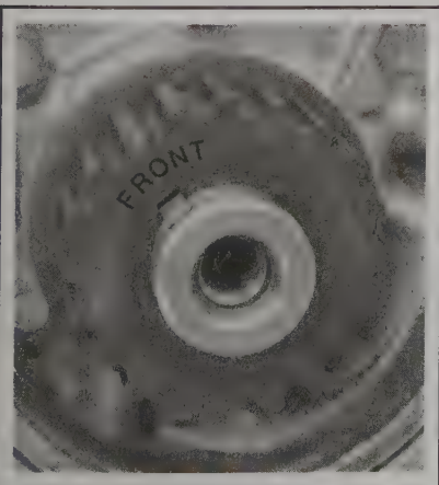
9.6a Crankshaft sprocket FRONT marking
