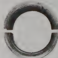
Damage from excessive thrust or insufficient axial clearance
