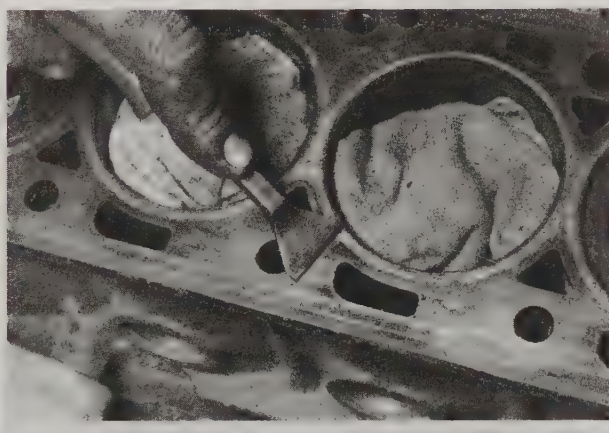
12.20 Stuff rags into the cylinder bores to keep debris from falling down where you can't retrieve it, then carefully scrape all old gasket material from the mating surface on the block (clean the cylinder head surface as well)
