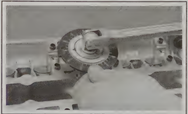
12.44 . . . then through the Stage 3 angle, here using an angle gauge
