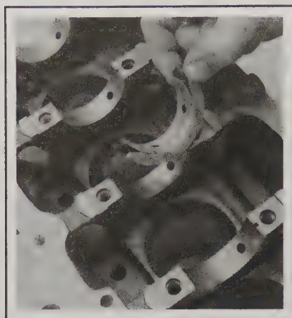
17.4b Note the thrustwashers fitted to the number 3 main bearing insert
