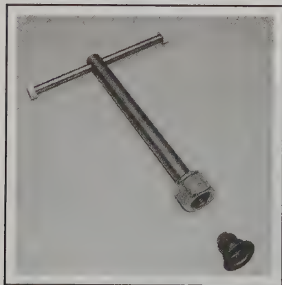
6.7a Make a seal removal tool with a bar, drill it for a cross-handle at the top, pin a large nut (whose threads just "bite" into the seal) on the bar so that the nut will turn with the bar
