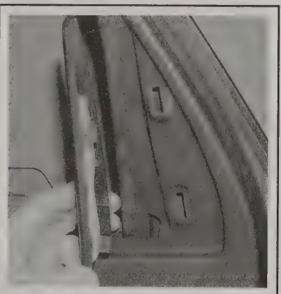
11.11 Unclip the trim from the window frame
