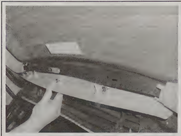
19.4b . . . then unclip the upper tailgate trim
