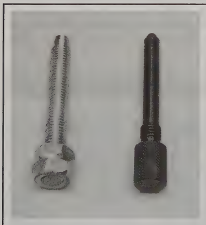
3.7a Home-made (left) and genuine (right) timing pins
