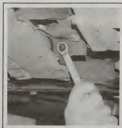
16.14a Unscrew the two nuts . . .
