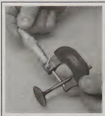
7.12 Measuring the diameter of a valve stem
