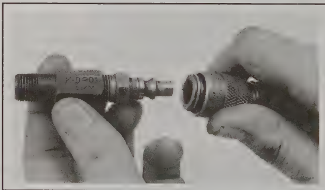
9.4 This is what the air hose adapter that threads into the spark plug hole looks like - they're commonly available from auto parts stores
