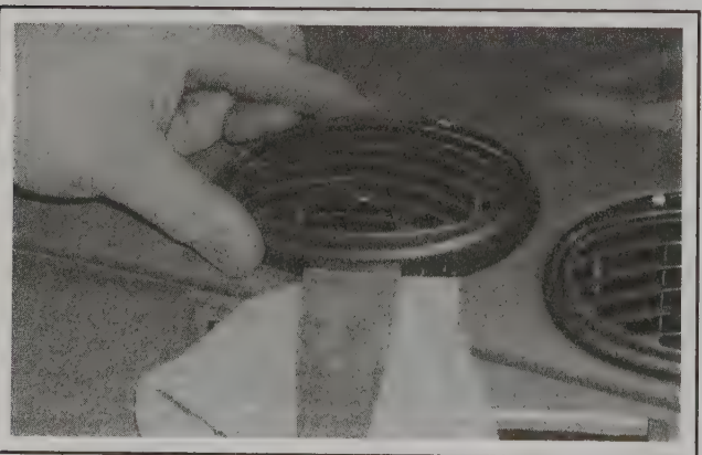
9.30 Carefully pry out the air vents
