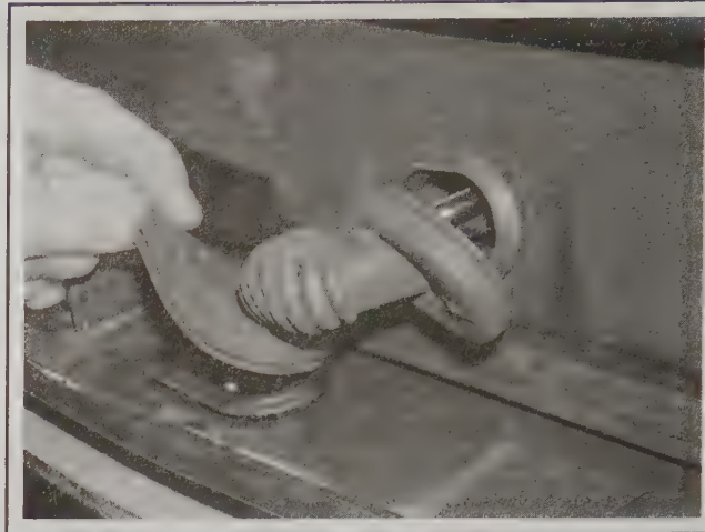
19.6 Unclip the rubber wiring grommet
