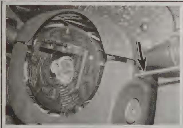
19.4a Unclip the upper shroud with a thin screwdriver (arrow) . . .
