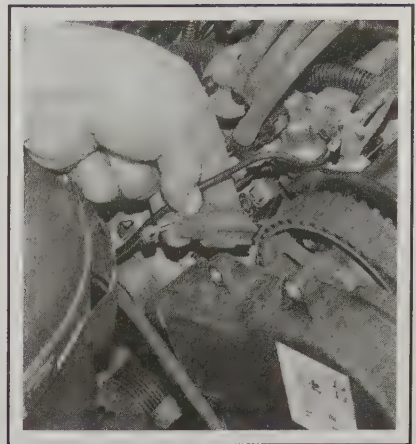
7.7a Unclip the wiring plug at the rear of the cover . . .
