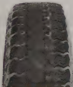
INCORRECT TOE-IN OR EXTREME CAMBER
