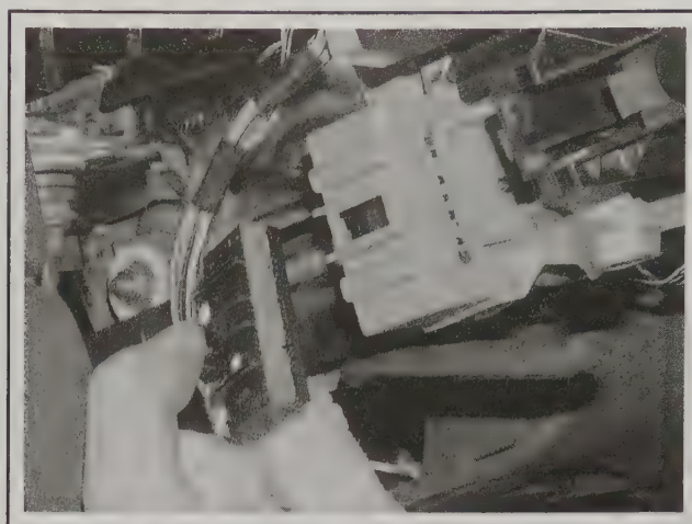
4.3a Disconnect the multi-plug . . .
