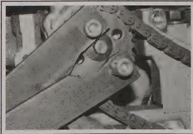
18.4b A socket of the correct size can be used to install the new seal
