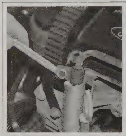
12.16 Unbolt one of the power steering fluid pipe brackets
