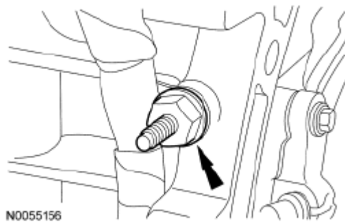
Fig. 495: Locating Wiring Harness Retainer Stud Bolt Courtesy of FORD MOTOR CO.
