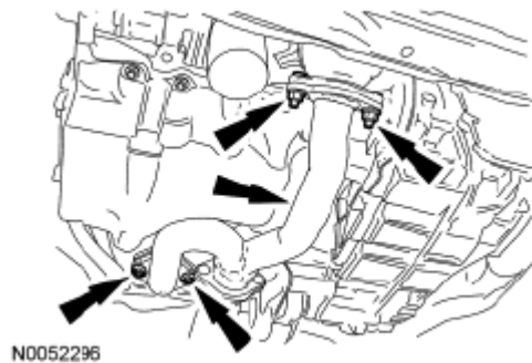
Fig. 173: Locating Exhaust Flexible Pipe Nuts Courtesy of FORD MOTOR CO.
