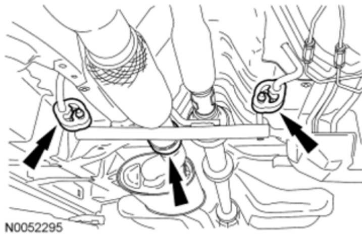
Fig. 37: Locating Exhaust Flexible Pipe Clamp Courtesy of FORD MOTOR CO.
