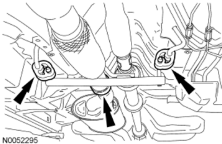
Fig. 285: Locating Exhaust Flexible Pipe Clamp Courtesy of FORD MOTOR CO.
