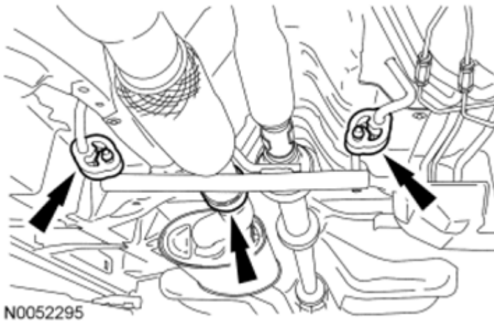
Fig. 908: Locating Exhaust Flexible Pipe Clamp Courtesy of FORD MOTOR CO.
