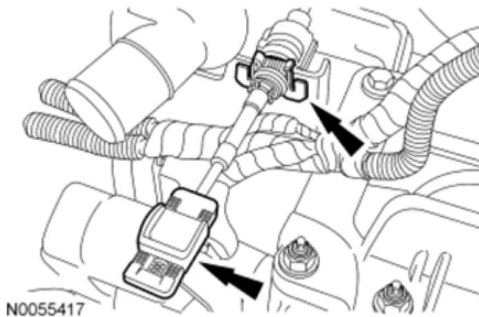
Fig. 272: Locating Transaxle Control Cable Courtesy of FORD MOTOR CO.
