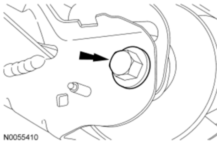
Fig. 171: Locating Engine Roll Restrictor-To-Subframe Through Bolt Courtesy of FORD MOTOR CO.
