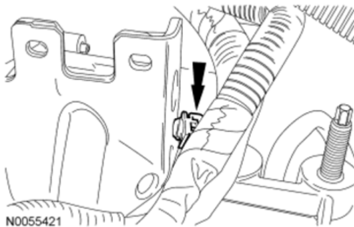
Fig. 922: Locating Wiring Harness Retainer Courtesy of FORD MOTOR CO.
