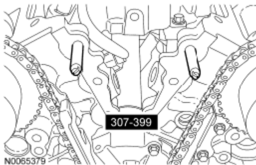
Fig. 678: Identifying Alignment Pins Courtesy of FORD MOTOR CO.
