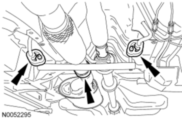
Fig. 156: Locating Exhaust Flexible Pipe Clamp Courtesy of FORD MOTOR CO.
