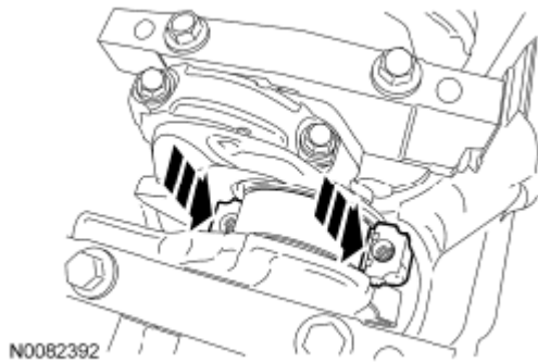
Fig. 585: Removing Piston/Rod Assembly From Engine Block Courtesy of FORD MOTOR CO.
