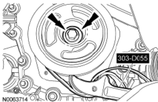
Fig. 103: Locating Crankshaft Pulley Washer And Bolt Courtesy of FORD MOTOR CO.
