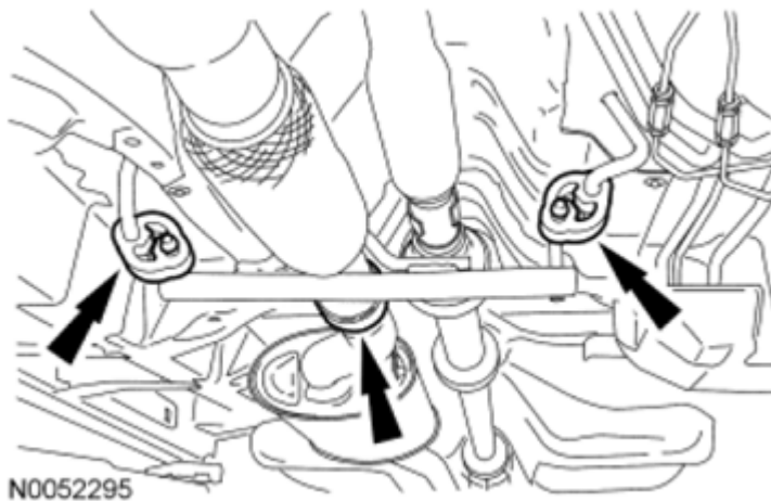
Fig. 100: Locating Exhaust Flexible Pipe Clamp Courtesy of FORD MOTOR CO.
