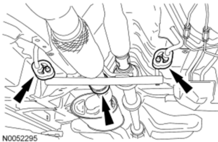
Fig. 803: Locating Exhaust Flexible Pipe Clamp Courtesy of FORD MOTOR CO.
