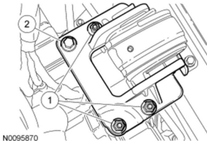
Fig. 770: Identifying Transaxle Support Insulator Bracket Nuts Courtesy of FORD MOTOR CO.
