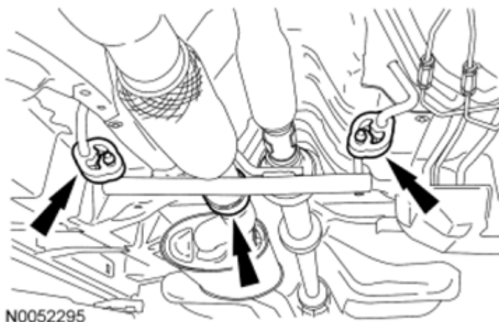
Fig. 174: Locating Exhaust Flexible Pipe Clamp Courtesy of FORD MOTOR CO.
