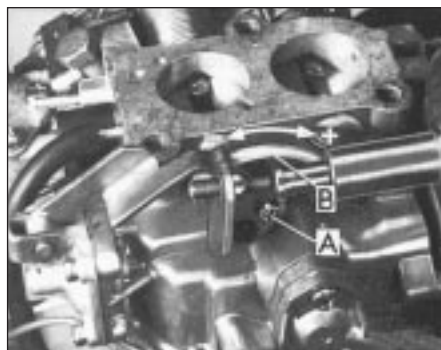
17.13 Loosen screw (A) and turn cam plate (B) in direction required to adjust accelerator pump injection capacity
