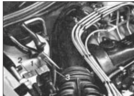
6.1 Idle speed boost valve check
