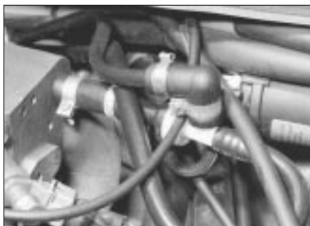
23.5 Vacuum hose-to-cylinder connector
