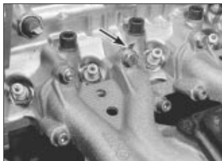
19.6 Inlet manifold-to-cylinder head securing nuts and bolts
