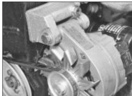
7.3 Alternator pivot bolt and bracket - 1.3 litre
