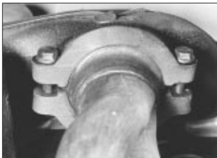
19.10 Exhaust downpipe-to-manifold flange connection - 1.3 litre
