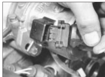
11.23a Ignition distributor electrical connection
