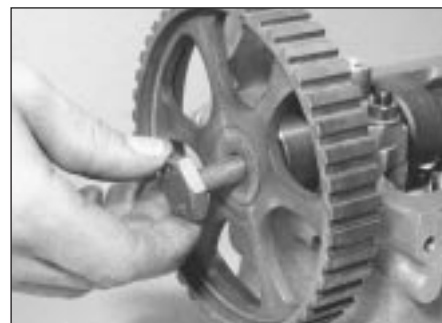
10.8 Fitting the camshaft sprocket bolt
