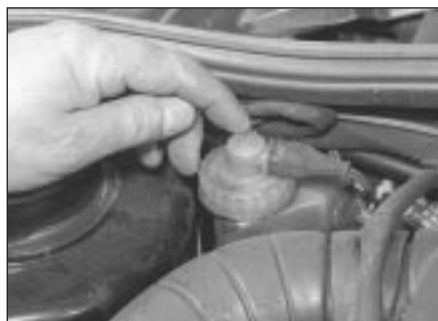
5.4 Check brake fluid level warning device
