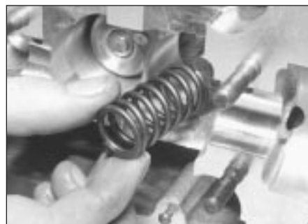
5.11b Removing an inner valve spring
