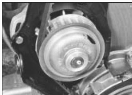
6.5 Disengage timing belt from coolant pump sprocket
