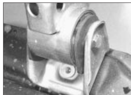
5.26a Undo front mounting through-bolt
