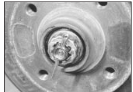
4.14 ... remove the split pin and lock ring ...
