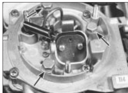
13.8 Carburettor securing bolts (arrowed) - Pierburg/Solex 2E3
