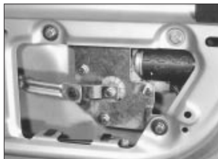
28.4b Rear wiper motor mounting in tailgate
