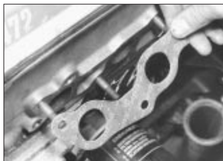
11.19 Fitting a new exhaust manifold gasket
