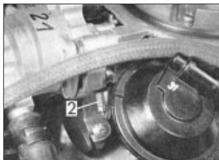
16.10 Fast idle speed adjustment screw (2)
