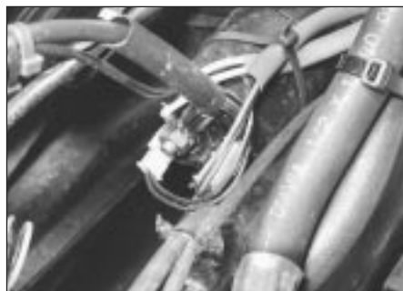
10.4 Starting motor solenoid wiring connections – 1.3 litre
