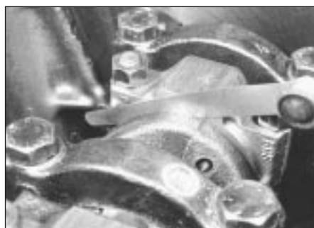
17.4 Checking connecting rod endfloat
