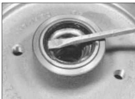
8.3 Prising out brake drum oil seal
