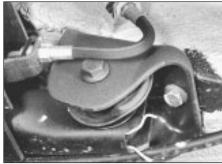
9.7 Axle beam pivot bolt head fitting position
