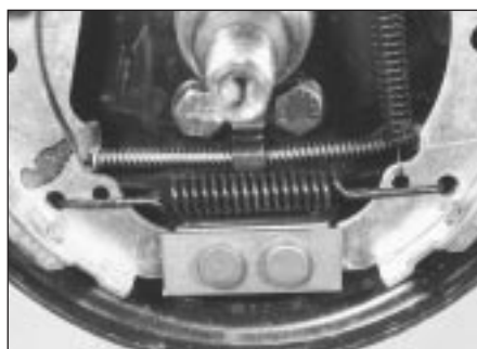
6.9 Lower return spring fixing points to brake shoes
