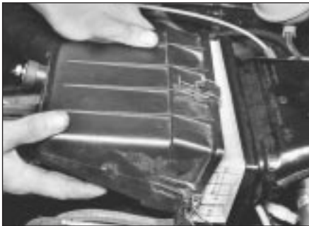
32.4c ... then remove cover to expose element - 1.6 and 1.8 litre, carburettor
