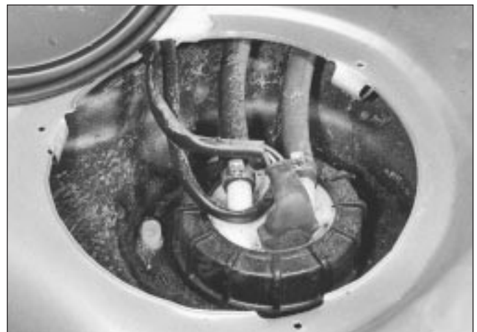
18.2 Fuel tank sender unit and connections
