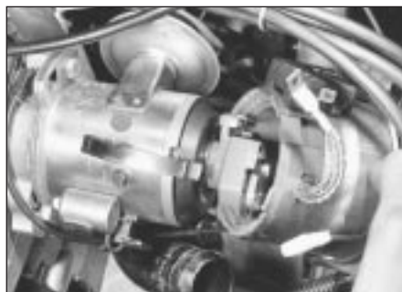
11.2 Withdraw distributor cap and screen ring
