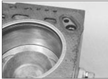
36.2 Correct fitting of cylinder head gasket
