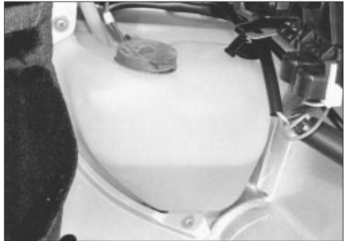
30.2 Rear window washer reservoir unit location
