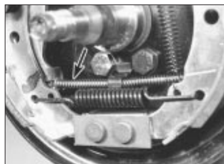
6.10 Handbrake cable attachment point to trailing brake shoe (arrowed)
