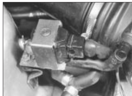
5.2 Increased idling speed valve (air conditioned models)
