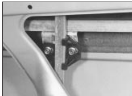
20.3b Lifting plate-to-window channel bolts
