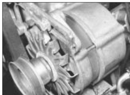
13.4b Alternator drivebelt tensioner link - 1.8 litre
