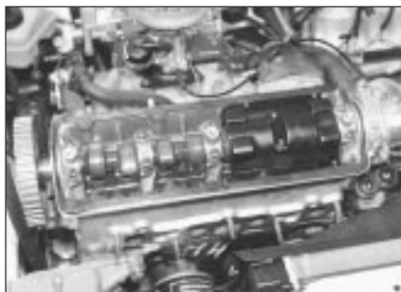
11.17 Plastic oil shield correctly located
