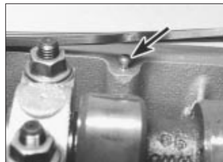
11.18 Locating dowel for valve cover gasket (arrowed)
