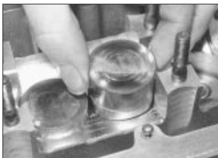
5.4 Removing an hydraulic bucket tappet
