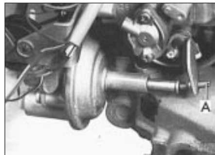
17.39b Fast idle adjustment screw (A)
