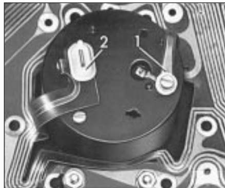
17.4 Normal type clock connections
