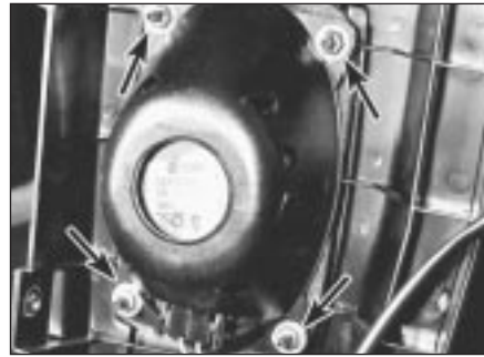
32.5 Luggage compartment loudspeaker retaining nuts (arrowed)
