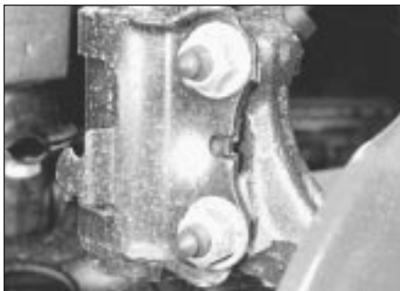
2.7 Strut-to-front wheel bearing housing retaining nuts/bolts
