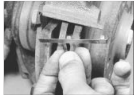
2.5 Removing a pad retaining spring
