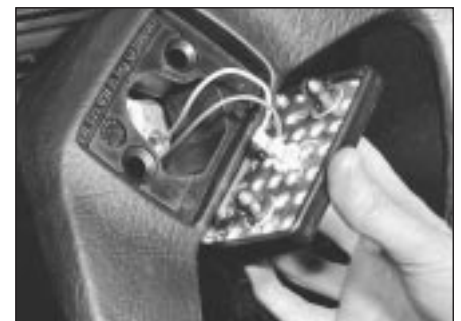
11.3a Removing steering wheel centre cover - 1.3 litre
