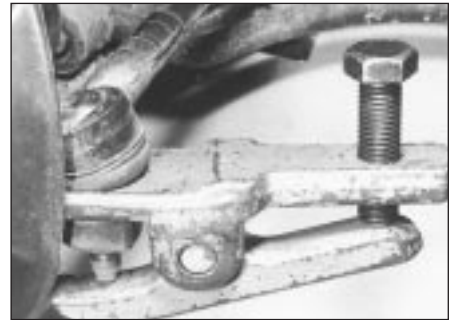
15.4 Balljoint separator tool in position on left-hand balljoint
