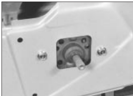
20.3a Window regulator securing bolts
