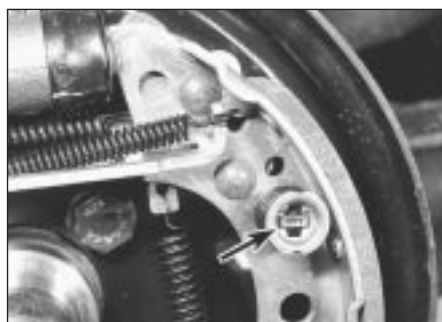
6.8 Brake shoe steady spring and cup (arrowed)
