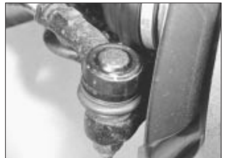
28.2 Inspect balljoint dust covers
