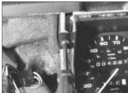
16.3 Instrument panel screw removal
