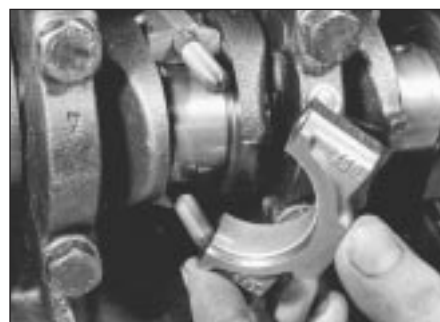
17.7 Withdrawing a big-end cap
