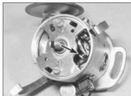
11.4 Contact breaker points viewed through window in bearing plate (arrowed) - Ducellier
