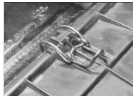
32.4a Unclip air cleaner cover ...
