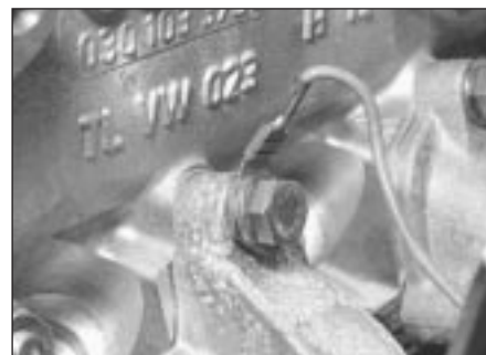
11.23d Earth lead under inlet manifold bolt head
