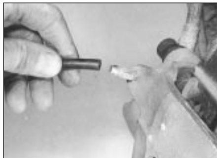
12.5 Connect bleed tube to bleed valve
