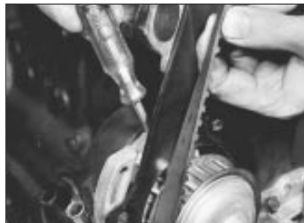
36.13 Tensioning timing belt
