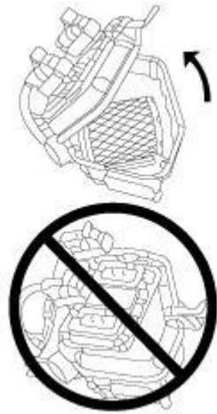
Fig. 62: Electrical Connectors At Powertrain Control Module (PCM) - DO NOT Unplug Courtesy of CHRYSLER GROUP, LLC
