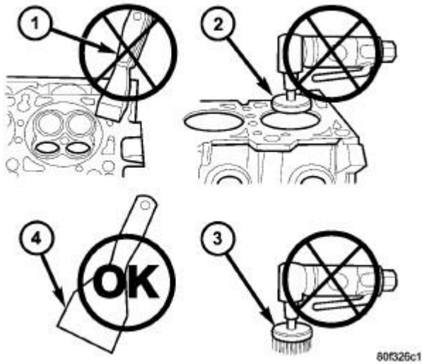
Fig. 103: Proper Tool Usage For Surface Preparation Courtesy of CHRYSLER GROUP, LLC
