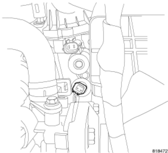
Fig. 281: Locating Variable Valve Timing Solenoid Courtesy of CHRYSLER LLC
