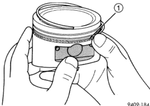
Fig. 247: Installing Side Rail Courtesy of CHRYSLER LLC
