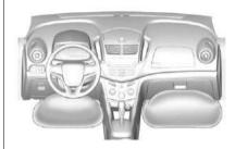
The driver knee airbag is below the steering column. The front outboard passenger knee airbag is below the glove box.
