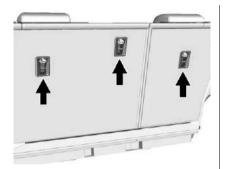
The top tether anchors are on the back of the rear seatbacks. Be sure to use an anchor on the same side of the vehicle as the seating position where the child restraint will be placed.
