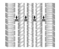
Treadwear indicators are one way to tell when it is time for new tires. Treadwear indicators appear when the tires have only 1.6 mm (1/16 in) or less of tread remaining. See *Tire Inspection on page 10-53* and *Tire Rotation on page 10-54*.
