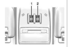
On vehicles with this feature, the sunroof only operates when the ignition is turned to ON/RUN or Retained Accessory Power (RAP) is active.
