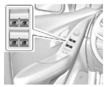
The driver door also has switches that control the passenger and rear windows. The switches work when the vehicle is in ON/RUN or ACC/ACCESSORY, or when Retained Accessory Power (RAP) is active. See Retained Accessory Power (RAP) on page 9-18.
