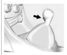
**R (Reverse):** To engage reverse, with the vehicle stationary, pull up on the button on the selector lever and engage the gear. If the gear
