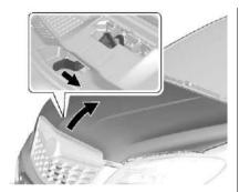
Go to the front of the vehicle and move the secondary hood release lever toward the right side of the vehicle.
