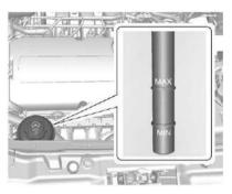
When the engine is hot, the level should be at the hot MAX level. When the engine is cold, the fluid level should be between MIN and MAX on the dipstick.
