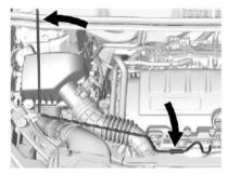
Lift the hood and release the hood prop from its retainer, above the radiator. Securely place the hood prop into the slot on the underside of the hood.
