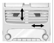
Use the air vents in the center and on the side of the instrument panel to direct the airflow. Move the slats on the center air vents to direct airflow.
