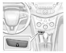
The rear door safety locks prevent passengers from opening the rear doors from inside the vehicle.
