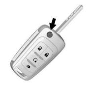
Press the key release button to extend the key blade. The key can be used for the ignition and all locks.
