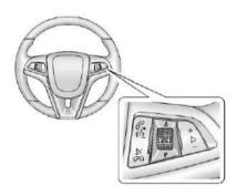
Vehicles with a Hands-Free Phone system can use a Bluetooth-capable cell phone with a hands-free profile to make and receive phone calls. The infotainment system and voice control are used to operate the
