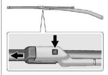
Press the release button on the top side of the wiper and pull the wiper blade out of the end of the wiper arm.
