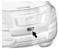
To open the liftgate from outside of the vehicle, press on the RKE transmitter, then use the touch pad.
