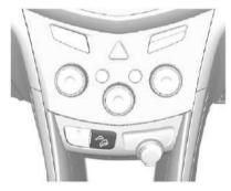
Turn the system on by pressing the DCS button located on the center stack. The green DCS light comes on steady in the instrument cluster when the system is on.
