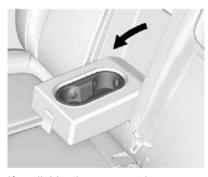
If available, the rear seat has an armrest in the center of the seatback. Lower the armrest to access the cupholders.
