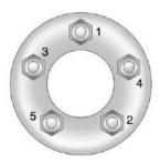
Tighten the wheel nuts firmly with the wheel wrench in a crisscross sequence, as shown. Notice: Wheel covers will not fit on the vehicle's compact spare. If you try to put a wheel cover on the compact spare, the cover or the spare could be damaged.
