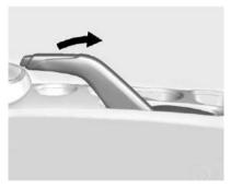
To set the parking brake, hold the brake pedal down and pull up on the parking brake lever. If the ignition is on, the brake system warning light will come on. See *Brake System Warning Light on page 5-16*.
