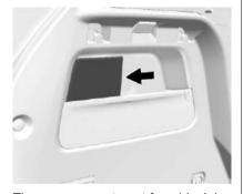
The rear compartment fuse block is behind a cover on the left side of the rear compartment. To access the fuses, remove the cover.
