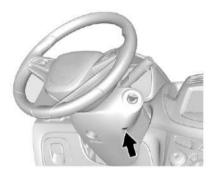
Vehicles with an automatic transmission may be equipped with an electronic key lock release system. This system is to prevent ignition key removal unless the shift lever is in P (Park).
