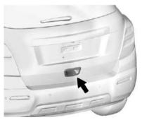
To open the liftgate, press an on the RKE transmitter, then use the touch pad.
