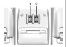
On vehicles with this feature, the sunroof only operates when the ignition is turned to ON/RUN or Retained Accessory Power (RAP) is active.
