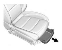
If equipped with storage under the front passenger seat, pull out to access the storage area.
