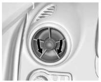
Turn the knobs on the side air vents counterclockwise or clockwise to open or close off the airflow.
