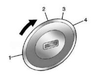
The ignition switch has four different positions.
