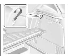
Fold the load floor. Place the hook from the load floor inside the hook on the side trim.
