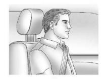
Adjust the head restraint so that the top of the restraint is at the same height as the top of the occupant's head. This position reduces the chances of a neck injury in a crash.
