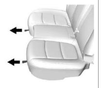
Pull the strap on the front edge of the rear seat cushion to release the cushion. Tilt the seat cushion forward toward the front of the vehicle
