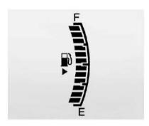
The fuel gauge indicates about how much fuel is left when the ignition is turned to ON/RUN.
