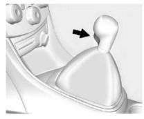
To engage reverse, with the vehicle stationary, pull up on the button on the selector lever and engage the gear. If the gear does not engage, set the lever in neutral, release the clutch pedal and apply it again; then repeat gear selection.
