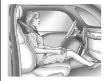
If a person of adult size is sitting in the front outboard passenger seat, but the off indicator is lit, it could be because that person is not sitting properly in the seat. Use the following steps to allow the system to detect that person and enable the front outboard passenger frontal airbag:
