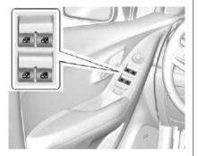
Press the switch to lower the window. Pull up on the front edge of the switch to raise it. See *Power Windows on page 2-14*.
