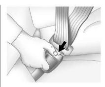
To unlatch the belt, push the button on the buckle. The belt should return to its stowed position. Slide the latch plate up the safety belt webbing when the safety belt is not in use.
