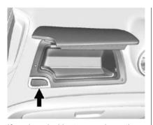
If equipped with storage above the glovebox, push the button to open.
