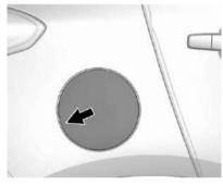
To open the fuel door, push the rearward center edge in and release and it will open.
