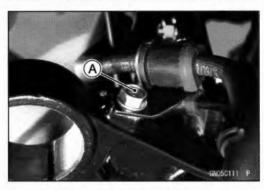
Remove: Steering Stem Head Nut Plug [A] Steering Stem Head Nut [B] Washer [C]
