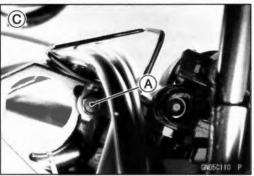
• Remove the brake hose bracket bolts [A].
