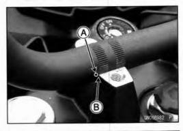
Install the handlebar holder [A] direction as shown.
