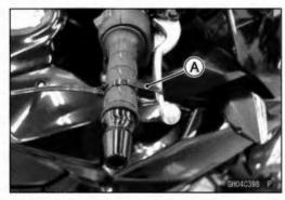
Remove the muffler mounting bolt [A] and move the exhaust pipe downward.
