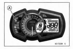
With the engine stopped and turned in the self-diagnosis mode, the service code [A] is displayed on the LCD by the number of two digits.
