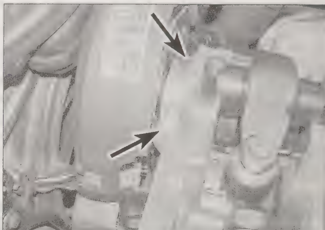
4.9b Apply sealant to the points (arrowed) on the cylinder head
