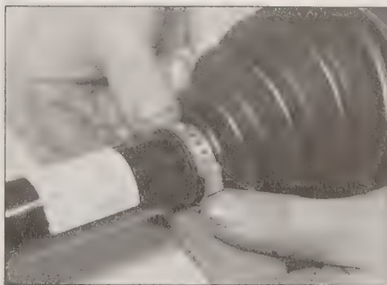
3.17a Compress the raised section of the gaiter securing clip ...
