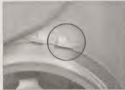
3.4c Timing mark scribed on inner flange of pulley aligned with TDC mark on timing belt cover – 1.4 litre engine
