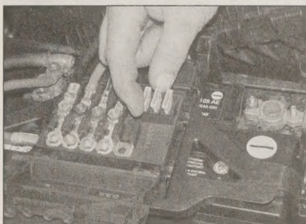
B Check the fuses and fusible links in the fusebox located on top of the battery.
