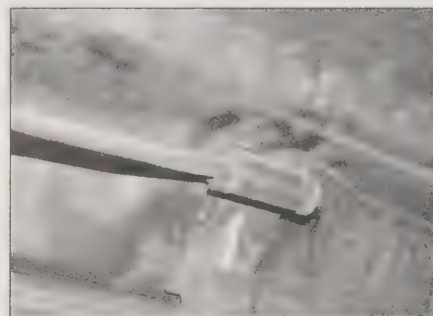
20.11 Turn the eccentric to adjust the jet
