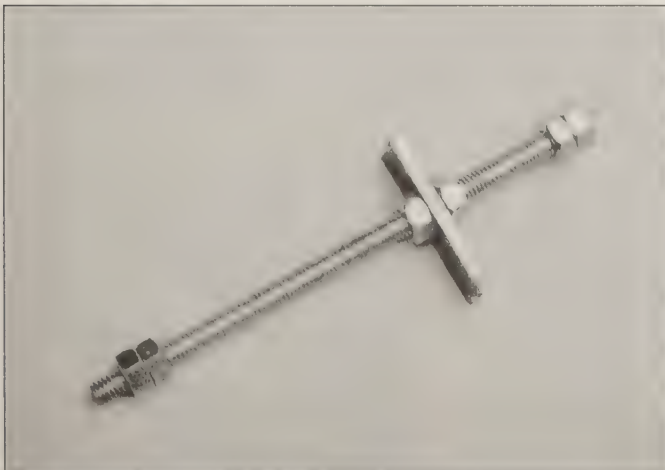
13.9a Home-made tool for locking camshaft adjuster, or chain tensioner, in position – 1.8 litre engine
