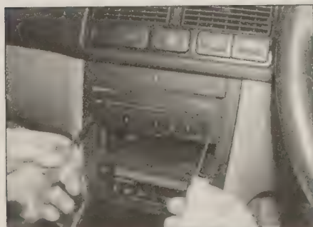
21.7a Using feeler blades to remove the CD player
