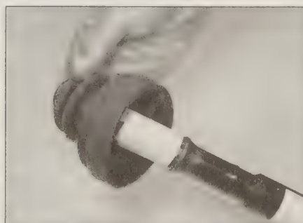
3.34a Tape over the driveshaft splines to protect the new gaiter ...
