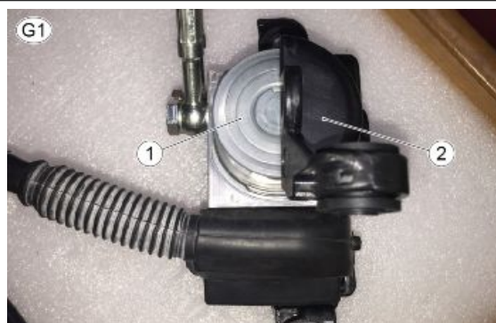
G TABLES - PRE-FITTING OF ABS - PROCEDURE FOR INSERTION OF ABS CONNECTOR
