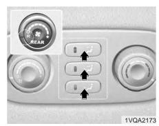
When the rear fan speed control (REAR) knob in the front climate control panel is in the R position, the rear mode is selected by pushing the rear mode selection button on the rear control panel as follows:
