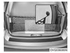
To keep items from shifting in the cargo area, you can use the four holders located in the cargo area to attach the luggage net.
