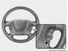
3. Push the COAST/SET switch, and release it at the desired speed. The SET indicator light in the instrument cluster will illuminate. Release the accelerator at the same time. The desired speed will automatically be maintained.
