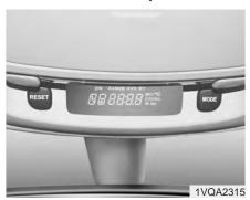
The trip computer is a microcomputercontrolled driver information system that displays information related to driving, including compass, distance to empty, driving time, average fuel consumption and outside temperature on the display when the ignition switch is in ON position. All stored driving information is reset if the battery is disconnected.
