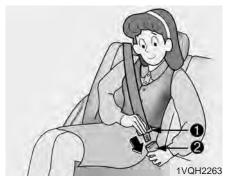
3. Insert the tongue plate (1) into the open end of the buckle (2) until an audible "click" is heard, indicating the belt is locked in the buckle.
