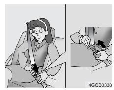
To unfasten the lap/shoulder belt: Press the release button on the buckle and allow the belt to slowly retract.
