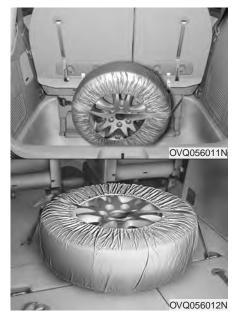
Place the flat tire in the cargo area when the 3rd row seat is upright position or on the floor when the 3rd row seat is stowed in the cargo area.
