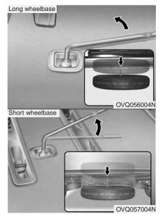
3. Use the wheel lug nut wrench to loosen the bolt enough to lower the spare tire.
