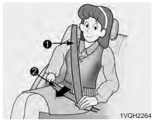
4. Position the lap portion (2) of the belt across your lap as LOW ON THE HIPS as possible to reduce the risk of sliding under it during an accident. Adjust the belt to a SNUG FIT by pulling up on the shoulder portion (1) of the safety belt. The belt retractor is designed to take up excess webbing automatically and to maintain tension on the belt. For your safety, do not put any excess slack into the safety belt at any location.
