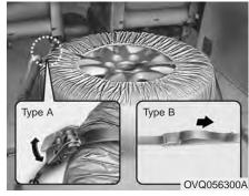
4. **Type A**: Tighten the strap firmly using the ratchet.
