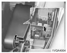
Pull the suspected fuse straight out. Use the removal tool provided on the main fuse box in the engine compartment.
