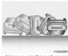
Air bags may not inflate in rollover accidents because air bag deployment would not provide proper protection to the occupants.
