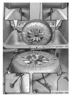
3. If necessary, connect the two straps with the buckle.
