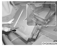
Release the strap and push the seat forward firmly until it clicks into place to insert the catches into the anchors.
