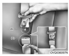
Insert the tongue plate (A) into the open end of the buckle (C) until an audible "click" is heard, indicating the latch is locked. Make sure the belt is not twisted.
