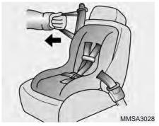
3. Pull the shoulder portion of the safety belt all the way out. When the shoulder portion of the safety belt is fully extended, it will shift the retractor to the "Auto Lock" (child restraint) mode.
