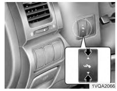
To adjust the position of the accelerator and brake pedals, push the switch with the shift lever in the P position.
