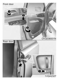
To lock a door without the key, push the inside door lock button (1) or door lock switch (2) to the "Lock" position and close the door (3).
