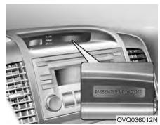
If there is no passenger in the front passenger seat or if the passenger in the front passenger seat is very light, (such as a child), the front **PASSENGER AIR BAG OFF** indicator may illuminate.
