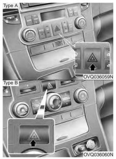
The hazard warning flasher causes the front and rear turn signal lights to flash on and off, which serves as a warning to other drivers to exercise caution when approaching or passing your vehicle.
