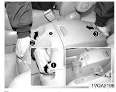
The center console storage can be removed and reinstalled.
