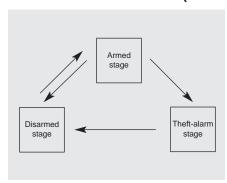
This system is designed to provide protection from unauthorized entry into the car. This system is operated in three stages: the first is the "Armed" stage, the second is the "Theft-alarm" stage, and the third is the "Disarmed" stage. If triggered, the system provides an audible alarm with blinking of the hazard warning lights.
