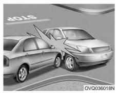
Front air bags may not inflate in side impact collision, because occupants move to the direction of the collision, and thus in side impacts, frontal air bag deployment does not provide occupant protection.
