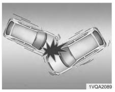
In a slant or angled collision, the force of impact may direct the occupants in a direction between the front and side air bags, and thus the sensors may not deploy any air bags.
