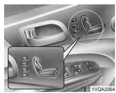
A driver position memory system is provided to store and recall the driver seat, outside rearview mirror and adjustable pedal positions with a simple button operation. By saving the desired positions into the system memory, different drivers can reposition the driver seat, outside rearview mirror and adjustable pedal based upon their driving preference.
