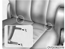
ISOFIX anchors have been provided in your vehicle. The ISOFIX anchors are located in the left and right outboard rear seating positions. Their locations are shown in the illustration. There is no ISOFIX anchor provided for the center rear seating position.
