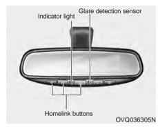
Your new mirror comes with an integrated HomeLink Universal Transceiver, which allows you to program the mirror to activate your garage door(s), estate gate, home lighting, etc. The mirror actually learns the codes from your various existing transmitters.
