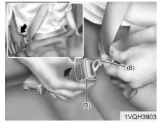
3. Pull the tongue plate (B) and insert the tongue plate (B) into the open end of the buckle (D) until an audible "click" is heard, indicating the latch is locked. Make sure the belt is not twisted.
