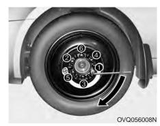
11. Once the wheel lug nuts have been tightened, lower the vehicle fully to the ground and continue to tighten the lug nuts until they are fully secured. Tighten the wheel lug nuts firmly in a " \* " pattern.
