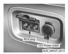
Connecting Other Devices to the RSE Electronic devices such as video game systems, VHS players, Camcorder or etc, can be played through the RSE. These external devices can be connected to the unit via RCA plugs available throughout the vehicle. DC power for additional electronic equipment is provided by one of the 12-volt power outlets located in the dash, third row and cargo areas. Additional information can be found in the vehicle manual.
