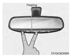
When programming the buttons for the first time, press and hold the left and center buttons (♠,♠) simultaneously until the indicator light begins to flash after approximately 20 seconds. (This procedure erases the factory-set default codes. Do Not perform this step to program additional hand-held transmitters.)
