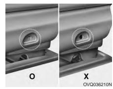
4. Make sure the green mark on the rear seat cushion frame is visible and the catches are locked in position by moving the seat forward and backward or lifting the front portion of the seat. If the green mark is invisible and the seat moves, it is not locked properly.
