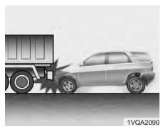
Just before impact, drivers often brake heavily. Such heavy braking lowers the front portion of the vehicle causing it to "ride" under a vehicle with a higher ground clearance. Air bags may not inflate in this "under-ride" situation because deceleration forces that are detected by sensors may be significantly altered by such "under-ride" collisions.
