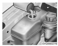
The coolant level should be filled between F and L marks on the side of the coolant reservoir when the engine is cool.
