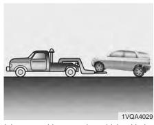
It is acceptable to tow the vehicle with the rear wheels on the ground (without dollies) and the front wheels off the ground. When being towed by a commercial tow truck and wheel dollies are not used, the front of the vehicle should always be lifted, not the rear.
