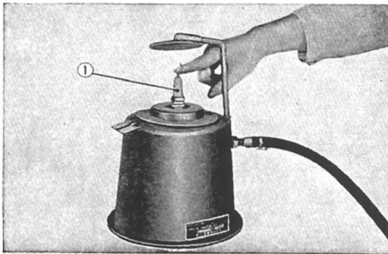
Fig. 6.12 Spark plug cleaning ① Spark plug
