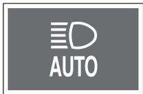
Pushing the light switch lever toward the instrument panel with the light switch in AUTO position activates the High Beam Assist System (HBAS) and turns on this indicator.
