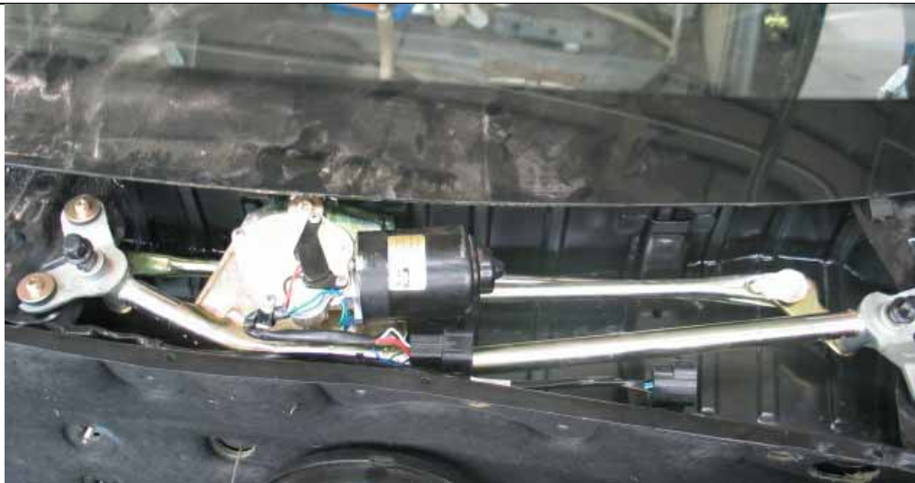
Installation of the wiper abutment
