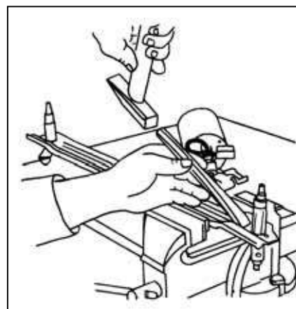
Removal of the wiper abutment
