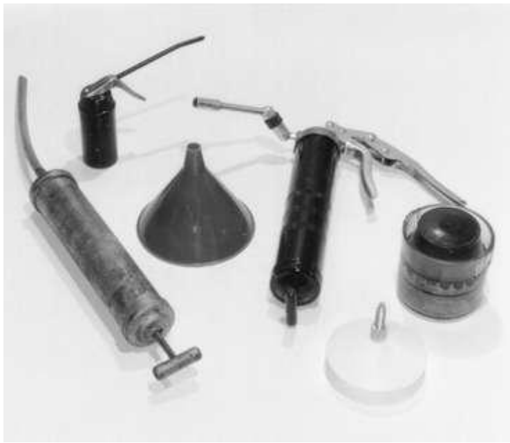
Fig. 5: Special tools make lubrication easier, from left to right: Oil Suction Gun; Oil Can; Funnel; Grease Gun; and Wheel Bearing Packers
