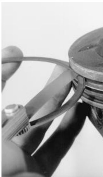
Checking ring groove clearance
