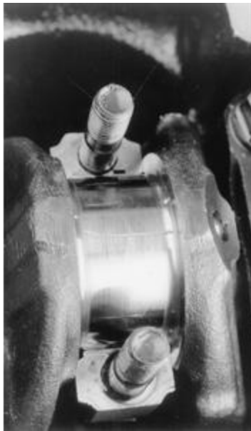
Checking bearing clearance with gauging material
