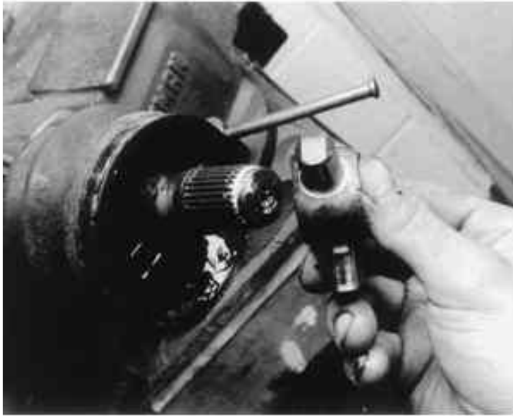
Removing the CV-joint inner snap ring
