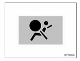
This indicator comes on when the ignition key is turned to the "ON" position. It goes off after about 6 seconds. This means the SRS side airbags and curtain shield airbags are operating properly.
