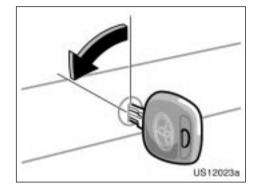
After closing the trunk lid, insert the master key and turn it counterclockwise to deactivate the lock release lever.
