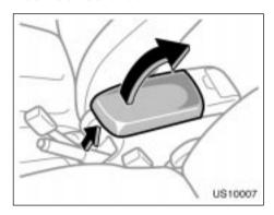
To access the rear console box, pull up the lock release lever while raising the rear console box lid.
