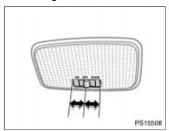
To turn on the interior light, slide the switch.
