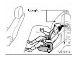
Split seat: When installing a child restraint system in the rear seat center position, return both the left and right seatbacks to the upright position. Otherwise, the child restraint system cannot be securely restrained and this may cause death or serious injuries in a collision.
