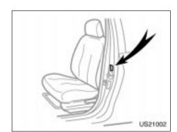
● The gross vehicle weight must not exceed the Gross Vehicle Weight Rating (GVWR) indicated on the Certification Label. The gross vehicle weight is the sum of weights of the unloaded vehicle, driver, passengers, luggage, hitch and trailer tongue load. It also includes the weight of any special equipment installed on your vehicle.
