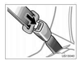
2. To remove the booster seat, press the buckle release button and allow the belt to retract.
