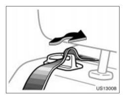
Remove the seat belt from the seat belt guide.
