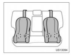
The lower anchorages for the child restraint system interfaced with the FMVSS225 or CMVSS210.2 specification are installed in the rear seat.
