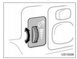
To adjust the brightness of the instrument panel lights, turn the dial.
