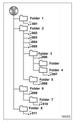
o The turn of play of the compact disc having the structure shown on the left is as follows:
