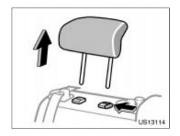
When the child restraint system is installed in a forward-facing position: Remove the head restraint.
