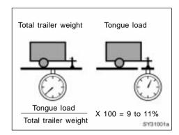
• The trailer cargo load should be distributed so that the tongue load is 9 to 11% of the total trailer weight, not exceeding the maximum of 32 kg (70 lb.). Never load the trailer with more weight in the back than in the front. About 60% of the trailer load should be in the front half of the trailer and the remaining 40% in the rear.
