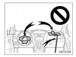
• Do not put anything or any part of your body on or in front of the dashboard or steering wheel pad that houses the front airbag system. They might restrict inflation or cause death or serious injury as they are projected rearward by the force of deploying airbags. Likewise, the driver and front passenger should not hold objects in their arms or on their knees.
