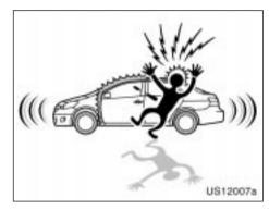
To deter vehicle theft, the system is designed to sound an alarm if any of the doors, trunk or hood is forcibly unlocked or the battery terminal is disconnected and the reconnected when the vehicle is locked.
