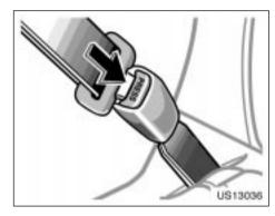
5. To remove the convertible seat, press the buckle release button and allow the belt to retract completely. The belt will move freely again and be ready to work for an adult or older child passenger. After returning the seat to its original position, be certain to replace the head restraint.
