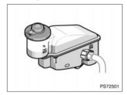
Before checking or adding the brake fluid, remove the cover. (See "(c) Jump starting" on page 215 in Section 4.)
