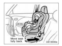
• A forward-facing child restraint system should be allowed to be installed on the front passenger seat only when it is unavoidable. Always move the seat as far back as possible even if the "AIRBAG OFF" indicator light is illuminated, because the front passenger airbag could inflate with considerable speed and force. Otherwise, the child may be killed or seriously injured.
