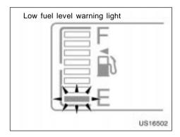
If the low fuel level warning light flashes, fill the fuel tank as soon as possible. Further fuel reduction makes the light blink quicker.
