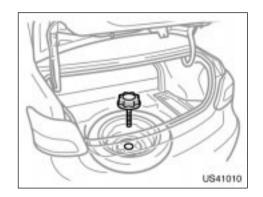
To remove the spare tire, loosen the bolt and remove it.
