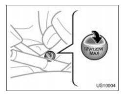
The power outlet is designed for power supply for car accessories. To use the power outlet, open as shown in the illustration.
