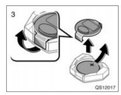
3. Remove the battery cover of the module.
