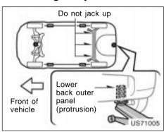
When jacking up your vehicle with the jack, position the jack correctly as shown in the illustration.
