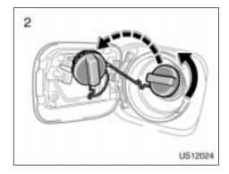
To remove the fuel tank cap, turn the cap slowly counterclockwise, then pause slightly before removing it. After removing the cap, hang it on the cap hanger.
