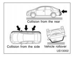
The SRS airbags are not generally designed to inflate if the vehicle is involved in a side or rear collision, if it rolls over, or if it is involved in a low-speed frontal collision. But, whenever a collision of any type causes sufficient forward deceleration of the vehicle, deployment of the SRS airbags may occur.
