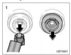
1. Open the hood. Unplug the connector. Remove the rubber cover.
