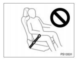
• If the seat belt extender has been connected to the driver's seat belt buckle without wearing the seat belt when using the extender in the driver's seat, the SRS driver's airbag system will judge that the driver wears the seat belt even if not wearing it. In this case, the driver's airbag may not activate correctly, causing death or serious injury in the event of collision. Be sure to wear the seat belt with the seat belt extender.
