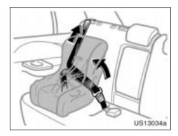
4. While pressing the convertible seat firmly against the seat cushion and seatback, let the shoulder belt retract as far as it will go to hold the convertible seat securely.
