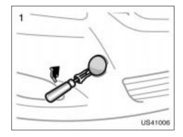
Remove the front towing eyelet cover on the front bumper, using a flathead screwdriver which is wrapped with a cloth.
