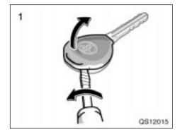
1. Open the cover using a flathead screwdriver wrapped with plastic tape.
