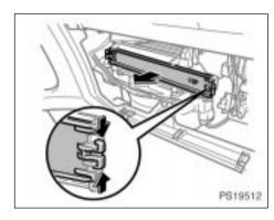
3. Pinch the knobs located on each side and remove the filter cover.
