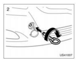
2. Use the towing eyelet in the tool bag. Secure the front towing eyelet to the hole on the front bumper by turning clockwise. (For the tool bag storage location, see "—Required tools and spare tire" on page 222.)
