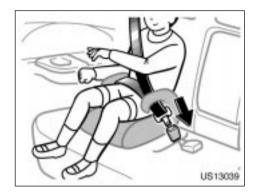
Sit the child on a booster seat. Run the lap and shoulder belt through or around the booster seat and across the child following the instructions provided by its manufacturer and insert the tab into the buckle taking care not to twist the belt.
