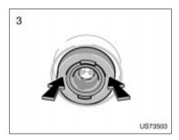
3. Install the rubber cover as shown and fit it securely on the boss. Plug in the connector.
