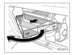
4. Pull out the filter and rotate it as shown in the illustration to remove. Inspect the filter on the surface.
