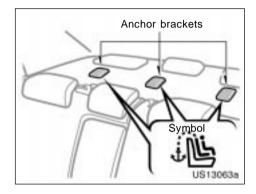
Use the anchor brackets on the luggage compartment to attach the top strap.
