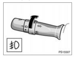
To turn on the front fog lights, twist the band of the headlight and turn signal switch lever. They will come on when the head lights are on low beam.
