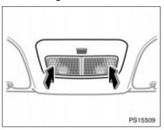
To turn on the personal light, push the lens. To turn the light off, push the lens once again.
