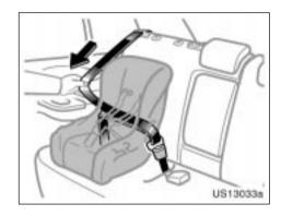
3. Fully extend the shoulder belt to put it in the lock mode. When the belt is then retracted even slightly, it cannot be extended.
