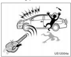
Pushing the panic switch for 1 second blows the horn intermittently and flashes the headlights, tail lights and emergency flashers and turns on the interior light.
