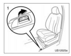
1. To open the fuel filler door, pull the lever up.
