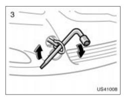
3. Tighten the front towing eyelet securely by a wheel nut wrench.
