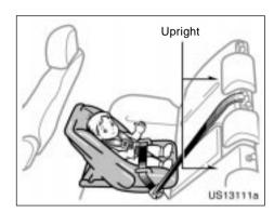
Split seat: When installing a child restraint system in the rear seat center position, return both the left and right seatbacks to the upright position. Otherwise, the child restraint system cannot be securely restrained and this may cause death or serious injuries in a collision.
