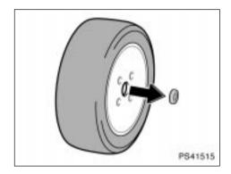
Aluminum wheels—Before stowing the flat tire, remove the center wheel ornament by pushing from the reverse side.
