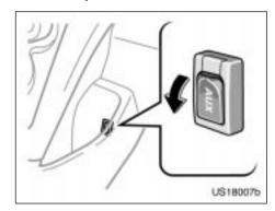
An AUX adapter is installed in the center pocket.
