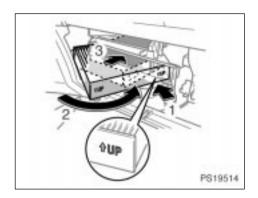
When inserting the filter in the filter outlet, keep the arrow pointing up and insert the filter as shown in the illustration above.
