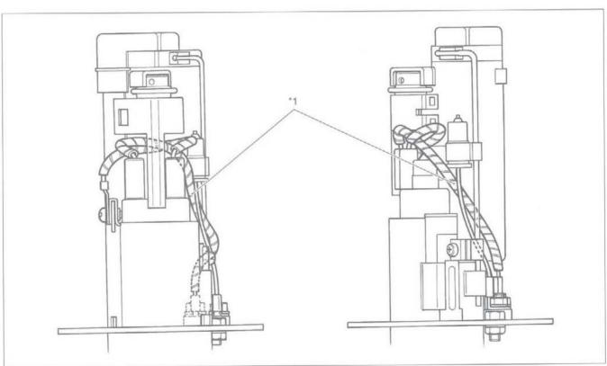
\*1: Pass through the wires behind the thermistors.
