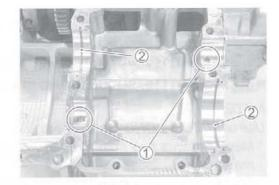
· Install the countershaft assembly on the middle crankcase.
