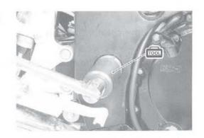
Hold the swingarm pivot shaft 6 and remove the swingarm pivot nut 7.
