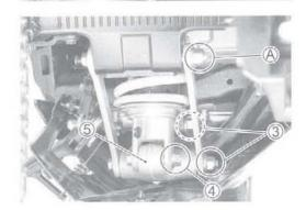
Remove the swingarm pivot shaft lock-nut with the special tool.
