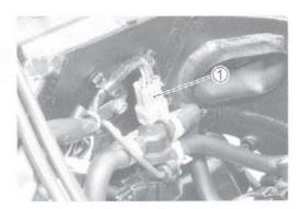
Remove the ignition switch mounting bolts with the special tools.
