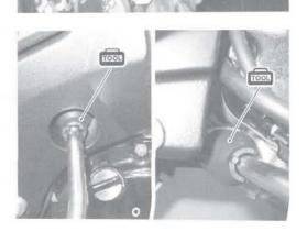
• Tighten all engine mounting bolts and nuts to the specified torque. ( 3-12)
