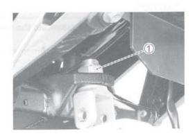
Install the rear shock absorber and tighten the rear shock absorber upper/lower mounting nuts to the specified torque.
