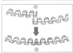
Install the 2nd ring ③ and the 1st ring ④ to the piston.
