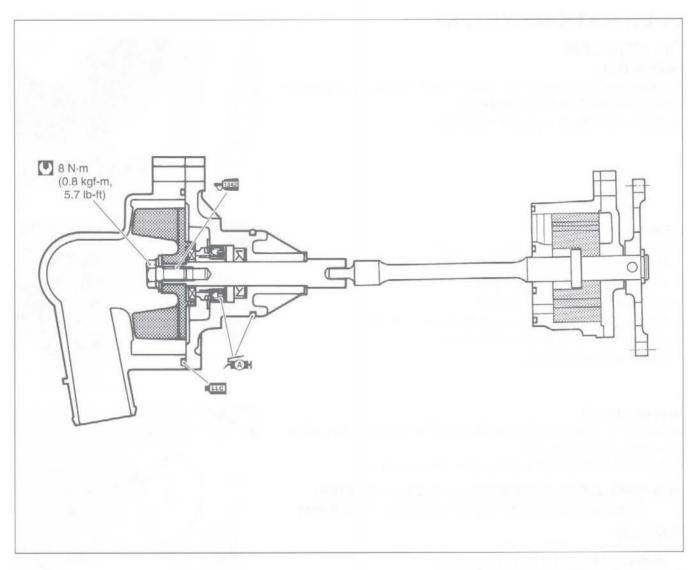
· Tighten the water pump mounting bolts to the specified torque.
