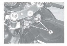
• Lift and support the fuel tank with the fuel tank prop stay 2.
