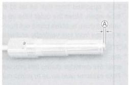
Install the front fork cap bolt ③ to the rebound damping force adjuster.
