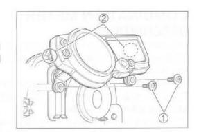
· Disassemble the combination meter as follows.
