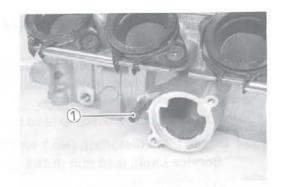
Apply SUZUKI BOND to the thread part of water bypass union and tighten it to the specified torque.
