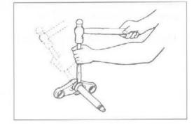
· Drive out the steering stem bearing outer races (upper and lower) using the steel rod.
