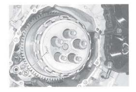
· Hold the clutch housing with the special tool.
