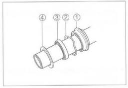
• Insert the inner tube into the outer tube and fit the oil seal and dust seal with the special tool.
