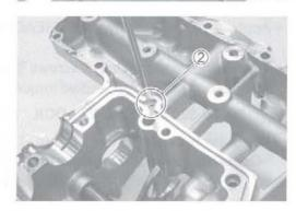
· Remove the oil jet 3 (for cam chain tension adjuster) from the cylinder head.
