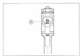
• Check the corresponding crank pin O.D. code number ("1", "2" or "3") 🖲.
