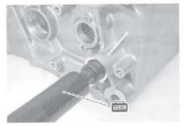
• Install the gearshift cam 4 with the bearing 5.
