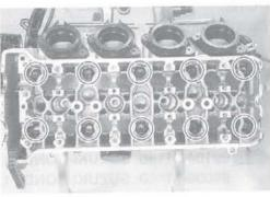
Apply SUZUKI SUPER GREASE "A" to the O-rings and install them into the cylinder head.
