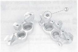
Place a rag over the pistons to prevent it from popping out and then force out the pistons using compressed air.
