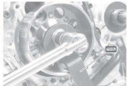
• Install a bolt (A) of suitable size to the left end of crankshaft.
