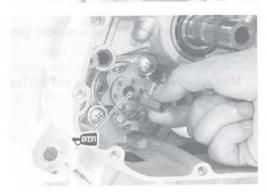
Install the gearshift shaft assembly 7 and washer 8 as shown.
