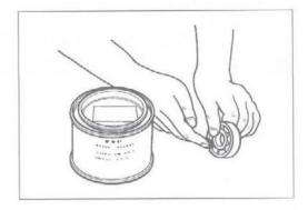
. Install the new bearing to the sprocket mounting drum with the special tool.
