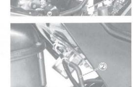
· Place the measuring cylinder and insert the fuel hose end into the measuring cylinder.
