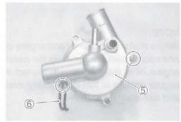
· Remove the impeller securing bolt by holding the impeller with a water pump pliers.
