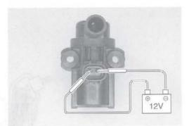
· Check the resistance between the terminals of the PAIR control solenoid valve.
