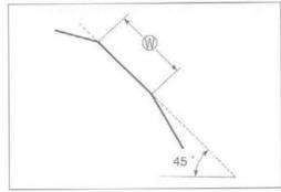
If the valve seat is pitted or burned, use the 45 ° cutter to condition the seat some more.
