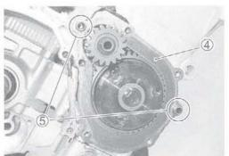
· Install the starter clutch cover and tighten its bolt as shown.
