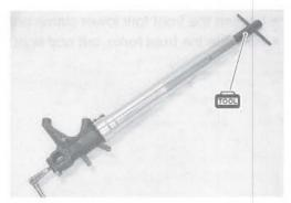
• Remove the inner rod/damper rod (cartridge) 8.
