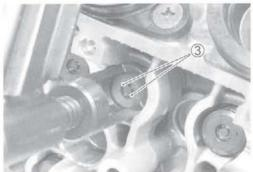
When compressing the exhaust valve spring, use a protector that is handcrafted from a 35-mm film cartridge as shown in the right illustration.
