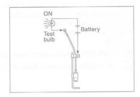
When the switch is immersed in water under the above condition, the bulb should go out. If the bulb remains lit, replace the unit with a new one.
