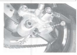
· Remove the brake pads.
