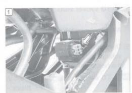
5) Measure the resistance between terminal (A) and terminal (B).
