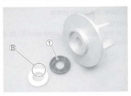
• Install the washer ② and seal washer ③ onto the impeller securing bolt 4).
