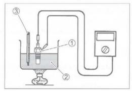
If the ECT sensor ohmic value does not change in the proportion indicated, replace it with a new one.
