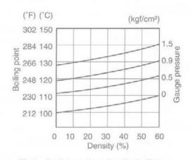
Fig.2 Engine coolant density-boiling point curve.
