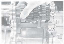
• Install the driveshaft assembly on the middle crankcase.
