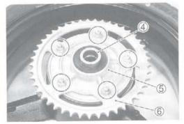
Remove the rear sprocket mounting drum spacer T.
