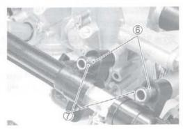
· Install the fuel delivery pipe assembly 6 to the throttle body assembly.
