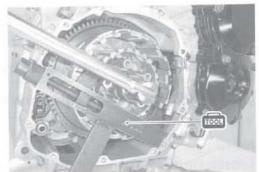
• Remove the concaved washer ⑦, washer ⑧ and clutch sleeve hub ⑨.
