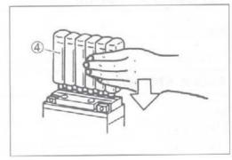
. Make sure air bubbles (5) are coming up each electrolyte container, and leave in this position for about more than 20 minutes.
