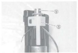
· Remove the fuel pump 10 from the fuel pump case/fuel filter cartridge 11).
