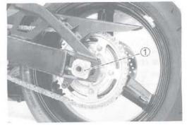
• Remove the rear wheel by disengaging the drive chain.
