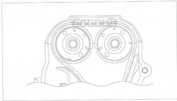
• Install the dowel pins 3.
