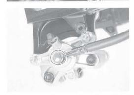
· Remove the brake hose guide 2.
