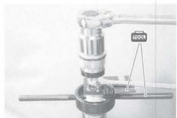
• Remove the front fork cap bolt/adjuster ②, rubber seat ③, washer ④, retainer ⑤, spacer ⑥ and spring ⑦.
