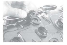
• Tighten the head cover bolts to the specified torque.
