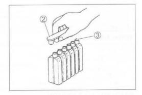
· Insert the nozzles of the electrolyte container 4 into the battery's electrolyte filler holes, holding the container firmly so that it does not fall. Take precaution not to allow any of the fluid to spill.
