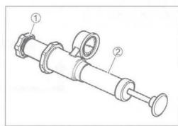
PATA Radiator cap valve opening pressure
