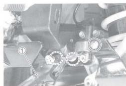
· Remove the rear brake hose union bolt.
