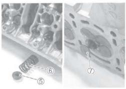
Remove the oil seal ® and spring seat ®.
