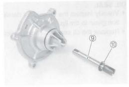
Remove the mechanical seal with the special tool.
