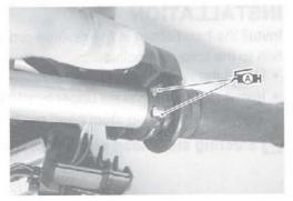
When installing the right and left handle switches, engage the stopper with the handlebar hole.
