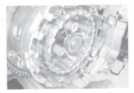
• Remove the clutch push rod 6.
