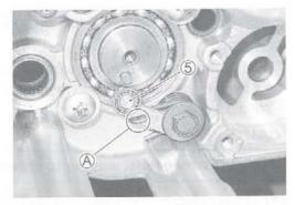
Install the gearshift cam stopper plate 6.
