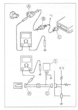
Disconnect the connector/coupler included in circuit (coupler
