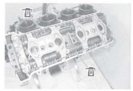
Install the PAIR reed valves ① along with the gaskets.
