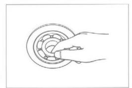
· Remove the sprocket mounting drum bearing 1 and wheel bearing 2 with the special tool.
