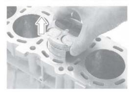
• Remove the piston pin circlip ①.
