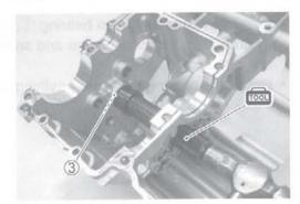
· Install the oil seal with the special tool.
