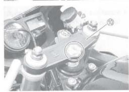
Remove the handlebars 11 to upward.
