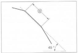
After the desired seat position and width is achieved, use the 45 ° cutter very lightly to clean up any burrs caused by the previous cutting operations.
