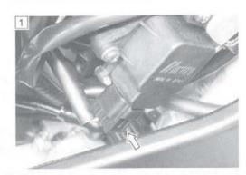
5) Turn the ignition switch ON to check the STVA operation. (STV operating order: Full open → 3/4 open)
