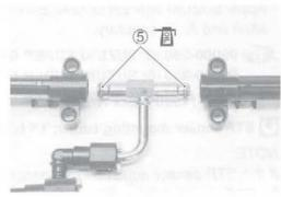
· Assemble the fuel delivery pipes as shown.
