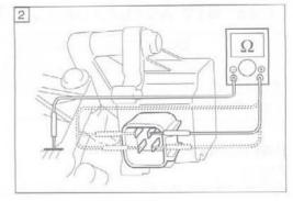
If OK, then measure the STVA resistance. (between terminal (A) and terminal (B) and (between terminal (C) and terminal (D))
