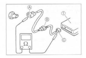
• Disconnect the coupler ® and measure resistance between couplers ® and ®.
