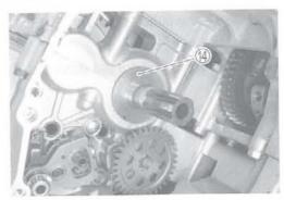
Remove the oil pump drive gear (5) from the primary driven gear assembly (6).
