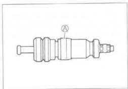
Any dust or rust around the valve hole  $\[mathbb{B}\]$  must be cleaned off. Then install the valve in the rim.
