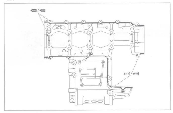
Tighten the crankshaft journal bolts (9 mm) in ascending order of numbers assigned to these bolts. Tighten each bolt a little at a time to equalize the pressure in the following two steps.
