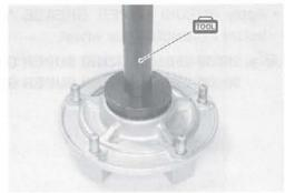
· First install the right wheel bearing, then install the left wheel bearing with the special tools.
