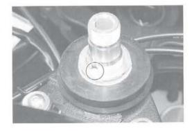
· Install the steering stem lock-nut and tighten it to the specified torque with the special tools.
