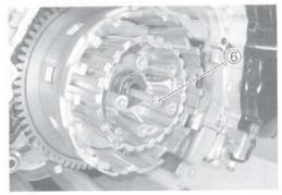
· Unlock the clutch sleeve hub nut.
