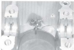
· Remove the oil jet ② (for transmission) from the lower crankcase.
