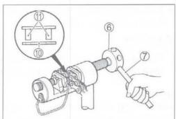
Continue pressing the joint plate until the distance between the two joint plates come to the specification.
