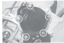
Remove the concaved washer ①, washer ② and starter idle gear No.1 ③.
