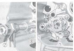
Install the washer ① and snap ring ①.
