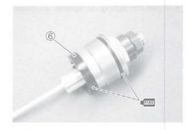
Pull up the inner rod with the special tool ©.
