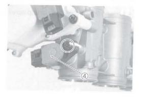
Remove the STP sensor (5) with the special tool.
