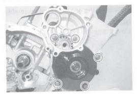
Remove the concaved washer ⑦, starter idle gear No.2 ® and shaft ⑨.
