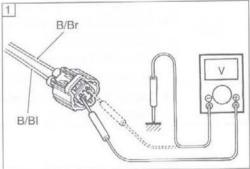
1) Connect the TP sensor coupler ① to the test harness.
