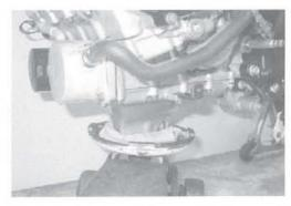
Remove the engine mounting bolts ①.
