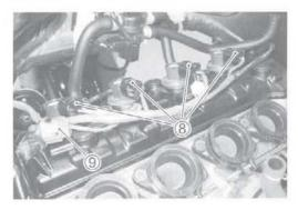
Remove the ignition coils/plug caps ①.
