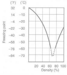
Fig.1 Engine coolant density-freezing point curve.
