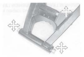
Draw out the swingarm pivot bearings ① and the swingarm cushion rod upper bearings ② with the special tool.
