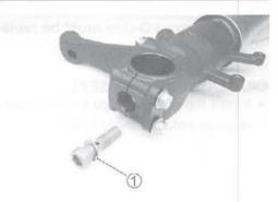
Tighten the damper rod bolt to the specified torque with the special tool.
