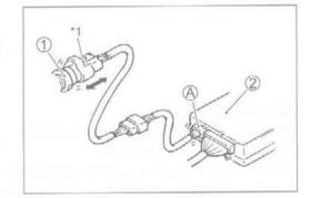
Using a test male terminal, check the female terminals of the circuit being checked for contact tension.
