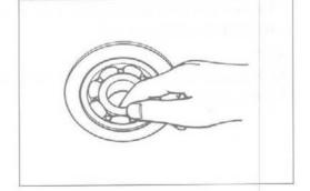
Remove the wheel bearings with the special tool.
