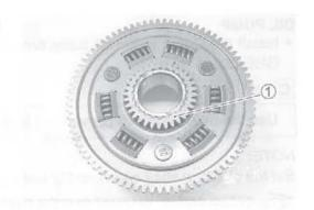
· Install the primary driven gear assembly.
