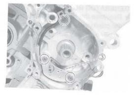
Apply SUZUKI BOND lightly to the groove of signal generator lead wire gromet.
