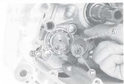
. Apply a small quantity of THREAD LOCK to the gearshift cam stopper plate bolt and tighten it to the specified torque.
