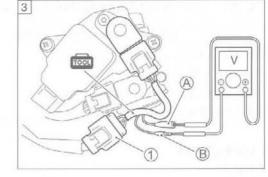
STP sensor output voltage
