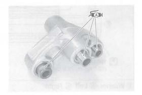
Assemble the cushion rods ① onto the swingarm temporarily.
