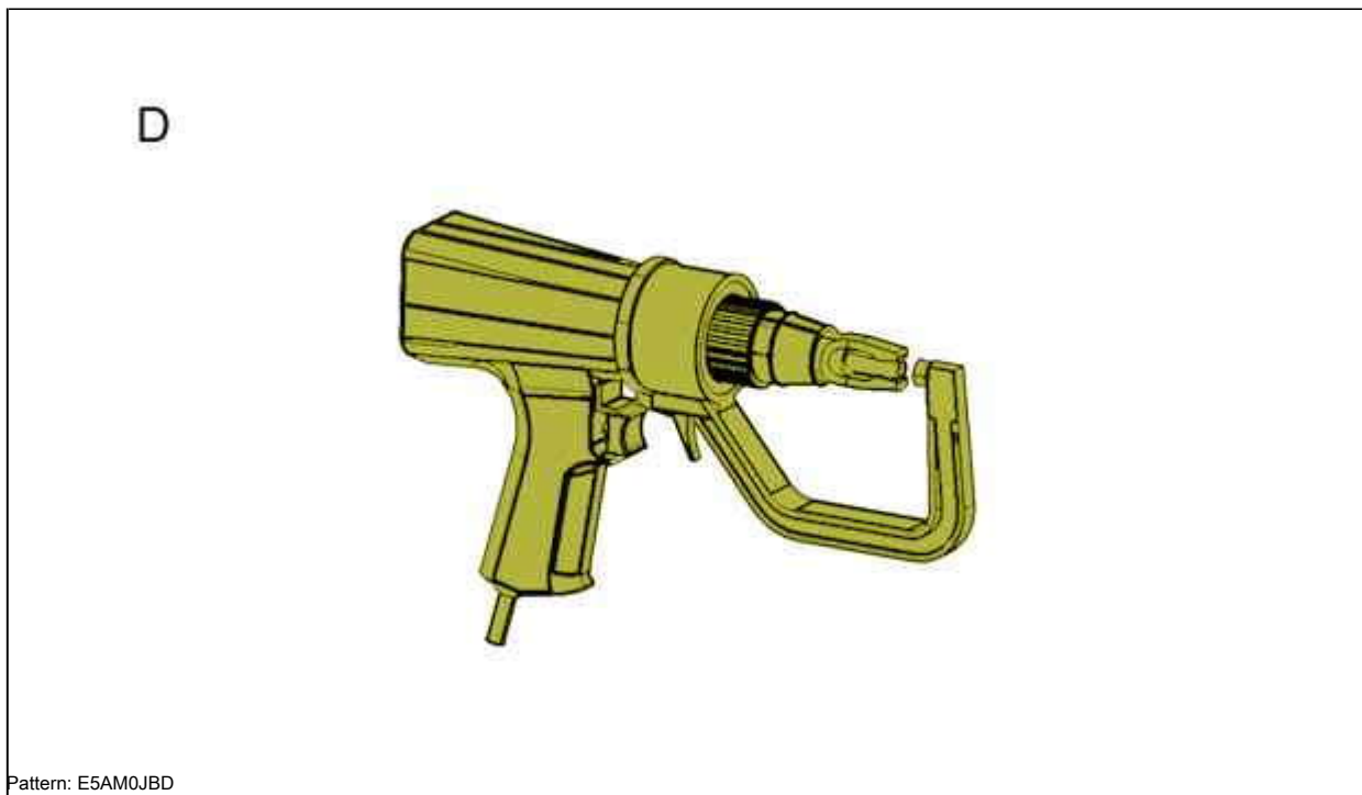
"D" S-shaped drill for drilling weld spots.
