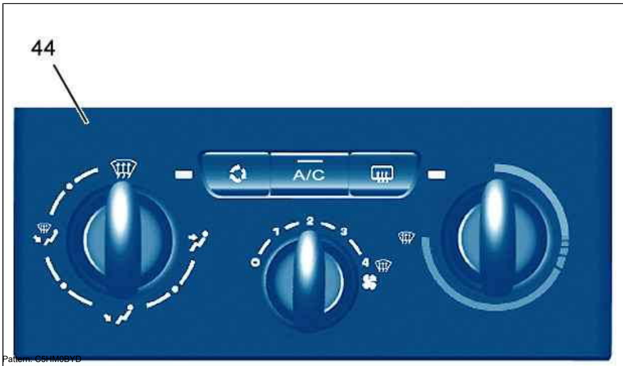
(44) Front panel of the basic air conditioner. Simple air conditioning system:
