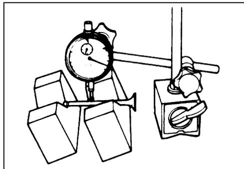
**DESCENTRAMIENTO RADIAL DE CABEZAS DE VÁLVULAS**
