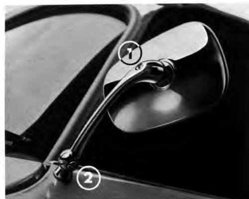
Fig. 9 - Outside rear-view mirror 1-2 - Adjusting screws
