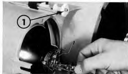
Fig. 46 - Long-range headlamps (small \varnothing ) directional 1 - Vertical adjuster
