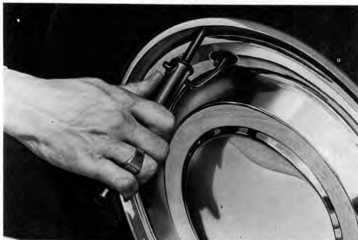
Fig. 33 - Removing a large wheel embellisher
