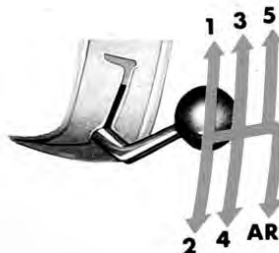
Fig. 14 - L.H.D. 5-speed diagram on manual gear-change version AR - Reverse gear
