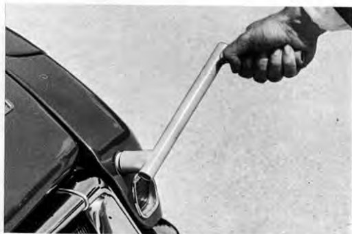
Fig. 32 - Removal of a rear wing
