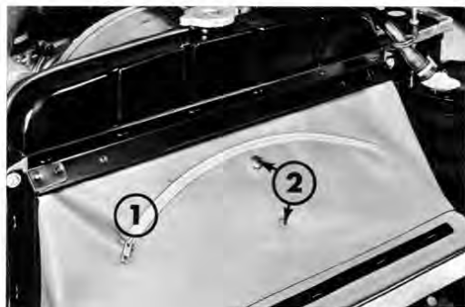
Fig. 29 - Cleaning the radiator
