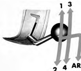
Fig. 14 a - L.H.D. 4-speed diagram on manual gear-change version AR - Reverse gear
