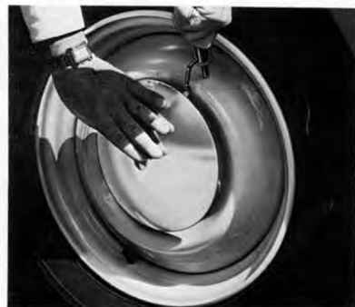
Fig. 33 a - Removing a small wheel embellisher
