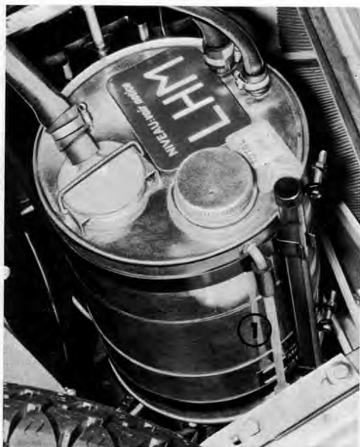
Fig. 26 - Hydraulic reservoir 1 - Level checking sight-tube
