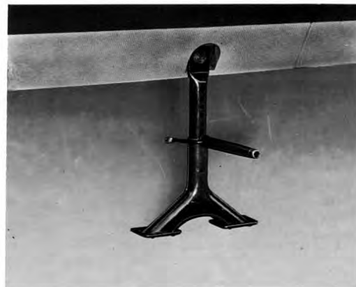
Fig. 34 - Positioning the jacking stay
