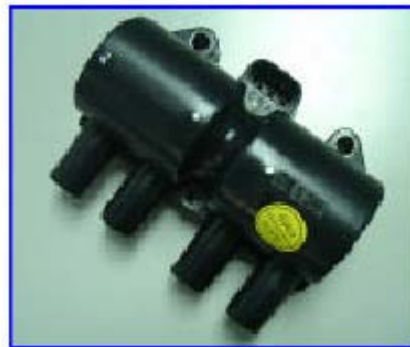
Profile of ignition coil
