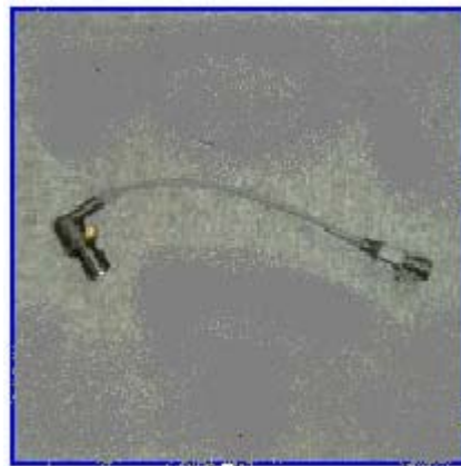
Profile of a crankshaft position sensor
