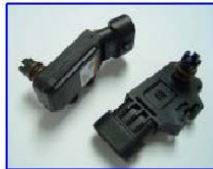
Absolute pressure/intake temperature sensor for intake manifold
