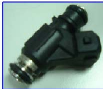
Profile of a electromagnetic injector
