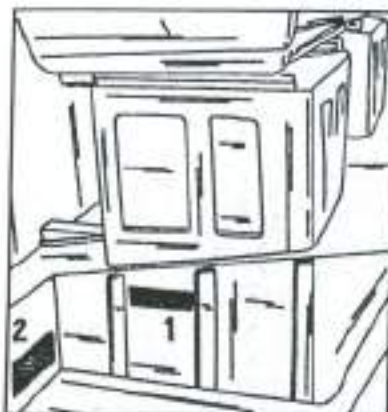
Fig. 0.2 - With the door open you will see a type plate (1) with details of the body and paint identification codes.
