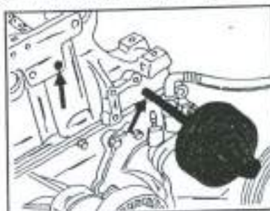
Fig. 1.68 - Remove the two bearing bolts in the manner shown out of the cylinder block.
