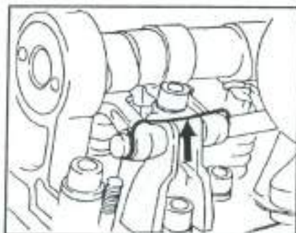
Fig. 9.20 - The arrow shows where the wire clip is fitted to the rocker arm pedestal.
