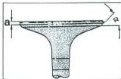
Fig. 9.12 - The valve head edge must be measured before a valve is refitted. The minimum permissible dimension is 1.5 mm.
