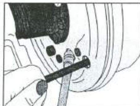
Fig. 7.6 - Checking the clearance between the brake shoe lining and the brake drum surface.
