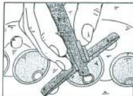
Fig. 9.8 - Measuring the distance between the cylinder head surface and the end of the fitted valve guide.
