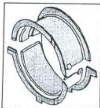
Fig. 1.52 - Fitting the main bearing cap together with the thrust washer.
