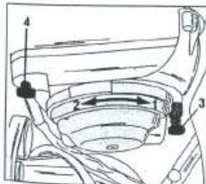
Fig. 8.5 - View of a headlamp unit from the rear. Remove the plastic cover in direction (1) and refit it in direction (2).
