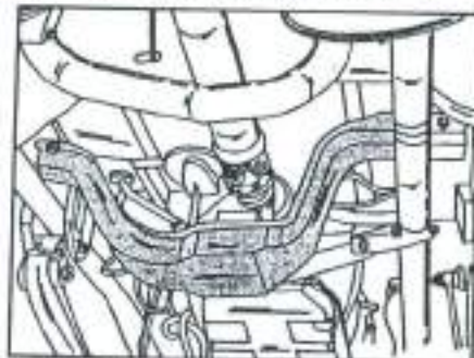
Fig. 1.5 - The attachment of the crossmember underneath the vehicle.
