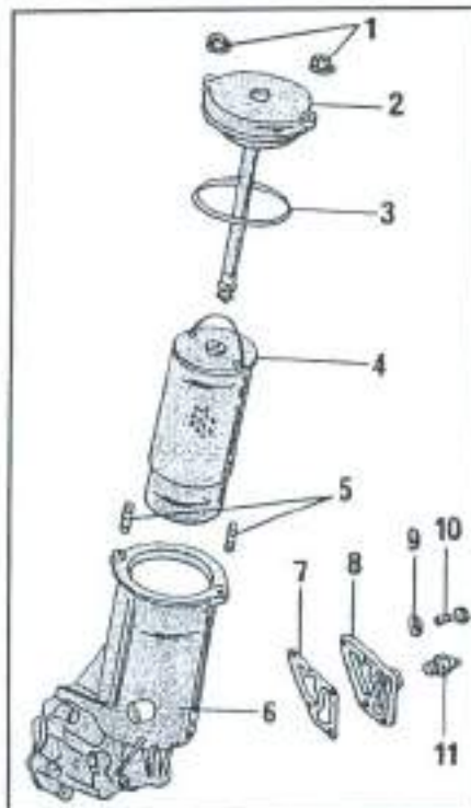
Fig. 9.30 – The component parts of an oil filter with combined filter element.
