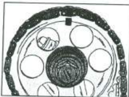
Fig. 9.2 - Mark the camshaft timing gear and the timing chain with a spot of paint before separation of the parts.
