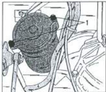
Fig. 1.80 - The two nuts (1) secure the cover at the upper end of the oil filter housing. The filter element will appear after removal of the cover.
