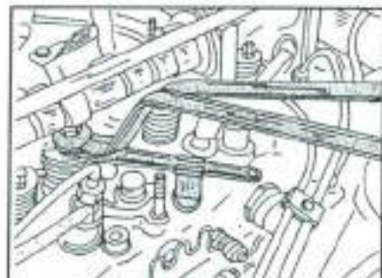
Fig. 9.15 - Using the two special wrenches to adjust the valve clearances.
