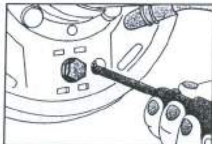
Fig. 7.19 – Measuring the gap between the brake shoe lining and the drum surface. The check must be carried out on each brake shoe.
