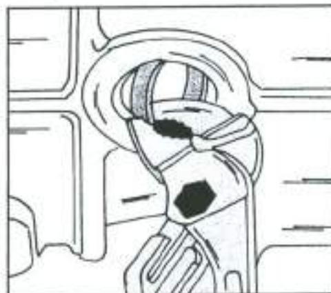
Fig. 1.45 - Removal of a welsh plug.
