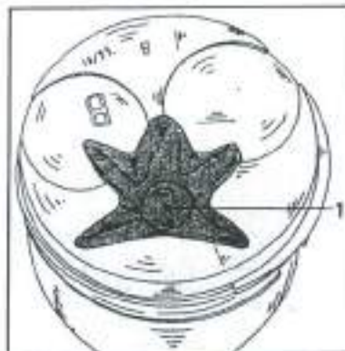
Fig. 1.28 - View of the piston, showing the combustion chamber with (1). The two recesses for the valves prevent contact between the valve heads and the piston crown.
