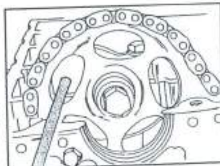
Fig. 1.71 - Counterholding the camshaft sprocket against rotation.
