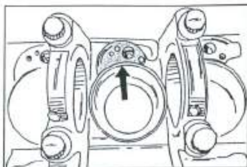
Fig. 1.46 - The arrow shows the oil splash jet (engine with EGR system).
