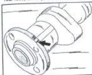
Fig. 1.70 - Camshafts are marked with a number at the position shown by the arrow.
