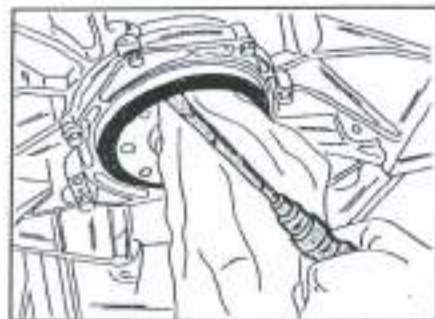
Fig. 1.59 - Removal of the rear crankshaft oil seal. Place a rag underneath the screwdriver to prevent damage.
