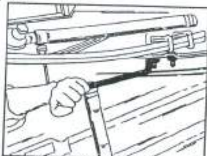
Fig. 4.3 - Removal or tightening of the spring "U" bolt nuts. When tightening use a ring spanner before applying a torque wrench and socket.
