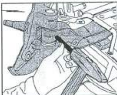
Fig. 4.6 - Drive out the pin to remove the steering knuckle from the axle beam.
