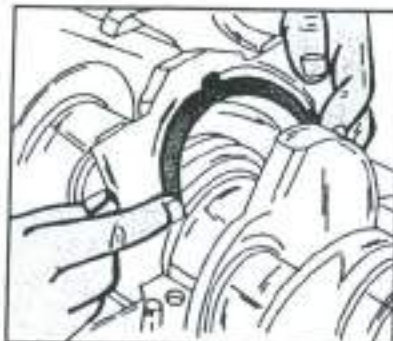
Fig. 1.52 - Fitting the main bearing cap together with the thrust washer.
