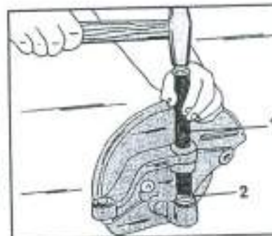
Fig. 4.9 - Fitting the king pin bush. A spacer washer (2) must be placed in position to drive the bush to the correct depth with a suitable mandrel.
