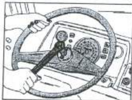
Fig. 6.10 - Removal of the steering wheel.
