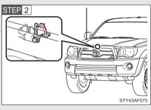
Pull up the hood catch lever and lift the hood.
