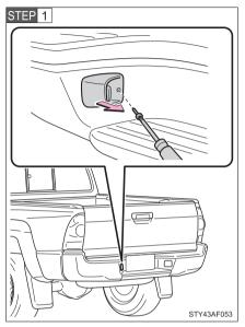
Remove the screw and light unit.
