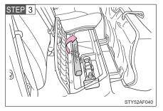
Unhook the strap and remove the tool bag.
