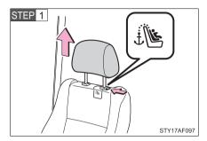
Remove the head restraint.
