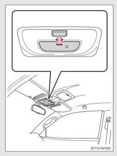
To turn the compass on or off, press the switch.
