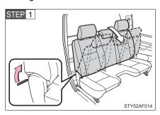
Pull the lever and fold down the seatback.
