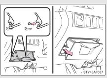
2.Pull up the box and disengage the claws. Remove the stoppers from the cutouts and remove the box. STEP 3 After a system failure, see "Fuse layout and amperage ratings" (→P. 411) for details about which fuse to check.
