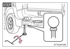
Raise the vehicle until the tire is slightly raised off the ground.
