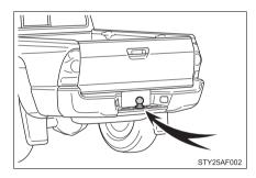
The rear bumper of your vehicle is equipped with a hole to install a trailer ball. If you have any questions, contact your Toyota dealer.
