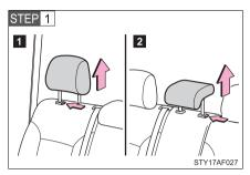
Remove the head restraint.
