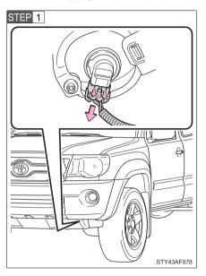
Unplug the connector while pulling the lock release.
