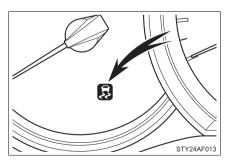
If four wheels spin, the slip indicator flashes to indicate that the active traction control system has been engaged.
