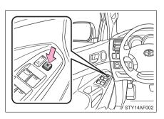
Press the switch down to lock passenger window switches.
