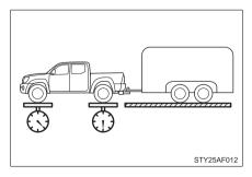
The maximum allowable gross axle weight. The gross axle weight is the load placed on each axle (front and rear).
