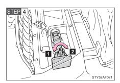
Loosen and remove the jack.
