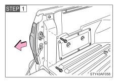
Remove the bolts and rear combination assembly.
