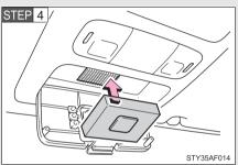
Place the transmitter with fastener square facing inside of box into the box.
