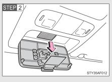
Remove the hook-and-loop fastener square.
