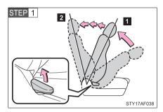
Fold down the front seat seatback and back to the 1st lock position (most upright position) until it locks into place. Adjust the seatback to the 10th lock position.
