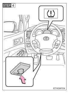
Press and hold the tire pressure warning reset switch until the tire pressure warning light blinks slowly 3 times.
