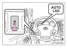
Quickly push and release the VSC OFF switch to turn off TRAC.
