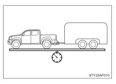
The maximum allowable gross combination weight. The gross combination weight is the sum of the total vehicle weight (including the occupants, cargo and any optional equipment installed on the vehicle) and the weight of the trailer being towed (including the cargo in the trailer).
