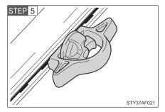
Check the tie-down cleat to confirm that it is locked into a detent and securely mounted to the deck rail system.
