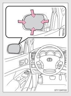
Adjust the mirror up, down, in or out by pushing the mirror surface.
