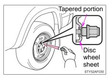
Tighten the nuts until the tapered portion comes into loose contact with the disc wheel sheet.
