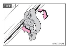
Insert the locking plate into the deck rail, rotate the tie-down cleat 90°, and release the thumb wheel.
