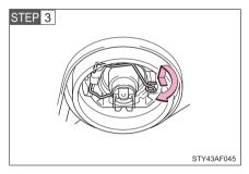
Release the bulb retaining spring.
