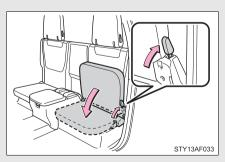
Push the bottom cushion down while pulling the lever until the bottom cushion locks into the seat position.
