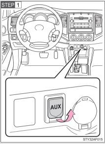
Connect the portable audio device.
