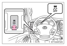
Press and hold the VSC OFF switch for more than 3 seconds while the vehicle is stopped to turn off both TRAC and VSC.
