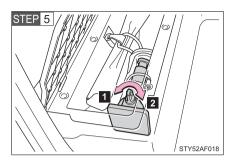
Loosen and remove the jack.
