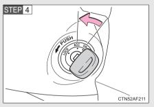
Stop the engine by turning the engine switch to the ACC position.
