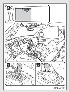
The rear view image is displayed on the inside rear view mirror when the shift lever is in the R.
