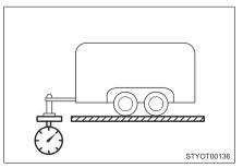
The load placed on the trailer hitch ball. ( $\rightarrow$ P. 221)
