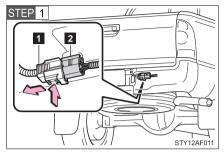
To disconnect the wire harness connectors (1 and 2), press and hold the lock of the tailgate wire harness connector (White) and pull apart.
