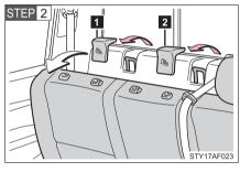
Swing the seatback forward slightly (→P. 46) and remove the anchor bracket covers.
