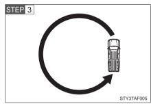
Drive the vehicle at 5 mph (8 km/h) or less in a circle until the direction is displayed.
