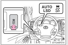
Press the VSC OFF switch to turn on the system.
