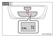
Press the switch until CAL appears on the display.
