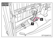
Loosen and remove the jack.
