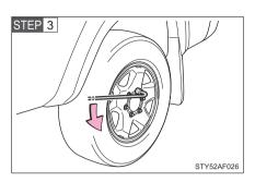
Slightly loosen the wheel nuts (one turn).
