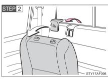
Swing the seatback forward slightly (→P. 46) and remove the anchor bracket cover.
