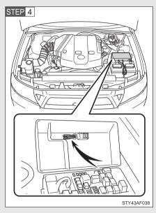
Remove the fuse with the pullout tool.
