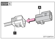
Attach the connector cover (Gray) to the tailgate wire harness connector (White).
