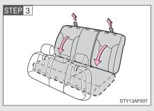
Fold down the seatback by pulling the lock release strap.
