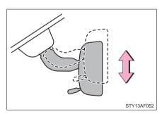
Adjust the height of the rear view mirror by moving it up and down.
