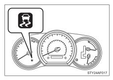
If the vehicle is in danger of slipping, the rear wheels (2WD models) or four wheels (4WD models) spin, the vehicle starts to roll backwards when starting an incline. this indicator on flashes to indicate that the VSC/ TRAC/hill-start assist control systems have been engaged.
