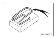
This clip must be removed prior to adhesion of the fastener.
