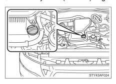
If the oil level is below or near the low level mark, add engine oil of the same type as already in the engine.
