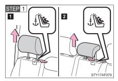
Remove the head restraint.
