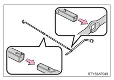
Assemble the jack handle extension as shown. Be sure to tighten each screw securely.
