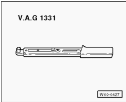
Fig. 159: Identifying Torque Wrench V.A.G. 1331 Courtesy of VOLKSWAGEN UNITED STATES, INC.
