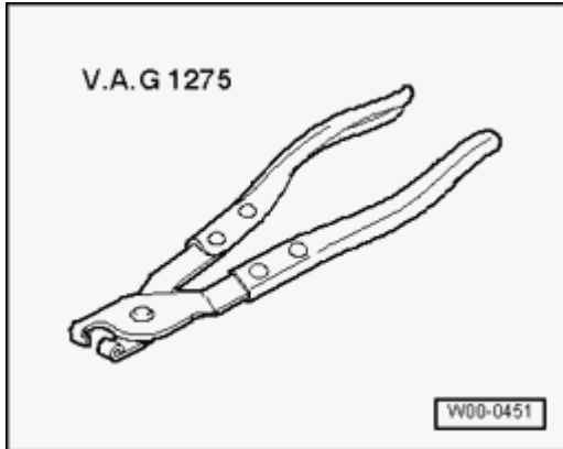
Fig. 524: Identifying Hose Clamp Pliers V.A.G 1275 Courtesy of VOLKSWAGEN UNITED STATES, INC.
