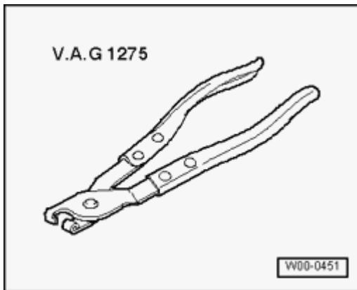
Fig. 406: Identifying Hose Clamp Pliers V.A.G 1275 Courtesy of VOLKSWAGEN UNITED STATES, INC.
