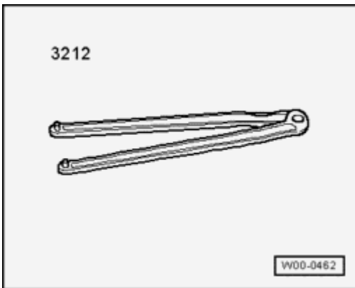
Fig. 570: Identifying Special Tool - Panner Wrench 3212 Courtesy of VOLKSWAGEN UNITED STATES, INC.
