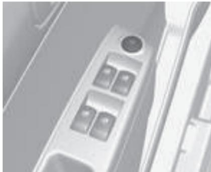
Pulse el interruptor
