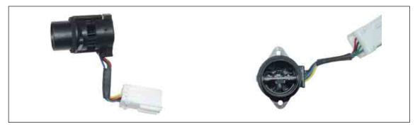
The AIH sensor is installed on the air conditioner controller unit. It is a sensor that detects interior temperature and humidity.
