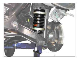
Unscrew the lower shock absorber bolt on coil spring link and the bolt/nut on sub frame of the coil spring link and knuckle to remove the coil spring link assembly.
