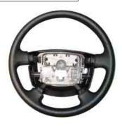
Put an installation mark on the steering wheel, column shaft and nut when removing the steering wheel. Place the steering wheel to the straight forward direction.
