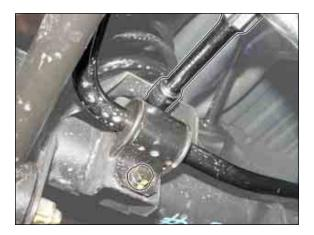
4. Remove the shock absorber between the frame and the axle.
