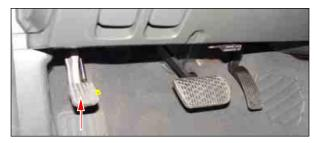
**Foot Operated Type** (Automatic Transmission Equipped Vehicle)
