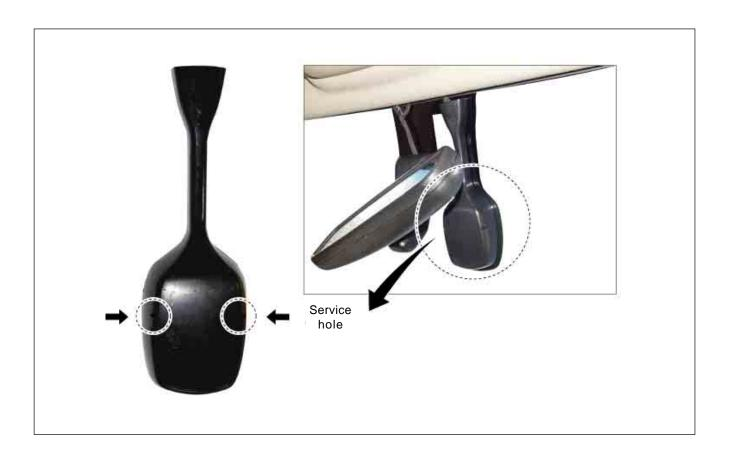
2. Disconnect the connector from the rain sensor unit located at the front windshield glass and then lift up the rain sensor unit to disconnect from the glass.
