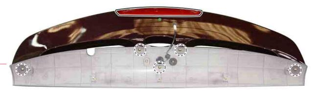
5. Replace the tailgate upper garnish assembly with new one.
