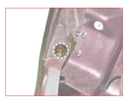
8. Unscrew the bolts and screws from the fender wheelhouse.
