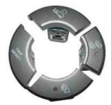
2) Remove the hazard switch mounting bracket and remove the hazard switch.
