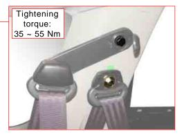
2. Unscrew the lower anchor bolt of the rear seat belt.
