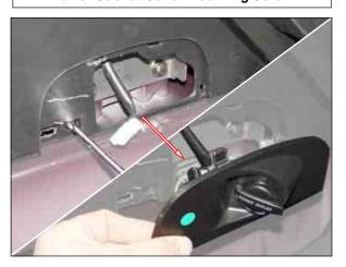
4. Unscrew two screws and remove the lower center air duct.
