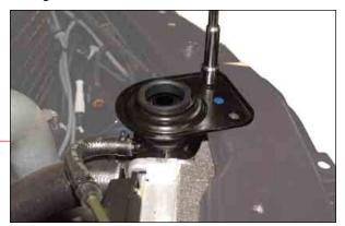
10. Unscrew three mounting bolts (10 mm) and then remove the front end panel.
