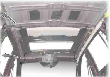
2. Unscrew the two bracket mounting bolts (10 mm) at both sides.
