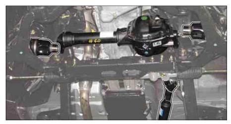
2. Removal of mounting bolt Unscrew the mounting nut (22 mm) at right side and remove the axle mounting bolt.
