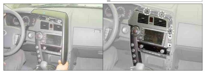
2. Remove four instrument panel mounting screws.
