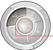
When you see a steep downhill ahead, press the HDC switch and the green HDC indicator comes on. When the G sensor within the sensor cluster detects a slope level exceeding 10%, the ESP's HDC function operates. When this occurs, the green HDC indicator flashes along with a loud operation sound.
