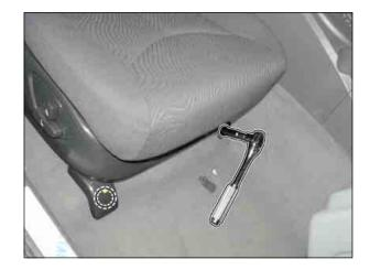
2. Move the seat forward as far as possible and unscrew the two rear mounting bolts (14 mm) at both sides.
