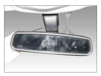
2. Disconnect the harness connector and remove the inside rearview mirror.
