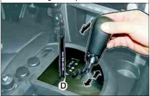
\* When the gear selector lever cannot be moved from "P" position to other positions, manually release the lock-up function as shown in figure.
