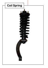
A section of spring steel rod is wound in a spiral pattern or shape coil provides a cushion to absorb road imperfections and returns the vehicle to a predetermined ride height. It is amajor contributor to a vehicle's handling balance and ride quality. Higher spring rates and shorter overall lengths are commonly used to lower the vehicle's ride height for enhanced appearance and improved handling.
