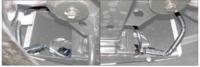
2. Remove the RH/LH sensor mounting cover and spring and then remove the sensor from the bumper.
