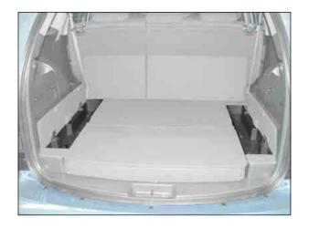
2. Unscrew the mounting bolts and remove the third row seat.
