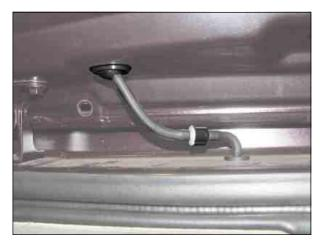
2. Close the tailgate and then remove the nozzle with a flat blade screwdriver or special tool.
