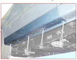
3. Carefully remove the side molding seal.
