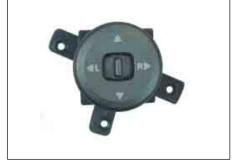
The outside rearview mirrors can be folded and unfolded within  $30 \pm 6$  seconds even after turning off the ignition switch. To prevent the outside rearview mirrors from stopping during its operation, the mirror operating time is extended 13 seconds when pressing the switch again.
