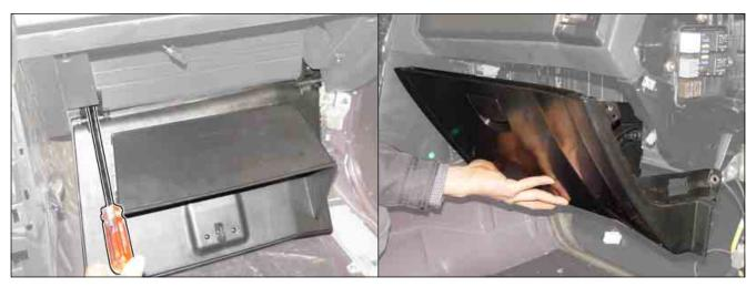
4. Open the DVD changer cover. Unscrew the mounting screws and remove the inner cover and outer cover.
