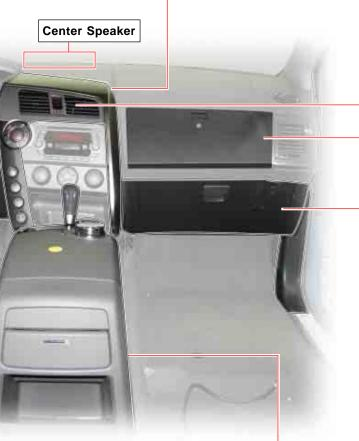
8) Remove the center console assembly and the center fascia lower tray.
