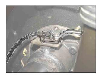
3. Unscrew the adjusting nut of the parking brake cable equalizer to loosen the parking brake cable.
