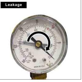
If the vacuum pressure is not maintained, replace the actuator with a new one.
