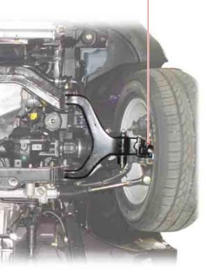
4. Place a safety jack under the lower arm and unscrew the lower shock absorber yoke bolt. Remove the yoke while raising the safety jack with lower arm.
