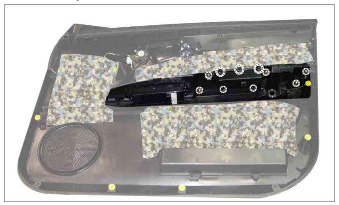
3. Remove the inner door handle and the memory seat switch assembly.
