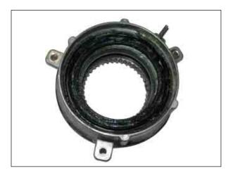
2. Replace the O-ring of the locking hub end with a new one.
