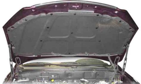
3. Slacken the mounting bolts on the hood hinge (Do not remove the bolts.)
