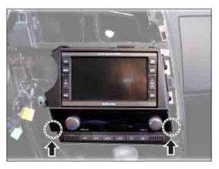
2. Disconnect the connectors from the A/C controller switch assembly.
