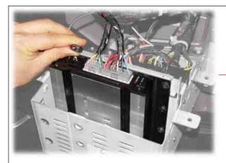
Check if the fiber optic cable is defective. If the red lamp comes on when the ignition switch is in "ON" position, the system receives the normal input signal.
