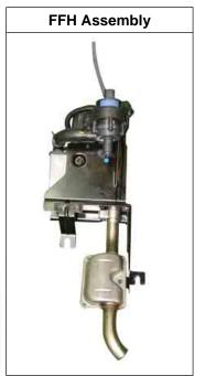
2) Unscrew the mounting nuts from the FFH coolant circulation pump.
