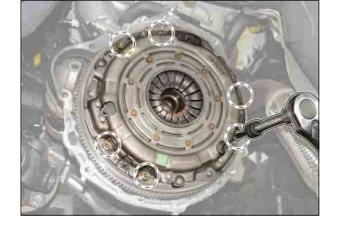
4. Unscrew the bolts and remove the clutch cover, pressure plate and clutch disc.
