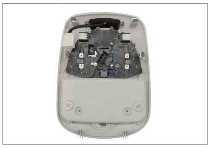
4. Unscrew three mounting screws and remove the sunroof switch.
