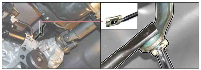
4. Unscrew the bolt and remove the link from the shift lever.
