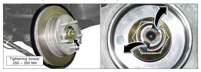
2. Make an alignment mark on the flanges of the axle shaft and the axle housing. Unscrew the six bolts (Torx 10 mm) and remove the axle shaft while lowering the axle shaft flange.
