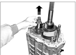
11. Remove the 5th gear retainer ring with a ring pliers.
