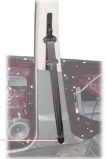
3. Remove the B pillar (lower) and disconnect the pretensioner connector.
