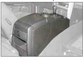
5) Unscrew three mounting screws and remove the left side panel from the center fascia panel and AV head unit.
