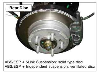
Rear Disc and Caliper (1 Internal Cylinder)
