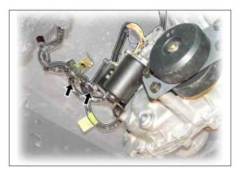
6. Support the underbody of transmission with a hydraulic jack not to deflect it and unscrew the bolts (14 mm - 4EA) and cross nuts (14 mm - 2EA) and remove the cross member.
