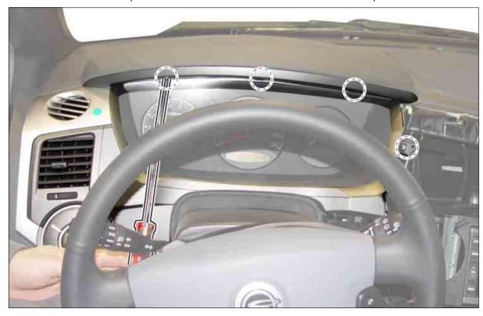
2. Disconnect the connector from the outside rearview mirror switch bezel assembly and remove the meter cluster fascia panel.
