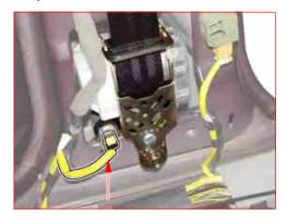
4. Unscrew the seat belt upper mounting bolt from the height adjuster.
