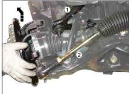
4. Remove the axle shaft.
