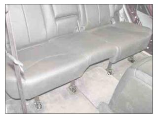
2. Lay down the seatback of the second row seat and remove the eight rear mounting nuts (14 mm). Insert a wrench between seatback and cushion to remove the mounting bolts with arrow mark.
