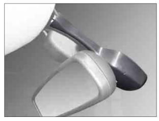
A sensor that emits infrared rays through LED and then detects the amount of rain drops by receiving reflected rays against sensing section (rain sensor mounting section on the windshield) with photodiode. The auto light sensor is Integrated into the rain sensor. (refer to the below picture)
