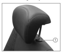
To raise the headrest, pull it up without pressing the release button. To lower the headrest, press the release button (1) on top of seatback and push the headrest down.
