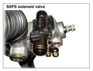
2. When the vehicle speed is at 0 km/h, check whether the electric current for solenoid is in specified range and check that the current is reduced as the vehicle speed increases.
