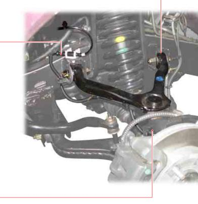
: Remove the split pin first and then remove the mounting nut.
