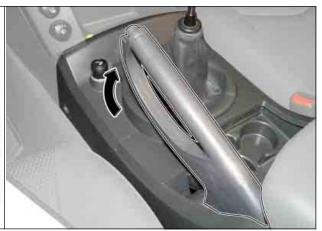
8. Disconnect the cigarette lighter connector and remove the center console assembly.
