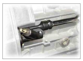
3. Unscrew three bolts and remove the concentric slave cylinder assembly on the input shaft of cylinder.
