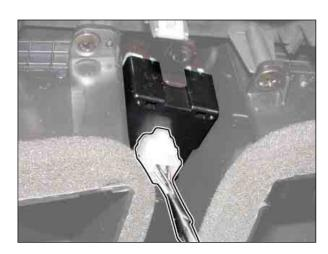
3. Unscrew three mounting screws and remove the digital clock from the center fascia panel.
