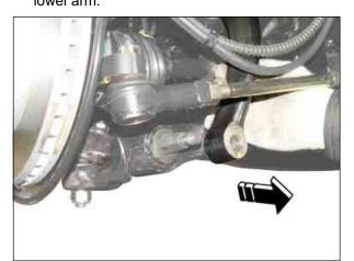
5. Remove the lower arm assembly from the vehicle.
