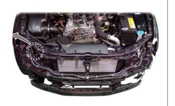
2. Unscrew the mounting nuts on the receiver dryer and remove the high/low pressure pipes.
