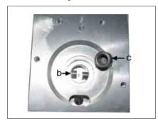
The cam bushing (c) is installed between plungers (b) and it draws and discharges the brake fluid.
