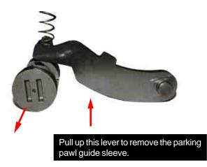
7. Replace the O-rings of the parking pawl guide sleeve and bushing.
