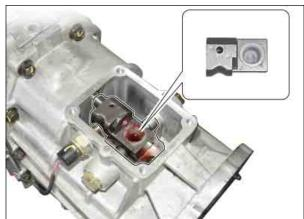
60. Apply the grease to the interlock bolt (17 mm) and insert it into the interlock plate hole and bolt hole.
