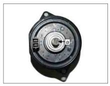
The motor is operated when ABS is activated. The cam-shaped output shaft of the motor (a) enables the brake system to receive and supply the brake fluid during the motor operation.
