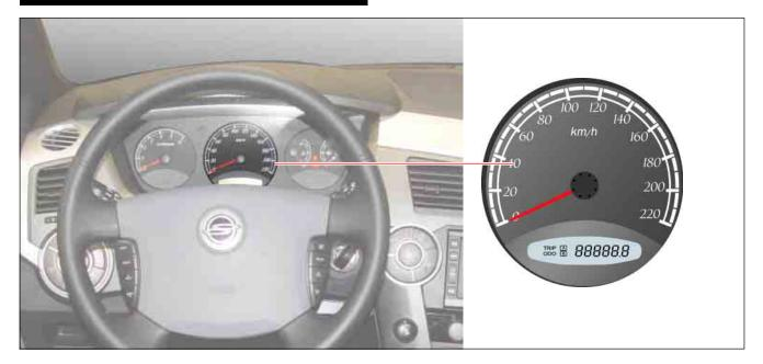
The speedometer indicates the vehicle speed by calculating the signals from the rear (right 8 LEFT) wheel speed sensor through ABS or ESP unit. In this model, the wheel speed sensor is installed at the rear tire area even though the ABS/ESP is not equipped. Its signal is used as a standard vehicle speed that is transmitted to instrument panel, TCU, TCCU, and engine ECU via CAN communication.
