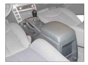
1. Unscrew two bolts (12 mm) and remove the change lever from shift lever.
