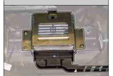
Detects A/C switch position, coolant temperature, engine condition and driving condition to control the air conditioner.
