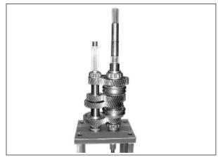
25. Place the output shaft assembly with the 1st gear facing down and remove the intermediate taper roller bearing with a special tool.
