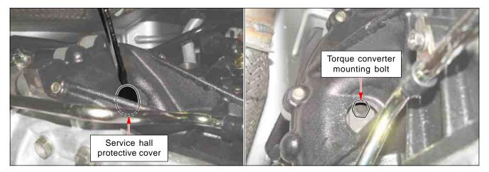
4. Unscrew the transmission mounting bolts and carefully remove the transmission with a transmission jack.
