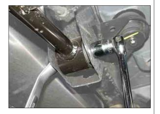
3) Unscrew lower arm mounting bolt/nut (22 mm) on axle.
