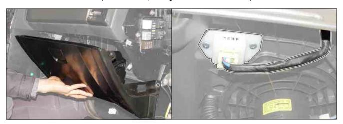
2. Unscrew the mounting screws and remove the power transistor.
