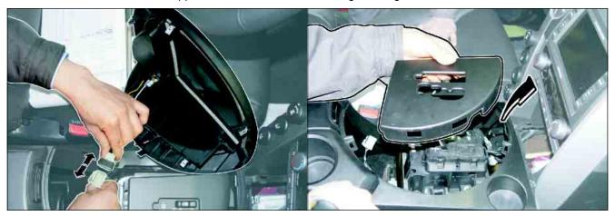
3. Separate the selector lever pin with a flat blade screwdriver.
