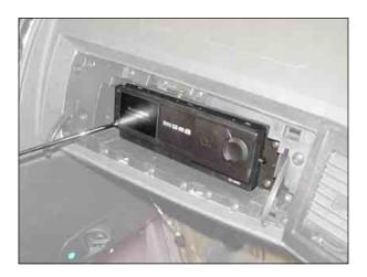
7. Disconnect the fiber optic cable from the DVD changer through the opening of lower instrument panel.
