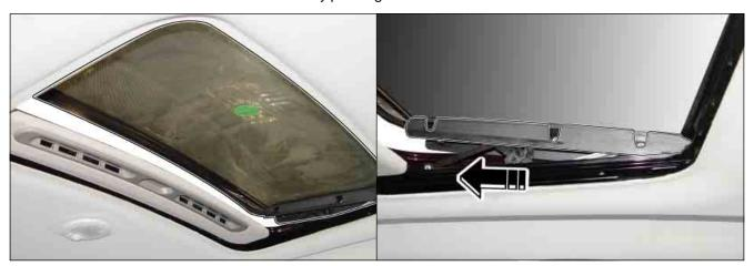
2. Remove the three mounting bolts (TORX bolts) of the glass panel with a special wrench (25 T).
