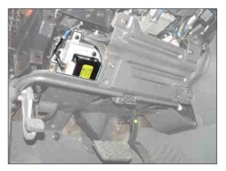
1. Disconnect the connectors from STICS unit and remove the RKSTICS antenna.
