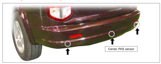
1. Disconnect the harness connector and then remove the center sensor by turning the mounting cover.
