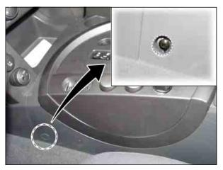
6. Remove the storage box cover and disconnect two mounting bolts (10 mm) in center console.
