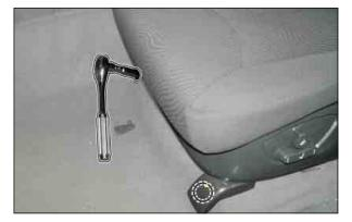
2. Move the seat forward as far as possible and unscrew the two rear mounting bolts (14 mm) at both sides.
