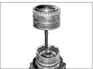
3. Remove the clutch C1 from converter housing assembly.
