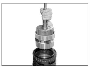
2. Remove the clutch C2 from converter housing assembly.
