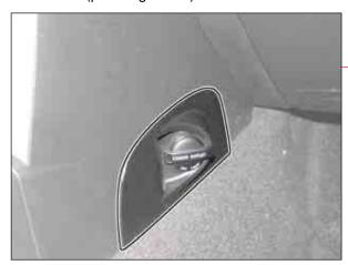
2. Disconnect the power outlet connector.
