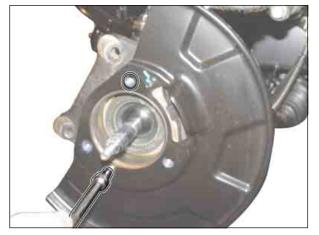
2. Pull out the upper arm lock pin and unscrew the mounting nut (19 mm). At this time, do not fully remove the nut.
