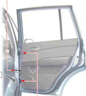
Disconnect the Door Wiring Harness.
