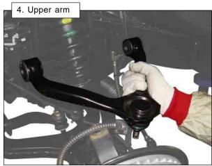
: Separate the upper arm from the frame first, and then separate it from the knuckle with a special tool.
