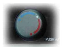
When pressing the air conditioner AUTO mode and temperature control dial switch, the system operates in AUTO mode and can set the desired temperature (18  $\sim$  32°C) by rotating. To get the desired temperature, the air conditioner controls compressor, door mode, air source door, air mix door and blower motor automatically.
