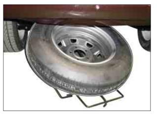
4. The spare tire carrier can be removed by pulling out the lock pin (arrow).
