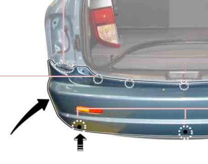
3. Unscrew the mounting screws from the wheelhouse.
