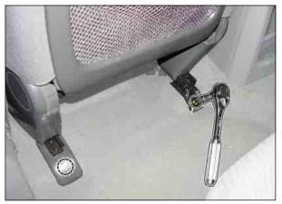
3. Pull up the seat and disconnect the harness connector. Remove the seat assembly.
