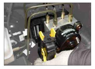
3. Disconnect the primary and secondary master cylinder pipes from HECU.
