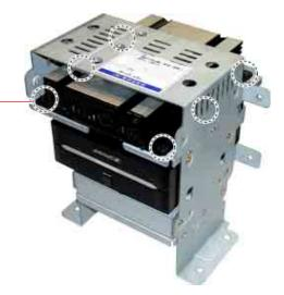
Unscrew six mounting bolts (10 mm) from the amplifier.
