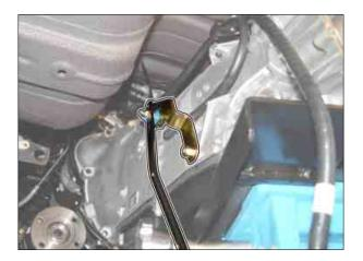
5. Disconnect the selector lever connector, unscrew the mounting bolts (three hexagon bolts), and remove the selector lever assembly.
