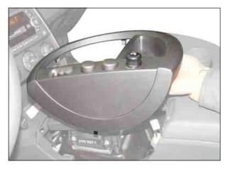
3. Remove the gear selector lever cover and storage box.
