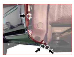
7. Unscrew the mounting bolt on the fender near the headlamp.
