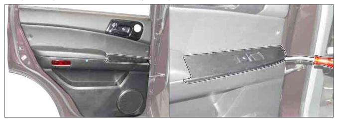
2. Disconnect the switch connector and remove the switch assembly.
