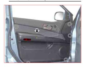
3. Separate the bottom of door trim and pull it up to remove.
