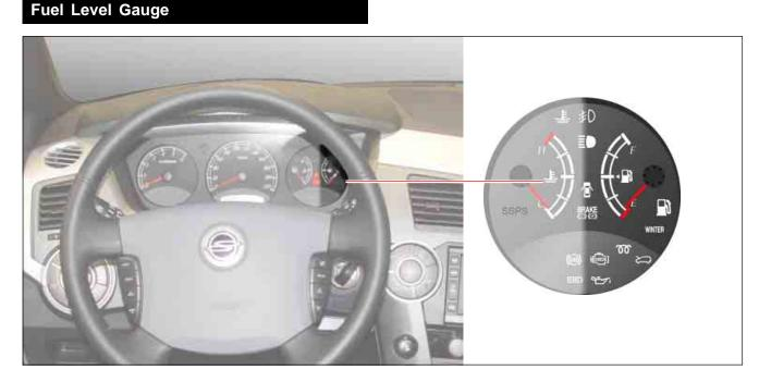
The fuel level gauge displays the resistance value of the float on the fuel sender in the fuel tank through a pointer. Note that this vehicle doesn't have a service hole for checking the fuel sender connector in the fuel tank.
