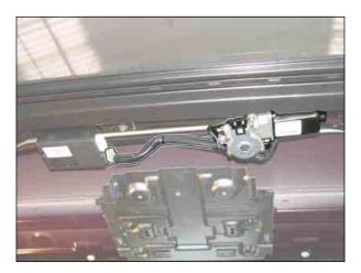
2. Unscrew the three mounting bolts (25T) with a special wrench and remove the motor assembly.
