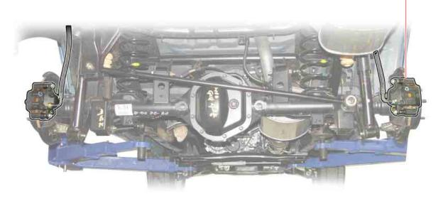
2. Unscrew the mounting bolt (10 mm) and disconnect the wheel speed sensor cable.
