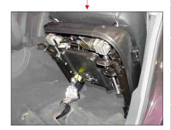
4. Unscrew the screws (arrows) and remove the protective cover.
