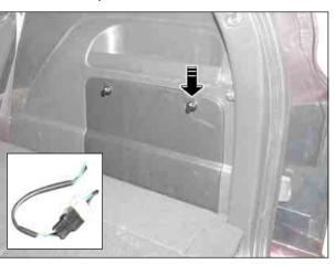
2. Unscrew eight screws and remove the power outlet mounting bracket.
