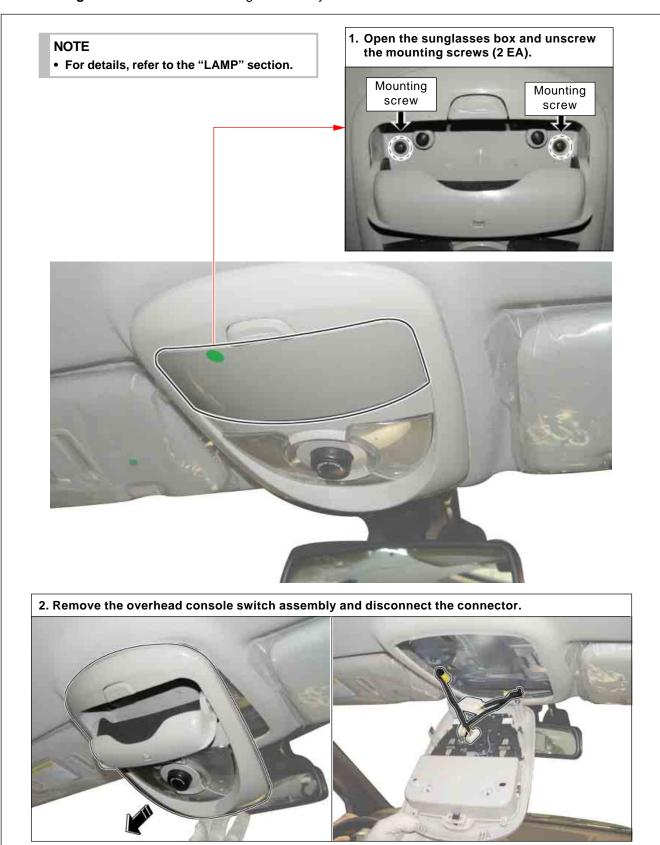
3. Remove the front room lamp switch from the removed overhead console switch assembly.
