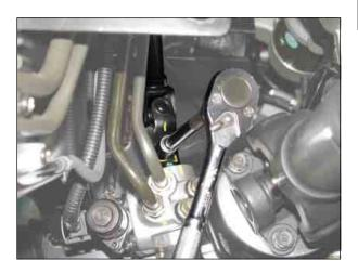
4. Disconnect the power steering pipes and remove the steering gearbox mounting bolts.
