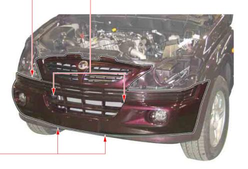
3. Unscrew the lower mounting bolts (10 mm).
