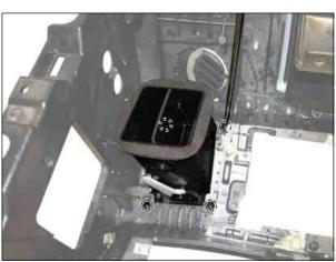
2. Pull the vent grille out of instrument panel.
