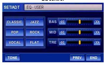
Adjusting the sound according to the music genre Press "EQ SETTING" button in "SET/ADJ" screen and adjust the sound.
