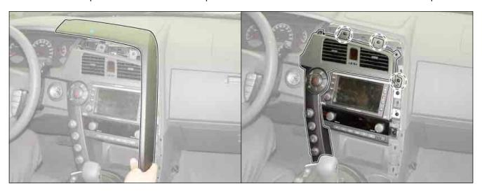
2. Disconnect the switch connectors and remove the center fascia panel assembly.
