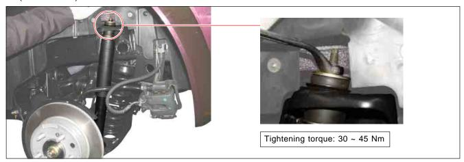
2. Unscrew the shock absorber lower bolt/nut (bolt: 14 mm / nut: 17 mm) on coil spring link.
