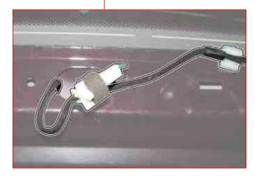
2. Remove the upper trim and disconnect the high mounted stop lamp.
