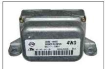
Sensor cluster: (Yaw rate + lateral sensor + longitudinal sensor)
