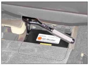
4. Disconnect the TCU connect and remove the TCU.
