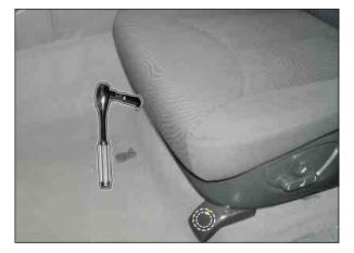
2. Slide the seat to the front stop and remove the seat rear mounting bolts (LH/RH: 14 mm - 1EA).
