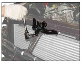
8. Unscrew the mounting bolt (10 mm) and remove the front support panel.
