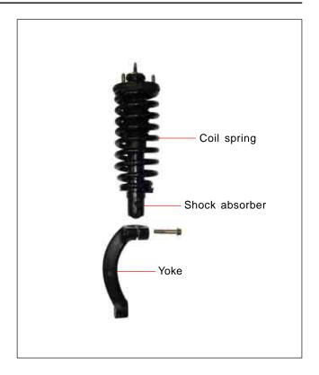
2. The telescopic shock absorber consists of a tube with piston and rod, and a cylinder tube. The piston has an orifice and valve and the cylinder is filled with oil.
