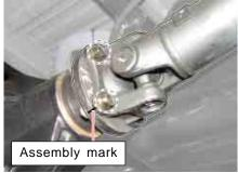
Tightening torque 70 ~ 80 Nm
