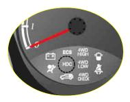
When pressing the HDC switch, the green HDC indicator on the instrument panel comes on, and when the HDC operates, the green HDC indictor blinks with 0.5 seconds of interval.
