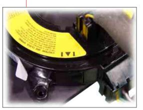
Align the alignment marks when installing
