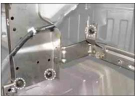
7) Unscrew the mounting bolts (A, B) from the passenger side instrument panel frame and air conditioner module.
