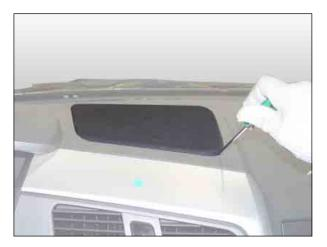
2. Unscrew the mounting screws and disconnect the harness connector to remove the center speaker.
