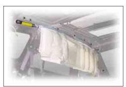
The curtain air bags are installed at the bottom of the roof trim and they enhance the passenger's safety. The driver's and passenger's curtain air bags individually deploy.
