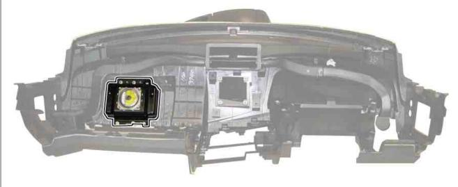
2. Unscrew five nuts on the air bag module (10 mm).
