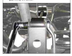
Tightening torque 150 ~ 180 Nm B. Unscrew upper arm mounting bolt/nut (22 mm) on frame.
