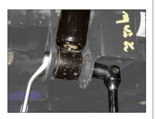
5. Remove the upper arm between frame and the axle.
