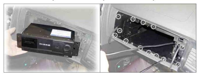
9. Disconnect the harness connector and pull out the DVD changer with case.
