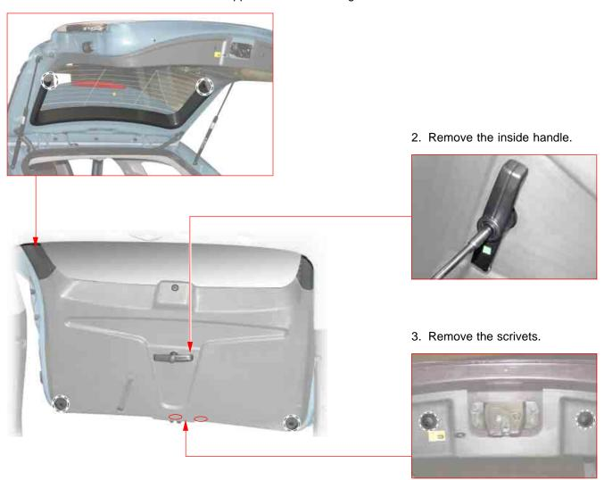
4. Remove the fasteners and then remove the lower trim.
