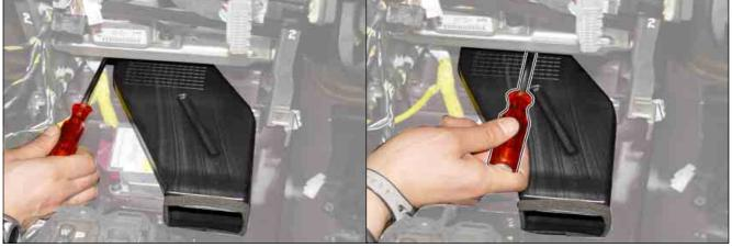
5. Disconnect the connector and remove the air bag unit.
