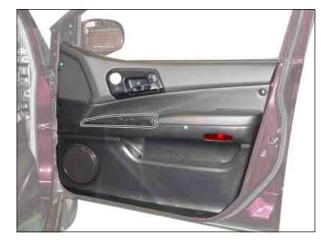
2. Unscrew the mounting screws and remove the inner door handle and the memory seat switch assembly from the passenger's door trim.
