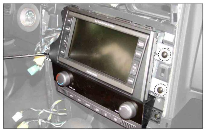
2. Disconnect the head unit harness connector and the fiber optic cable.
