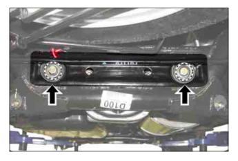
4. Unscrew the mounting bolt (30 mm) and carefully lower the safety jack with axle housing assembly.
