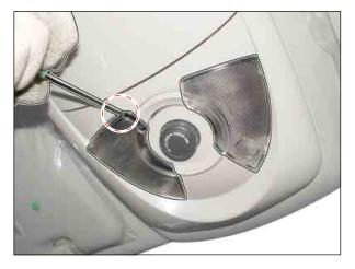
2. Carefully remove the bulb from the lamp and replace it with new one.
