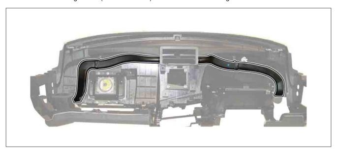
3. Unscrew the mounting screws (one at each side) and remove the upper air duct.
