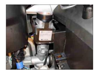
3. Remove the connector from the key switch and disconnect the immobilizer unit.
