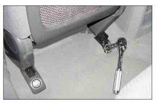
3. Lay down the seatback and disconnect the connector under the seat and then remove the seat assembly.
