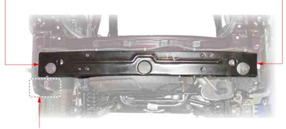
A. Disconnect the rear main wiring (parking aid sensor) connector.
