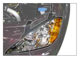
2. Remove the headlamp lower cover from the upper front bumper and unscrew the headlamp lower mounting nut (10 mm).
