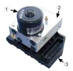
This section is provided only for the understanding of HECU. Note that this component cannot be disassembled for repair and maintenance. HECU consists of motor pump, valve body, solenoid valve and ECU.
