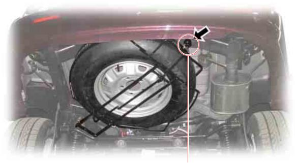
1. Remove the butterfly nut from the spare tire carrier and loosen the lock bolt until the hook is released.
