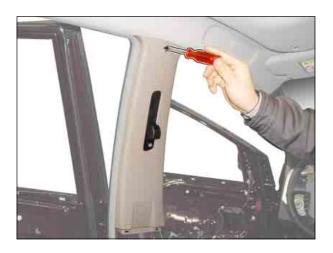
7. Unscrew the mounting bolts and remove the height adjuster.
