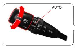
These senses the ambient illumination intensity to determine the timing for turning the headlamps and tail lamps on or off automatically when the light switch is set to "AUTO".
