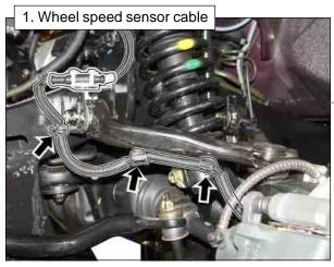
: Remove the wheel speed sensor cable and the connector from the upper arm.
