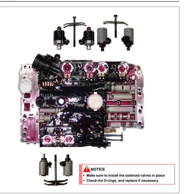
5-3. Remove the electronic control module from the shift plate.
