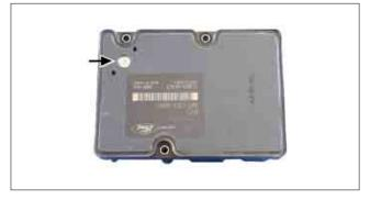
The electrical components are weak to moisture. To protect ECU, Gore Tex-based plate is used at ECU lower cover. The vent hall (arrow) allows air to ventilate but does not allow moisture to penetrate.
