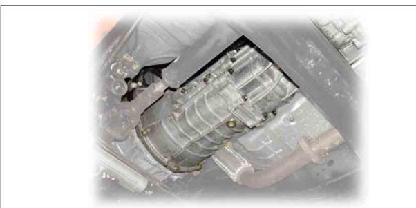
Insert the centering pin (special tool) into center spline.
