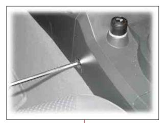
6. Remove the storage box cover and unscrew the mounting bolts in center console.
