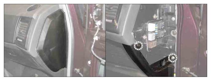
3. Unscrew the inner and outer mounting screws from the glove box and remove the lower instrument panel.
