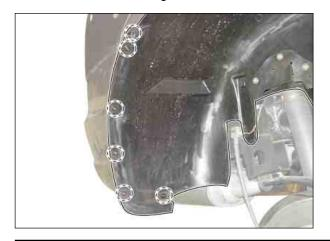
4. Unscrew the lower mounting screws from the bumper.
