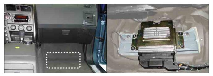
2. Disconnect the SSPS control unit connector and separate the SSPS control unit from engine ECU.
