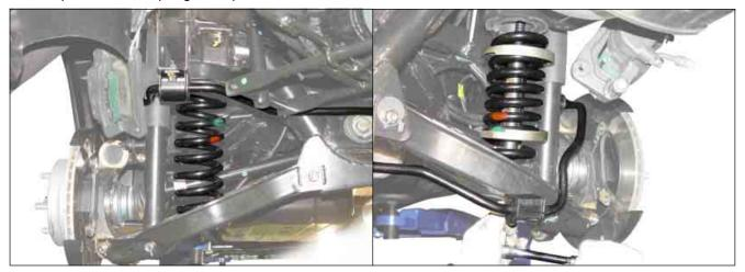
2. Release the compression force of coil spring by loosening the lower shock absorber bolt/nut and remove the coil spring and upper spring seat.
