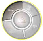
When you see a steep downhill ahead, press the HDC switch and the green HDC indicator comes on. When the G sensor within the sensor cluster detects a inclination exceeding 10%, the ESP's HDC function operates. When this occurs, the green HDC indicator goes off along with a loud operation noise.
