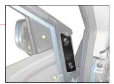
Unscrew the mounting screws with dotted circle and remove the door trim from lower side (For details, refer to "Door" section.).
