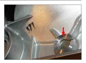
5. Push out the parking pawl guide bushing from inside with a proper tool.
