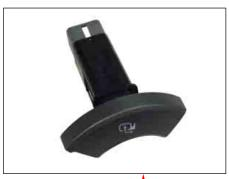
To fold the outside rearview mirrors, press the switch. To unfold the mirrors, press it again.
