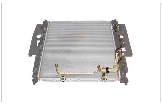
15. Unscrew five mounting bolts (10 mm) and remove the air conditioner condenser assembly.
