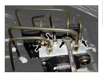
5. Unscrew two mounting nuts and carefully remove HECU.
