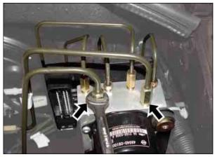
3. Disconnect the front and rear wheel brake pipes.
