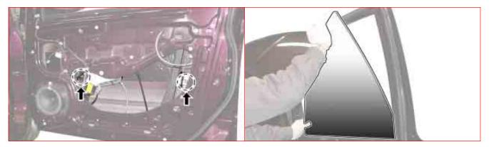
2. Disconnect the window motor connector and unscrew the mounting bolts from the window regulator.
