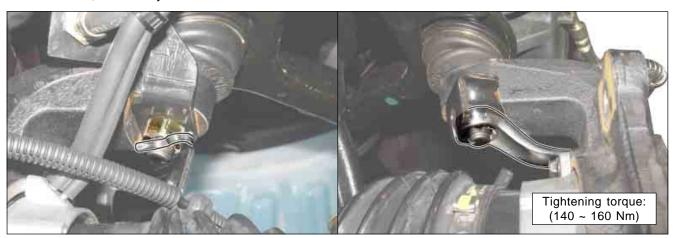
3. Pull out the steering gear linkage lock pin from the knuckle. Unscrew the mounting nut (19 mm) and remove the tie rod end.
