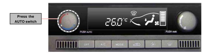
2. When pressing the AQS switch, the AQS indicator on display window comes on, and the air source selection is automatically changed to recirculation mode (REC). At this moment, the self diagnosis and preheating mode of AQS is performed for 35 seconds.
