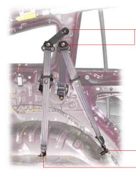
1. Open the bolt cap and unscrew the upper mounting bolt.
