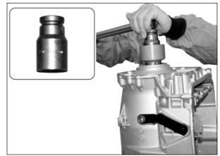
5. Remove the rear oil seal ring.
