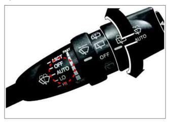
**AUTO**: Wiper operates automatically by rain sensor **FAST** ↔ **SLOW**: Auto delay/Auto speed control. A position that can control sensitivity against rains in the windshield and transmits wiping demand signal accordingly
