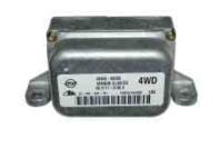
The G Sensor within the sensor cluster <u>detects the steepness of driving roads</u>. When the HDC switch is in operation, if the G sensor detects a downhill steepness exceeding 10%, it transmits the HDC operation signal to the ESP HECU.
