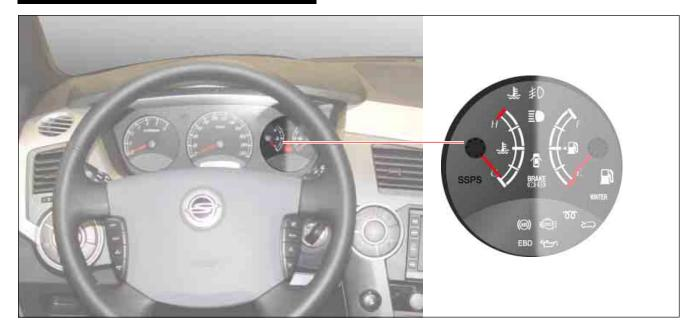
The coolant temperature gauge displays the coolant temperature with a pointer. The angle of pointer that changes by coolant temperature is as shown below.
