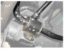
Tightening torque 40 ~ 60 Nm
