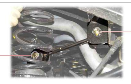
A. Unscrew upper arm mounting bolt/nut (22 mm) on axle.
