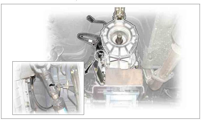
10. Support the transmission housing with a hydraulic jack and unscrew eleven transmission bolts (17 mm). (Tightening torque: 50 ~ 60 Nm)
