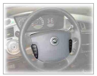
2. Disconnect all connectors and remove the air bag assembly.
