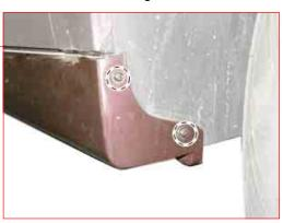
2. Unscrew four mounting screws from the front/rear side seal moldings.
