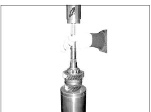
29. Remove the reverse gear inner race.
