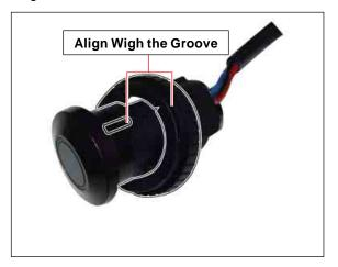
2. Insert the sensor upper cover into the sensor groove.
