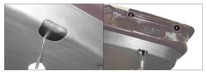
2. Disconnect the connector and remove the rear combination lamp assembly.
