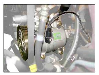
Unscrew the flange nuts of pressure pipes and compressor mounting bolts and remove the compressor assembly.
