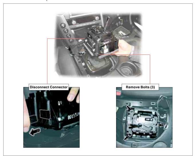
6. Install in the reverse order of removal. Make sure the selector lever and the shift lever are at the same position.
