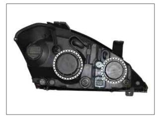
2. Disconnect the high/low beam connectors from the headlamp assembly.
