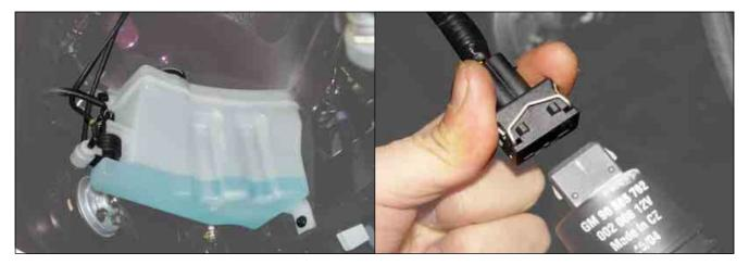
4. Disconnect the washer hose connecting the reservoir tank and nozzle from the reservoir tank wheel house. Unscrew the washer reservoir tank mounting bolt and then remove it.
