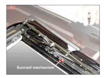
3. Push down the outside cover to install into the roof panel and lock it to the sunroof system with a pliers.
