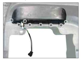
3. Remove the power outlet from the bracket.
