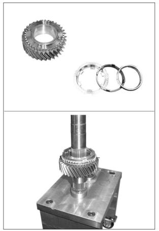
3. Insert three keys into 1/2 synchronizer hub and double synchronizer sleeve. Install the synchronizer spring in offset so that it should not be missed out.
