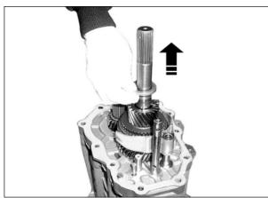
13. Remove the 5th gear and pull out the spring pin.
