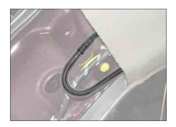
3) Remove the roof wiring connector (A) and rear washer fluid hose (B) in driver side.
