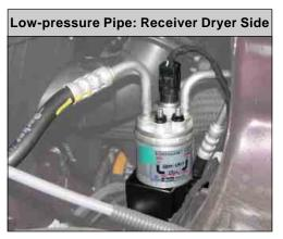
Plug the pipe openings with a seal caps after disconnecting the high/ low pressure pipes.
