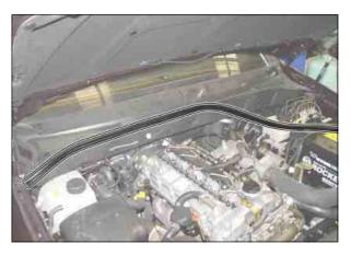
4. Remove the cowl mounting clip and then disconnect the cowl from the left (driver side).
