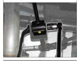
Tightening torque 150 ~ 180 Nm
