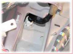
Disconnect the Door Wiring Harness.
