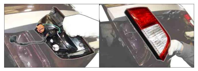
3. Open the bulb holders/connectors by turning them counterclockwise and remove the bulbs.
