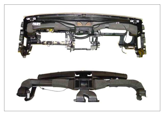
1. Unscrew the mounting screws (one at each side and four in center area) and remove the front air duct.
