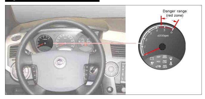
The tachometer indicates engine speed in revolutions per minute. Multiply 1,000 to the current number, then it will be the current number of engine revolutions.
