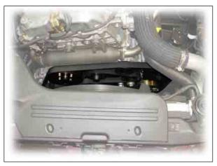
2. Disconnect the power steering return hose and remove the high pressure pipe nut.
