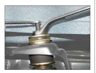
2) Remove the lower bolt/nut (17 mm).
