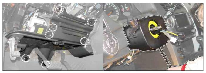
5. Disconnect the contact coil and connector from the column shaft and remove the contact coil assembly.
