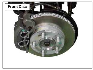
Front Ventilated Disc and Caliper (2 internal Cylinders)
