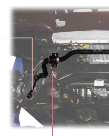
2. Unscrew the two bracket mounting bolts (14 mm) and remove the stabilizer bar assembly.
