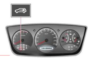
This indicator comes on when the ignition key is communicating with the engine control unit (during engine starting) and goes out after starting the engine.
