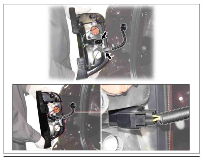
3. Open the bulb holders/connectors by turning them counterclockwise and remove the bulbs.
