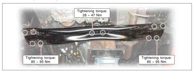
7. Unscrew two bolts (14 mm) at both sides and remove the transmission mounting insulator. Unscrew the mounting bolts (14 mm, 2) at both sides and remove the mounting insulator bracket.
