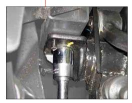
C. Sub frame coil bolt (front - 14 mm) Tightening torque: 95 ~ 142 Nm
