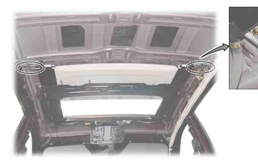
3. Unscrew the mounting bolts (10 mm) at both sides.
