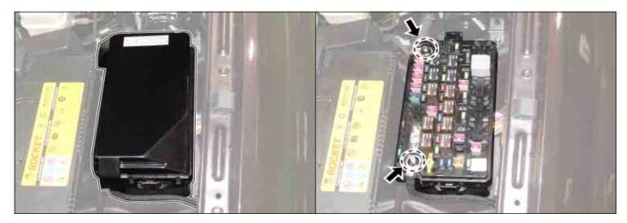
2. Lift the fuse and relay box assembly and disconnect connectors behind the assembly.
