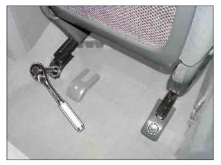
3. Lay down the seatback and disconnect the connector under the seat and then remove the seat assembly.
