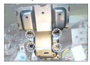
4) Disconnect the center wiring connector and unscrew the mounting bolt.
