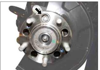
5. Slightly pull the wheel end hub until the wheel speed sensor is visible. Unscrew the mounting bolt (5 mm) and remove the wheel speed sensor.
