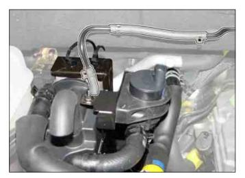
3. Unscrew the hose clamps on the FFH coolant circulation pump and remove the inlet and outlet hoses.
