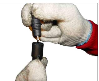
2. Remove one of self-locking bolt (10 mm). Remove rear wheel speed sensor.
