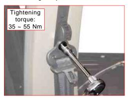
5. Carefully lower the seat belt and unscrew the mounting screws and bolts to remove the seat belt.
