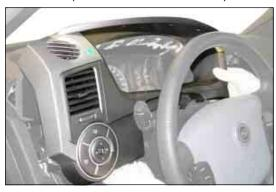
7) Remove the DVD changer and passenger side lower instrument panel (Refer to "AV System" section.).
