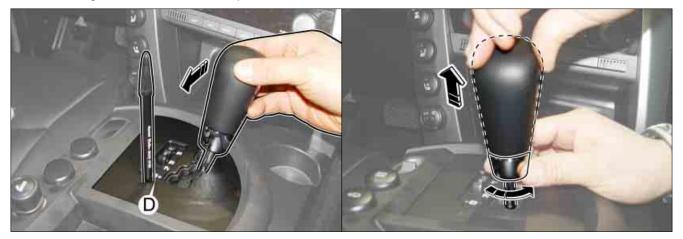
2. Remove the center console upper cover and disconnect the cigarette lighter. Remove the selector lever cover
