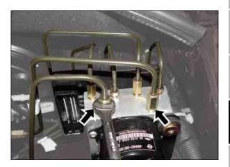
4. Disconnect the front and rear wheel brake pipes.
