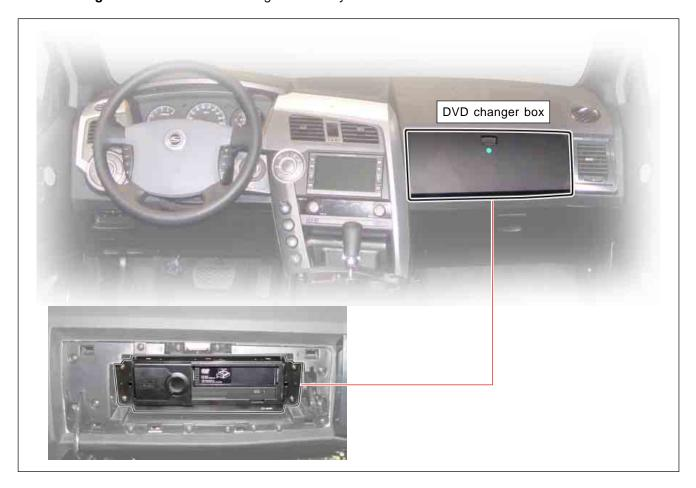
1. Remove the glove box lamp and release the locking device to lower the glove box.
