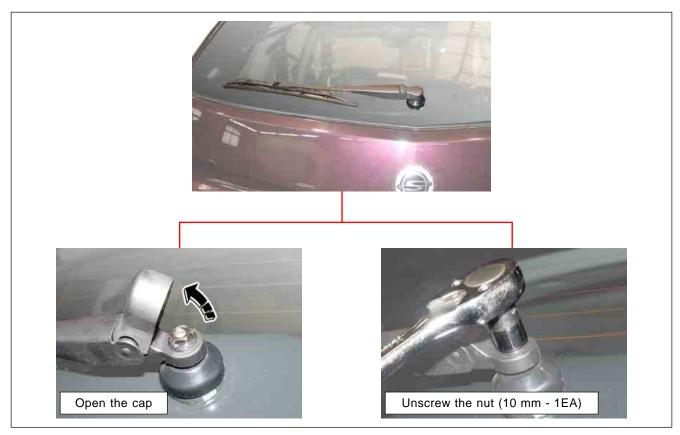
4. Remove the wiper blade and then unscrew the wiper motor cap and the mounting nut (17 mm - 1EA).
