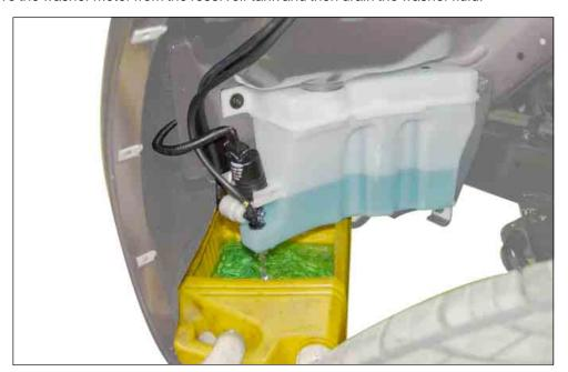
3. Disconnect the washer motor connector from the reservoir tank. Be careful not to contact the washer fluid or foreign materials into the motor and connector after disconnecting.
