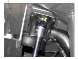
D. Sub frame bolt (rear - 14 mm) Tightening torque: 95 ~ 142 Nm
