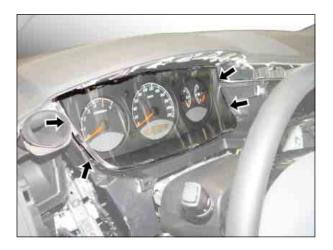
5. Disconnect the connectors from the back of meter cluster and remove the cluster from the instrument panel.
