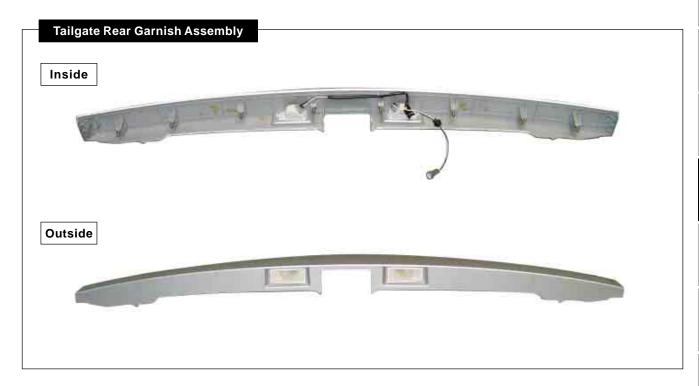
2. Disconnect the bulb and bulb cable from the removed rear garnish assembly and then remove the lamp by pressing (A) section of the lamp.
