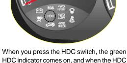
When you press the HDC switch, the green HDC indicator comes on, and when the HDC operates, the green HDC indictor flashes at 0.5 second of interval.
