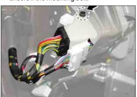
3) Disconnect the main wiring connector (A) and air bag connector (B).
