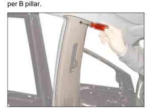
Unscrew the upper screw and remove the up-
