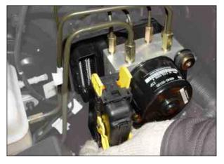
2. Disconnect the primary and secondary master cylinder pipes from HECU.
