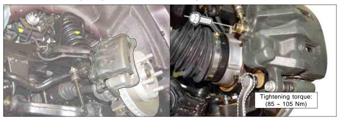
2. Unscrew the two screws and remove the brake disc.
