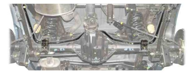
2) Remove the mounting cap bracket and bushing from the stabilizer bar (LH/RH).
