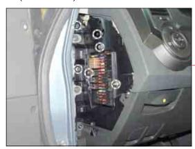
4) Remove the parking brake lever bracket and fuse/ relay box assembly.
