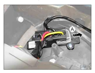
2. Unscrew two mounting bolts and remove the PTC assembly from the A/C module assembly.
