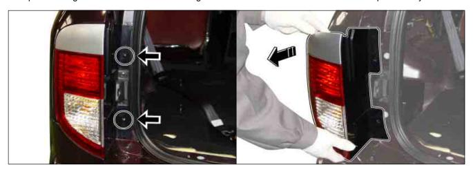
2. Disconnect the connector and remove the rear combination lamp assembly.
