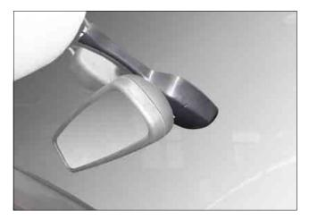
A sensor that emits infrared rays through LED and then detects the amount of rain drops by receiving reflected rays against sensing section (rain sensor mounting section on the windshield) with photodiode (auto light sensor integrated type)
