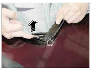
3. Unhook the wind deflector bottom locks as shown in figure (A).
