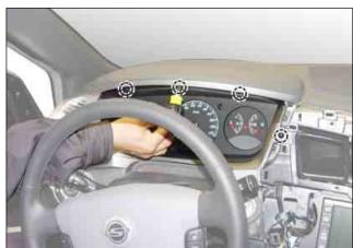
3. Disconnect the outside mirror switch bezel connector and remove the meter cluster panel assembly.
