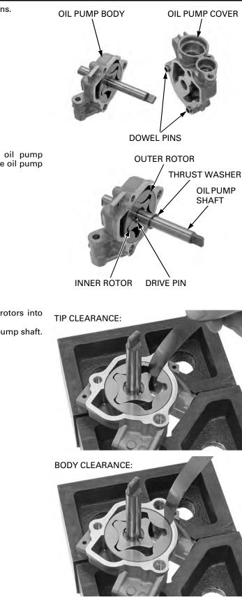
Remove the thrust washer, drive pin, oil pump shaft, outer rotor and inner rotor from the oil pump body.
