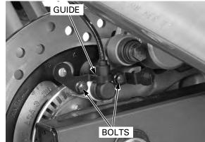
Remove the wheel speed sensor from the caliper bracket.
