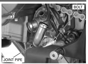
Connect the bypass hose, then tighten the hose band screw (page 6-22).
