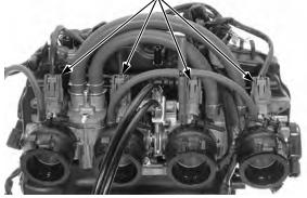
Release the CKP sensor 2P (Red) connector from the stay.
