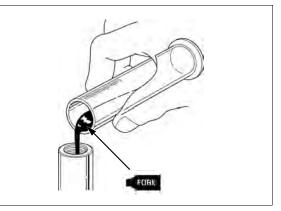
temporarily install the fork spring, spring seat, spring collar and fork cap.
