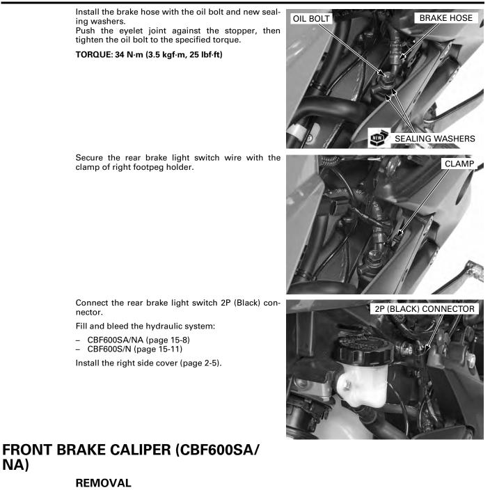
Drain the front brake hydraulic system (page 15-7). Remove the brake pads (page 15-15).
