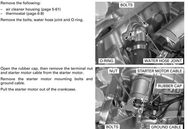
Remove the O-ring from the starter motor.
