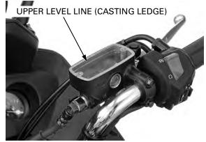
Install the diaphragm and set plate. Install the reservoir cap and tighten the screws to the specified torque.
