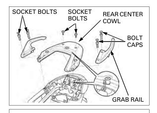
Remove the socket bolts and special bolts/collars. Remove the trim clips.
