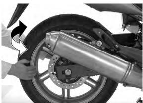
Check for worn swingarm bearings by grabbing the rear swingarm and attempting to move the swingarm side to side.
