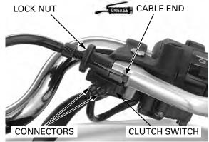
with its hook to the groove on the clutch lever bracket. Connect the clutch switch wire connectors to the switch.
