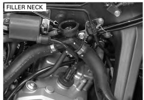
Remove the radiator reserve tank cap and fill the reserve tank to the upper level line.
