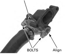
Install a new O-ring to the thermostat housing groove.
