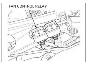
Connect the ohmmeter to the fan control relay connector terminals.
