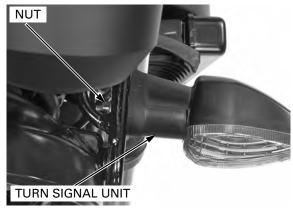
At installation, align the tab of the turn signal lens with the slit of the turn signal unit.
