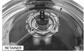
halogen headlight bulb. Finger prints can create hot spots that cause a bulb to break.
