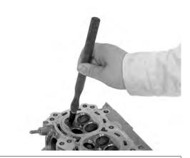
Remove the valve and inspect the valve seat face. The valve seat contact should be within the specified width and even all around the circumference.
