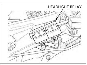
Connect the ohmmeter to the headlight relay connector terminals.
