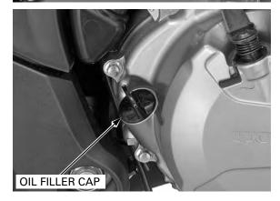
Fill the recommended engine oil up to the upper level line.
