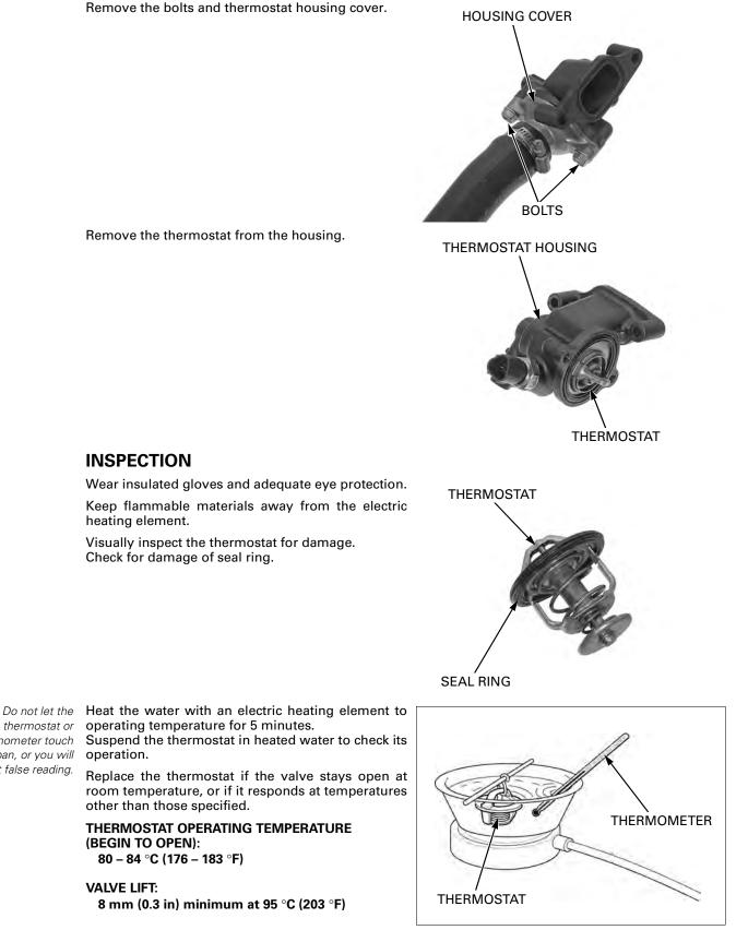
Remove the thermostat from the housing.
