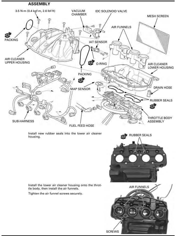
Install the mesh screen by aligning with the guides of upper air cleaner housing.
