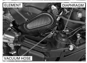
Disconnect the vacuum hose from the diaphragm. Remove the air cleaner element.
