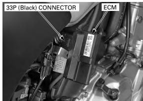
Ground the White/blue wire terminal of the wire harness side connector with a jumper wire.
