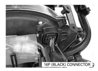
Remove the combination meter mounting bolts. Remove the combination meter.
