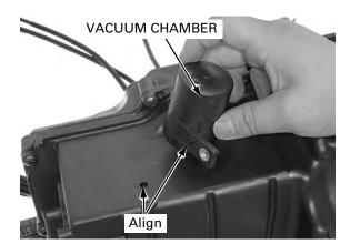
chamber boss with the hole on the air cleaner housing.
