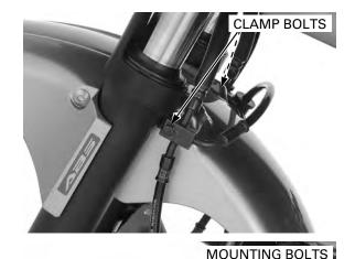
Remove the mounting bolts and front fender.
