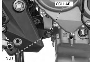
Carefully install the engine into the frame.
