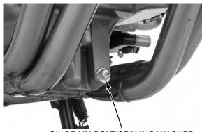
OIL DRAIN BOLT/SEALING WASHER
