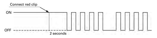
• The immobilizer system (HISS) enters the registration mode. Registrations of all key except the original key inserted in the ignition switch are cancelled. (Registration of the lost key or spare key is cancelled.)
