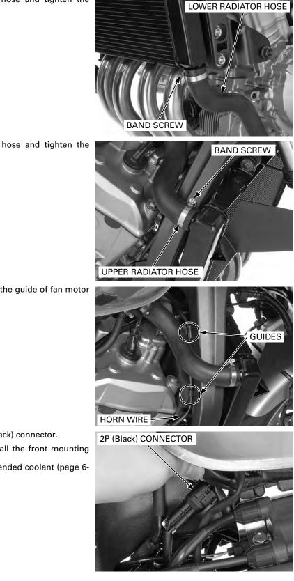
Connect the upper radiator hose and tighten the hose band screw (page 6-22).
