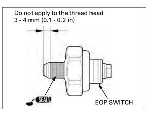
Install and tighten the EOP switch to the specified torque.
