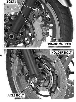
CBF600SA/NA:Be careful not to damage the speed sensor on the brake caliper. Loosen the left axle holder bolt. Remove the axle and the front wheel.
