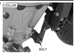
Remove the left front engine hanger bracket bolts, washers and nuts.
