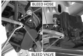
Pressurize the system with the brake lever until lever resistance is felt.
