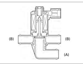
Check the resistance between the terminals of the PAIR control solenoid valve.
