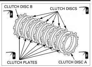
Install the tabs of outside clutch disc A into the shallow slots of the clutch outer.
