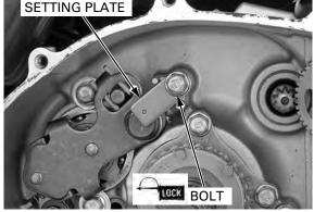
Install the gearshift arm to the gearshift spindle, aligning the arm slit with the punch mark on the gearshift spindle.
