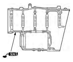
Install the oil orifices, aligning its cut-out with the groove of upper crankcase.
