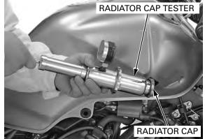
Pressure the radiator, engine and hoses, and check for leaks.
