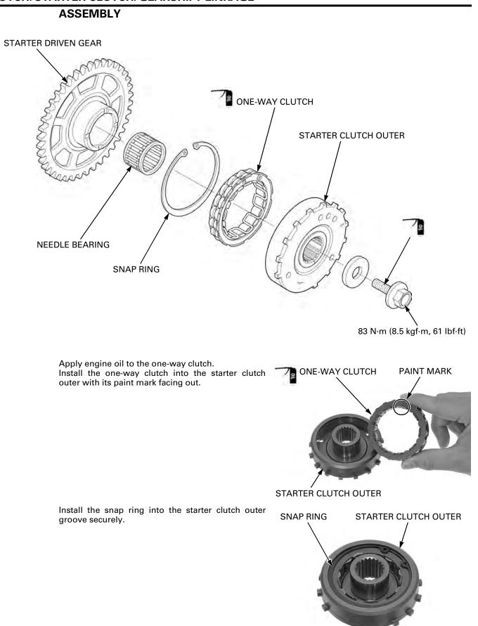
Install the starter driven gear into the starter clutch outer while turning the starter driven gear clockwise.
