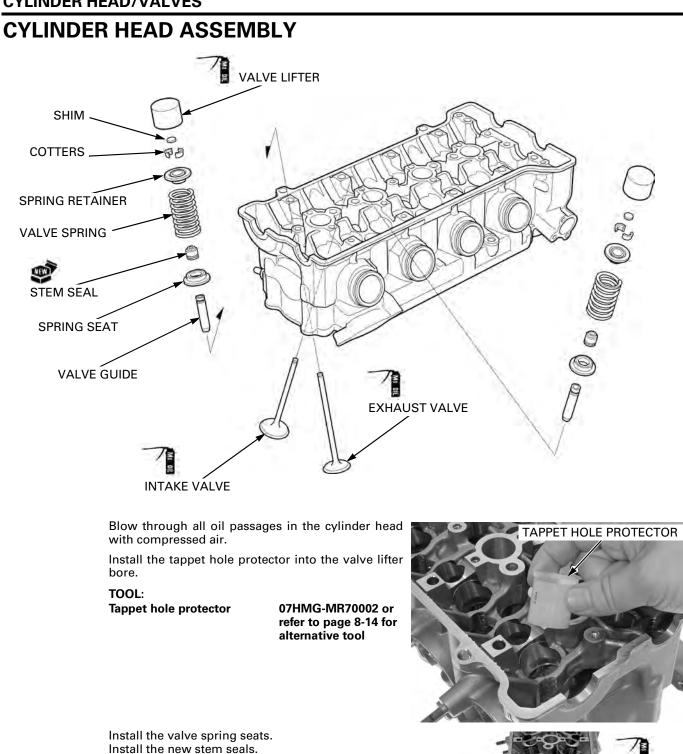
Lubricate the valve stems with molybdenum oil solution.
