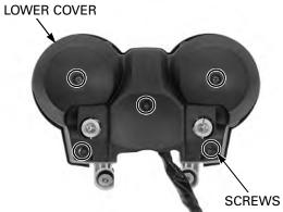
Remove the screws and lower cover.
