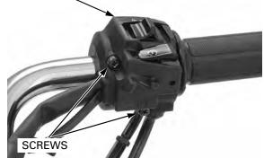
Disconnect the throttle cable ends from the throttle pipe and remove the right handlebar switch/throttle housing.
