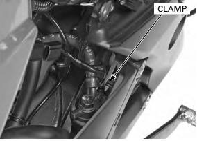
Avoid spilling fluid Remove the brake hose oil bolt, sealing washers on painted, plastic, and brake hose.
