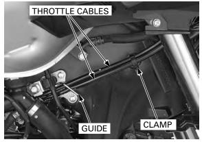
Route the wires properly (page 1-24). Route the throttle cables properly. Connect the throttle cables to the throttle pipe. Install the right handlebar switch housing (page 13-11).
