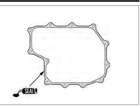
Install the oil pan onto the lower crankcase. Install the flange bolts.
