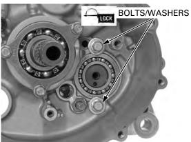
Apply a locking agent to the shift drum bearing set bolt threads.
