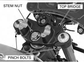
Remove the handlebar (page 13-8). Remove the steering stem nut.
