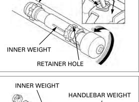
Remove the grip end from the handlebar weight. Discard the retainer.
