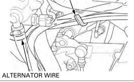
The alternator cover (stator) is magnetically attached to the flywheel, be careful during removal.
