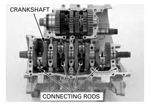
Apply molybdenum oil solution to the crankpin bearing sliding surfaces on the connecting rod bearing caps.
