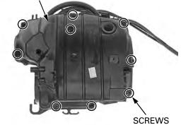
Install a new right air cleaner duct packing into the groove on the housing.
