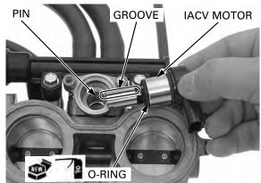
Install the setting plate while aligning the cut-out with the lug on the IACV motor.
