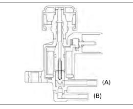
Check the resistance between the terminals of the IDC solenoid valve.
