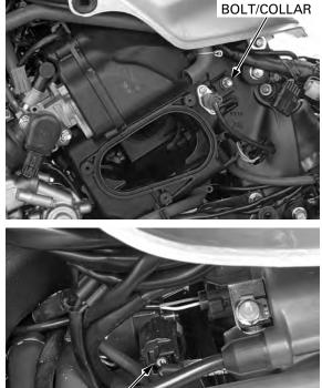
Connect the PAIR control solenoid valve 2P (Black) connector.
