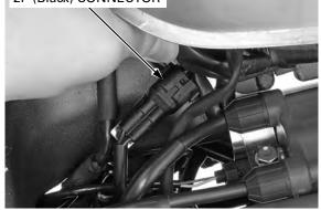
Release the horn wire from the guide of fan motor shroud.
