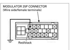
7. Logic Ground Line Open Circuit Inspection
