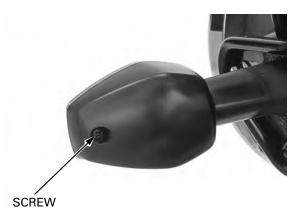
While pushing in, turn the bulb counterclockwise to remove it and replace with a new one.
