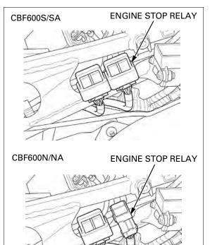
Connect the ohmmeter to the engine stop relay connector terminals.
