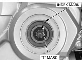
Turn the crankshaft clockwise, align the "T" mark on the CKP sensor rotor with the index mark on the right crankcase cover.
