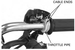
Remove the bolts and handlebar holders. Remove he handlebar.
