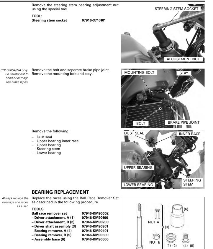
Note the installation<br/>direction of the<br/>assembly base; the<br/>small 1.D. side<br/>facing the upper<br/>attachment.Install the ball race remover into the head pipe as<br/>shown.Align bearing remover A with the groove in the<br/>steering head.<br/>Lightly tighten nut B with a wrench.
