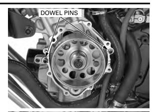
The alternator cover (stator) is magnetically attached to the flywheel, be careful during installation.
