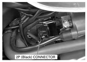
Pull the PAIR control solenoid valve out the stay. Installation is in the reverse order of removal.
