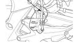
Install mounting bolt with the collar, then tighten the bolt securely.
