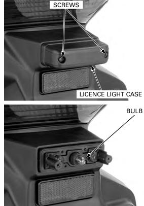
Remove the license light bulb and replace with a new one.
