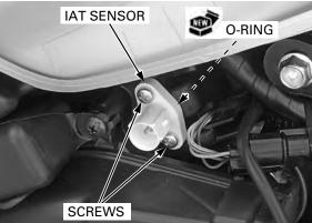
Remove the screws and IAT sensor from the air cleaner housing.
