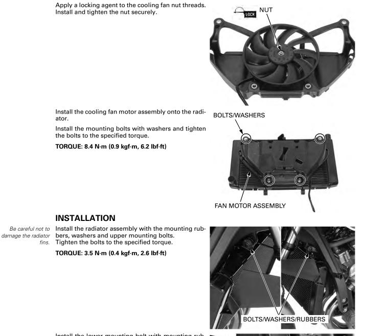
Install the lower mounting bolt with mounting rubber and washer.
