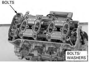
Loosen and remove the camshaft holder bolts/ Suspend the cam washers, then remove the camshaft holders and chain with a piece of wire to prevent camshafts. the chain from NOTE: falling into the
