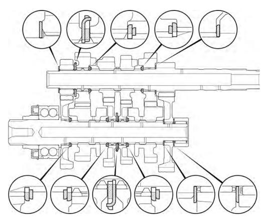
Assemble the transmission gear and shafts.
