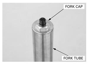
Remove the B-clip and plate from the fork cap.
