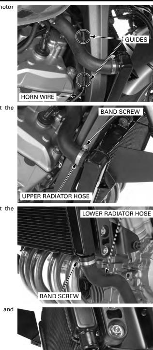
Loosen the hose band screw and disconnect the upper radiator hose.
