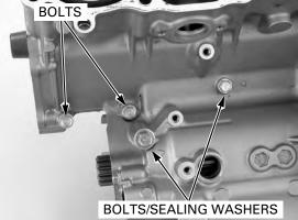
Remove the bolts and sealing washers.
