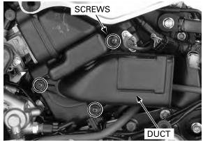
Refer to the wires Route the wires and hoses to the guides of air properly cleaner housing. (page 1-24).
