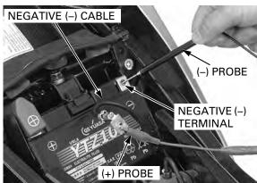
If current leakage exceeds the specified value, a shorted circuit is likely. Locate the short by disconnecting connections one by one and measuring the current.
