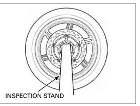
To balance the wheel, install wheel weights on the highest side of the rim, the side opposite the chalk marks. Add just enough weight so the wheel will no longer stop in the same position when it is spun. Do not add more than 60 grams to the wheel.
