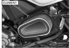
Remove and inspect the air cleaner element in accordance with the maintenance schedule (page 3-4).
