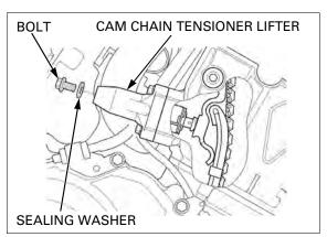
Failure to release the cam chain tensioner will result in inaccurate valve clearance reading.
