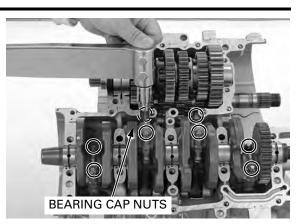
Remove the bearing caps and measure the compressed plastigauge at its widest point on the crankpin to determine the oil clearance.
