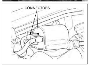
Connect the #1/#4 ignition coil connectors.
