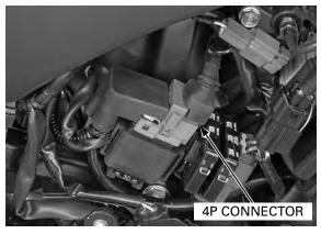
Remove the bolts and disconnect the starter relay cables.
