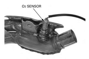
Remove the O<sub>2</sub> sensor using the special tool.
