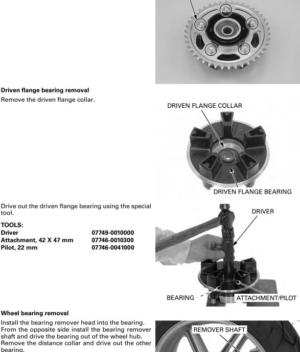
Drive out the driven flange bearing using the special tool.
