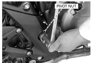
Install the shock absorber lower mounting bolt/nut, then tighten the nut to the specified torque.
