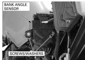
Install the bank angle sensor with its "UP" mark facing up. Installation is in the reverse order of removal. Tighten the mounting screws securely.
