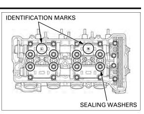
Gradually tighten the camshaft holder bolts until the camshaft holders lightly contact the cylinder head surface.
