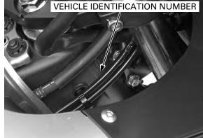
The registered number plate is located on left side of the frame tube.
