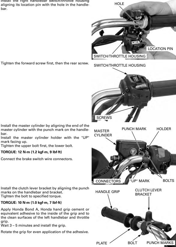
Install the master cylinder by aligning the end of the master cylinder with the punch mark on the handlebar.
