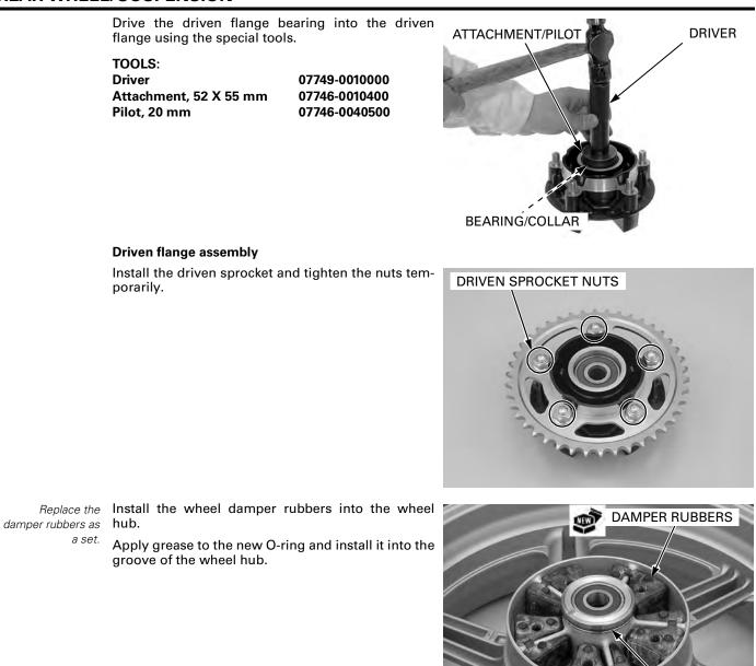
Apply grease to the driven flange and rear wheel
