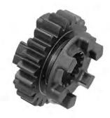
Check the gear dogs, dog holes and teeth for abnormal wear or lack of lubrication.
