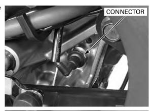
Remove the neutral switch and sealing washer.
