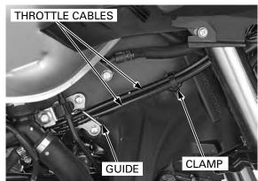
*CBF600S/SA only:* Release the throttle cables from the clamp. Release the throttle cables from the guide.
