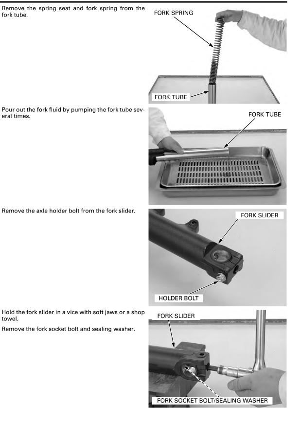
If the fork piston turns together with the socket bolt, temporarily install the fork spring, spring seat, spring collar and fork cap.
