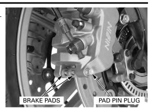
Remove the pad pin and brake pads.
