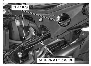
Secure the alternator wire with the clamps.
