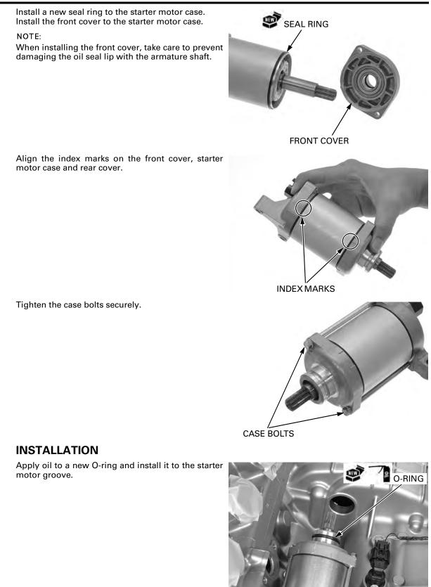
Install the starter motor into the crankcase.
