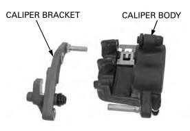
Remove the pad retainer and caliper pin boot from the caliper bracket.
