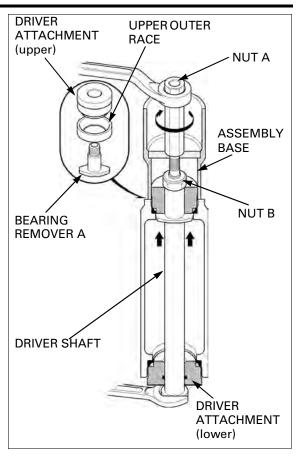
Note the installation direction of the assembly base; the large I.D. side facing the lower attachment. Be careful not to bend or damage the brake pipes (CBF600SA/NA)
