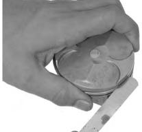
Push the rings into the cylinder with the top of the piston to be sure they are squarely in the cylinder.
