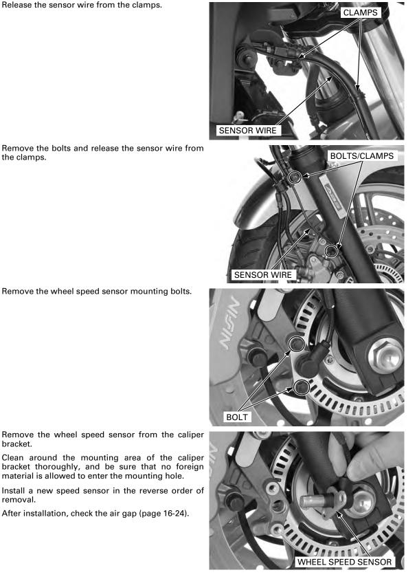
Remove the bolts and release the sensor wire from the clamps.
