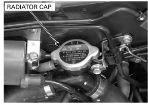
Test the coolant gravity using a hydrometer (see below for "Coolant gravity chart").
