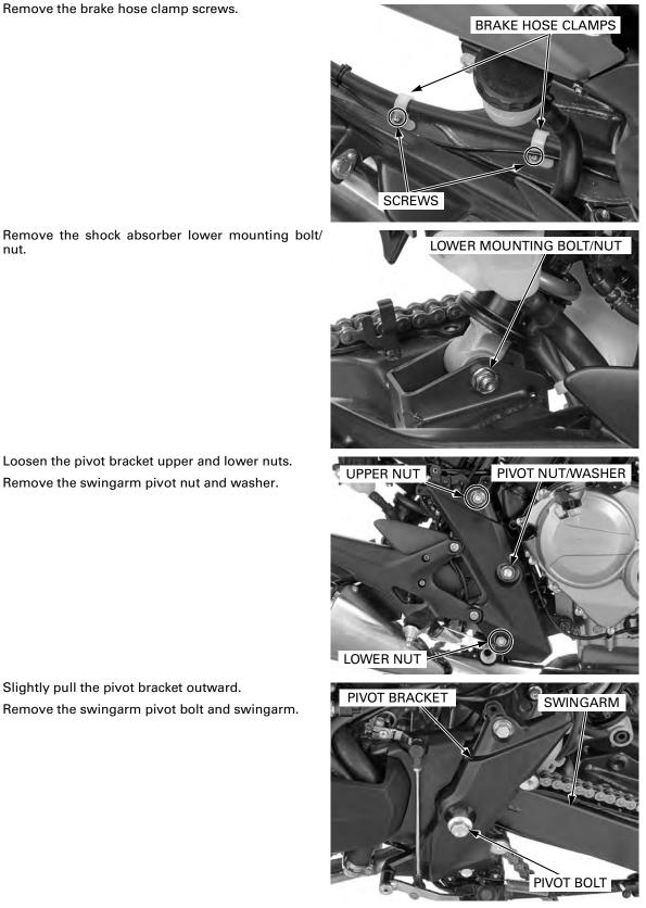
Remove the shock absorber lower mounting bolt/ nut.
