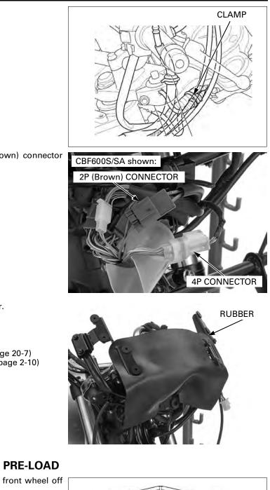
Connect the ignition switch 2P (Brown) connector and immobilizer 4P connector.
