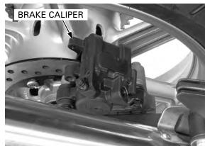
Connect the brake hose to the rear caliper with the oil bolt and new sealing washers. Push the brake hose eyelet to the stopper on the caliper, then tighten the oil bolt to the specified torque.
