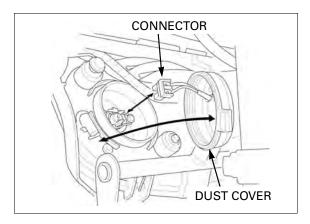
Avoid touching halogen headlight bulb. Finger prints can create hot spots that cause a bulb to break. Unhook the bulb retainer and remove the headlight bulb.
