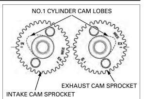
Clean and apply a locking agent to the cam sprocket bolt threads. Install the cam sprocket bolts.
