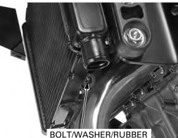
Connect the lower radiator hose and tighten the hose band screw (page 6-22).
