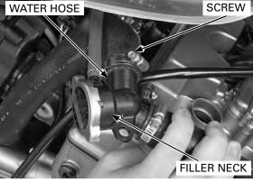
Disconnect the ETC sensor 3P (Black) connector. Loosen the hose band screw and disconnect the bypass hose from the thermostat housing. Remove the bolts, thermostat housing and O-ring.
