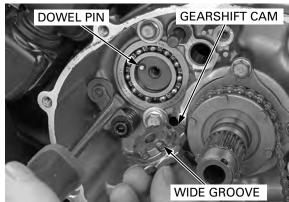
Apply a locking agent to the shift drum center socket bolt threads. Tighten the socket bolt to the specified torque.
