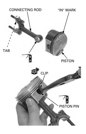
Coat the cylinder walls, pistons and piston rings with engine oil.
