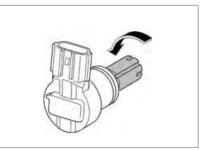
Apply oil to new O-ring and install it to the IACV motor.
