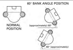
Place the bank angle sensor horizontal as shown, and turn the ignition switch ON and engine stop switch " $\bigcirc$ ".
