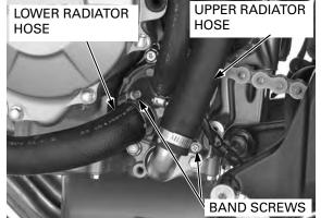
Loosen the hose band screw and disconnect the bypass hose from the water pump cover.
