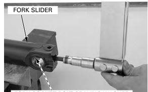
FORK SOCKET BOLT/SEALING WASHER
