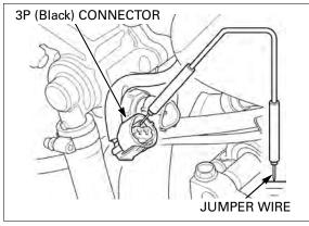
Turn the ignition switch to "ON" and check the engine coolant temperature indicators.
