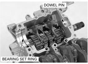
Remove the shift drum bearing set bolts/washers.
