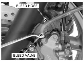
Connect a bleed hose to the right caliper bleed valve. Loosen the upper bleed valve and pump the brake lever until no more fluid flows out of the bleed valve.
