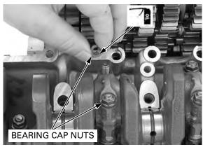
Tighten the nuts in two or three steps alternately, then tighten the nuts to the specified torque.
