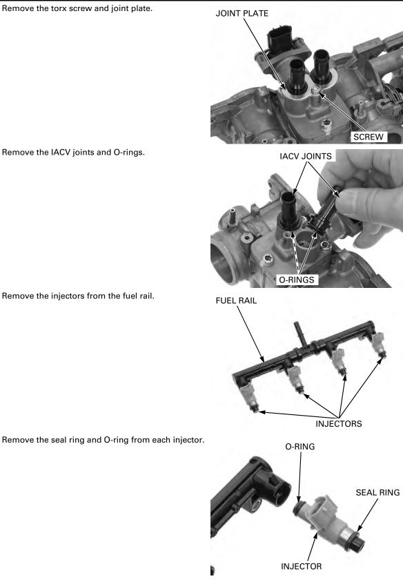
Remove the IACV joints and O-rings.
