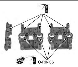
Note the correct locations with the identification marks as shown.
