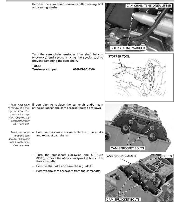
Remove the bolts and cam chain guide B.
