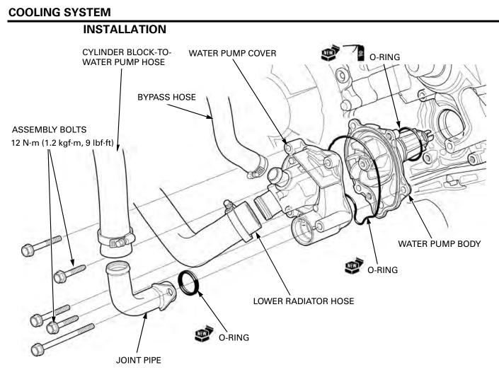
Apply engine oil to a new O-ring and install it onto the stepped portion of the water pump body.
