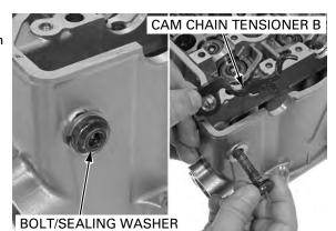
Remove the bleeding joint, sealing washer from the cylinder head.
