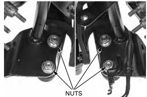
Tighten the lower engine mounting nut to the specified torque.
