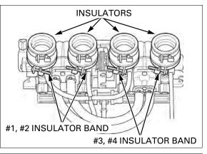
Tighten the throttle body side insulator band screws so that the width between the band ends is  $7 \pm 1$ mm (0.28  $\pm$  0.04 in).
