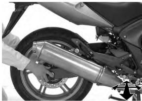
Check the action of the shock absorber by compressing it several times.
