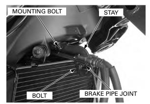
*CBF600N/S only* Apply a locking agent to the hose clamp bolt. Install the brake hose clamp and tighten the bolt to the specified torque.
