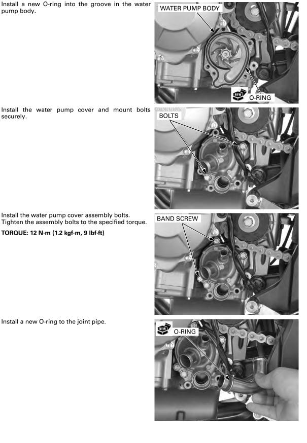
Install the water pump cover and mount bolts securely.
