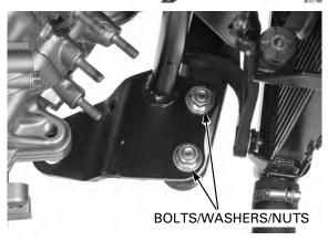
Install the front engine hanger bracket to the frame. Install the right front engine hanger bracket bolts, horn stay and nuts.
