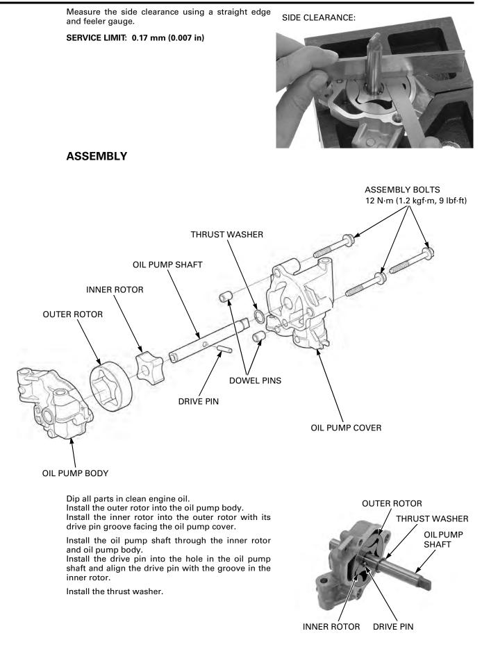
Install the dowel pins into the oil pump cover. Install the oil pump cover to the oil pump body.
