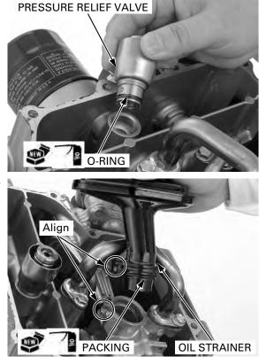
Apply engine oil to a new packing and install it onto the oil strainer flange.
