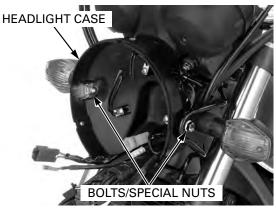
Remove the bolts, special nuts and headlight case.
