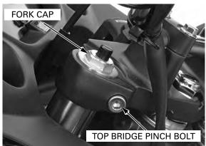
Loosen the fork bottom bridge pinch bolt and remove the fork tube from the fork top bridge and steering stem.
