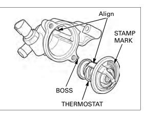
Install the thermostat housing cover to the housing by aligning the bosses of housing and cover. Tighten the bolts to the specified torque.
