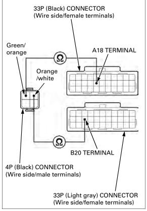
3. O<sub>2</sub> Sensor Short Circuit Inspection
