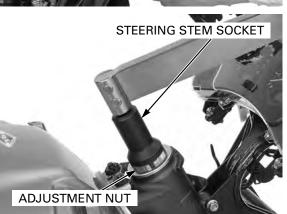
Install a new lock washer onto the steering stem. Align the tabs of the lock washer with the grooves in the adjustment nut and bend two opposite tabs (shorter) down into the adjustment nut groove.
