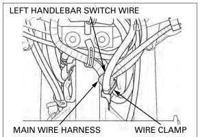
CBF600S/SA only: Install the main wire harness and left handlebar switch wire to the wire clamp securely.
