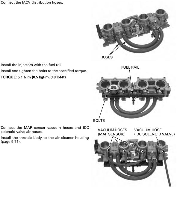
Install the injectors with the fuel rail. Install and tighten the bolts to the specified torque. TORQUE: 5.1 N·m (0.5 kgf·m, 3.8 lbf·ft)
