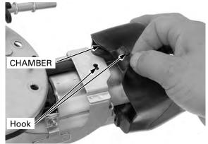
Always replace the Place a new packing onto the fuel pump unit. packing with a new one.
