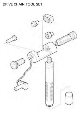
Locate the crimped pin ends of the master link from the outside of the chain, and remove the link with the drive chain tool set.
