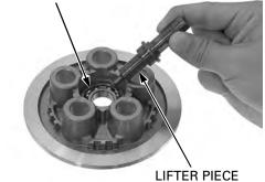
Install the pressure plate. Install the clutch springs and spring bolts. Tighten the bolts to the specified torque in a crisscross pattern in two to three steps.
