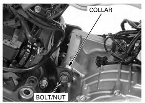
Remove the rear upper engine mounting bolt/nut and collar.
