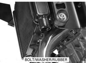
Be careful not to Remove the upper mounting bolts, washers and damage the radiator mounting rubbers, then remove the radiator assembly. fins.
