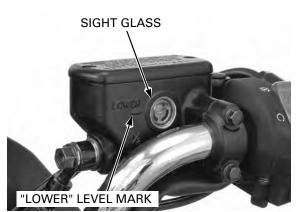
If the fluid level is near the "LOWER" level mark, remove the reservoir cap, set plate and diaphragm, and fill the reservoir with DOT 4 brake fluid from a sealed container to the casting ledge.
