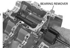
Drive in a new Drive a new bearing into the crankcase using the bearing squarely with the marking side facing up.
