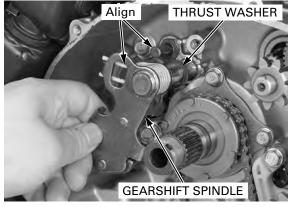
Apply a locking agent to the setting plate bolt threads. Install the setting plate and tighten the bolt securely.
