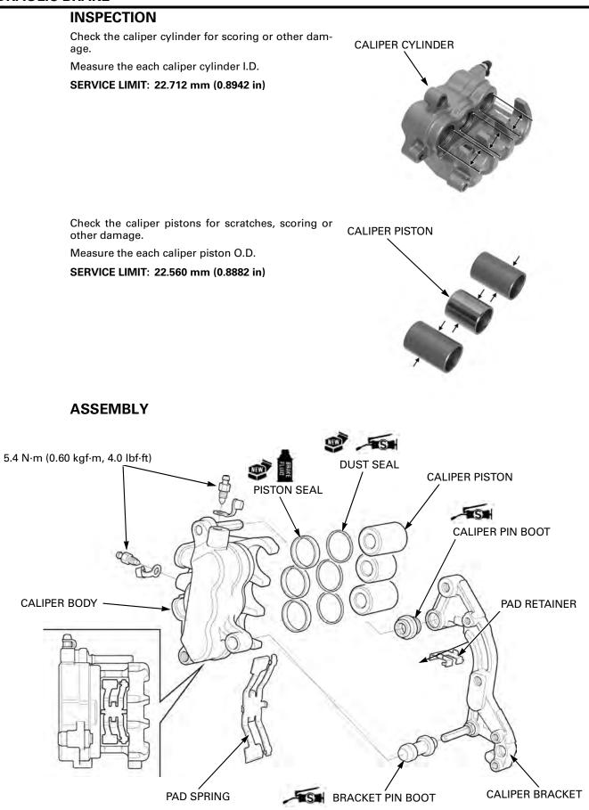
Coat new piston seals with clean brake fluid and install them into the seal grooves in the caliper. Coat new dust seals with silicone grease and install them into the seal grooves in the caliper.
