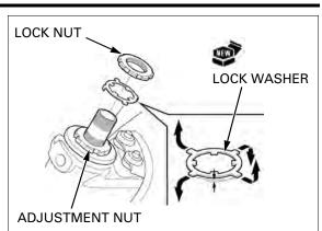
Do not over tighten the lock nut until the lock washer being flat.
