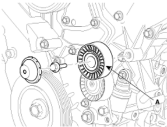
Fig. 65: Identifying Drive Belt Idler
