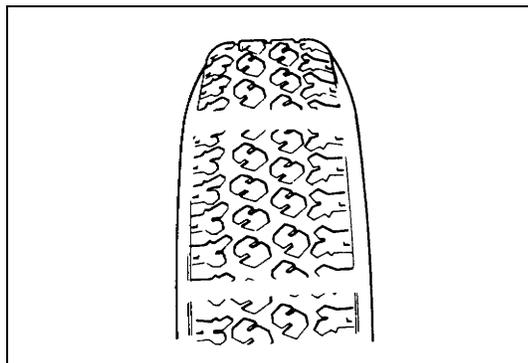
The original equipment tires have built-in tread wear indicators to show when tires need replacement. These indicators will appear as 12 mm (0.47 inch) wide bands when the tire tread depth becomes 1.6 mm (0.063 inch). When the indicators appear in 3 or more grooves at 6 locations, tire replacement is recommended.
