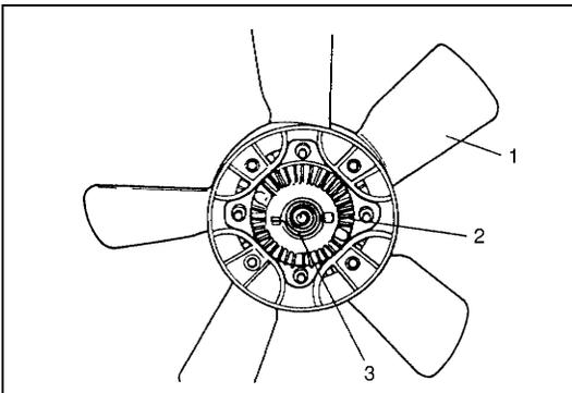
Fluid is enclosed in the cooling fan clutch (2) and at its center front, there is a bimetal (3) whose thermal reaction and the engine speed control the cooling fan speed.
