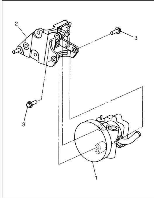
5) Remove P/S pump (1) removing 3 mounting bolts (3).
