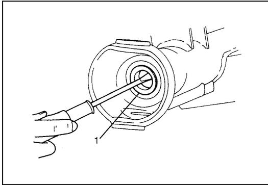
5) Remove oil seal (1) from axle housing (for 4WD).
