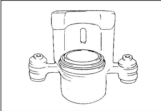
Check boots for breakage, crack and damage. If defective, replace.
