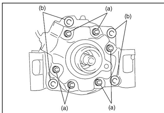
6) Tighten new front head bolts to specified torque.
