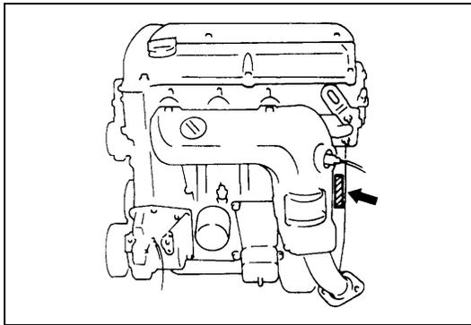
The number is punched on the cylinder block.
