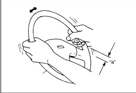
Check steering wheel for play and rattle, holding vehicle in straight forward condition on ground.
