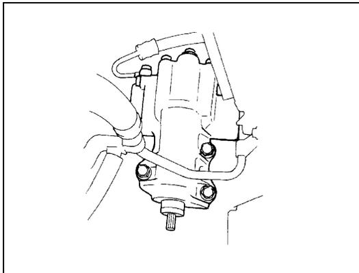
9) Remove gear box assy from vehicle.
