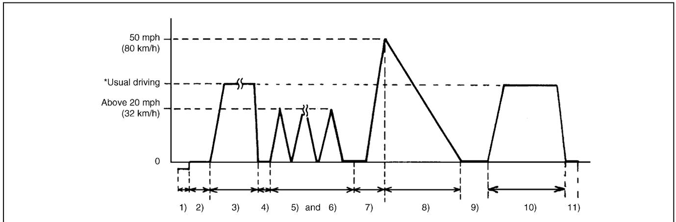
\*Usual driving : Driving at 30 – 40 mph, 50 – 60 km/h including short stop according to traffic signal. (under driving condition other than high-load, high-engine speed, rapid accelerating and decelerating)
