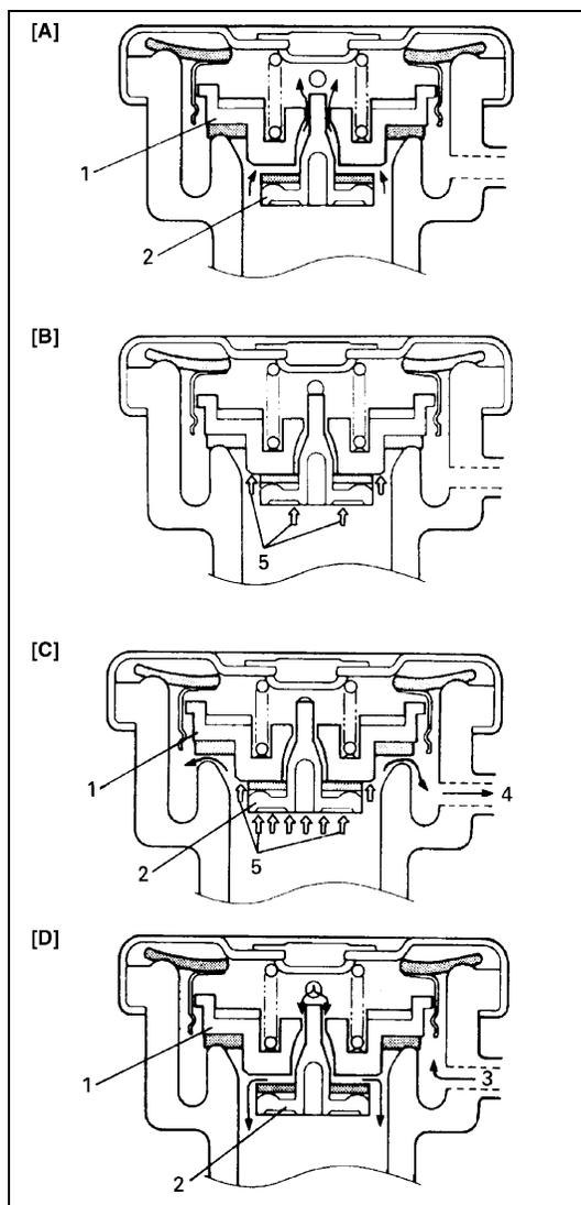
A pressure-vent cap is used on the radiator. The cap contains a pressure valve (1) and ventilation valve (2).
