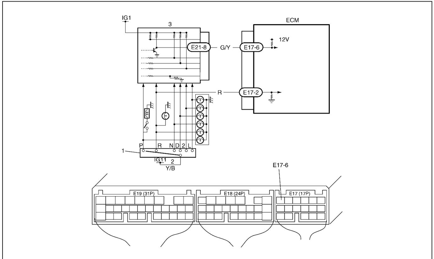
1. Transmission range switch    2. From ignition switch    3. TCM
