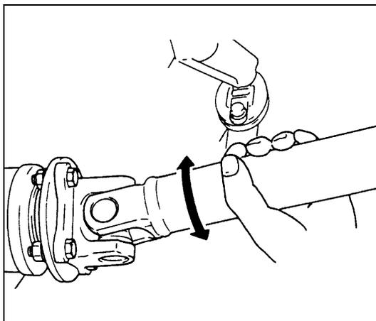
If universal joints are suspected of producing chattering or rattling noise, inspect them for wear. Check to see if cross spider rattles in yokes or if splines are worn down and replace defective propeller shaft with new one.
