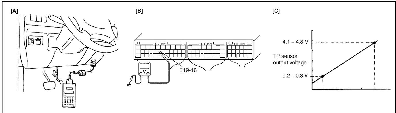
[A]: When using SUZUKI scan tool.
