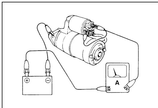
Connect battery and ammeter to starter as shown. Check that starter rotates smoothly and steadily with pinion moving out. Check that ammeter indicates specified current.
