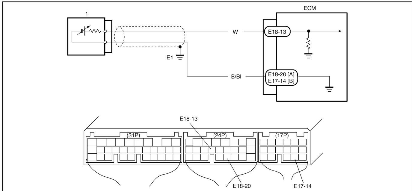
1. Heated oxygen sensor-2 (HO2S-2)
