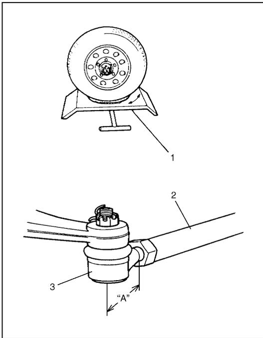
When tie rod (2) or tie rod end (3) was replaced, check toe and then also steering angle with turning radius gauge (1).
