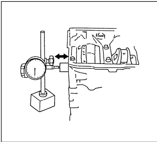
Use a dial gauge to read displacement in axial (thrust) direction of crankshaft.
