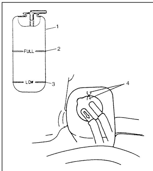
When engine is cool, check coolant level in reservoir (1).
