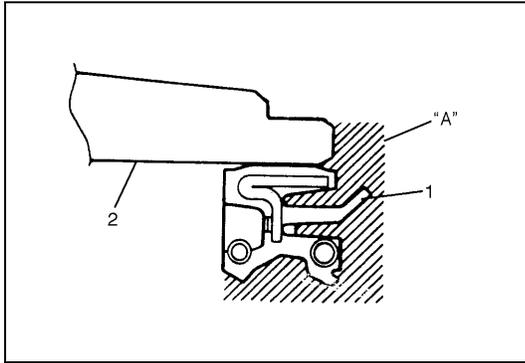
5) Apply lithium grease to lip portion and hollow of oil seal (1).
