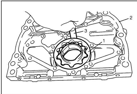
Check radial clearance between outer rotor (1) and case (2), using thickness gauge (3).
