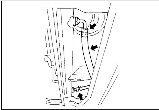
Replace inlet and outlet hoses of cooler hose and their clamps. For replacement procedure, refer to “Oil Cooler Hoses” in Section 7B.
