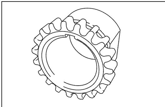
**Crankshaft timing sprocket**
