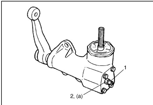
If measured torque is not within specification, carry out adjustment with adjusting bolt (1) to meet specification and check to confirm it again.
