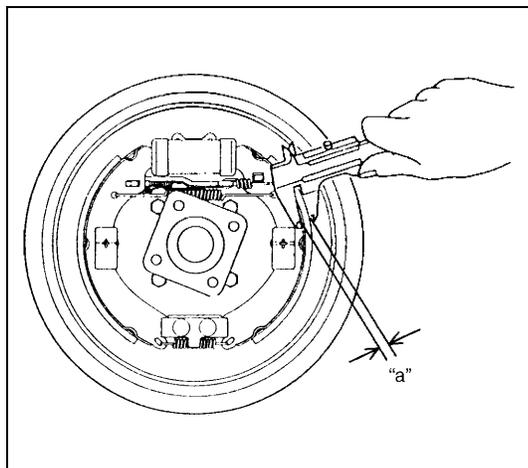
Where lining is worn out beyond service limit, replace shoe. If one of brake linings is to service limit, all linings must be replaced at the same time.
