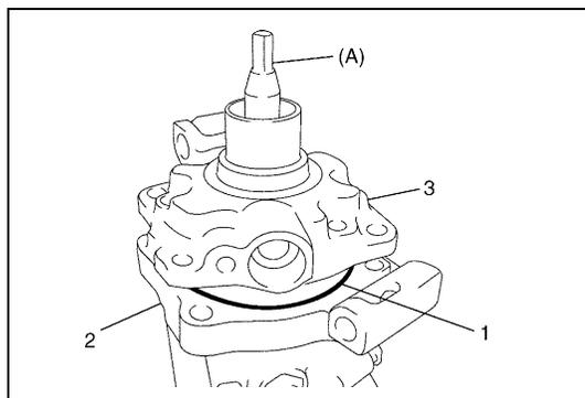
3) Install O-ring (1) to compressor body assembly (2).
