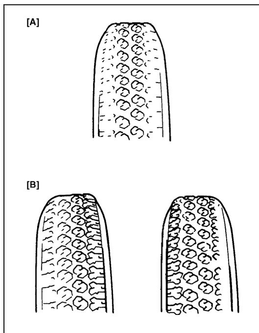
Irregular and premature wear has many possible causes. Some of them are: incorrect inflation pressures lack of tire rotation, driving habits, improper alignment.
