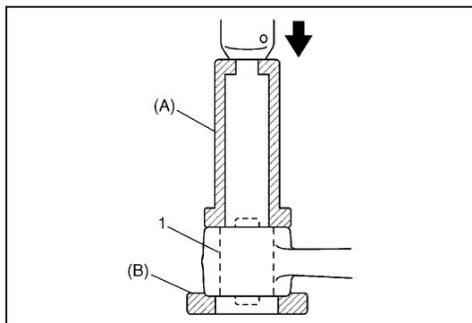
1) Install bushings (1) by using hydraulic press and special tools, noting the following points.
