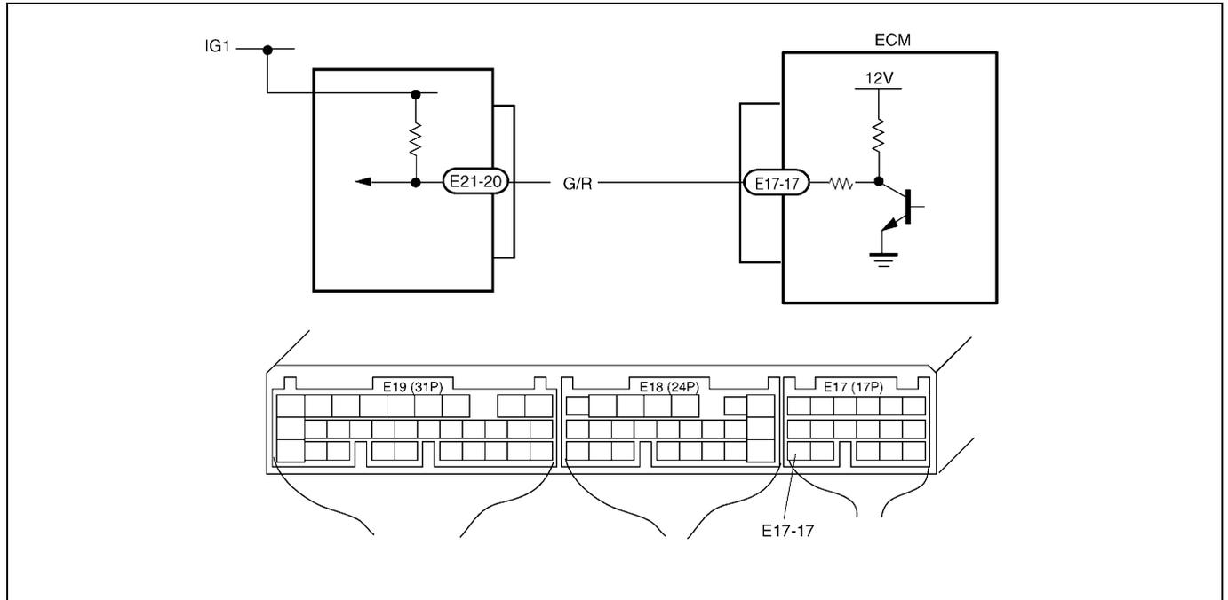
The serial data line is pulled up to about 12 V by ECM and TCM transmits information to ECM through it by controlling its grounding.
