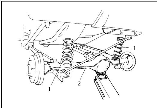
5) Lower rear axle housing (2) gradually as far down as where coil spring (1) can be removed.
