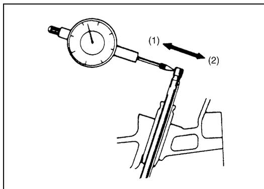
If bore gauge is not available, check end deflection of valve stem with a dial gauge instead.
