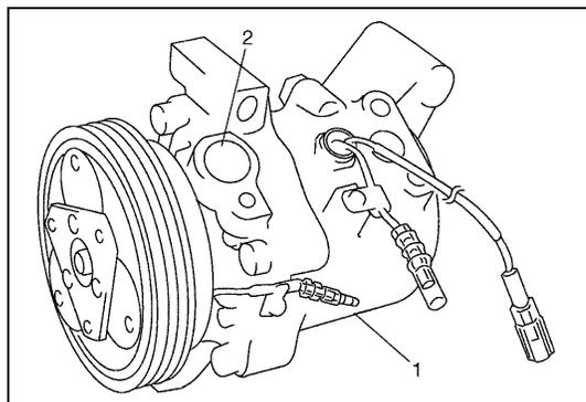
It is necessary to replenish specified amount of compressor oil to compressor (1) from compressor suction side hole (2) before evacuating and charging refrigerant.
