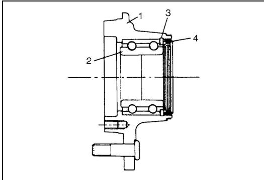
7) Remove front wheel bearing washer.
