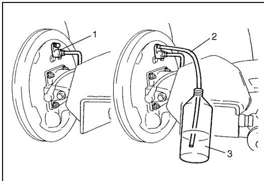
1) Fill master cylinder reservoir with brake fluid and keep at least one-half full of fluid during bleeding operation.
