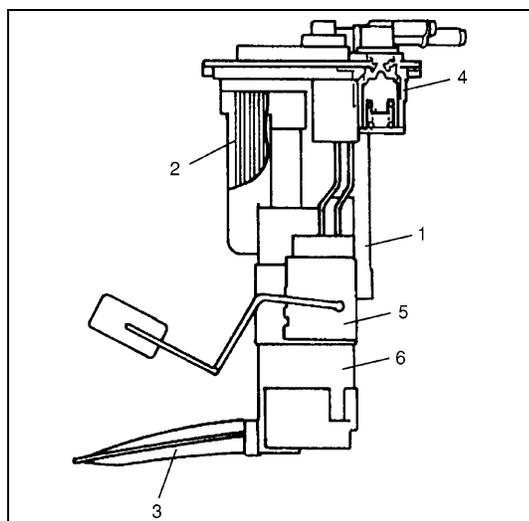
The fuel pump assembly (1) consists of fuel pump (6), fuel filter (2), fuel level gauge (5) and fuel cut valve (4).
