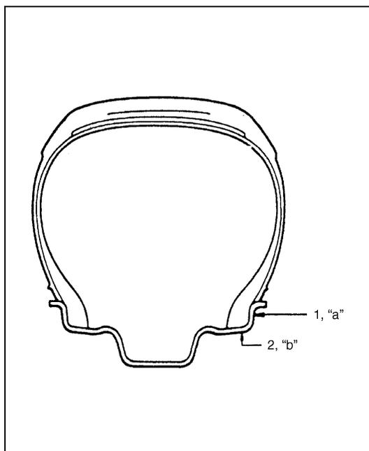
To measure the wheel runout, it is necessary to use accurate dial indicator. The tire may be on or off the wheel. The wheel should be installed to the wheel balancer of the like for proper measurement. Take measurements of both lateral runout (1) and radial runout (2) at both inside and outside of the rim flange. With dial indicator set in place securely, turn the wheel one full revolution slowly and record every reading of the indicator.
