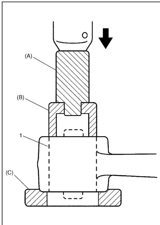
7) Remove bushings (1) by using hydraulic press and special tools.
