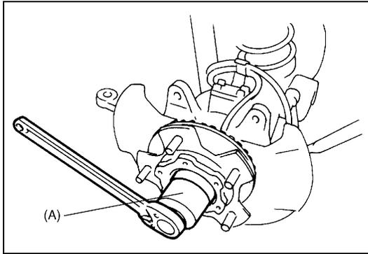
6) Remove front wheel bearing lock nut by using special tool.
