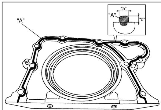
7) Apply sealant to mating surface of rear oil seal housing (1).
