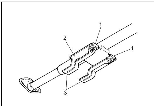
1) Check that two capsules (1) are attached to steering column bracket (2) securely. Check clearance between capsules and steering column bracket. Clearance should be 0.0 mm (0.0 in.) on both sides.
