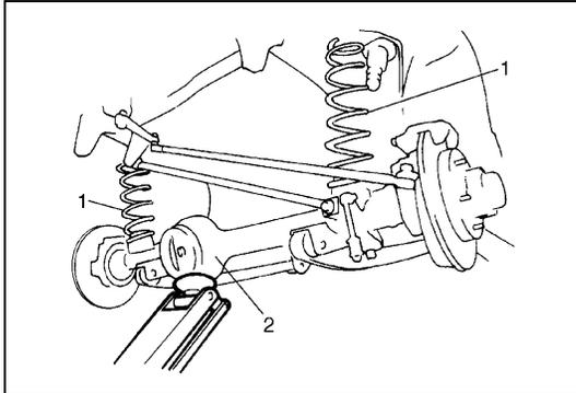
6) Lower front axle housing (2) gradually as far down as where coil spring (1) can be removed.
