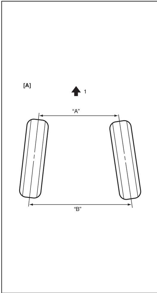
Front alignment refers to the angular relationship between the front wheels, the front suspension attaching parts and the ground. Generally, the only adjustment required for front wheel alignment is toe setting.
