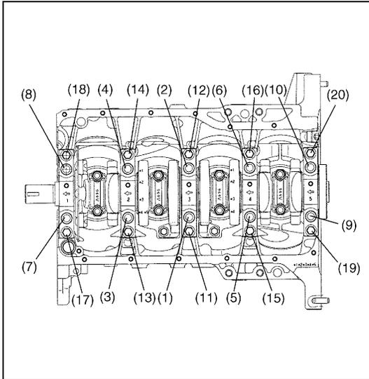
Tighten bearing cap No.1 bolts (1) – (10) and No.2 bolts (11) – (20) gradually as follows.
