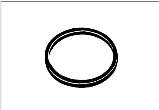
Excessive or uneven wear of pad lining may indicate unsmooth return of the piston. In such a case, replace rubber seal.
