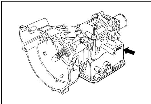
The automatic transmission identification number is located on the transmission case.
