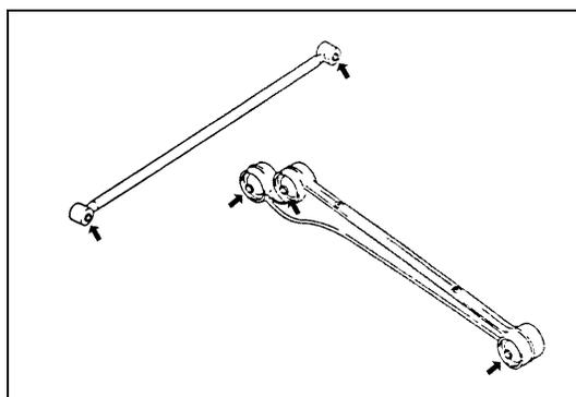
Inspect for wear and breakage. If found defective, replace.
