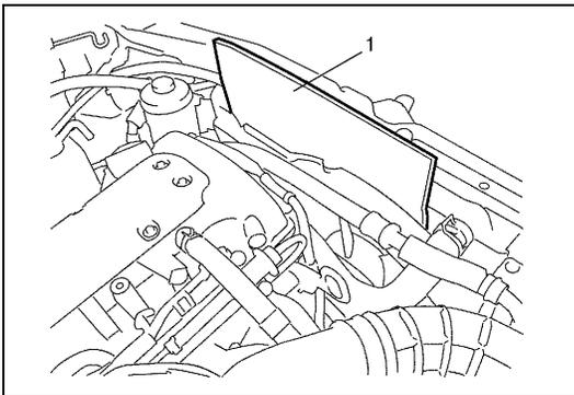
8) Remove fan shroud upper bolts and install board (1) or the like. This prevents damage to radiator fins when removing and installing radiator.
