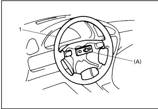
5) Remove steering wheel (1) with special tool.
