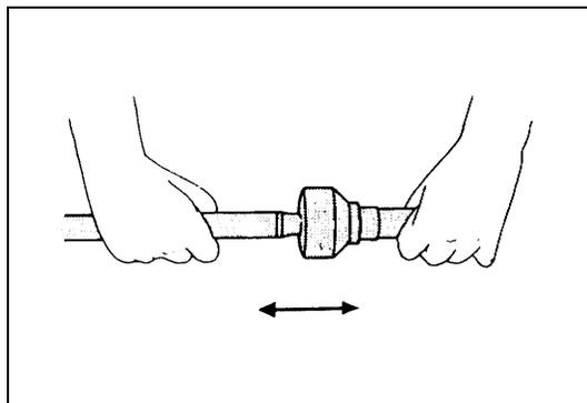
To be checked on this joint is its axial play, which shows up when a push-and-pull motion is given to live axle shaft and wheel spindle held in both hands, as shown in figure. There should be no play at all but a play of up to 1.5 mm (0.06 in.) is permissible. If play exceeds service limit, replace it.
