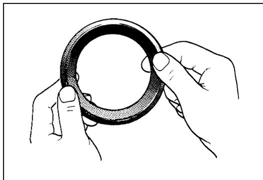
The knuckle seal used at the spherical sliding joint between the knuckle and the inner case accomplishes the additional purposes of keeping out road dust and of acting as the damper for the steering handwheel. As the wear of this seal advances, its damping effect decreases and thus make the front wheel develop a tendency to "shimmy" not only that road dust begins to creep into the sliding clearance to promote the wear of the spherical sliding surfaces.
