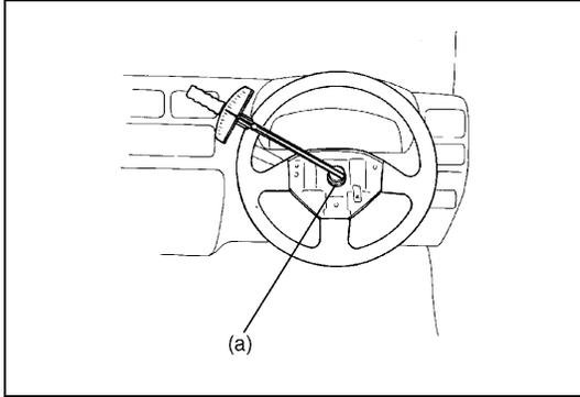
3) Tighten steering shaft nut to specified torque.
