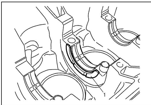
Measure this play with crankshaft set in cylinder block in the normal manner, that is with thrust bearing (1) and journal bearing caps installed.
