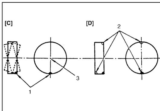
Dynamic balance, as shown in left figure, is equal distribution of weight on each side of wheel centerline so that when the tire spins there is no tendency for the assembly to move from side to side. Wheels that are dynamically unbalanced may cause shimmy.
