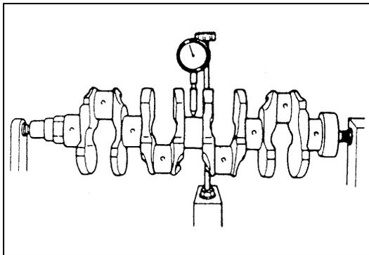
Using a dial gauge, measure runout at center journal. Rotate crankshaft slowly. If runout exceeds its limit, replace crankshaft.
