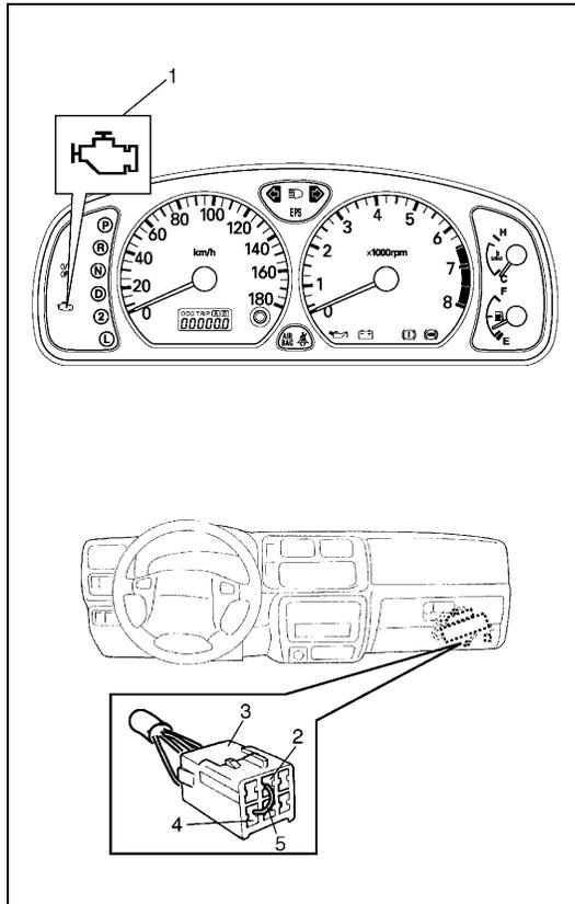
ECM diagnosis troubles which may occur in the area including the following parts when the ignition switch is ON and the engine is running, and indicates the result by turning on or flashing malfunction indicator lamp (1).
