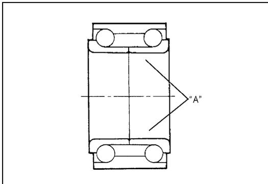
7) Apply lithium grease inside wheel bearing thin.
