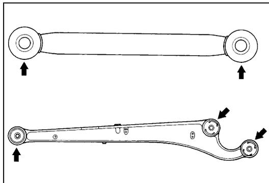
Inspect for damage, wear or deterioration.
