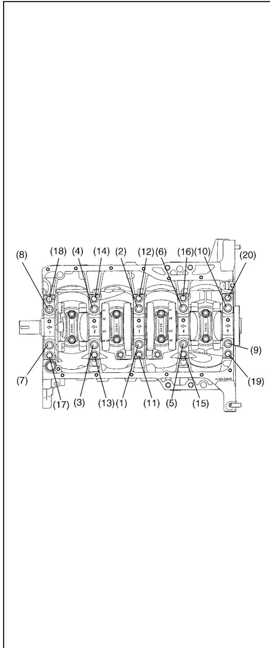
5) Install crankshaft to cylinder block.
