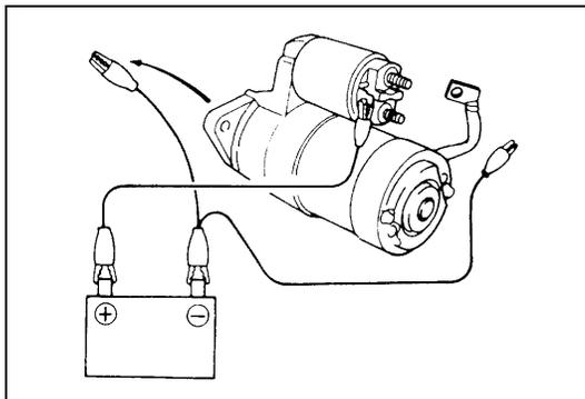
Disconnect negative lead from starting motor body. Check that plunger and pinion return inward. If plunger and pinion don't return, replace magnetic switch.
