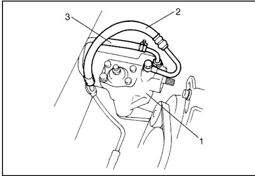
8) Disconnect high pressure hose (2) and return hose (3) from gear box (1).
