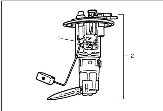
Fuel filter (1) is a part of fuel pump assembly (2) which is installed in fuel tank. Replace fuel filter with new one periodically, referring to “Fuel Pump Assembly (with Fuel Filter, Fuel Level Gauge and Fuel Cut Valve)” in Section 6C for proper procedure.
