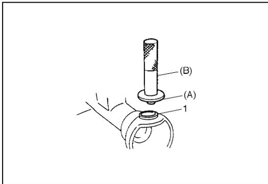
1) Install kingpin bearing outer race (1) to front axle housing by using special tools.
