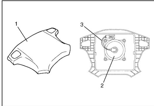
Check air bag (inflator) module visually and if any of the following is found, replace it with a new one.
