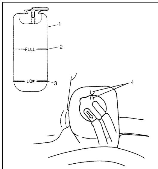
A “see-through” plastic reservoir (1) is connected to the radiator by a hose.
