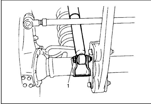
4) Support front axle housing by using floor jack.
