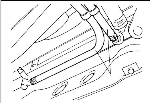
6) Disconnect radiator inlet and outlet hoses from each pipe.
