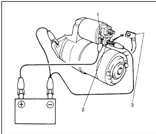
Connect battery to magnetic switch as shown. Check that plunger and pinion move outward. If plunger and pinion don't move, replace magnetic switch.
