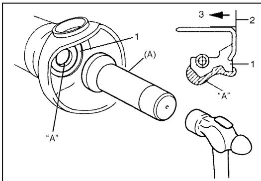
2) Press-fit oil seal (1) until it becomes flush with inner surface of front axle housing (2) by using special tool.
