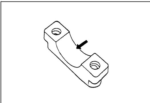
Check clearance by using gauging plastic. Checking procedure is as follows.
