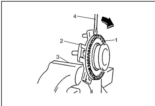
9) Remove sensor rotor from wheel hub as shown (if equipped with ABS).
