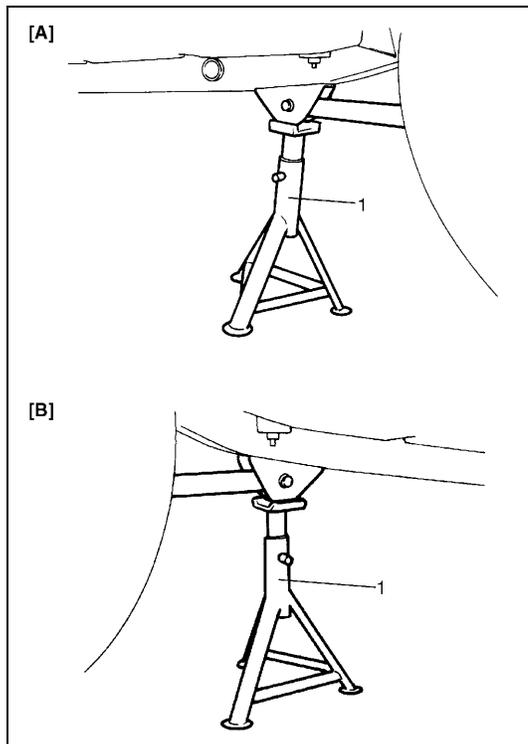
To perform service with either front or rear vehicle end jacked up, be sure to place safety stands (1) under chassis frame so that body is securely supported. And then check to ensure that chassis frame does not slide on safety stands (1) and the vehicle is held stable for safety's sake.
