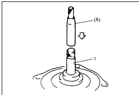
2) Coat special tool surface with compressor oil and place it on compressor shaft (1).
