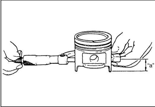
3) Using micrometer, measure piston diameter.
