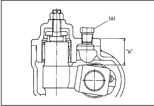
Oil surface should be up to the level as shown in figure. If not, add prescribed gear oil, SAE 90.
