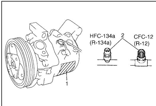
Whether the A/C in the vehicle being serviced uses HFC-134a (R-134a) or CFC-12 (R-12) is indicated on compressor label (1). Also, it can be checked by the shape of the service (charge) valve (2).
