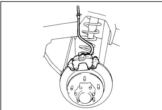
The brake hose assembly should be checked for road hazard damage, for cracks and chafing of the outer cover, for leaks and blisters. A light and mirror may be needed for an adequate inspection. If any of the above conditions are observed on the brake hose, it is necessary to replace it.
