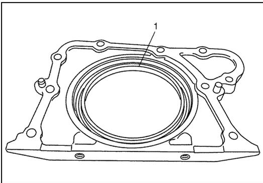
Carefully inspect oil seal (1) for wear or damage. If its lip is worn or damaged, replace it.
