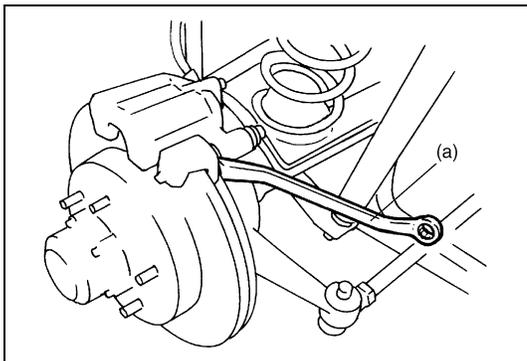
4) Connect stabilizer ball joint to axle housing and tighten nut referring to “Stabilizer Bar” in this section for tightening torque specification.
