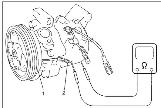
**Magnet Clutch coil resistance**
