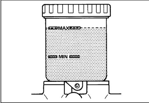
Fluid to fill reservoir with is indicated on reservoir cap of that vehicle with embossed letters or in owner's manual supplied with it. Add fluid up to MAX line.
