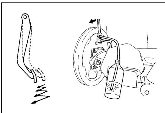
3) Depress brake pedal several times, and then while holding it depressed, loosen bleeder plug about one-third to one-half turn.
