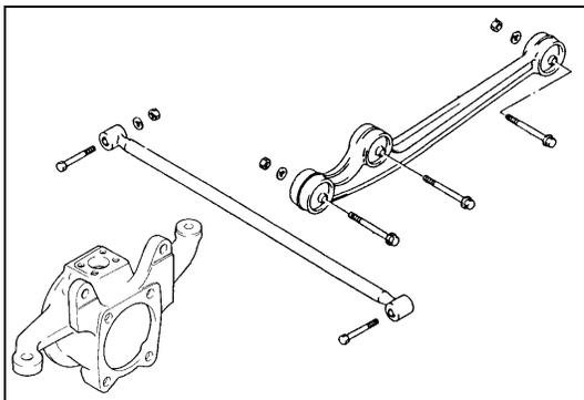
Inspect for cracks, deformation or damage.
