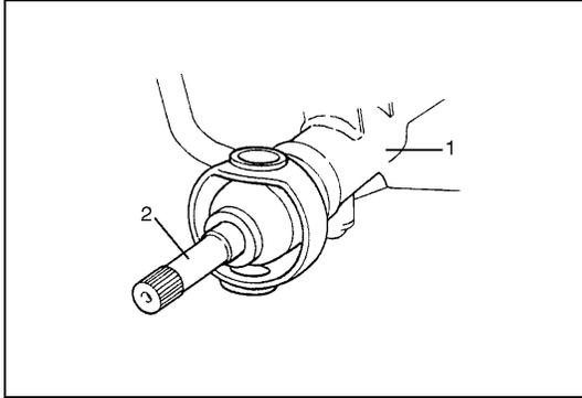
4) Install axle shaft (2) to front axle housing (1) (for 4WD).
