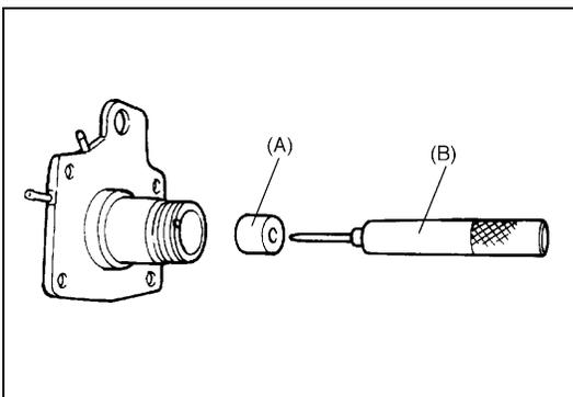
11) Remove spindle bushing by using special tools.
