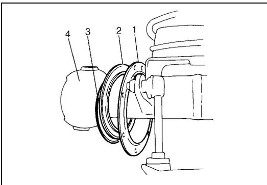
9) Remove knuckle seal cover (1), knuckle seal (2) and knuckle seal retainer (3) from front axle housing (4).
