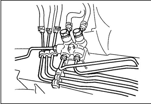
Inspect the tube for damage, cracks, dents and corrosion. If any defect is found, replace it.
