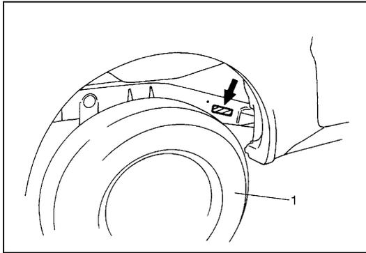
The vehicle body number is punched on the chassis inside the tire housing on the right rear side.
