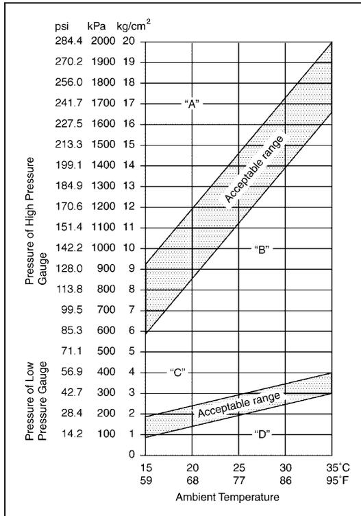
8) Check if each pressure on low side and on high side is within shaded range of the graph.
