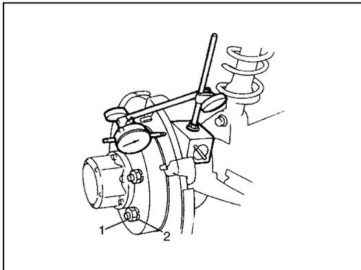
Use wheel nuts (1) and suitable plain washers (2) to hold the disc securely against the hub, then mount a dial indicator as shown and measure the runout at 10 mm (0.39 in.) from the outer edge of the disc.
