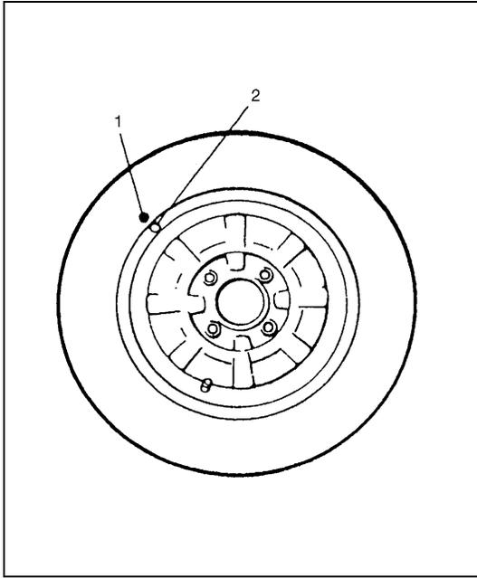
Tires and wheels are matchmounted at the assembly plant.
