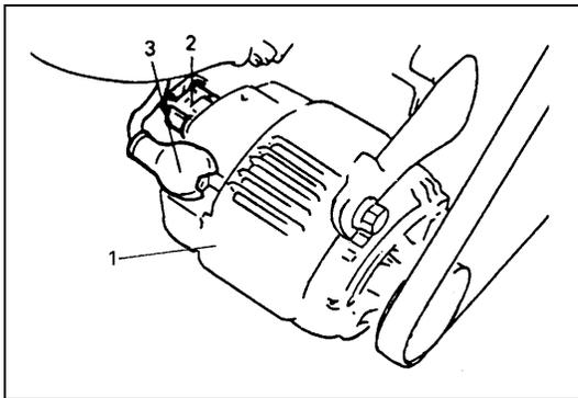
3) Disconnect "B" terminal wire (3) and coupler (2) from generator (1).
