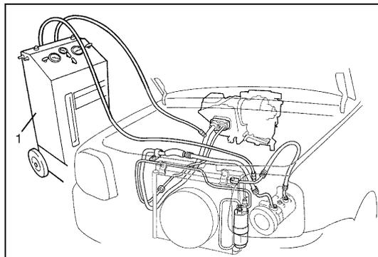
When evacuating A/C system, always recover refrigerant by using equipment (1) for refrigerant recovery and recycling. Discharging refrigerant HFC-134a (R-134a) into atmosphere would cause adverse effect to environments.
