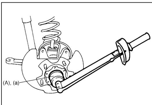
10) Tighten wheel bearing lock nut to specified torque while turning wheel hub by hand.
