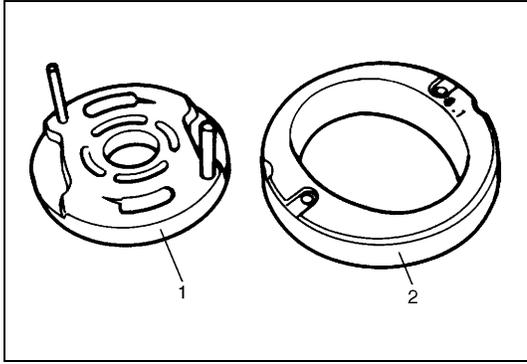
Check vane sliding surface of cam ring (2) for wear and damage. If any defect is found, replace pump assembly.
