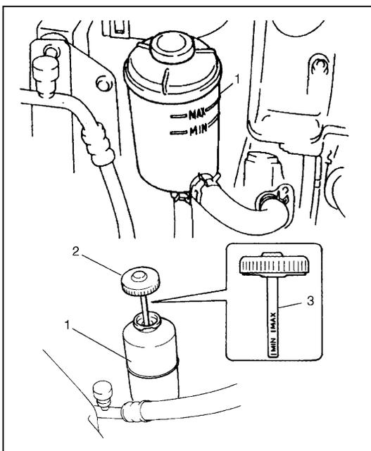
With engine stopped check fluid level indicated on P/S fluid reservoir (1) or level gauge (3), which should be between MAX and MIN marks. If it is lower than lower limit (MIN), replenish fluid up to upper limit (MAX) mark.
