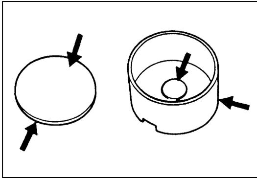
Check tappet and shim for pitting, scratches or damage. If any malcondition is found, replace.
