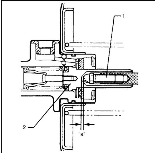
The length of booster piston rod (1) is adjusted to provide specified clearance "a" between piston rod end and master cylinder piston (2).
