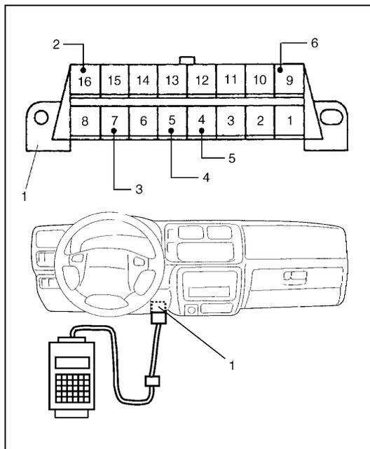
DLC (1) is in compliance with SAEJ1962 in its installation position, the shape of connector and pin assignment. Serial data line (K line of ISO 9141) (3) is used for SUZUKI scan tool or generic scan tool to communicate with ECM, TCM, Air Bag SDM and ABS control module. SUZUKI serial data line (6) is used for SUZUKI scan tool to communicate with immobilizer control module.
