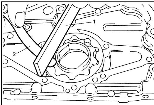
Using straight edge (1) and thickness gauge (2), measure side clearance.
