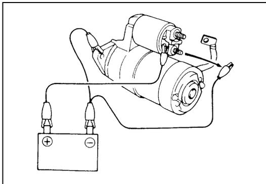
While connected as above with plunger out, disconnect negative lead from terminal "M". Check that plunger and pinion remain out. If plunger and pinion return inward, replace magnetic switch.
