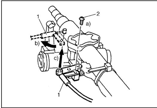
8) If equipped with shift (key) interlock cable (1), remove shift (key) interlock cable screw (2) and then disconnect its cable from ignition switch in order a) – c) as shown in the figure.
