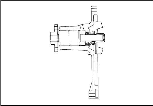
The centrifugal type water pump is used in the cooling system. The pump impeller is supported by a totally sealed bearing. The water pump can not be disassembled.
