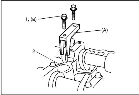
2) Lift valve by turning crankshaft and then remove camshaft housing bolts (1) where the shim to be replaced.
