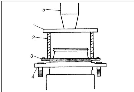
6) Install sensor rotor (3) as shown (if equipped with ABS).
