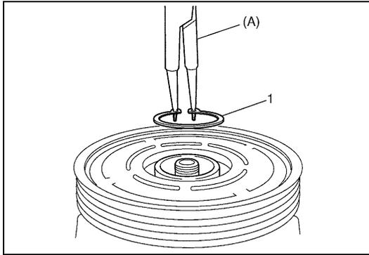
4) Remove circlip (1) using special tool.
