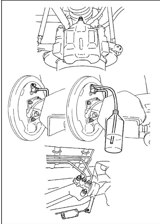
Bleeding operation is necessary to remove air whenever it entered hydraulic brake system.
