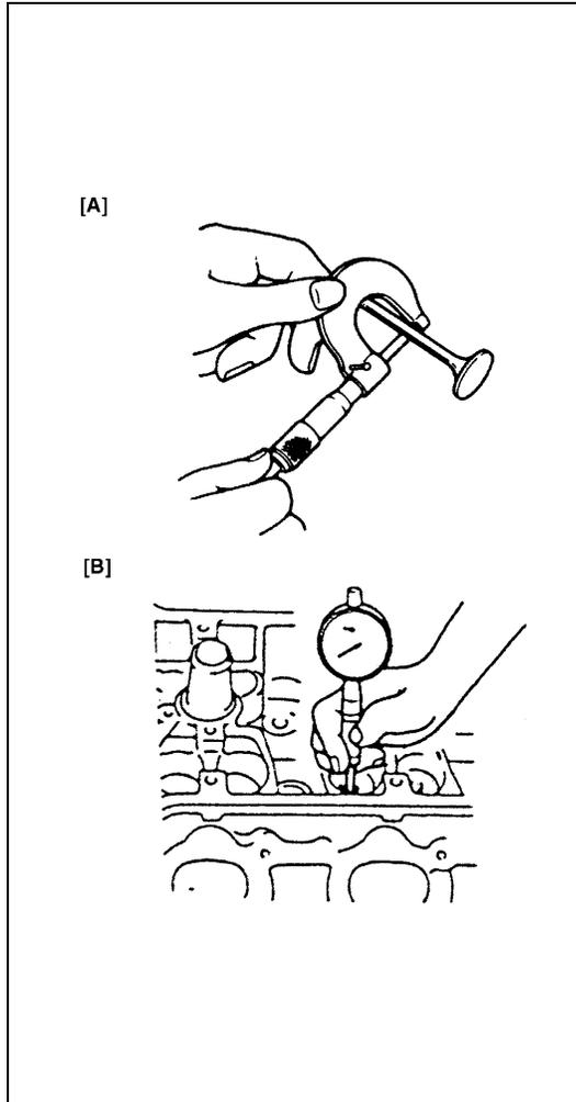
Using a micrometer and bore gauge, take diameter readings on valve stems and guides to check stem-to-guide clearance. Be sure to take reading at more than one place along the length of each stem and guide.
