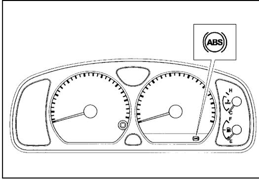
Turn ignition switch ON and check that “ABS” warning lamp comes ON for about 2 seconds and then goes OFF. If any faulty condition is found, advance to Diagnostic Flow Table-A, B or C.
