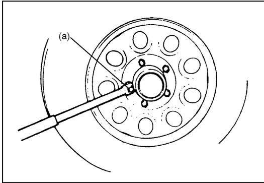
5) Install wheel and tighten wheel nuts to specified torque.
