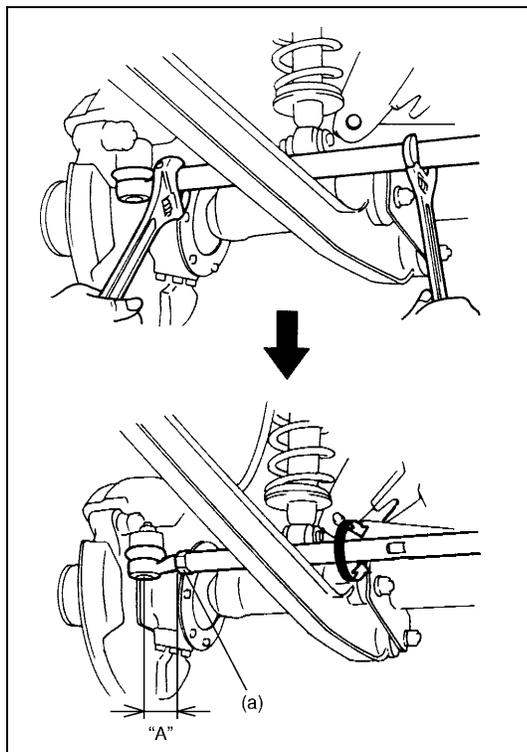
Toe is adjusted by changing tie rod length. Loosen right and left tie rod end lock nuts first and then rotate tie rod to align toe-in to specification.
