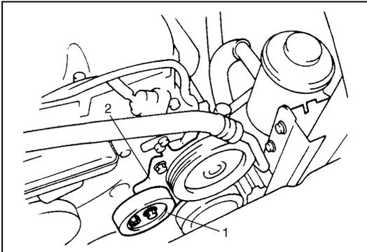
10) Remove A/C compressor and/or P/S pump belt tension pulley (1) (if equipped).
