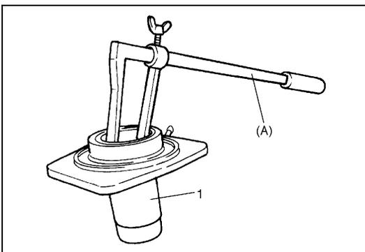
10) Remove spindle oil seal by using special tool.
