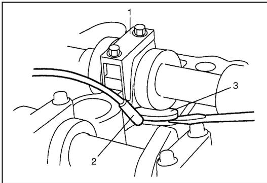
4) Turn camshaft by approximately 90° clockwise and remove shim (3).
