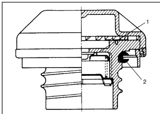
The fuel tank filler neck has a vacuum cap.
