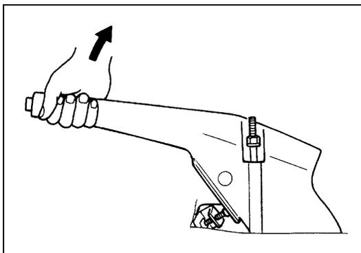
Hold center of parking brake lever grip and pull it up with 20 kg (44 lbs) force.
