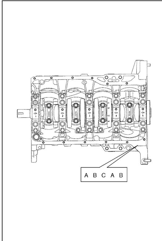
2) Next, check bearing cap bore diameter without bearing. On mating surface of cylinder block, five alphabets are stamped as shown in figure.
