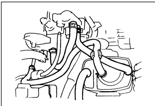
Check hoses for connection, leakage, clog and deterioration. Replace as necessary.
