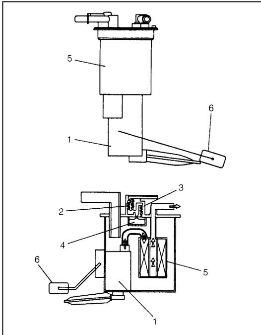
An in-tank type electric pump has been adopted for the fuel pump (1). Incorporated in the pump assembly are;
