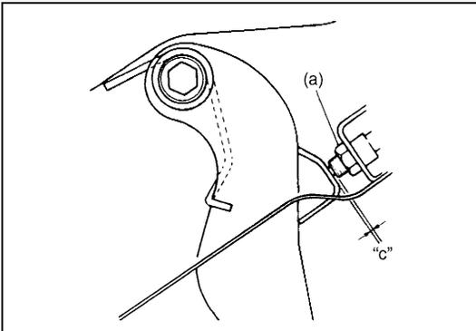
Adjustment should be made as follows when installing switch. Pull up brake pedal toward you and while holding it there, adjust switch position so that clearance between end of thread and brake pedal is specified. Then tighten lock nut to specified torque.
