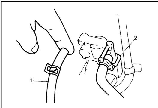
Start engine and run it at idle speed. Disconnect vacuum hose (1) from EVAP canister purge valve (2). With finger placed against hose disconnected, check that vacuum is applied.
