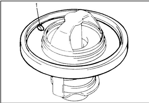
A wax pellet type thermostat is used in the cooling system. The temperature at which the valve begins to open is stamped on thermostat. In the top portion of the thermostat, an air bleed valve (1) is provided; this valve is for venting out the gas or air, if any, that is accumulated in the circuit.
