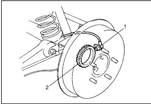
5) Remove rear wheel speed sensor (1) from rear axle housing.
