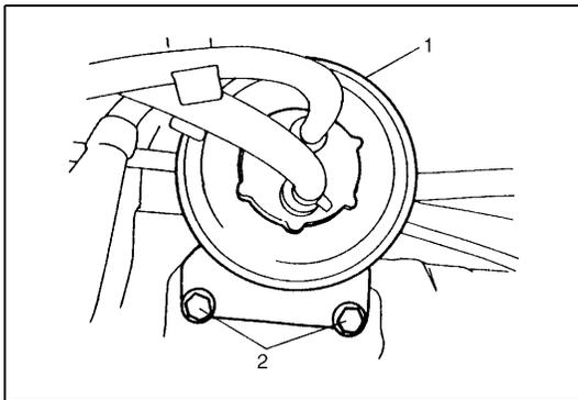
2) Remove bolts (2) and then canister (1) together with its bracket.
