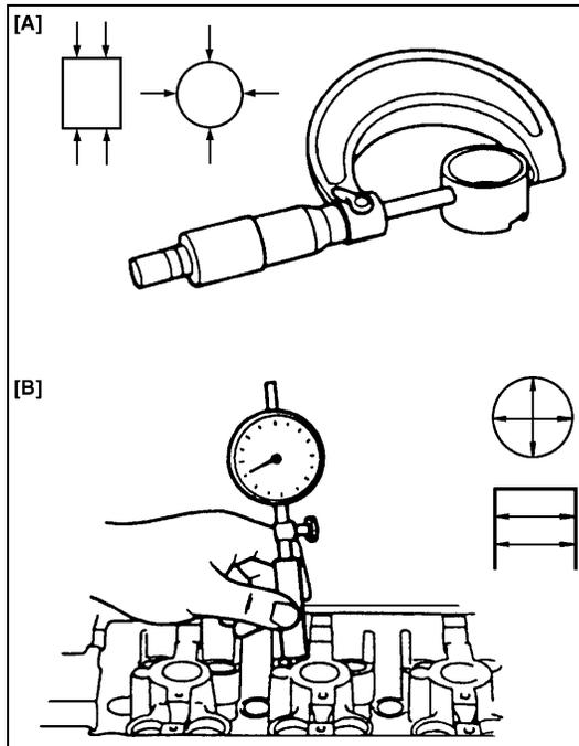
Measure cylinder head bore and tappet outside diameter to determine cylinder head-to-tappet clearance. If clearance exceeds limit, replace tappet or cylinder head.
