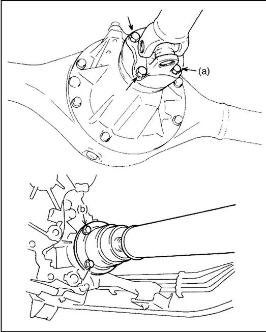
Install propeller shaft(s) reversing removal procedure noting following points :
