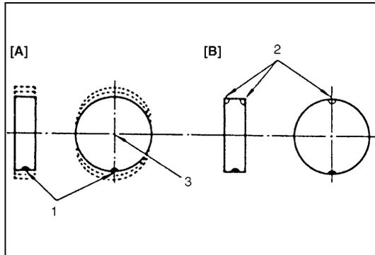
There are two types of wheel and tire balance: static and dynamic. Static balance, as shown in figure, is equal distribution of weight around wheel. Wheels that are statically unbalanced cause bouncing action called tramp. This condition will eventually cause uneven tire wear.
