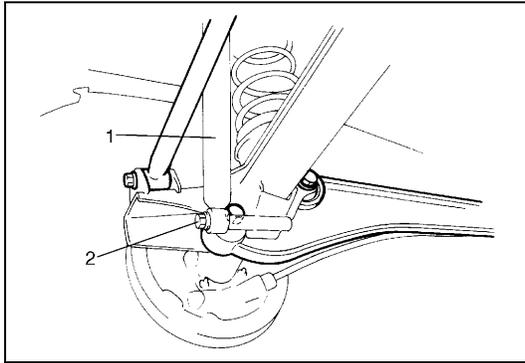
4) Remove shock absorber lower mounting bolt (2).
