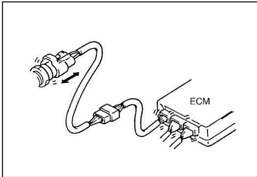
When checking system circuits including an electronic control unit such as ECM, TCM, ABS control module, etc., it is important to perform careful check, starting with items which are easier to check.
