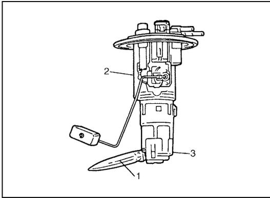
Check fuel pump assembly for damage.
