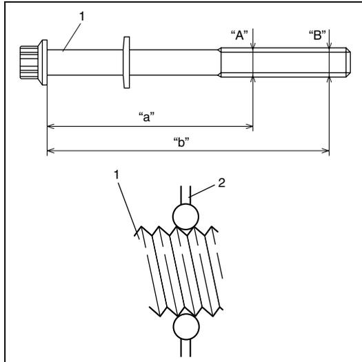
Measure each thread diameter of bearing cap No.1 bolts (1) at "A" on 60 mm (2.36 in.) from seat side of flange bolt and "B" on 90 mm (3.54 in.) from seat side of flange bolt by using a micrometer (2).
