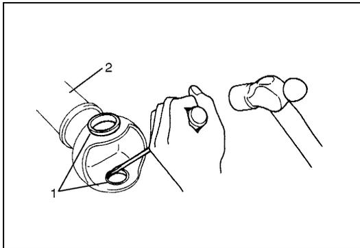
6) Drain out kingpin bearing outer race (1) from front axle housing (2).
