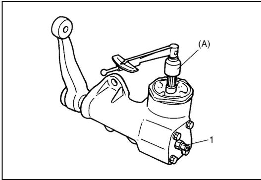
Steering gear box has adjusting bolt (1) which gives preload to sector shaft.
